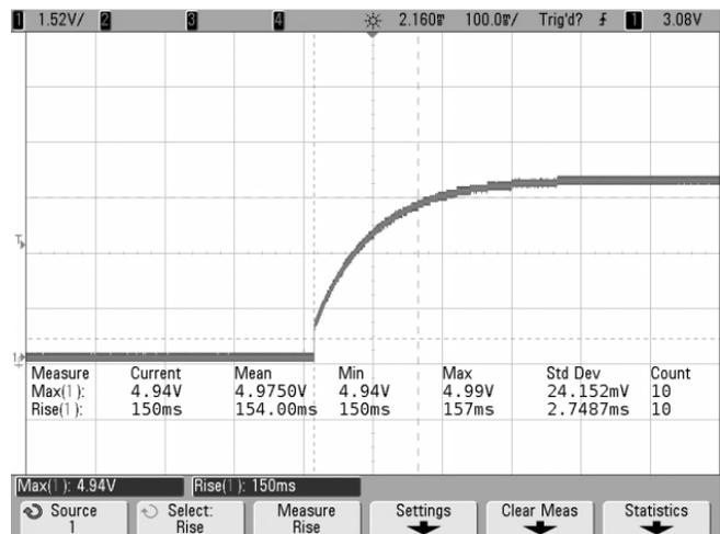
**Figure 11. Tau = 100 ms; Measured  $T_{RISE} = 153$  ms**
