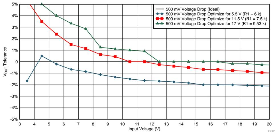
**Figure 5. Output Voltage Tolerance at  $500 mV_{DROP}$  versus Input Voltage**
