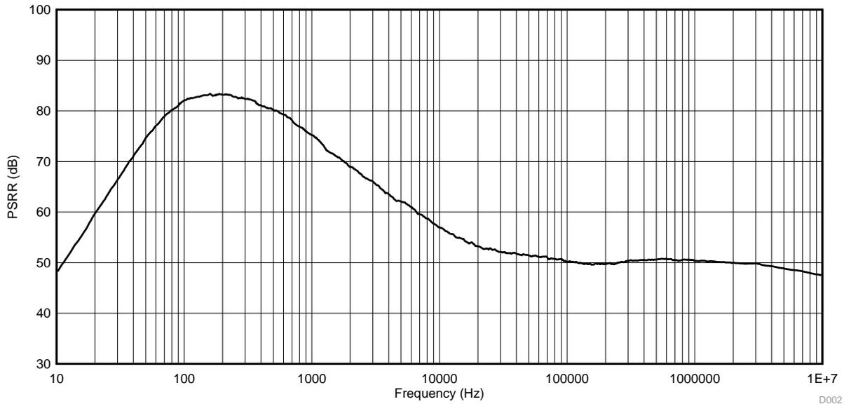
**Figure 4. Frequency versus PSRR**
