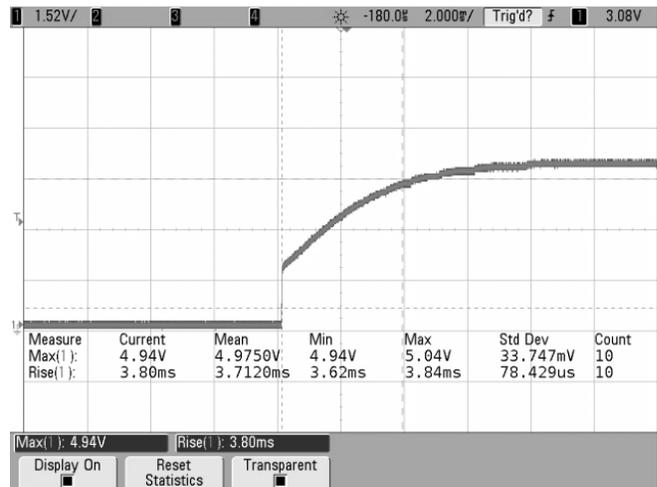
**Figure 9. Tau = 1 ms; Measured  $T_{RISE} = 3.80$  ms**
