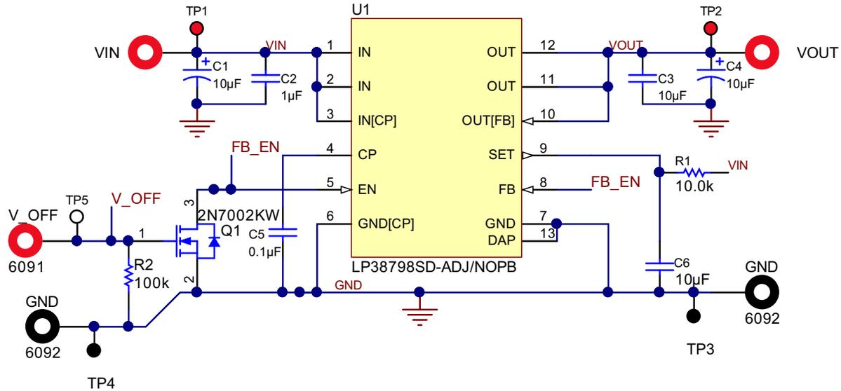
Figure 14. TIDA-00533 Schematic
