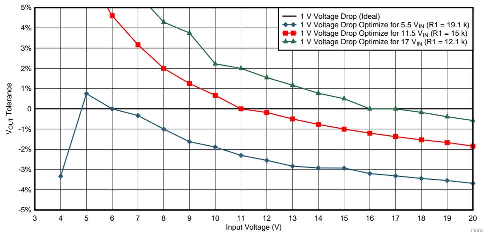
**Figure 6. Output Voltage Tolerance at  $1 V_{DROP}$  versus Input Voltage**
