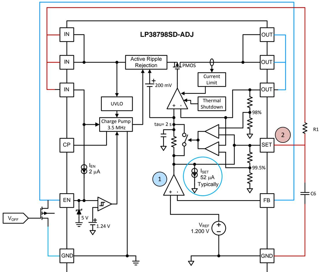
Figure 2. LP38798SD-ADJ Functional Block Diagram
