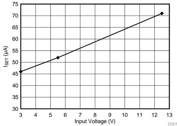
**Figure 3.  $I_{SET}$  versus Input Voltage**
