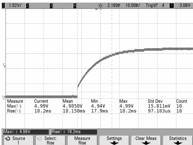
**Figure 10. Tau = 10 ms; Measured  $T_{RISE} = 18.2$  ms**
