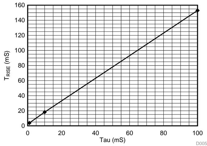
**Figure 7. Output Voltage Rise Time ( $T_{RISE}$ ) versus RC Time Constant ( $\tau$ )**
