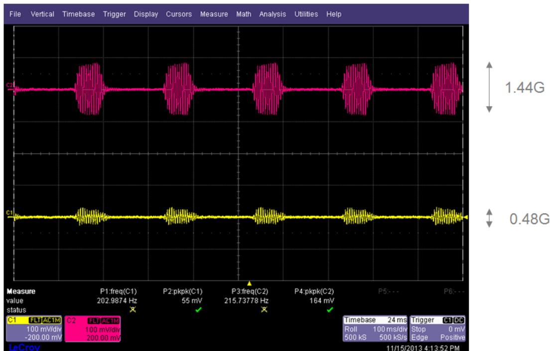
Figure 23. Acceleration Measurements for Piezos—Top Placement
