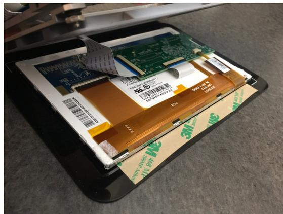
**Figure 42. Tape on Backside of Touch Screen**
