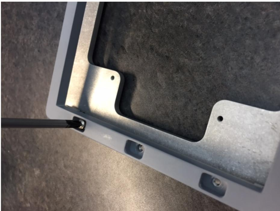
Figure 38. Securing Plastic Touch Screen Frame to Bracket
