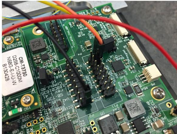
**Figure 49. I<sup>2</sup>C and Ground Connections**
