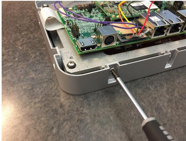
**Figure 45. Secure Chassis to Carrier Frame**
