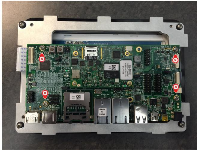
Figure 43. Motherboard and Carrier Frame Screw Locations
