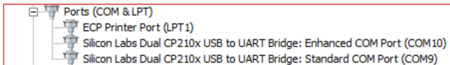
**Figure 4. 66AK2L06 EVM Virtual COM Ports**
