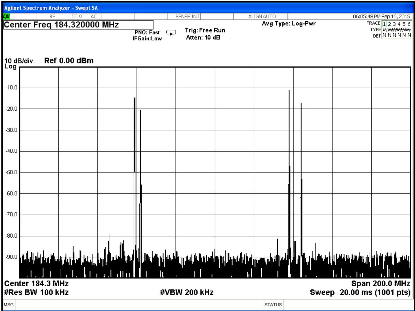
Figure 25. DAC Output – 2x75 MHz 2-Tone Data
