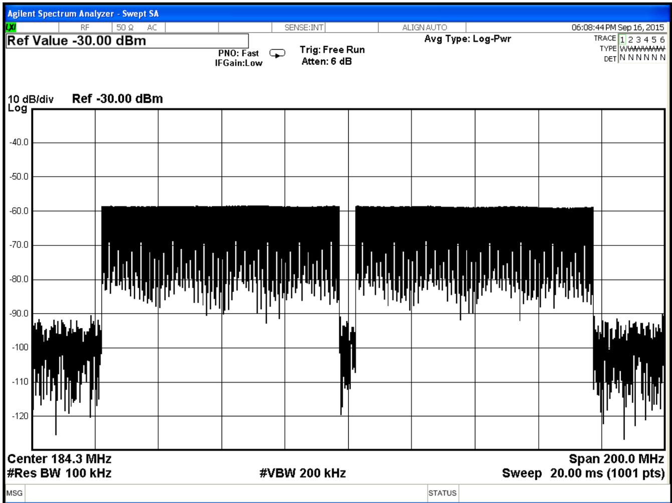
Figure 26. DAC Output -- 2x75 MHz Multi-Tone Data
