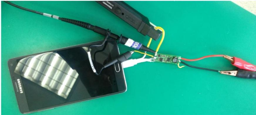
**Figure 12 Setup to Charge a Mobile Phone**
