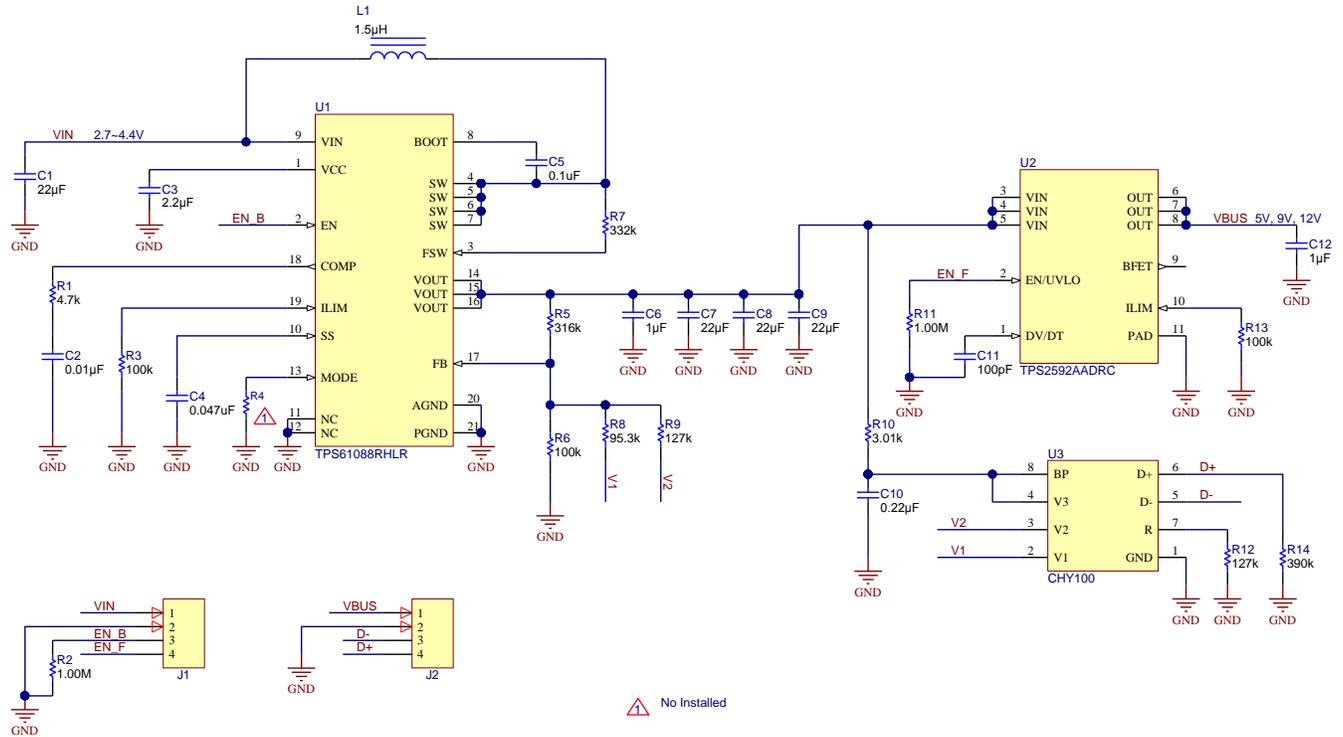
Figure 14 PMP9773 Schematic
