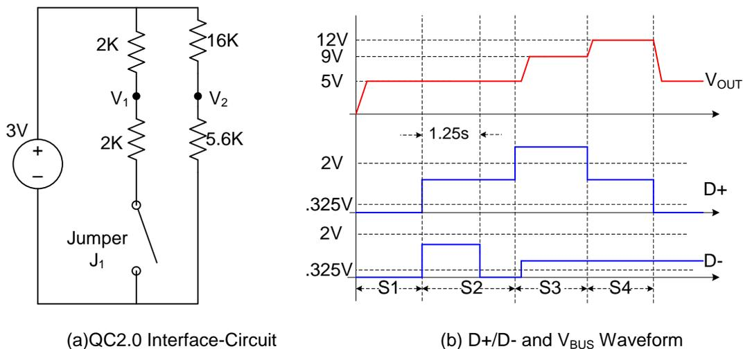
**Figure 3 An Interface-Circuit to Enter Quick Charge 2.0**
