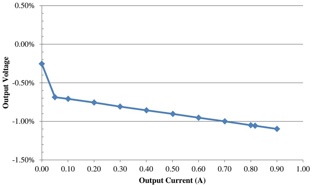
**Figure 17 Output regulation of MGTAVCC 1V output**
