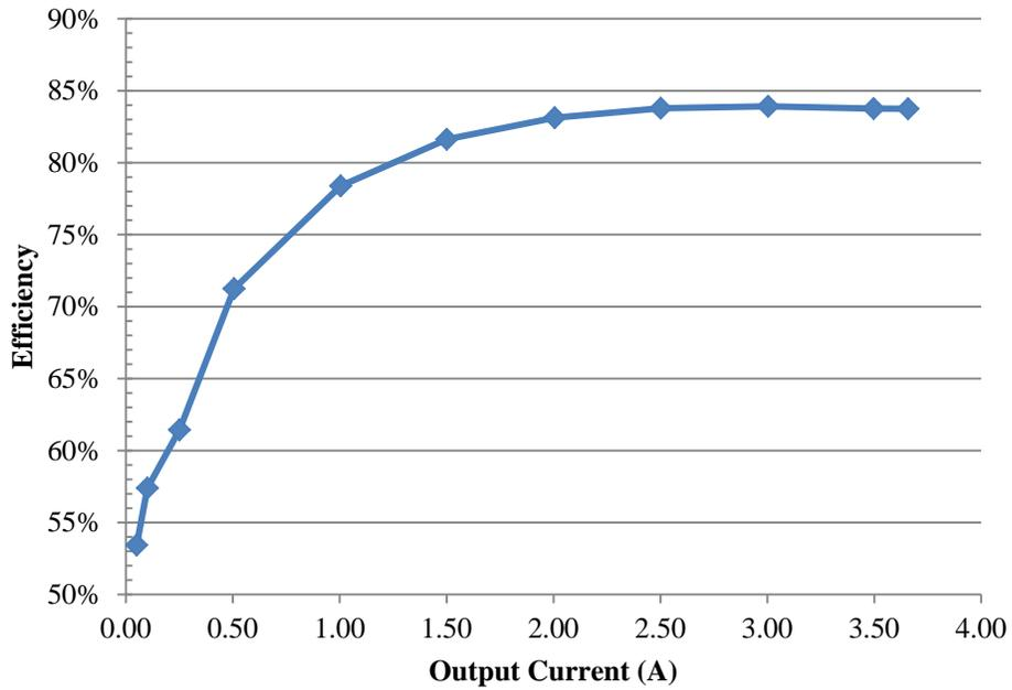
**Figure 11 Power efficiency of VCCINT 0.9V output**
