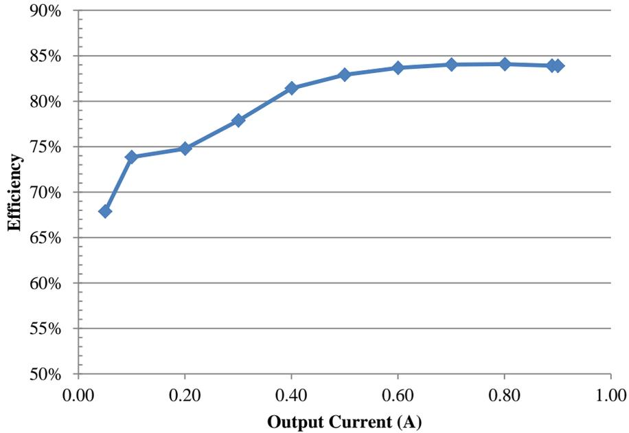
**Figure 13 Power efficiency of VCCAUX 1.8V output**
