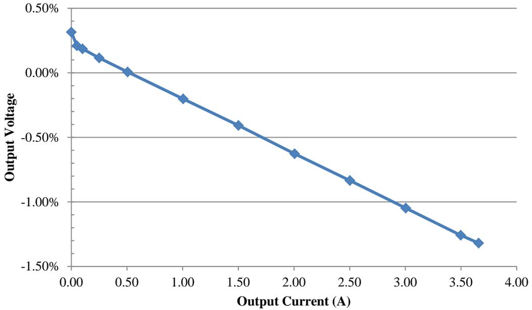
**Figure 16 Output regulation of VCCINT 0.9V output**
