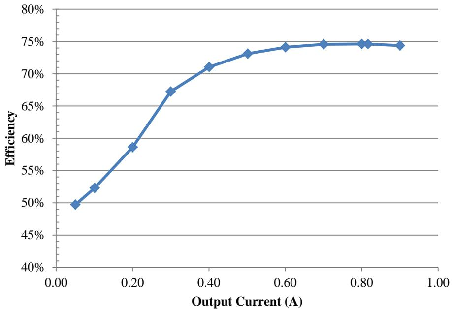
**Figure 12 Power efficiency of MGTAVCC 1V output**
