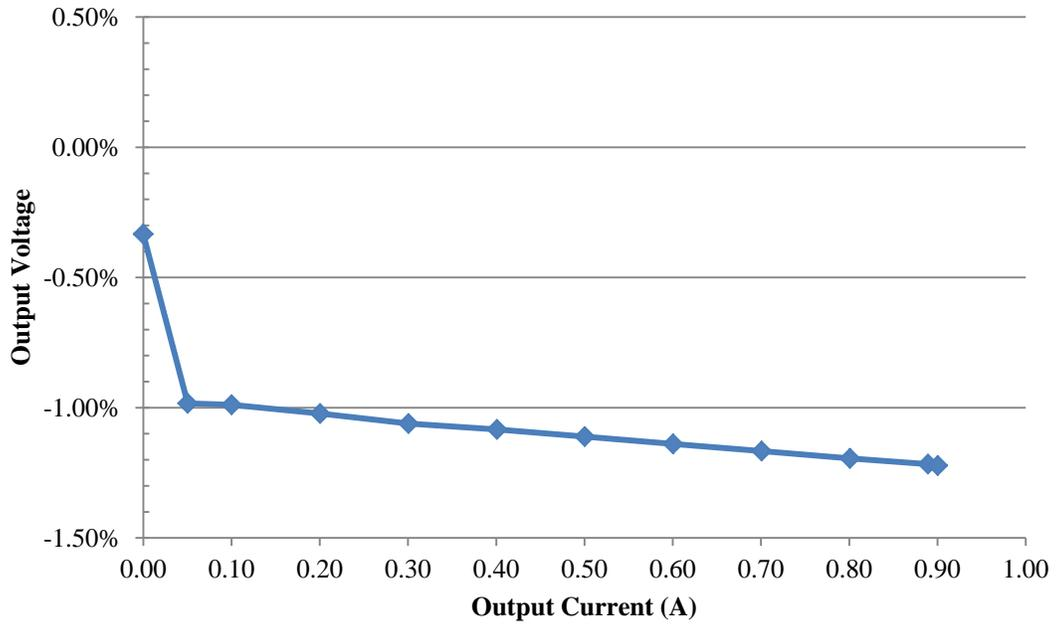
Figure 18 Output regulation of VCCAUX 1.8V output
