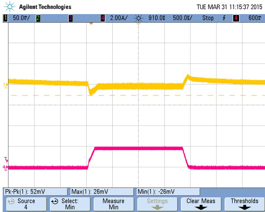
Figure 19 Output load transient of VCCINT 0.9V output
