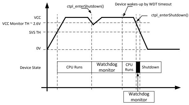
Figure 5. Power-Up and Down Conditions
