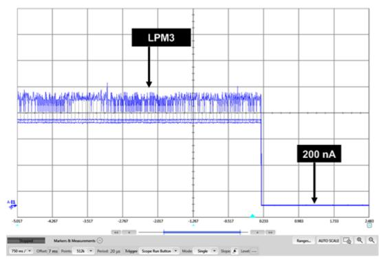
Figure 10. CTPL Enters Shutdown or LPM4.5 with Interrupts Disabled
