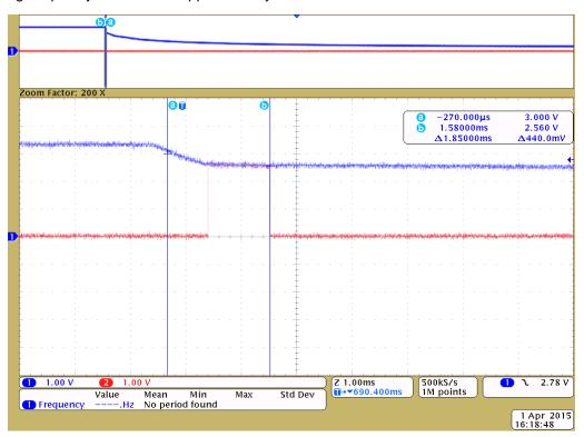
Figure 3. VCC Drop When Micro-USB is Disconnected
