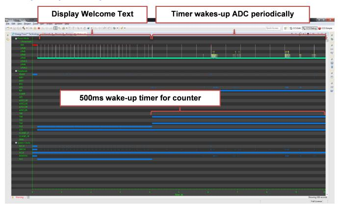
Figure 7. EnergyTrace++ Capture on Reset
