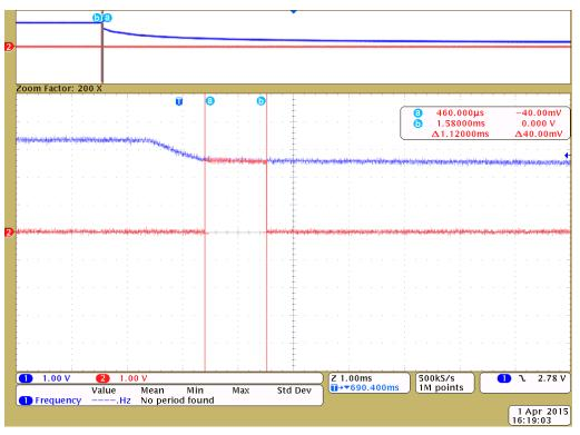
Figure 4. Ctpl\_enterShutdown() Execution Time at 1 MHz
