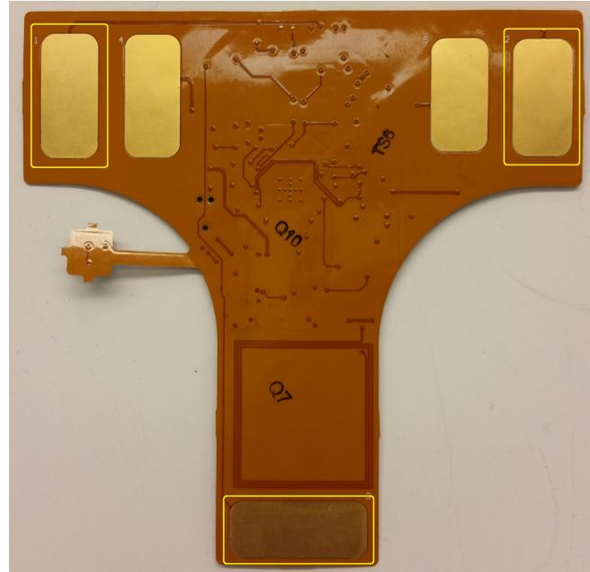
**Figure 9. ECG Subcircuit—Probes System Back Location**
