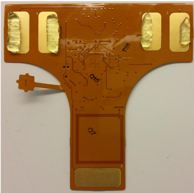
Figure 28. Conductive Gel Application
