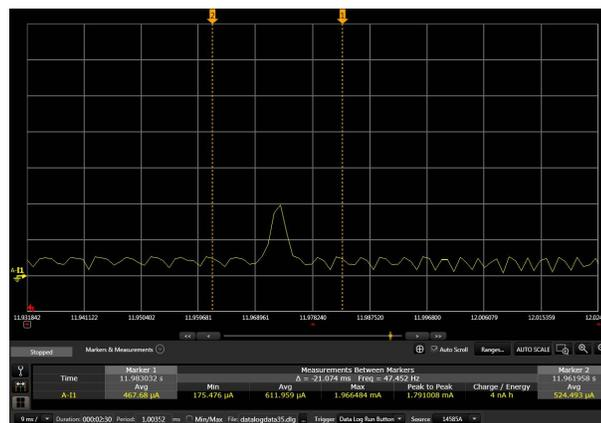
Figure 64. TSM Power Down State—Disable TMP112A Stage
