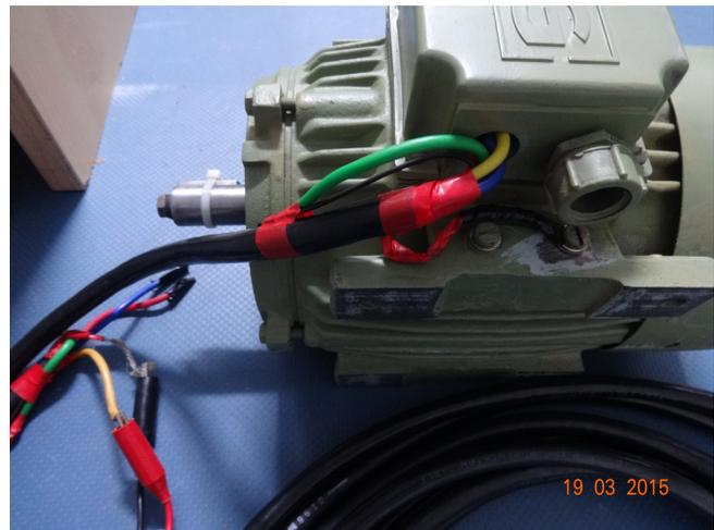
Figure 52. Zoomed-In Photo of of Motor Used for Testing TIDA-00440
