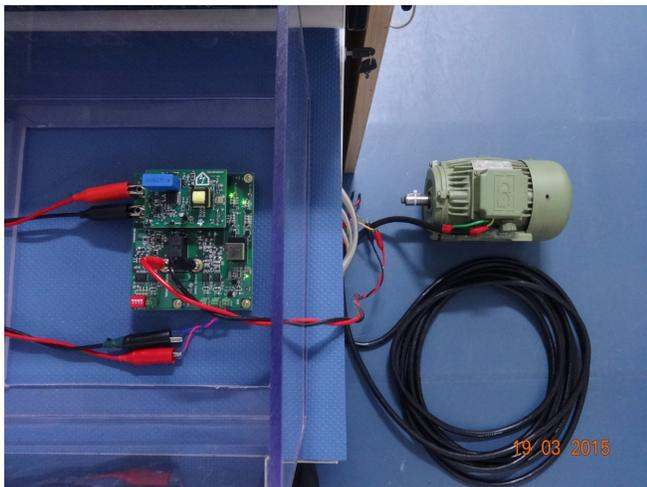
Figure 51. Motor Used for Testing TIDA-00440
