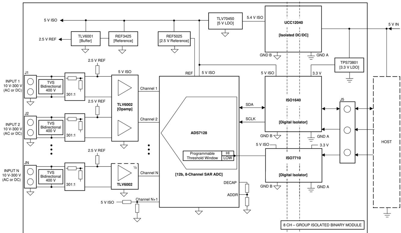
Figure 2-2. Block Diagram of ADC-based BIM Design (ADS7128)
