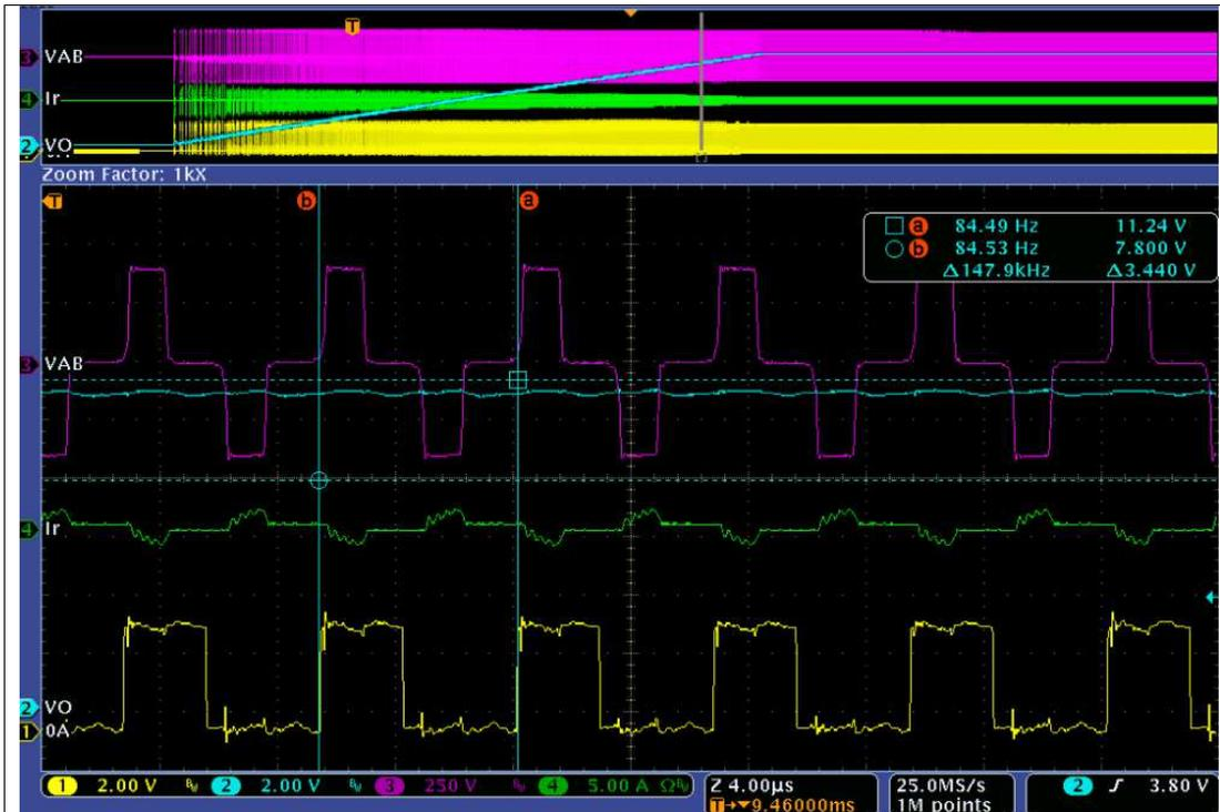
Phase shift mode in low output voltage.  $V_{in}=380V_{dc}$ ,  $V_o=12V$ ,  $I_o=10A$
