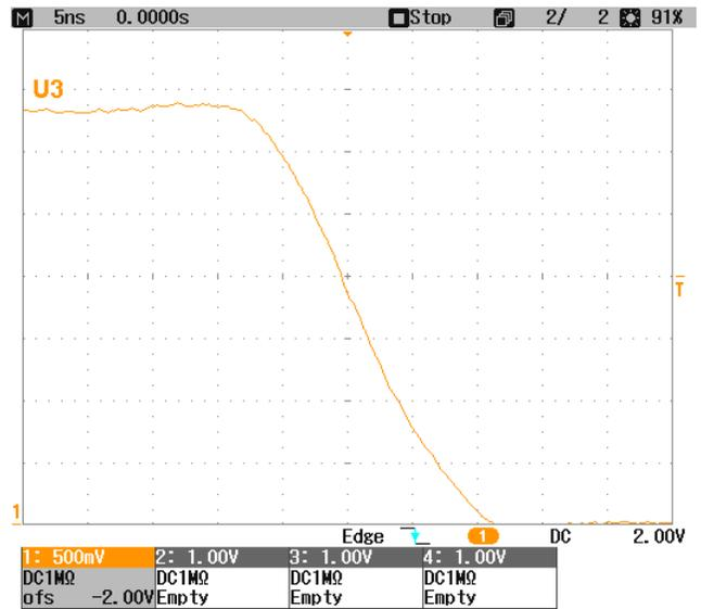
**Hall sensor pulldown (open-drain output)**
