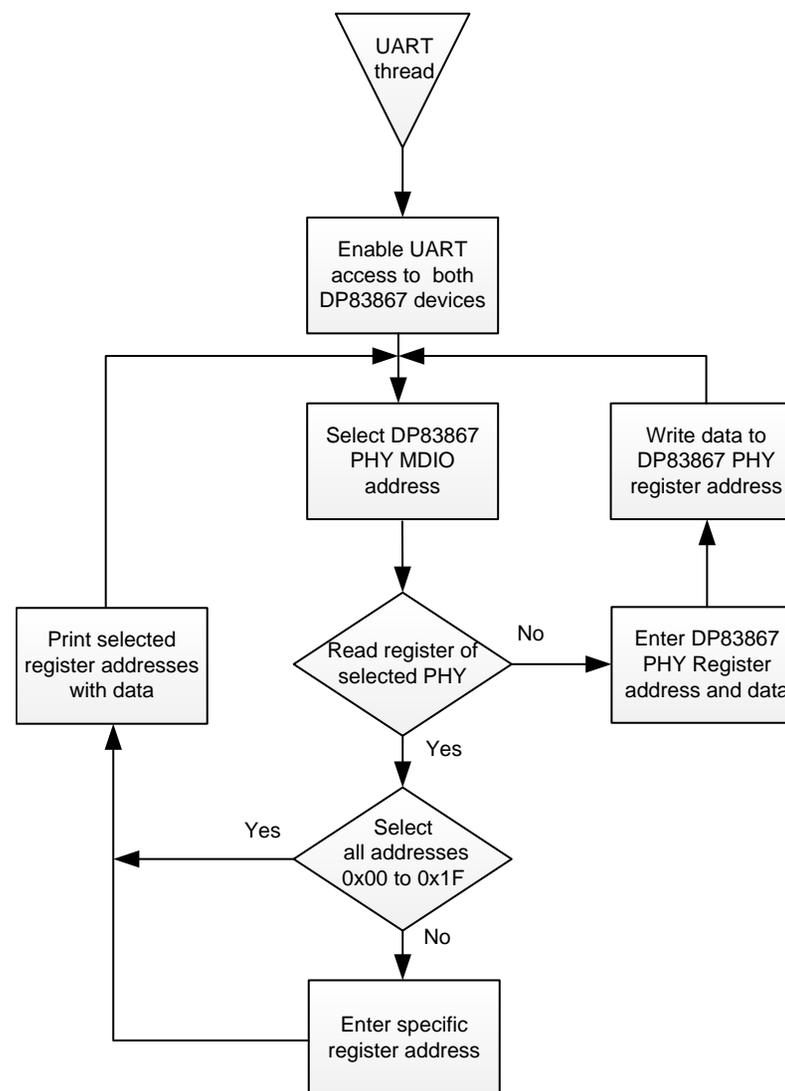
Figure 24. AM3359 UART Thread Flowchart
