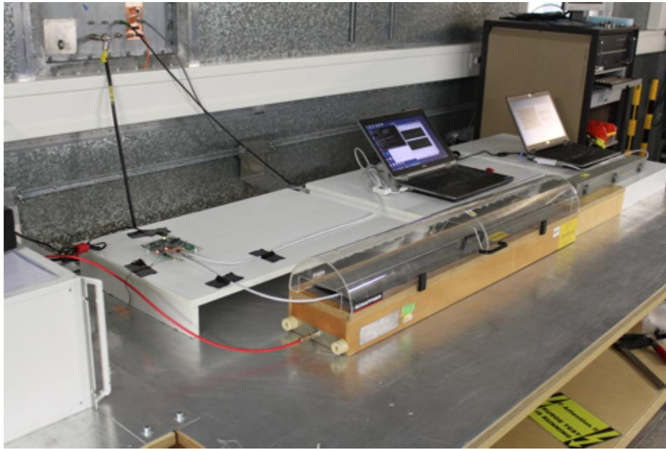
**Figure 64. IEC61000-4-4 EFT Test Setup for TIDA-00204**
