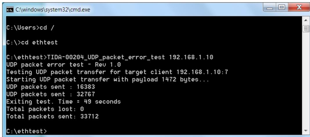
Figure 29. Command Prompt UDP Packet Error Test Print
