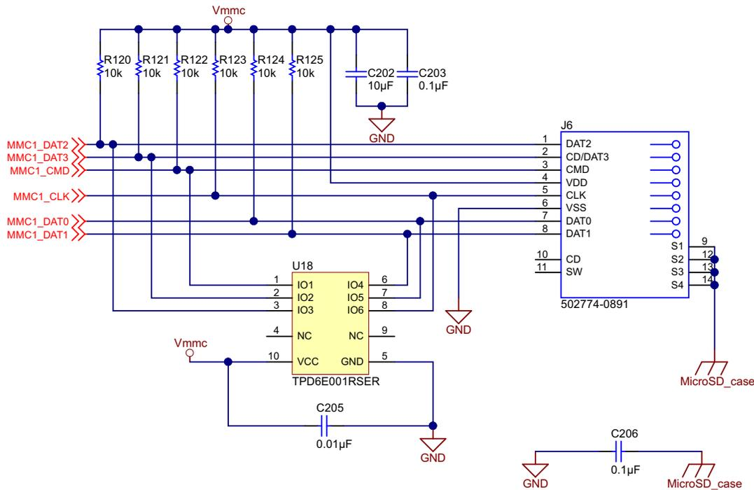
Figure 10. MMC1 Micro SD-Card Interface With ESD Protection
