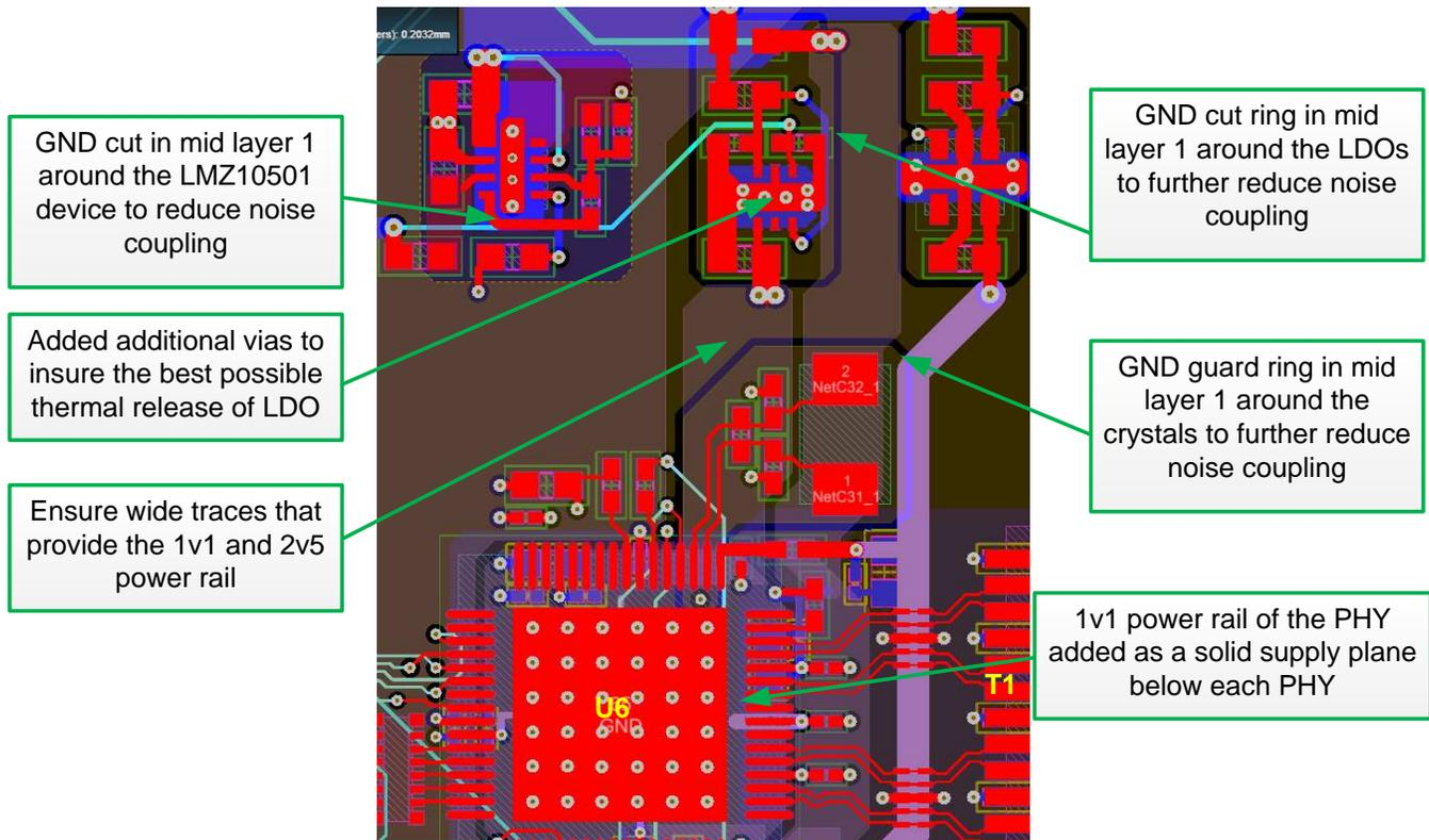
Figure 74. Layout Guidelines for PHY Power Supply
