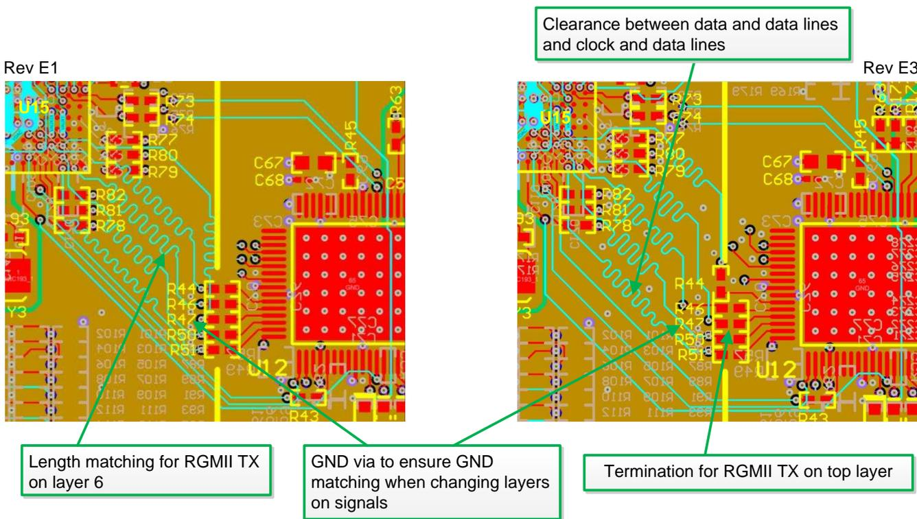
Figure 71. Layout Guidelines for RGMII TX Signals Comparing E1 and E3
