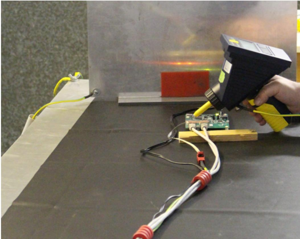
**Figure 62. IEC61000-4-2 Test Setup for TIDA-00204 (Picture of 6-kV CD)**
