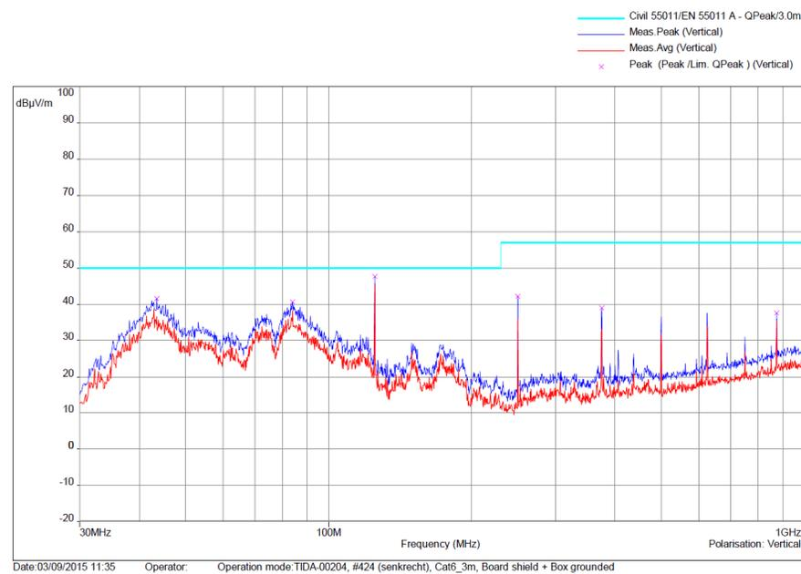
**Figure 61. Measured EMI Spectrum According to EN55011;
