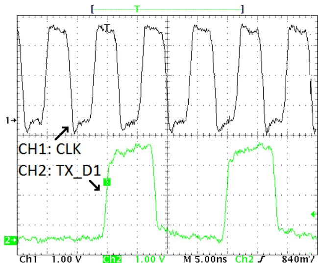
**Figure 40. ETH1 RGMII TX Clock and Data During Gigabit Ethernet Connection**
