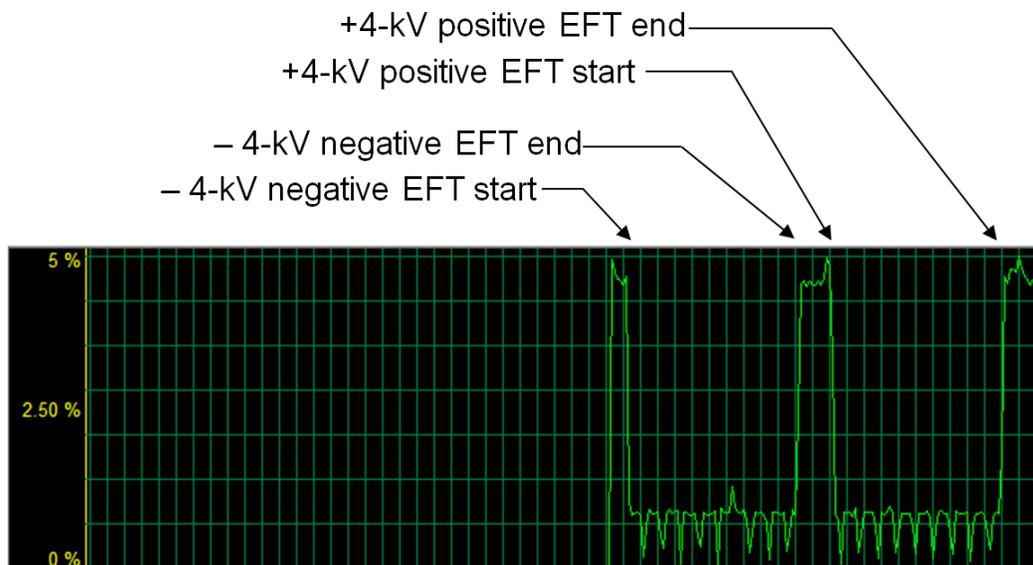
Figure 66. IEC61000-4-4 ±4-kV EFT: Network Utilization With UDP Packet Error Test on Gigabit Ethernet Port 1
