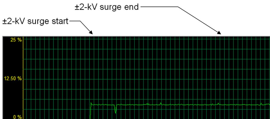
**Figure 68. IEC61000-4-5 ±2-kV Surge: Network Utilization With UDP Packet Error Test on Gigabit Ethernet Port 1**
