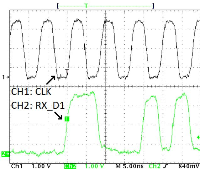
**Figure 39. ETH1 RGMII RX Clock and Data Signal During Gigabit Ethernet Connection**
