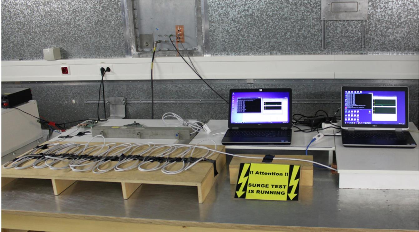
Figure 67. IEC61000-4-5 Surge Test Setup for TIDA-00204
