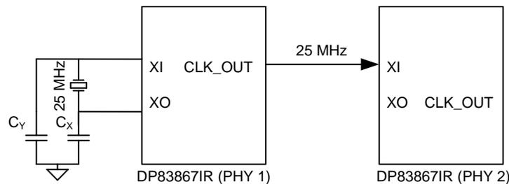
**Figure 16. Crystal Configuration for DP838671R and Option to Clock the Second DP838671R PHY From the First DP838671R**
