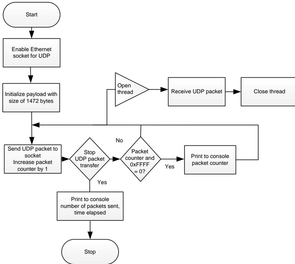
Figure 26. Flowchart of UDP Throughput Test Software
