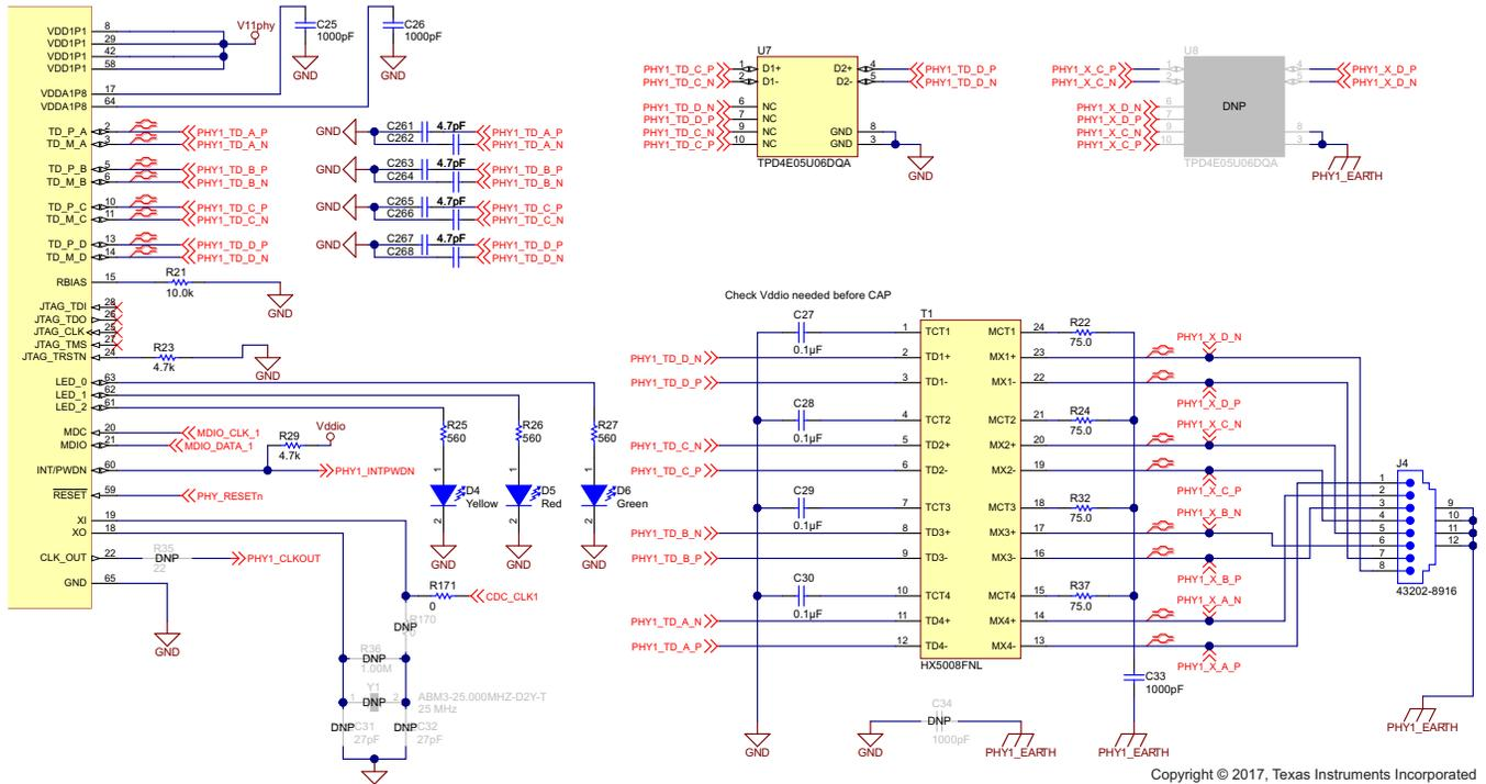
Figure 7. Schematic of Media Dependent Interface of ETH1
