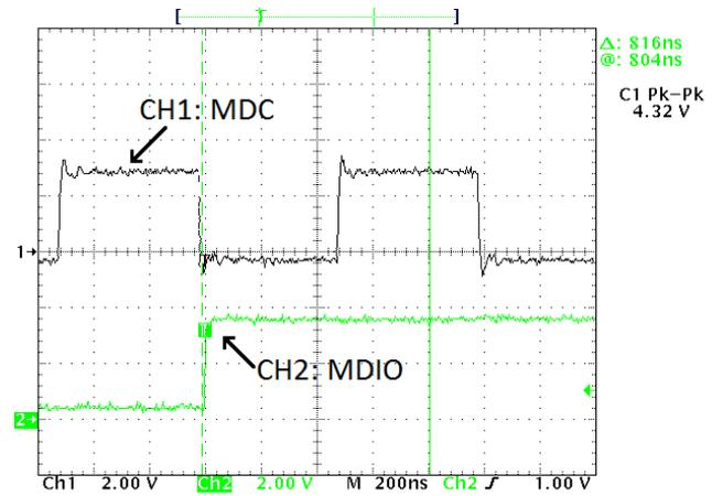
Figure 44. SMI Clock and Data Signal at 2.5 MHz at DP83867IR ETH2
