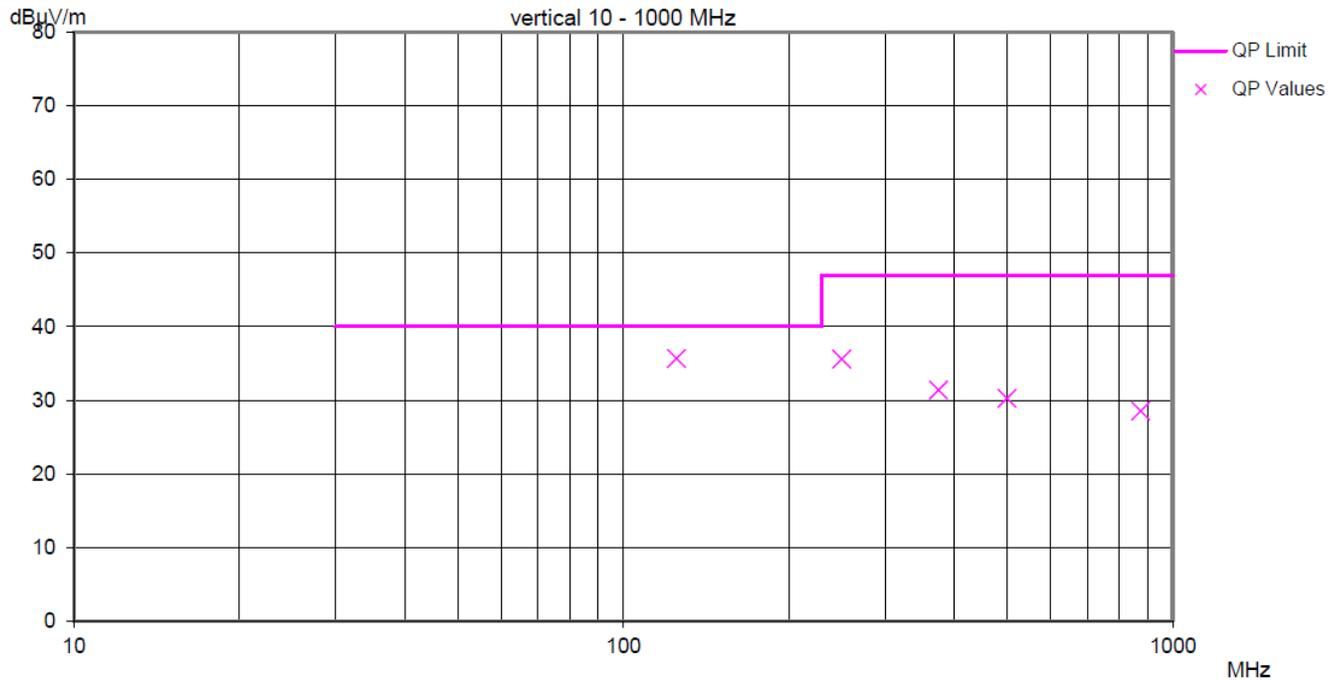
**Figure 58. Measured EMI Spectrum (Quasi-Peak) According to EN55011;
