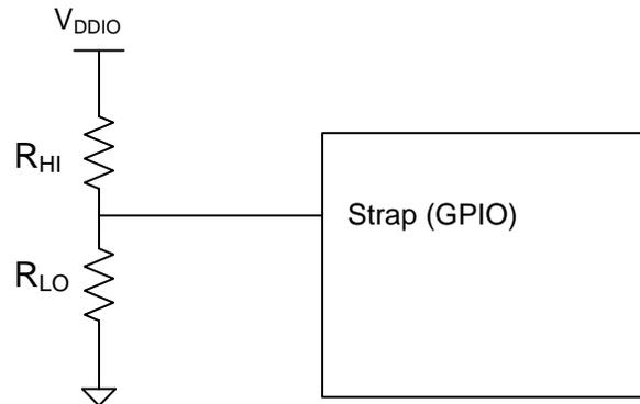
Figure 4. Strap Circuit
