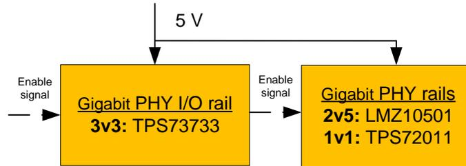
Figure 14. Power Stage for Two Gigabit Ethernet PHYs
