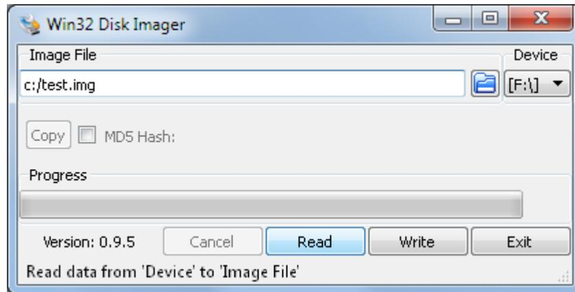
**Figure 25. Procedure to Create SD-Card Image With Win32 Disk Imager**
