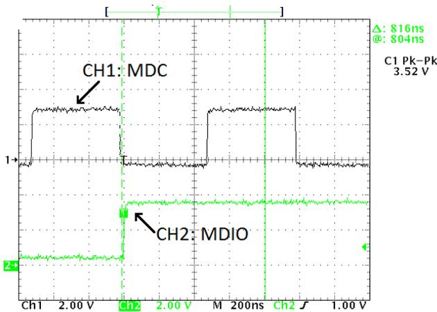
Figure 43. SMI Clock and Data Signal at 2.5 MHz at DP83867IR ETH1
