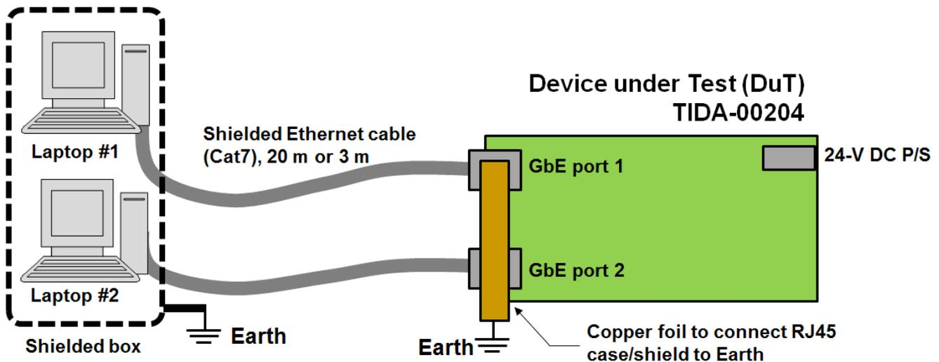
Figure 55. TIDA-00204 Test Equipment Overview for EMI/EMC Tests
