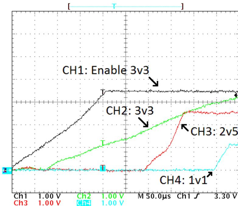
**Figure 48. PHY Power Supply Voltage Rails During Startup**
