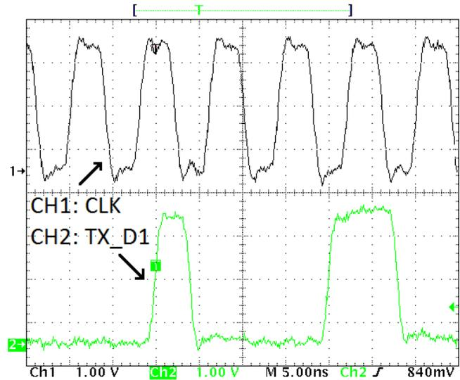
Figure 42. ETH2 RGMII TX Clock and Data Signal During Gigabit Ethernet Connection
