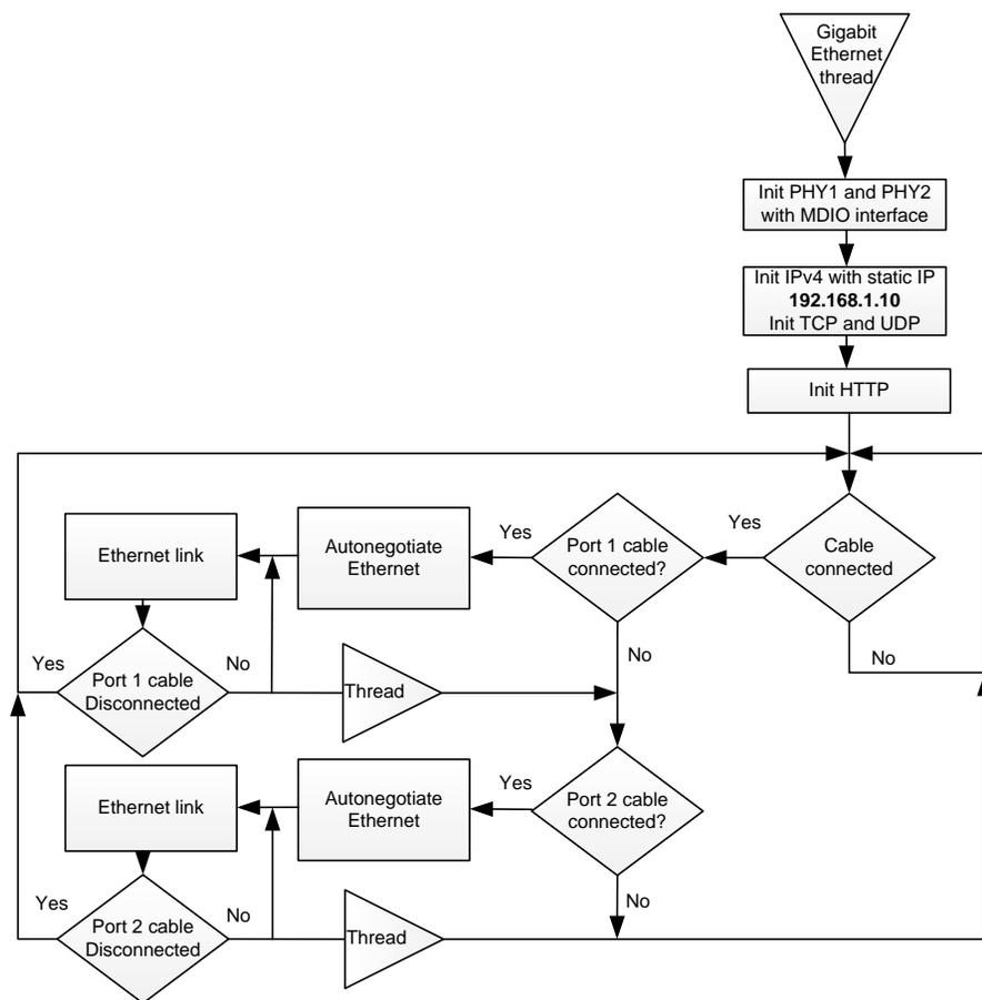
Figure 23. AM3359 Gigabit Ethernet Thread Flowchart
