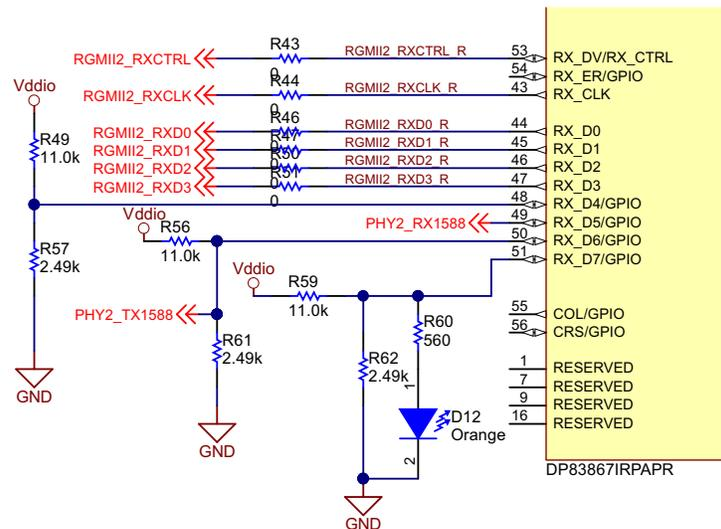
Figure 5. Schematic for DP83867IR Strap Configuration on ETH2
