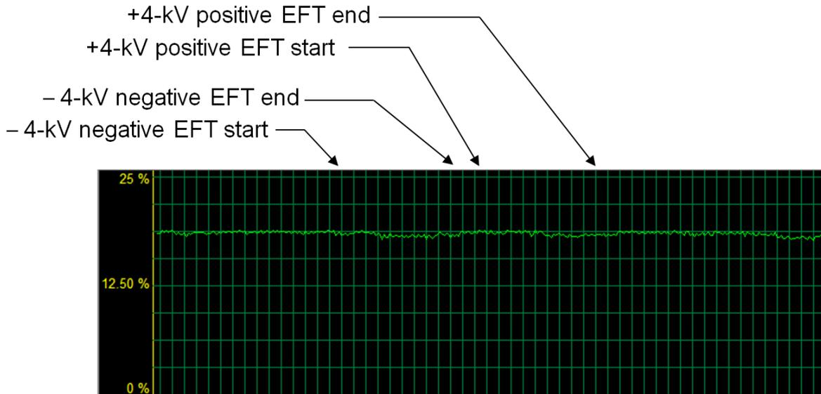
Figure 65. IEC61000-4-4 ±4-kV EFT: Network Utilization With UDP Throughput Test on Gigabit Ethernet Port 1
