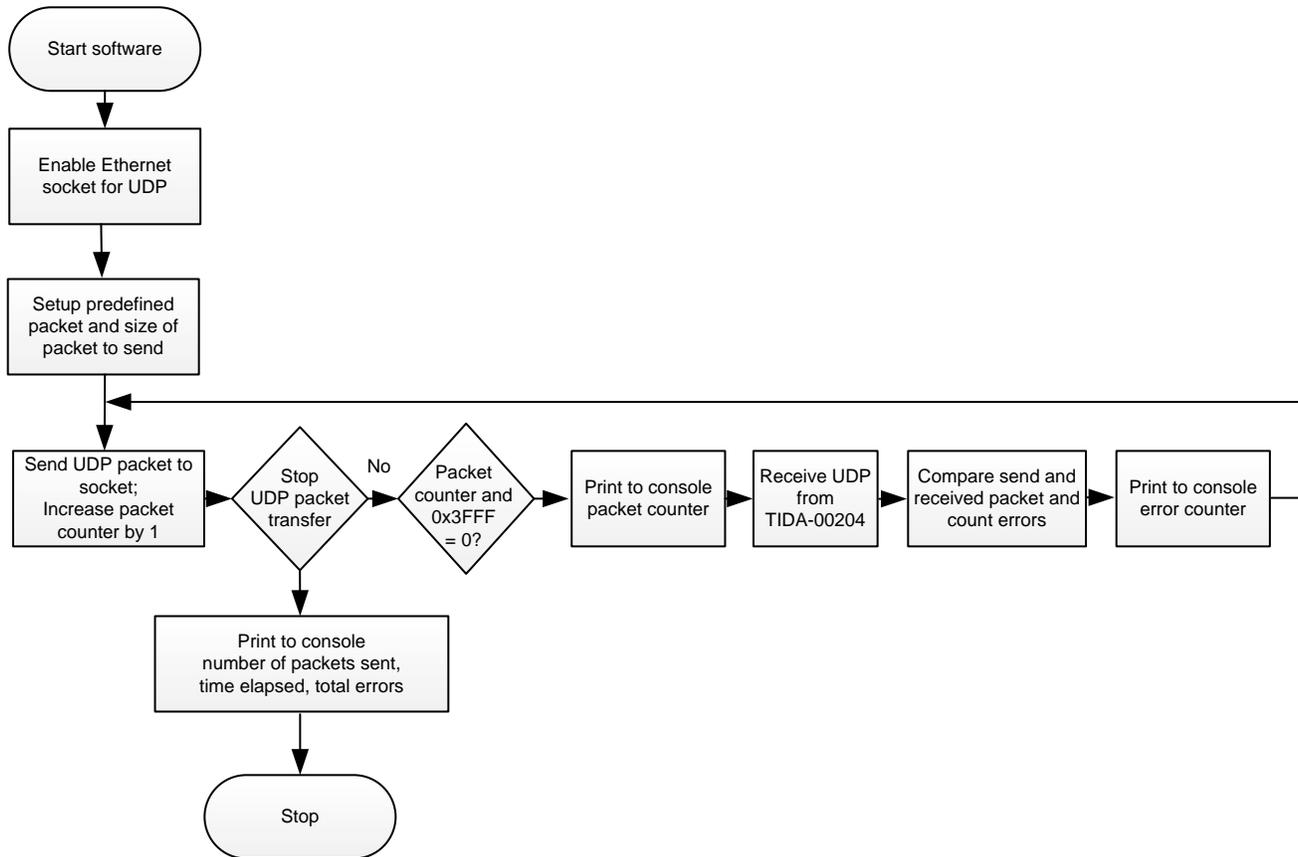
Figure 28. Flowchart of UDP Packet Error Test Software
