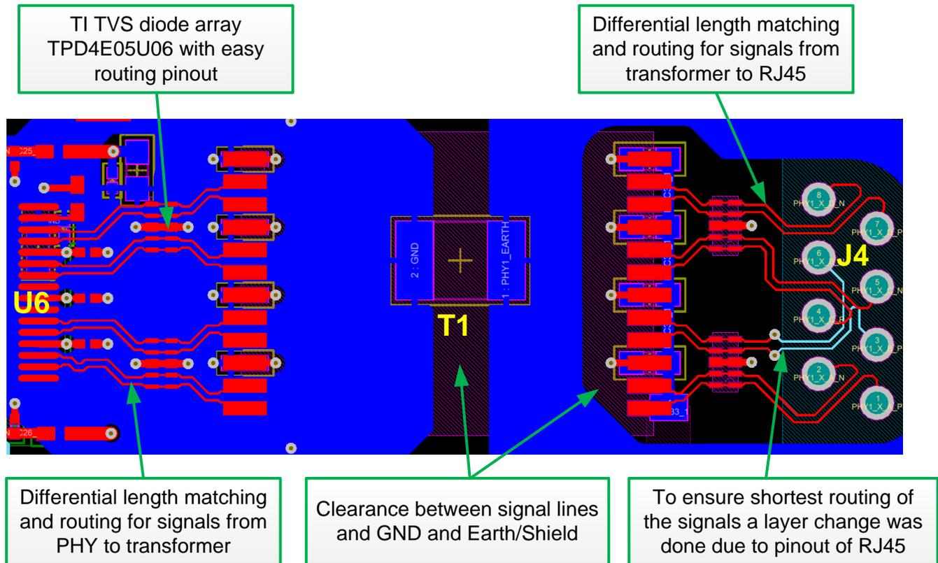
Figure 73. Layout Guidelines for PHY Differential Signals
