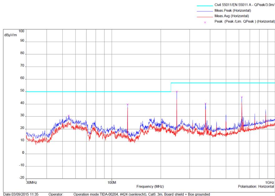
**Figure 60. Measured EMI Spectrum According to EN55011;
