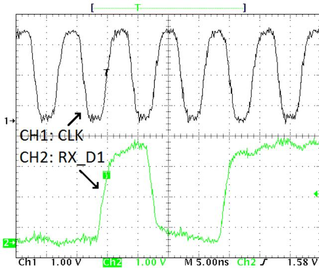
Figure 41. ETH2 RGMII RX Clock and Data Signal During Gigabit Ethernet Connection
