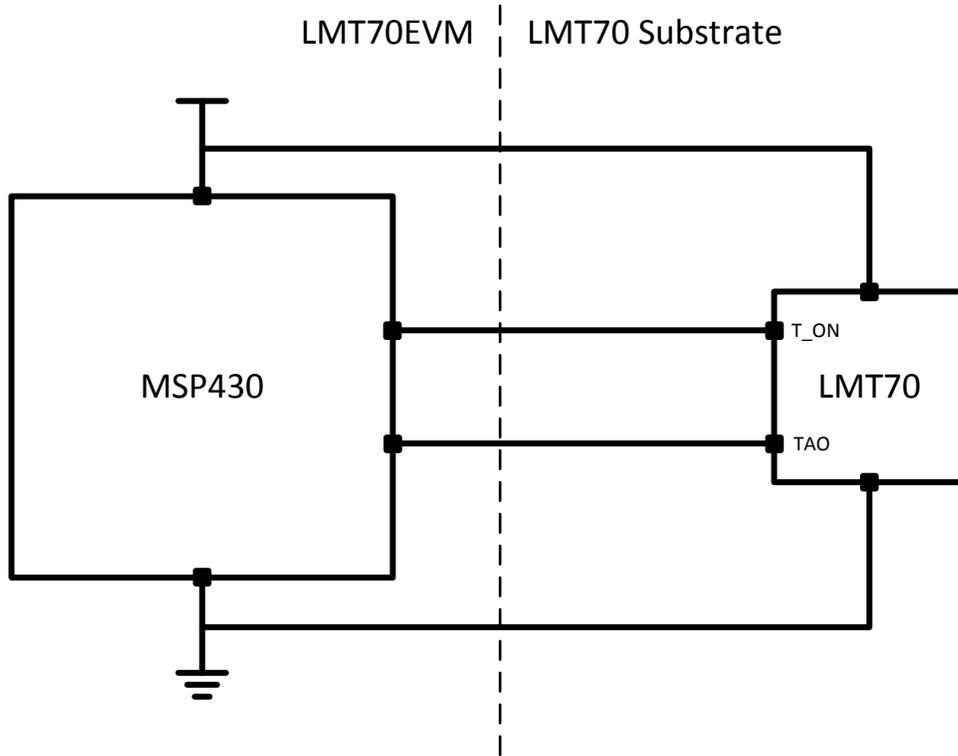
Figure 5: Block Diagram
