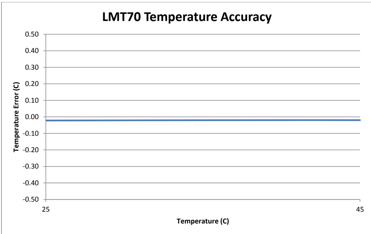
**Figure 4: LMT70 Temperature Accuracy (25°C to 45°C)**
