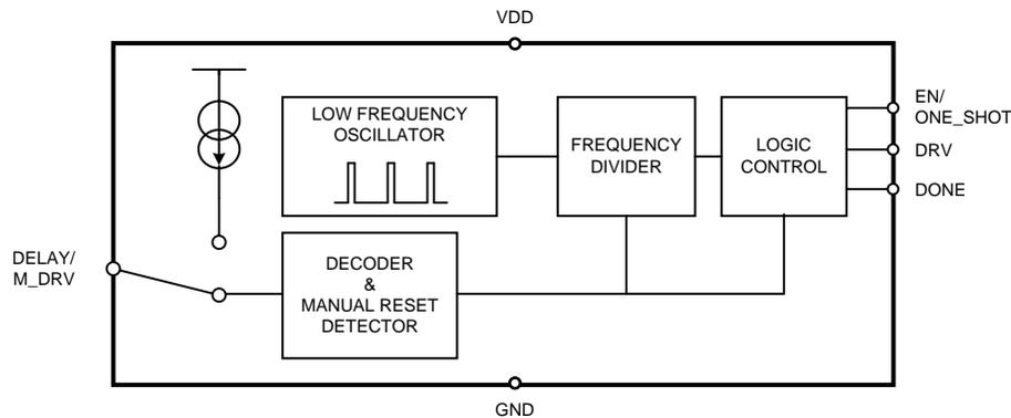
**Figure 4. TPL5110 Functional Block Diagram**
