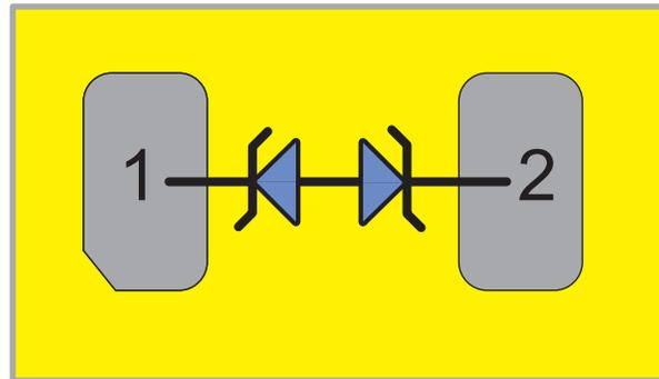
**Figure 6. TPD1E10B06 Device Configuration**
