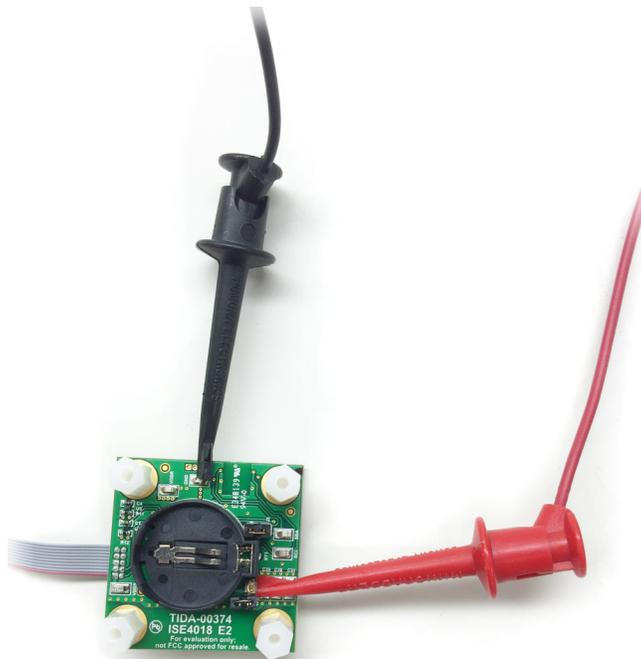
**Figure 9. Configuration of Jumpers and Power for Programming and Debugging**
