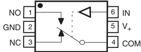
**Figure 5. TS5A3160 Package Diagram**
