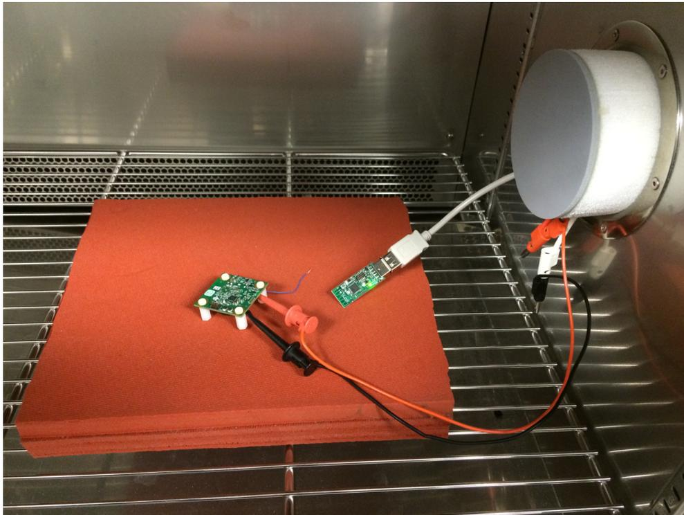
**Figure 19. Temperature Test Setup**
