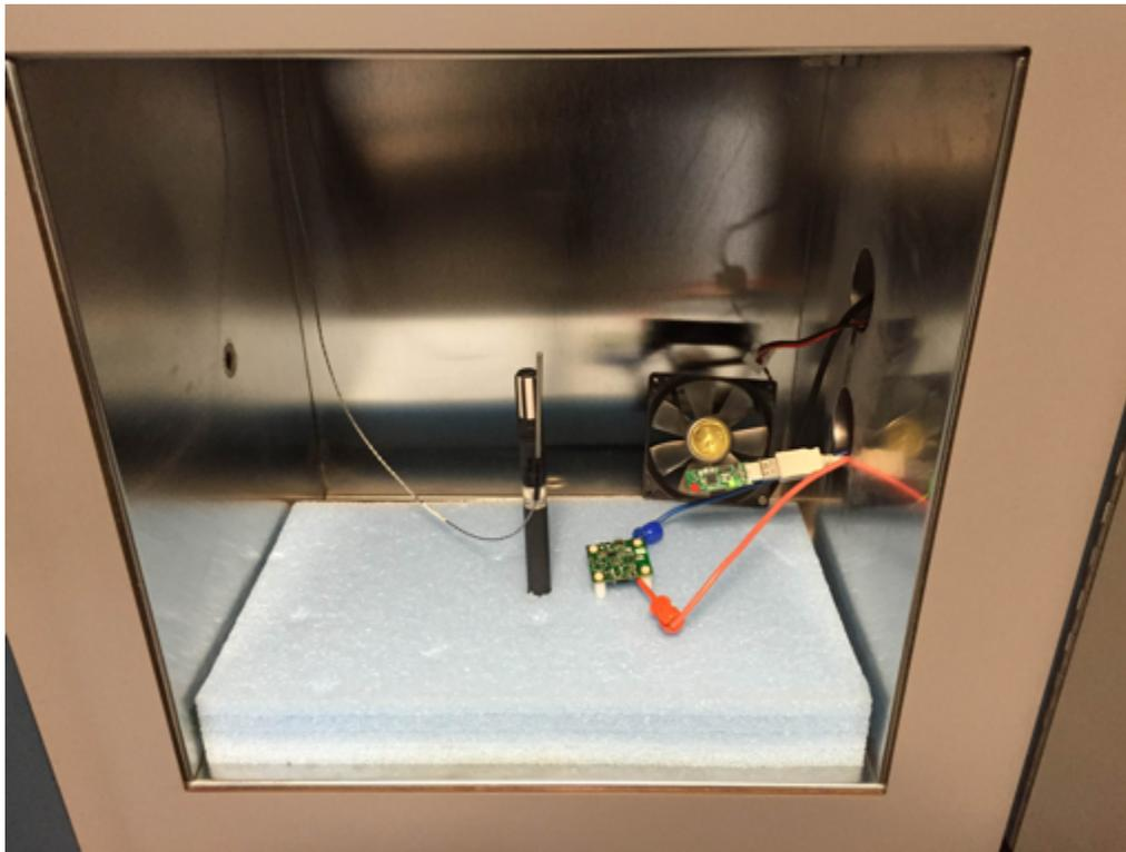
**Figure 17. Relative Humidity Test Setup**
