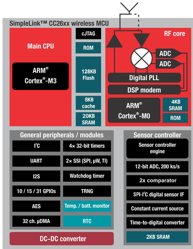
Figure 3. CC2650 Functional Block Diagram
