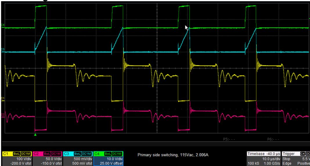
Figure 7. Primary Side Switching Waveform
