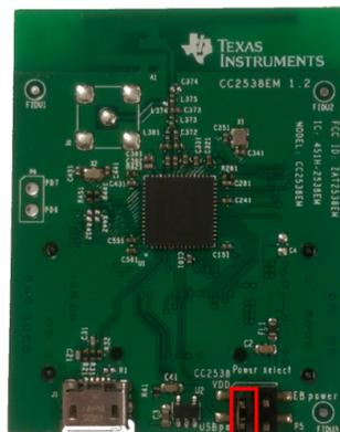
Figure 9. Jumper Position for USB Connection
