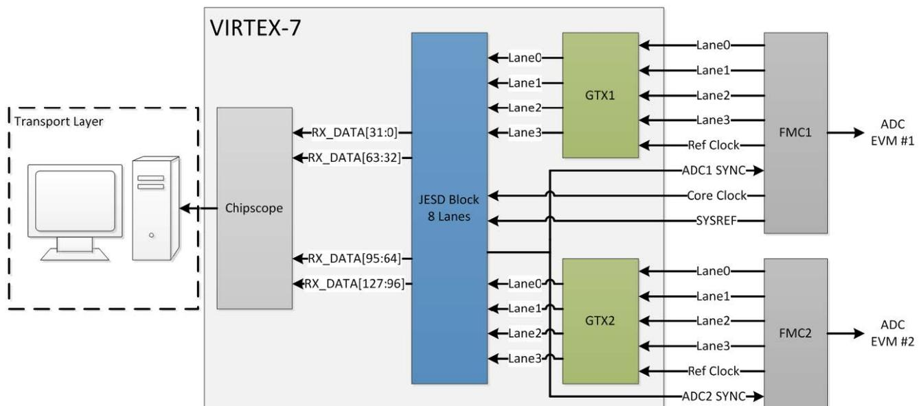
Figure 5. Block Diagram of the VC707 Firmware
