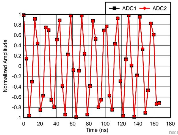
**Figure 6. Sampled Signals at 70 MHz With Complex Mixer Disabled (NCO Frequency = 0)**
