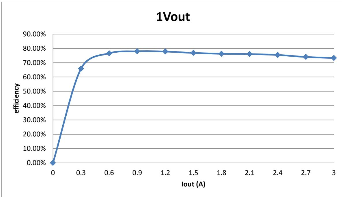
Figure 6. VIN = 12V, VCCINT Efficiency
