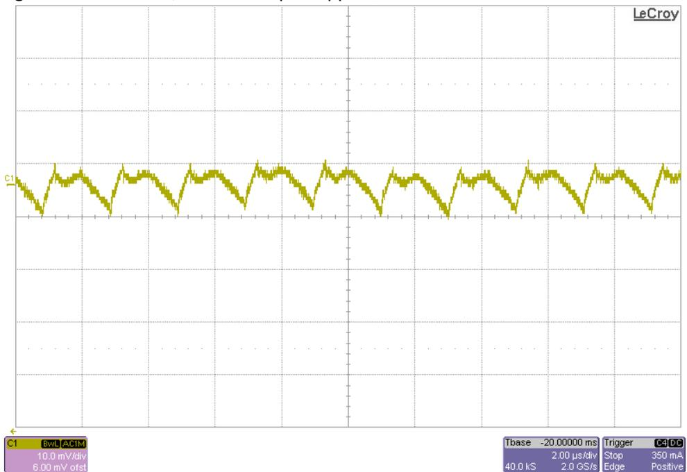
Figure 11. VIN = 12V, VCCAUX Output Ripple @ IOOUT = 3A
