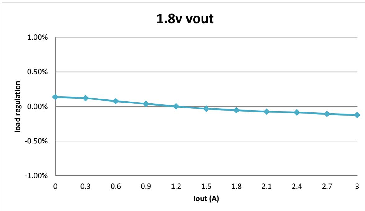
Figure 9. VIN = 12V, VCCAUX Load Regulation
