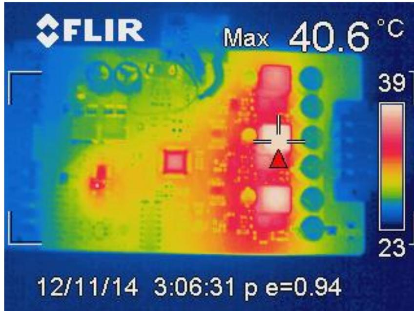
**Figure 39. Thermal Image with 8Ω Load (VIN = 6V, Boost)**
