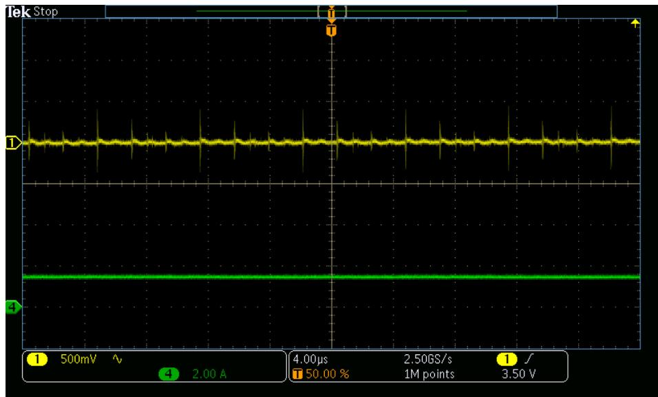
Figure 29. AC Coupled Output Voltage Ripple with 8Ω Load (VIN = 6V, Channel 1 = VOUT, Channel 4 = IOU)
