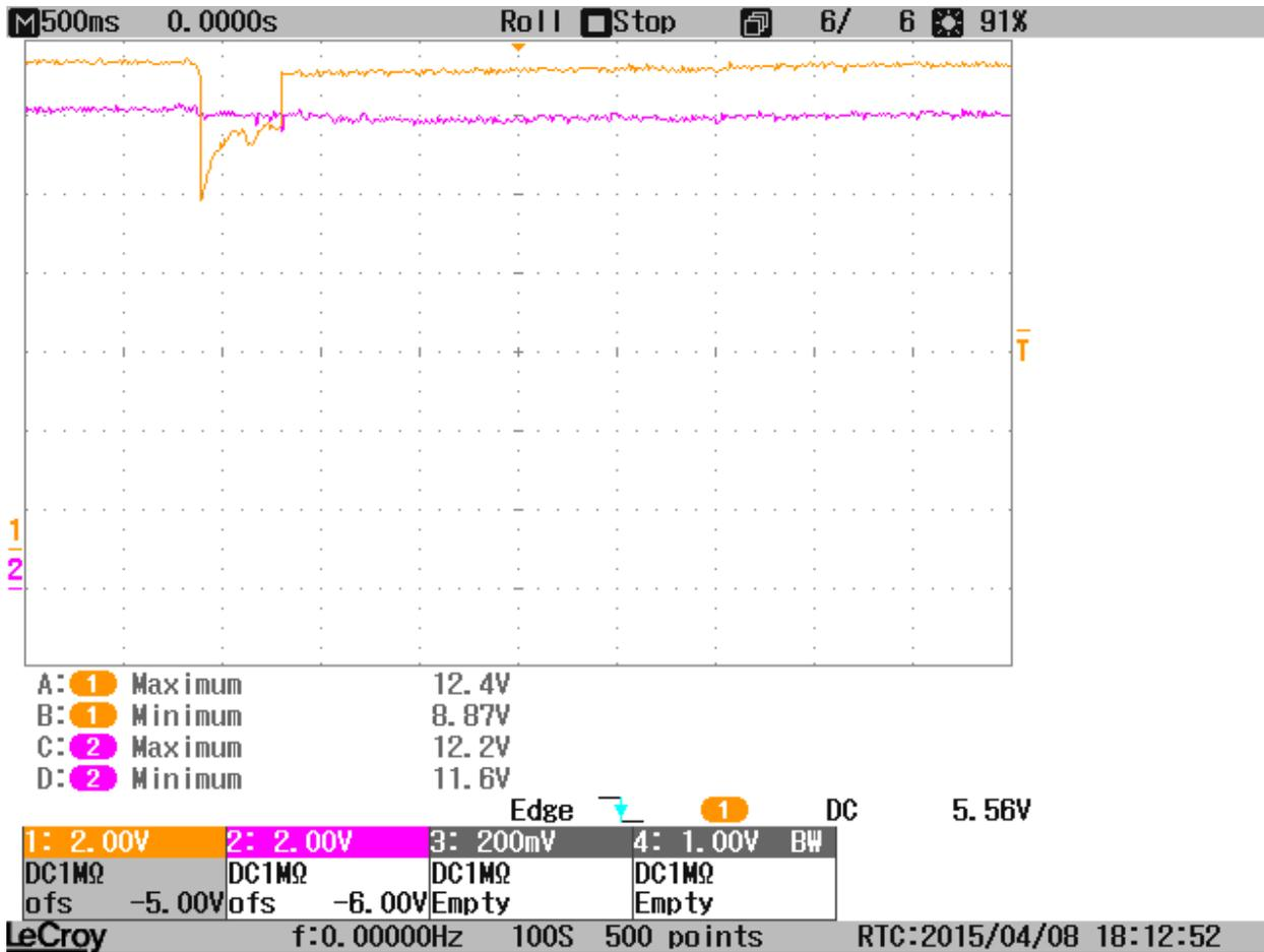
Figure 32. In-vehicle crank event (no external load) – second example
