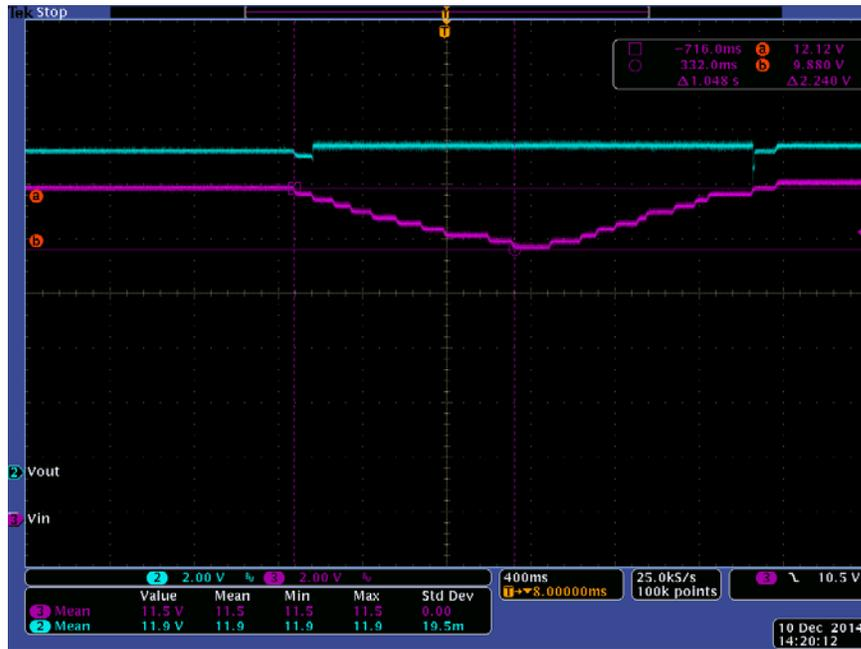
Figure 25. Bypass to Boost and Boost to Bypass Transitions with 33A Load (Channel 2 = VOUT, Channel 3 = VIN)
