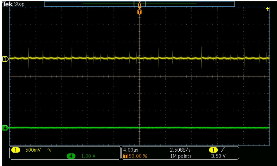
Figure 28. AC Coupled Output Voltage Ripple with No Load (VIN = 6V, Channel 1 = VOUT, Channel 4 = IOU)
