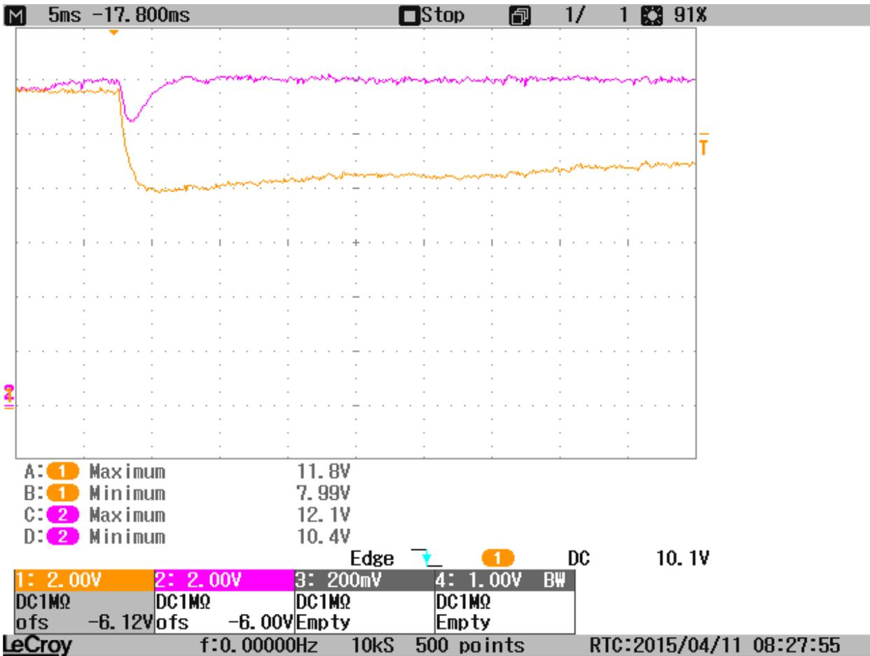
**Figure 37. In-vehicle drank event with 4 Ohm load (expanded time scale)**
