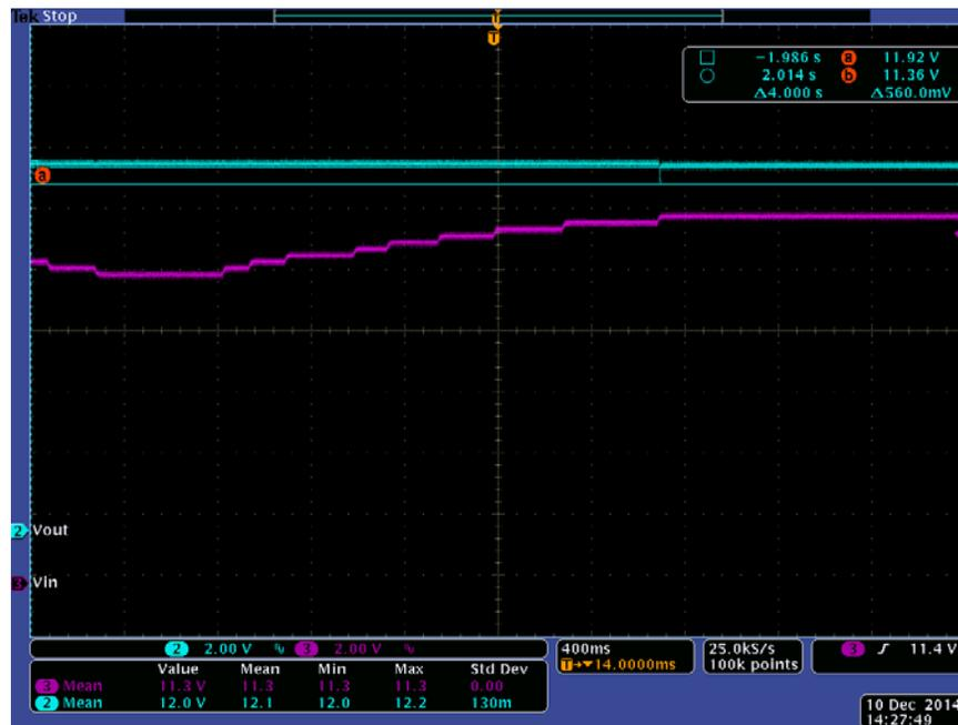
Figure 19. Boost to Bypass Transition with No Load
