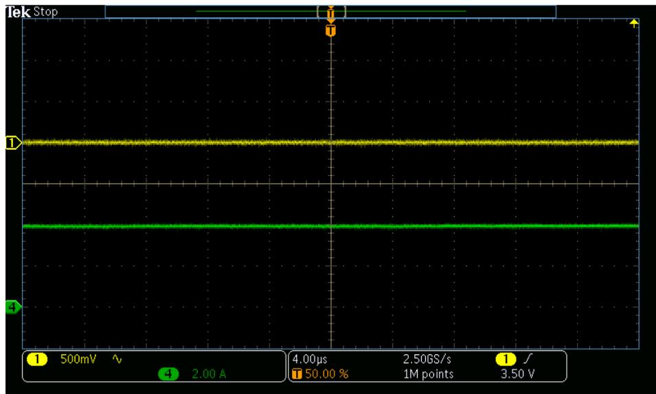
Figure 27. AC Coupled Output Voltage Ripple with 3Ω Load
