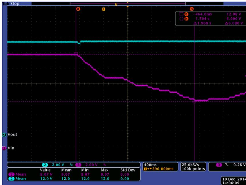
Figure 8. Bypass to Boost Transition with 7.5A Load (Channel 2 = VOUT, Channel 3 = VIN)
