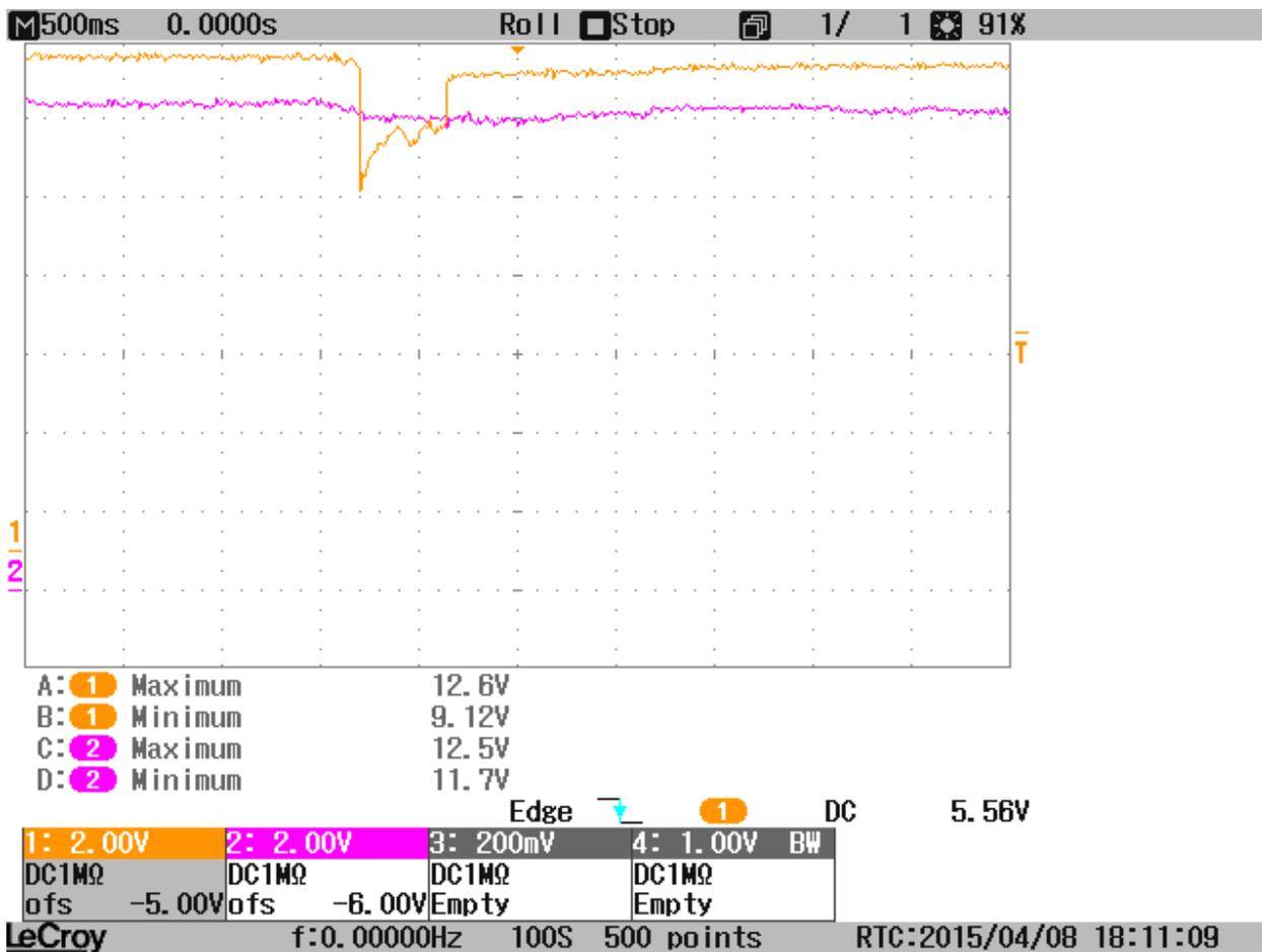
**Figure 31. In-vehicle crank event (no external load) – first example**
