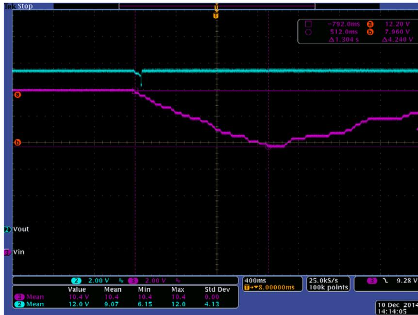
Figure 14. Bypass to Boost Transition with 22.5A Load
