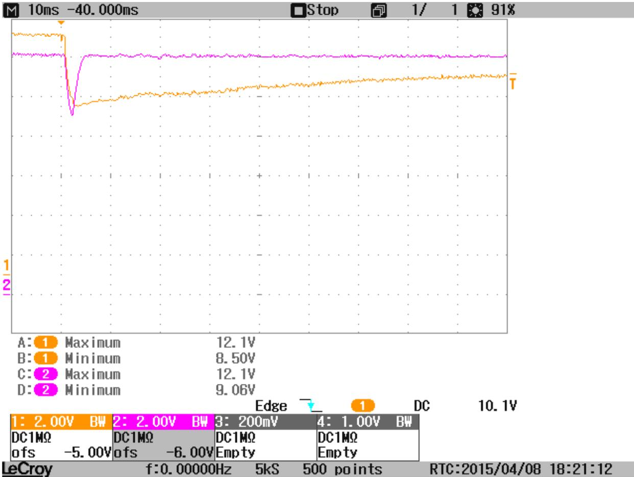
**Figure 36. In-vehicle drunk event with no external load (expanded time scale)**
