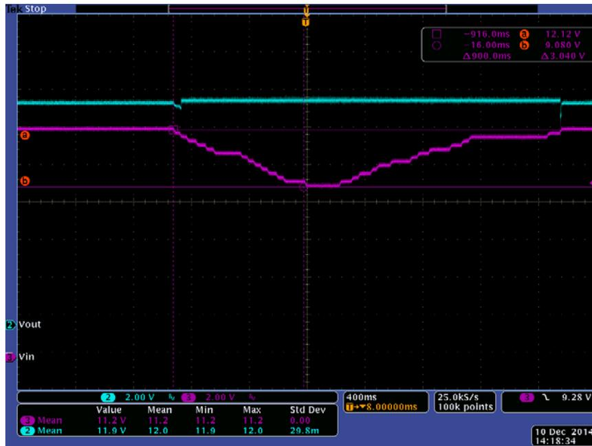
Figure 24. Bypass to Boost and Boost to Bypass Transitions with 30A Load (Channel 2 = VOUT, Channel 3 = VIN)
