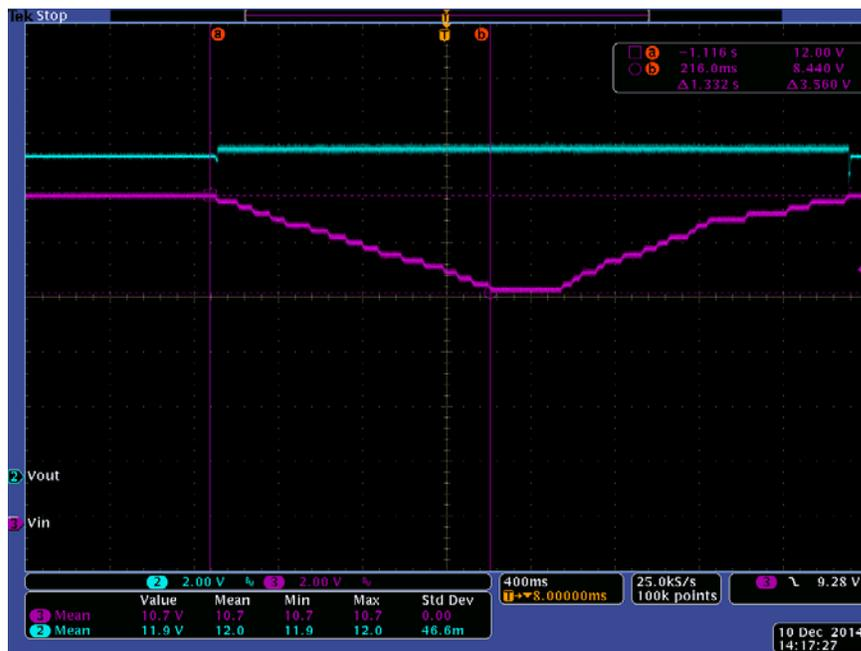
Figure 23. Bypass to Boost and Boost to Bypass Transitions with 27.5A Load (Channel 2 = VOUT, Channel 3 = VIN)
