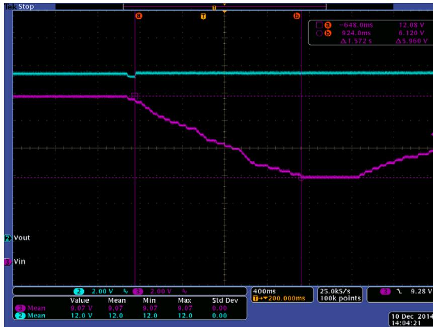
**Figure 6. Bypass to Boost Transition with 2.5A Load
