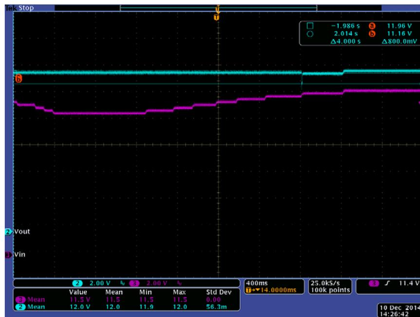
Figure 21. Boost to Bypass Transition with 20A Load
