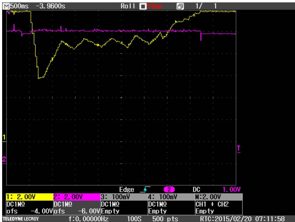
**Figure 30 Performance with 25A load during simulated engine crank**
