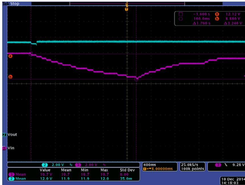
Figure 16. Bypass to Boost Transition with 27.5A Load (Channel 2 = VOUT, Channel 3 = VIN)
