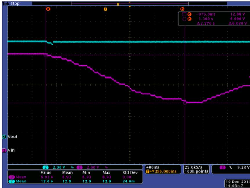
Figure 9. Bypass to Boost Transition with 10A Load (Channel 2 = VOUT, Channel 3 = VIN)
