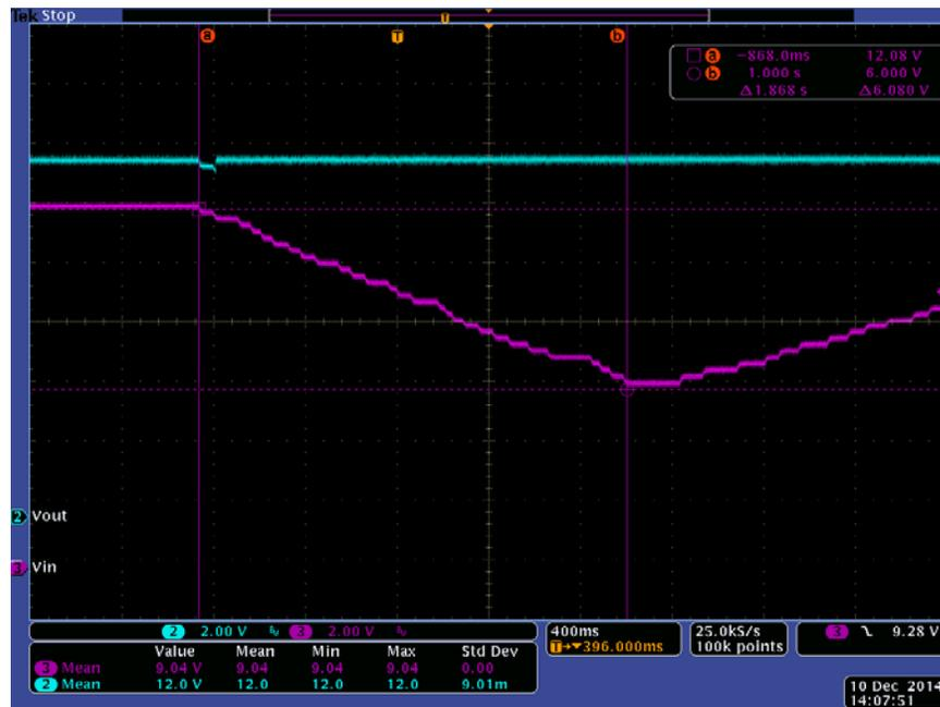
Figure 11. Bypass to Boost Transition with 15A Load
