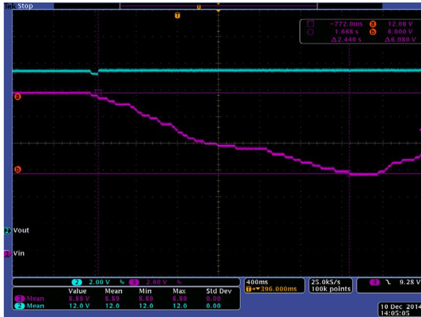
**Figure 7. Bypass to Boost Transition with 5A Load
