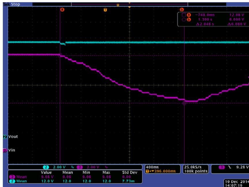
Figure 10. Bypass to Boost Transition with 12.5A Load
