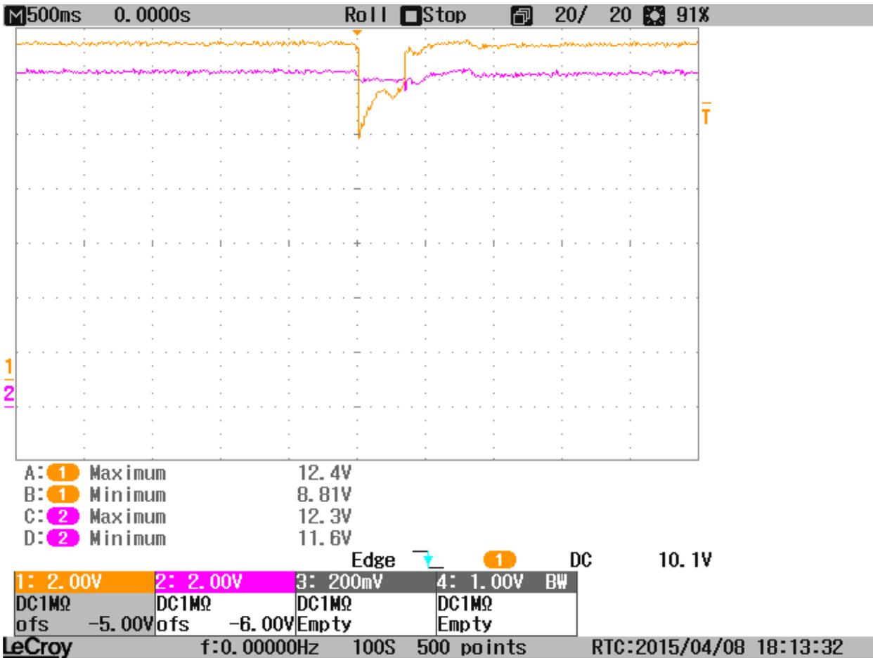
Figure 33. In-vehicle crank event (no external load) – third example
