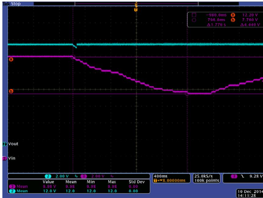
Figure 15. Bypass to Boost Transition with 25A Load
