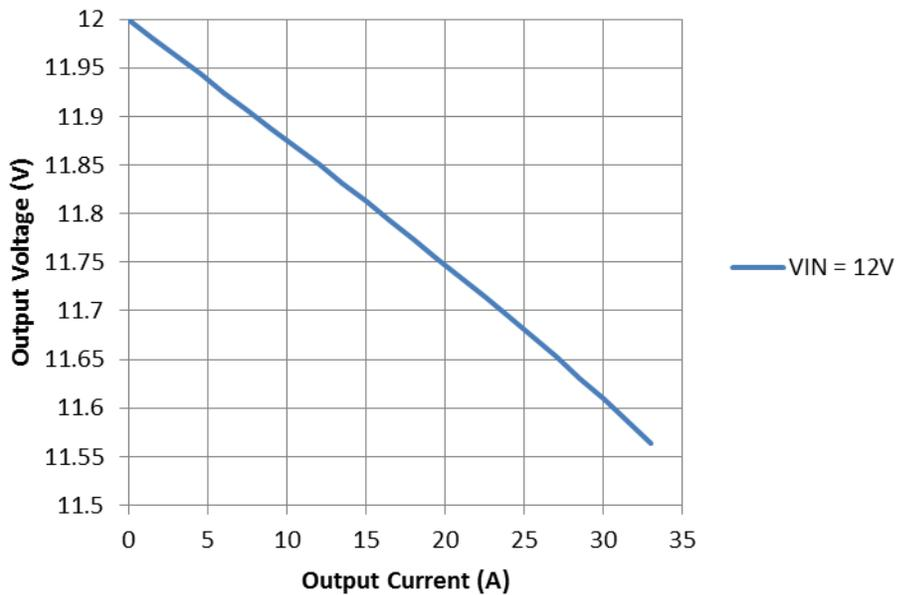
**Figure 3. Output Voltage Regulation vs Output Load Current (VIN = 12V, Bypass)**
