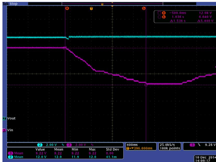
Figure 12. Bypass to Boost Transition with 17.5A Load
