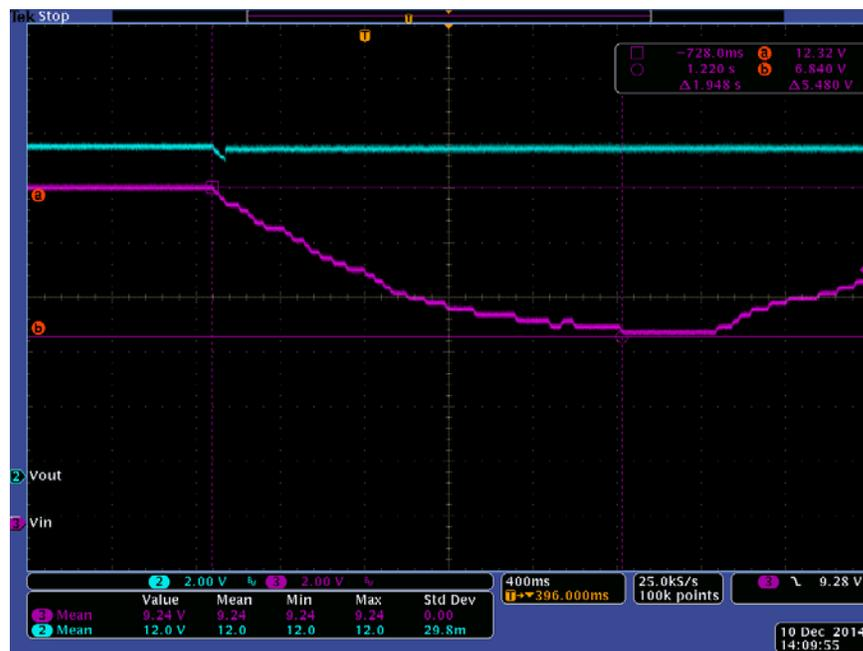
Figure 13. Bypass to Boost Transition with 20A Load
