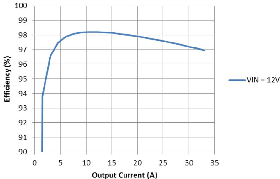
Figure 1. Efficiency vs Output Load Current (VIN = 12V, Bypass)
