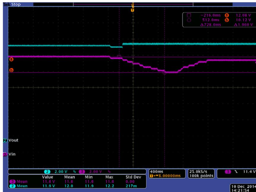
Figure 18. Bypass to Boost Transition with 33A Load
