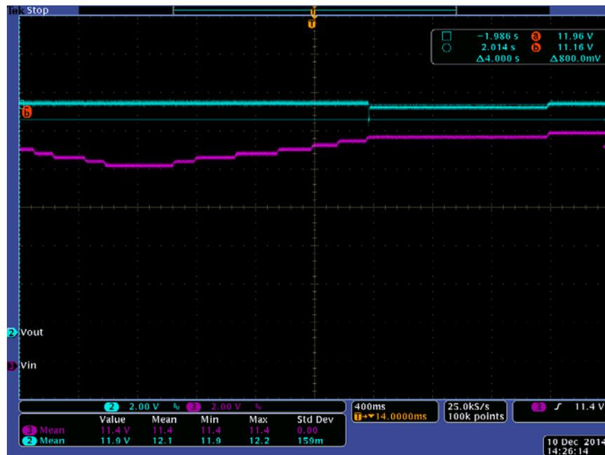
Figure 20. Boost to Bypass Transition with 15A Load
