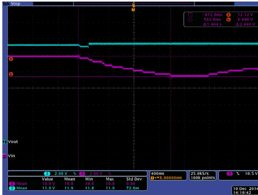
Figure 17. Bypass to Boost Transition with 30A Load (Channel 2 = VOUT, Channel 3 = VIN)
