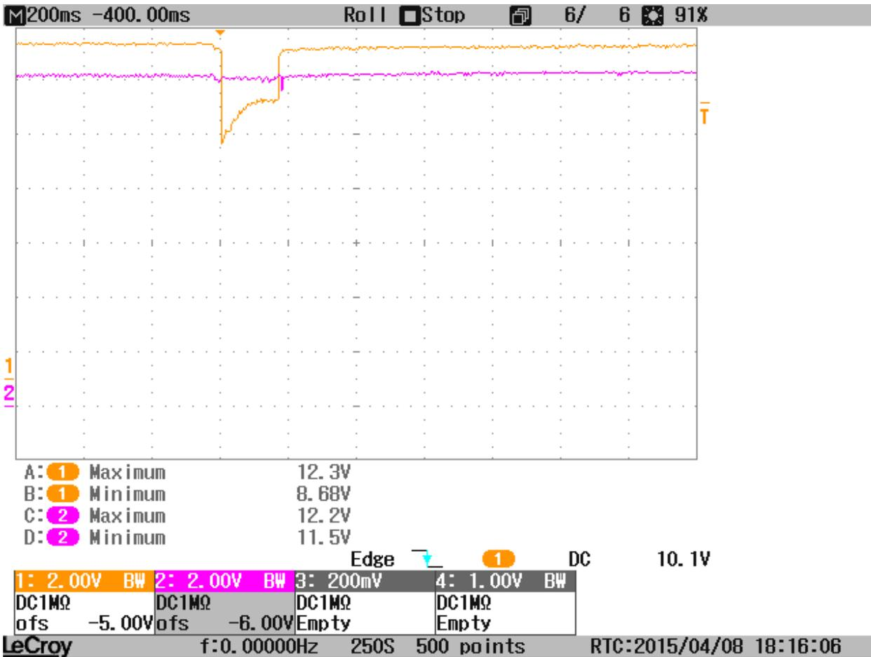
Figure 34. In-vehicle crank event (no external load) – fourth example – starter “bump”
