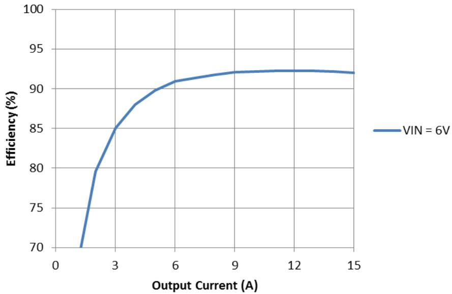
**Figure 2. Efficiency vs Output Load Current (VIN = 6V, Boost)**
