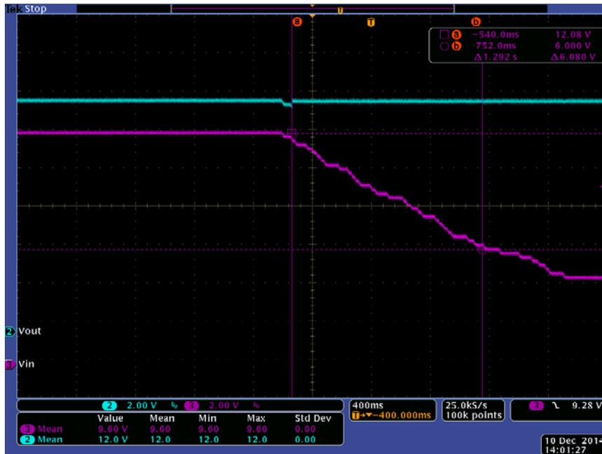
**Figure 5. Bypass to Boost Transition with No Load (Channel 2 = VOUT, Channel 3 = VIN)**
