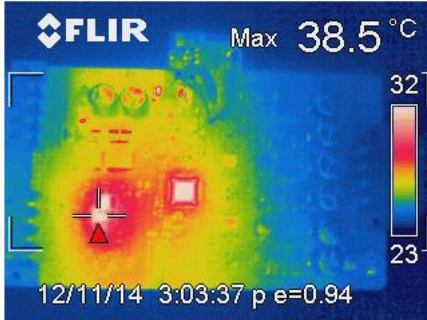
**Figure 38. Thermal Image with 3Ω Load (VIN = 12V, Bypass)**
