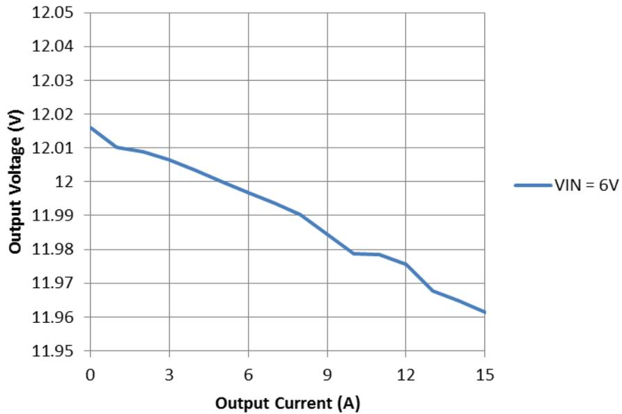
**Figure 4. Output Voltage Regulation vs Output Load Current (VIN = 6V, Boost)**
