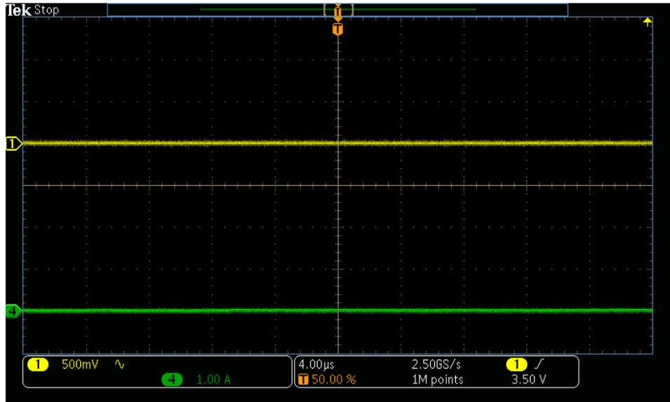
Figure 26. AC Coupled Output Voltage Ripple with No Load
