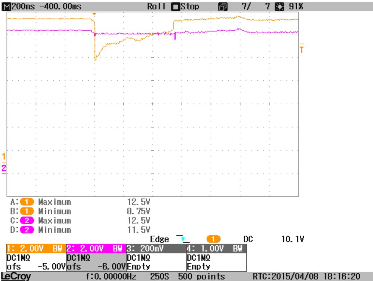
Figure 35. In-vehicle crank event (no external load) – fifth example – full start crank
