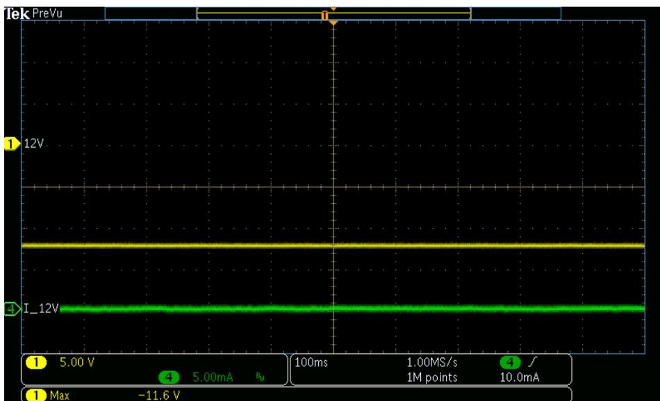
Figure 9: Reverse polarity current on J1 (12V)
