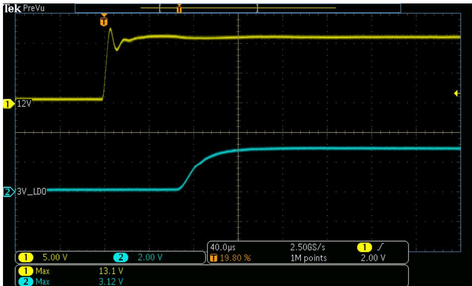
Figure 5: LDO Startup with LED Driver Disabled
