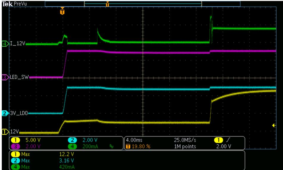
Figure 6: LDO Startup with 100% PWM on LED Driver
