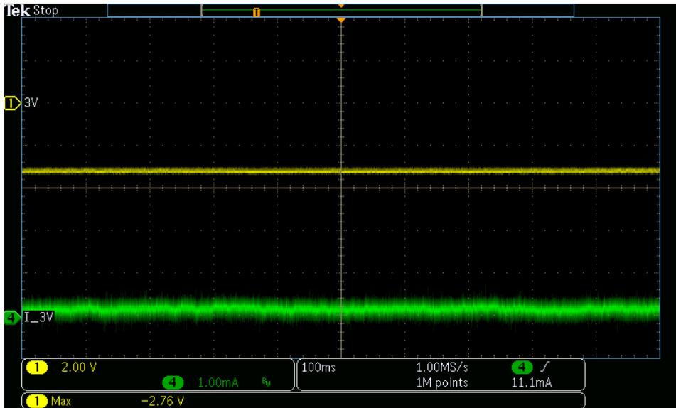
Figure 3: Reverse polarity current on BT1 (3V)
