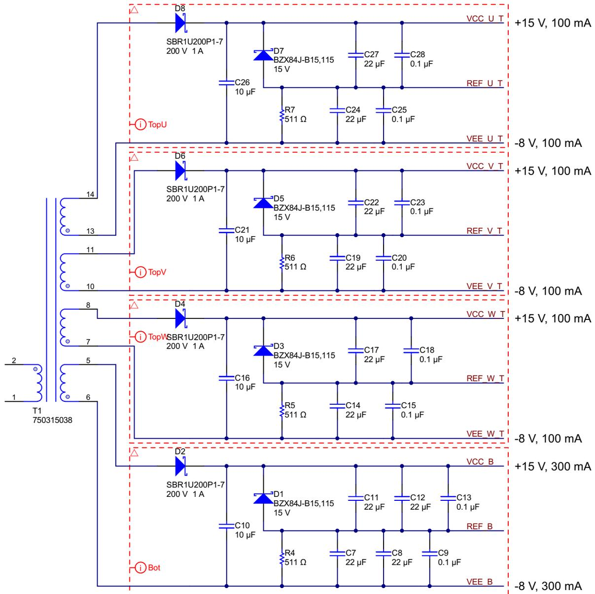
Figure 9. Secondary Section of the Schematic
