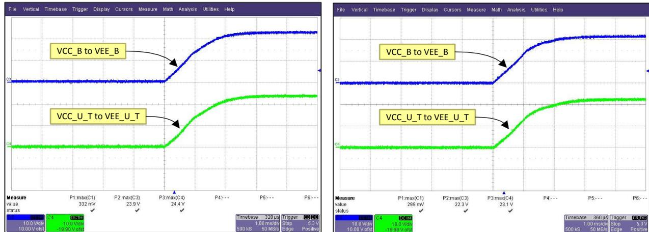
Figure 10. Start-Up into (Left) No Load at 24 V<sub>IN</sub> and (Right) Full Load at 24-V<sub>IN</sub>
