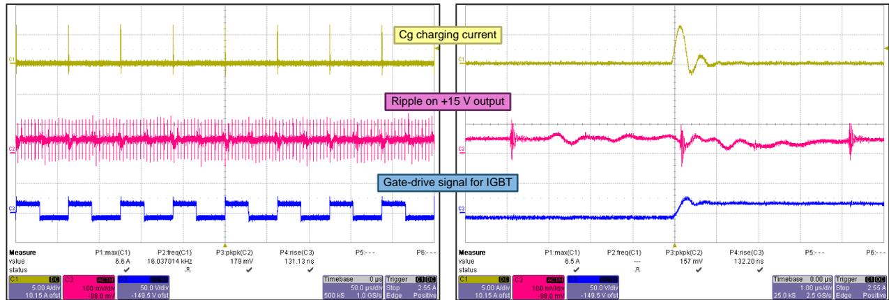
Figure 25. (A) Ripple on 15-V Output for 6-A Peak Load Current With IGBTs (B) Zoomed Waveforms
