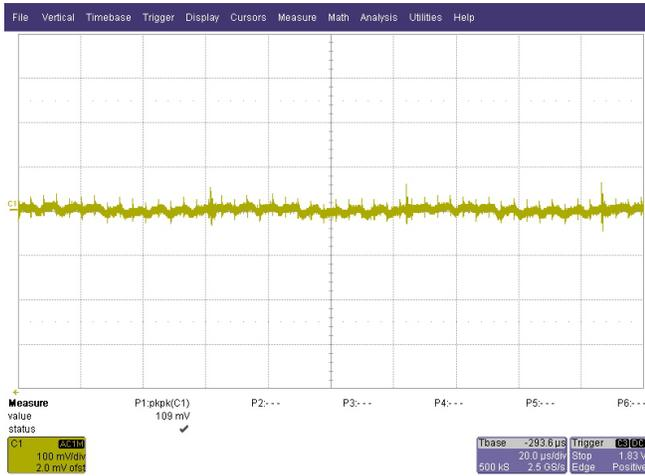
**Figure 23. Ripple on 15-V Output (for  $dv/dt = 5.6 \times E9$  V/s on the Output Load)**
