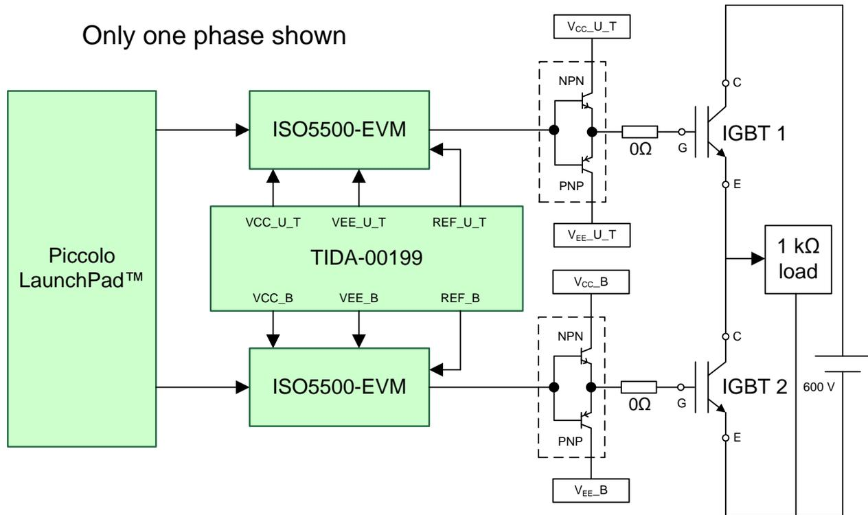
Figure 21. Setup for Testing TIDA-00199 Design With TI's ISO5500 and IGBTs
