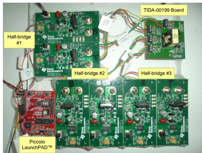
Figure 22. Board Setup Image
