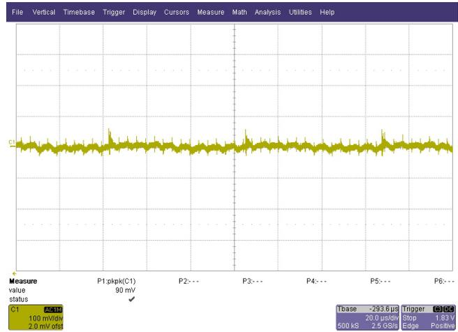
**Figure 24. Ripple on -8-V Output (for  $dv/dt = 5.6 \times E9$  V/s on the Output Load)**
