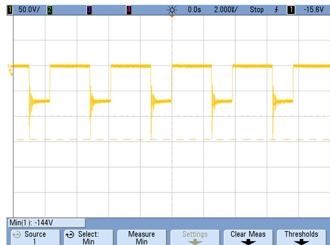
Figure 14. Bottom Output Diode Voltage at Full Load at 30-V<sub>IN</sub>
