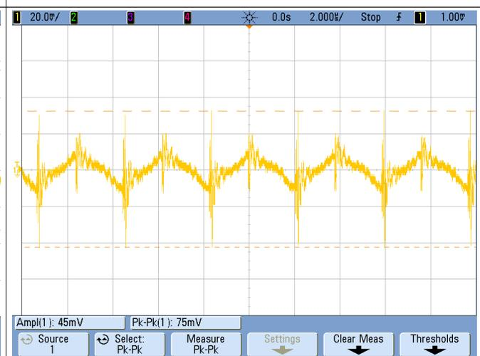
Figure 20. VEE\_B Output Ripples at Full Load at 24-V<sub>IN</sub>
