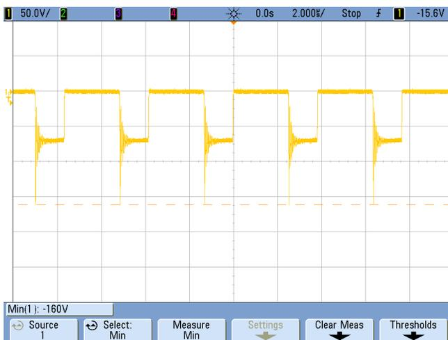
Figure 13. U<sub>T</sub> Output Diode Voltage at Full load at 30-V<sub>IN</sub>
