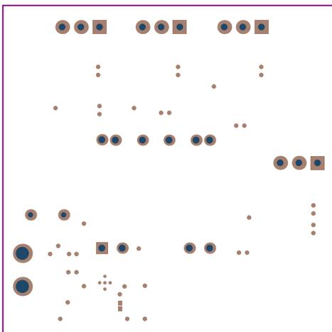
Figure 34. Bottom Solder Mask
