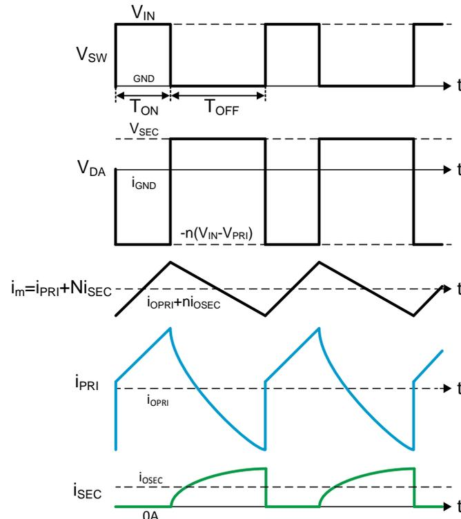
**Figure 7. Fly-Buck Operation Waveform**
