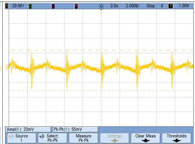
Figure 18. VEE\_U\_T Output Ripple at Full Load at 24-V<sub>IN</sub>
