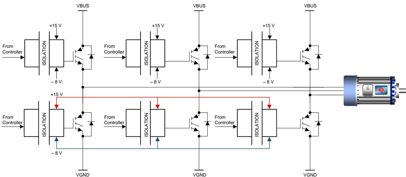
Figure 1. 3-Phase Inverter With Isolated Gate-drive
