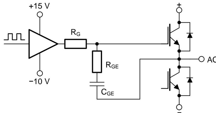
**Figure 2. IGBTs With Gate Drive Circuitry for Gate Power Calculation**
