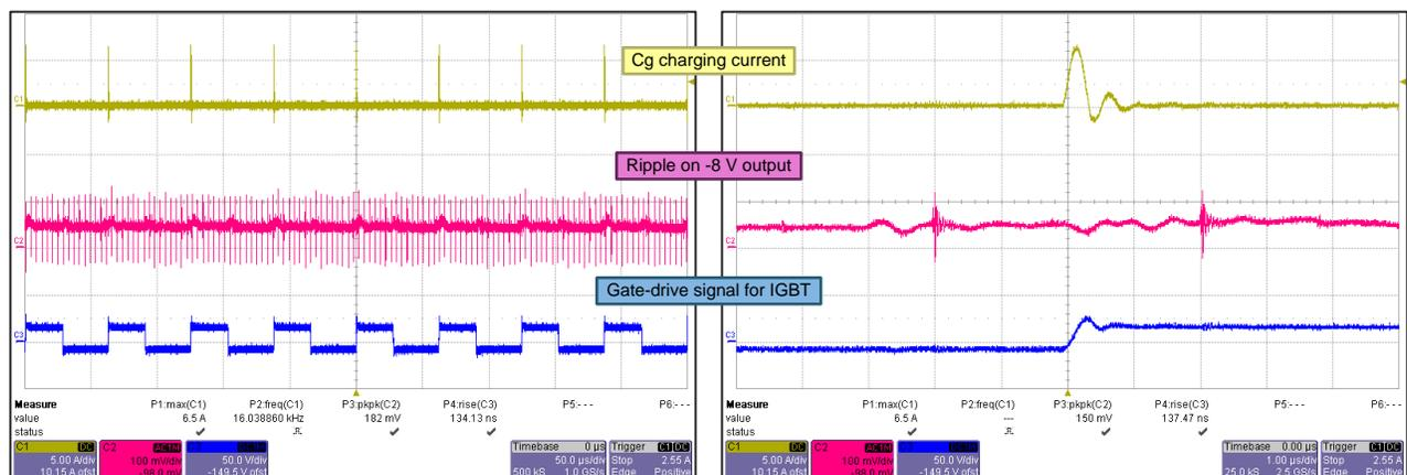
Figure 26. (A) Ripple on -8-V Output for 6-A Peak Load Current With IGBTs (B) Zoomed Waveforms
