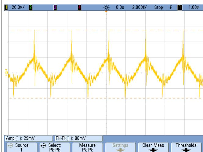
Figure 19. VCC\_B Output Ripple at Full Load at 24-V<sub>IN</sub>
