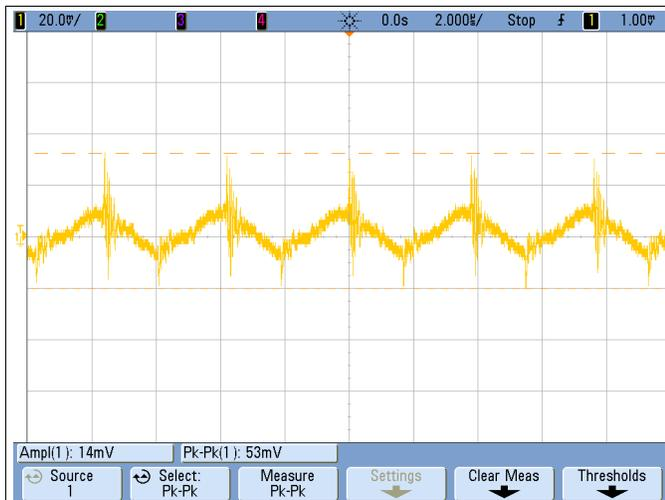
Figure 17. VCC\_U\_T Output Ripple at Full Load at 24-V<sub>IN</sub>
