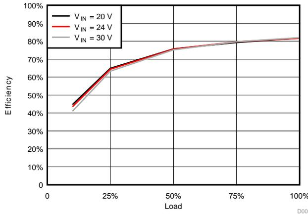
Figure 15. Total Efficiency Under Balanced Load
