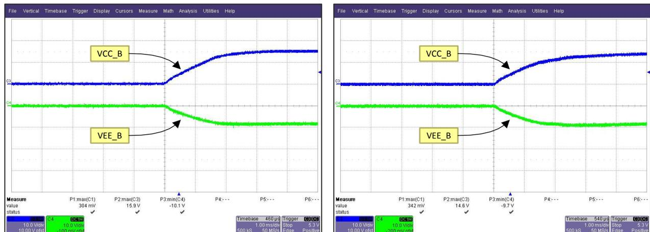
Figure 11. VCC\_B and VEE\_B Start-Up into (Left) No Load at 24-V<sub>IN</sub> and (Right) Full Load at 24-V<sub>IN</sub>
