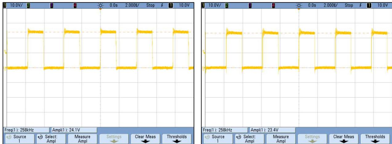
Figure 12. Switching Waveform at (Left) No Load at 24-V<sub>IN</sub> and (Right) Full Load at 24-V<sub>IN</sub>
