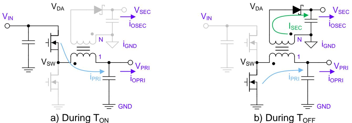
Figure 6. The Fly-Buck in ON and OFF time
