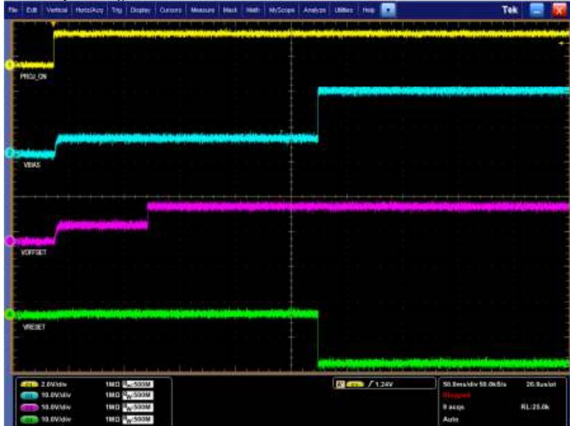
Power down Timing Measurements
