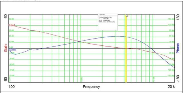
Frequency loop response of the converter – resistive load
