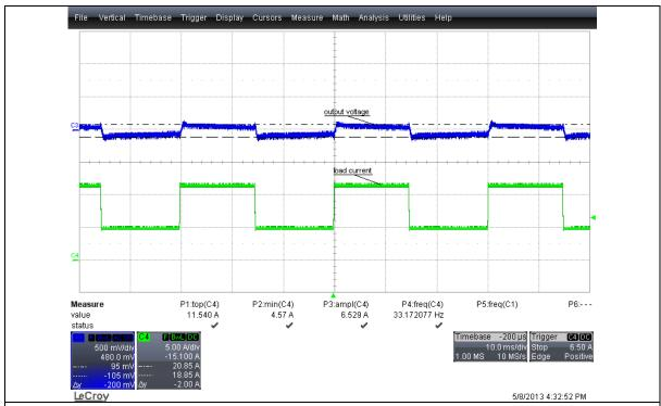
CH3 (Blue) 500mV/div – Output voltage AC coupled – 200mVpp CH4 (Green) 5A/div – Output current – 5A basic load, 7A load step.
