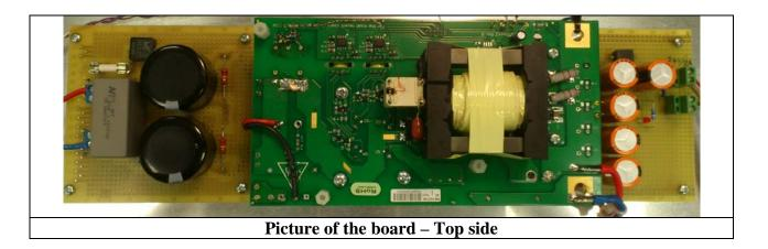
This board has been tested, according to the test report, 350V, 500Vin, full load, with a cooling fan with 32 cfm placed at 10cm distance.
