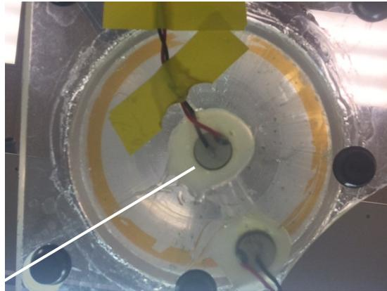
Figure 2 - Transducer glued to the bottom of tube
