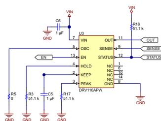
**Figure 11. DRV110 Circuit With Reference Setting Resistors**
