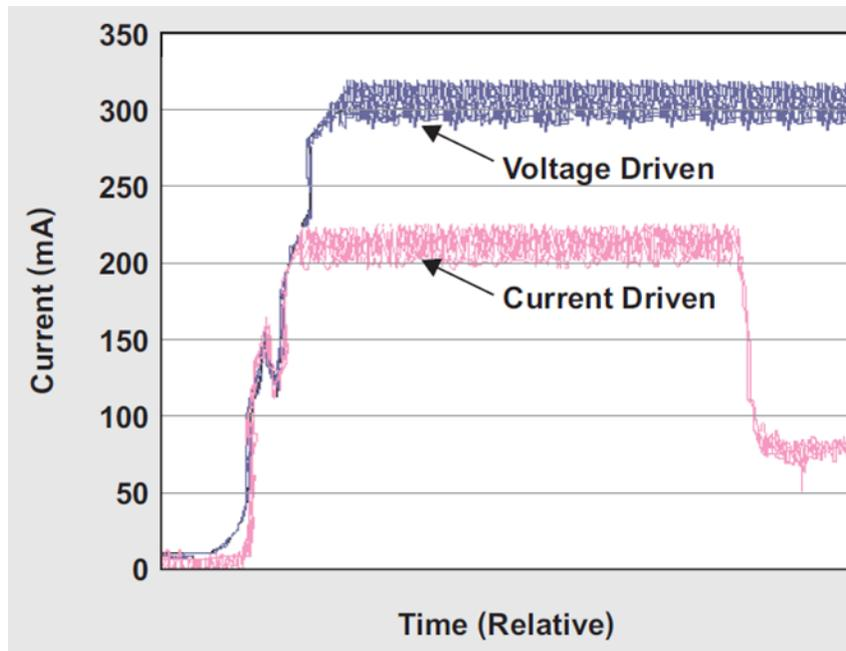
Figure 4. Solenoid Current With Voltage Drive and Current Drive
