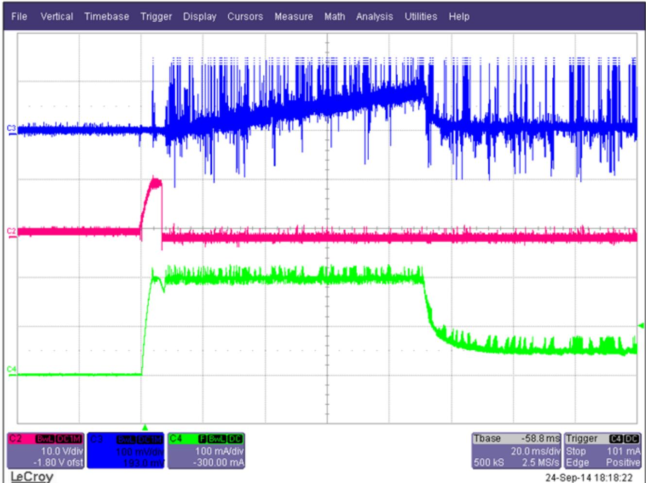
Ch3 – Voltage across the keep capacitor Ch2 – Hall sensor output (Position FB) Ch4 – Solenoid current
