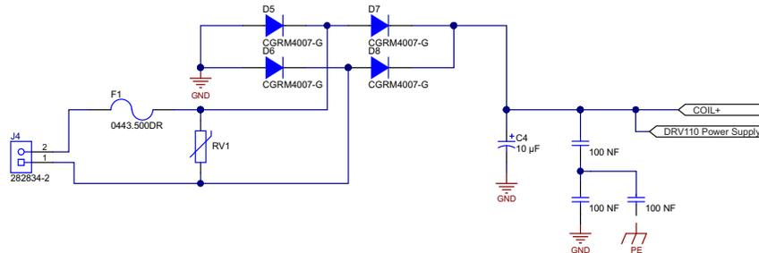
**Figure 30. EMC Filter Connected Across the DC Bus**
