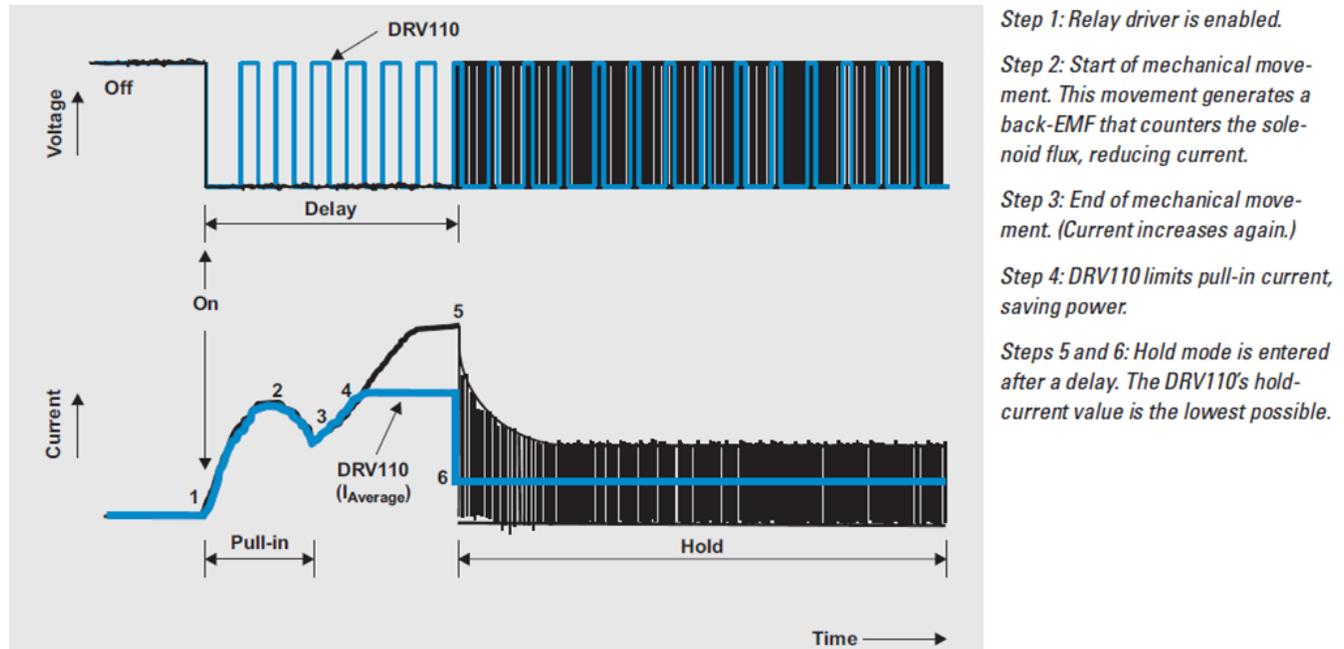
Figure 5. Operation of a Conventional Driver Versus DRV110
