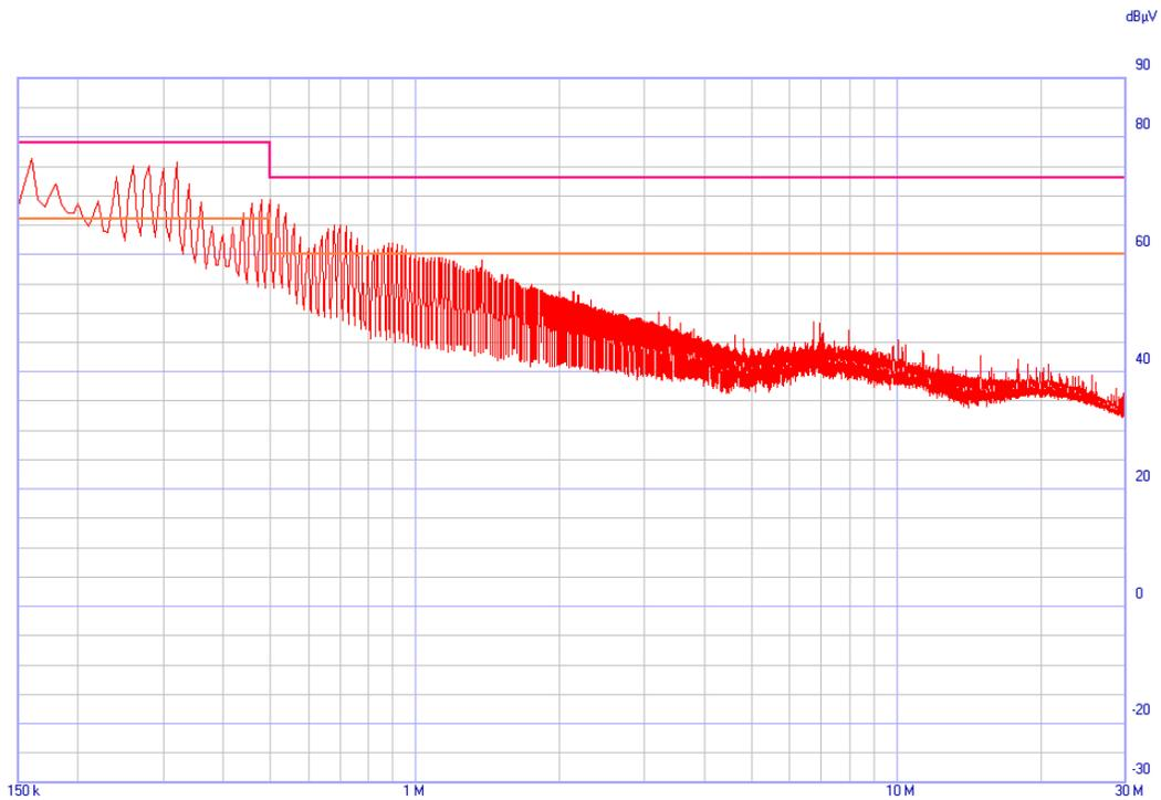
**Figure 32. EMC Test Results — Quasi Peak Detector Output**
