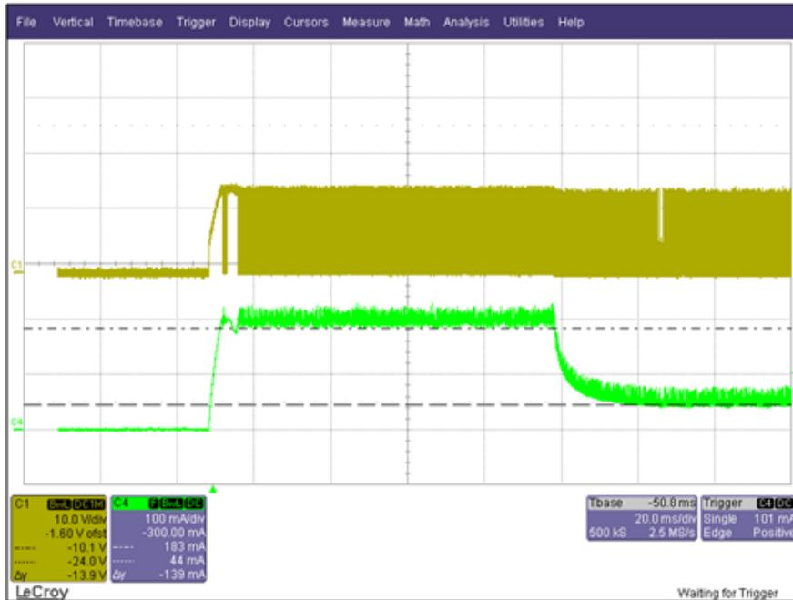
Ch1 – Gate signal from DRV110 (OUT) Ch4 – Solenoid current
