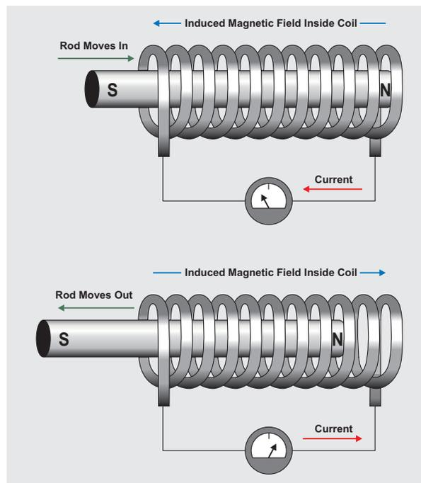
**Figure 1. Function of a Solenoid Coil**
