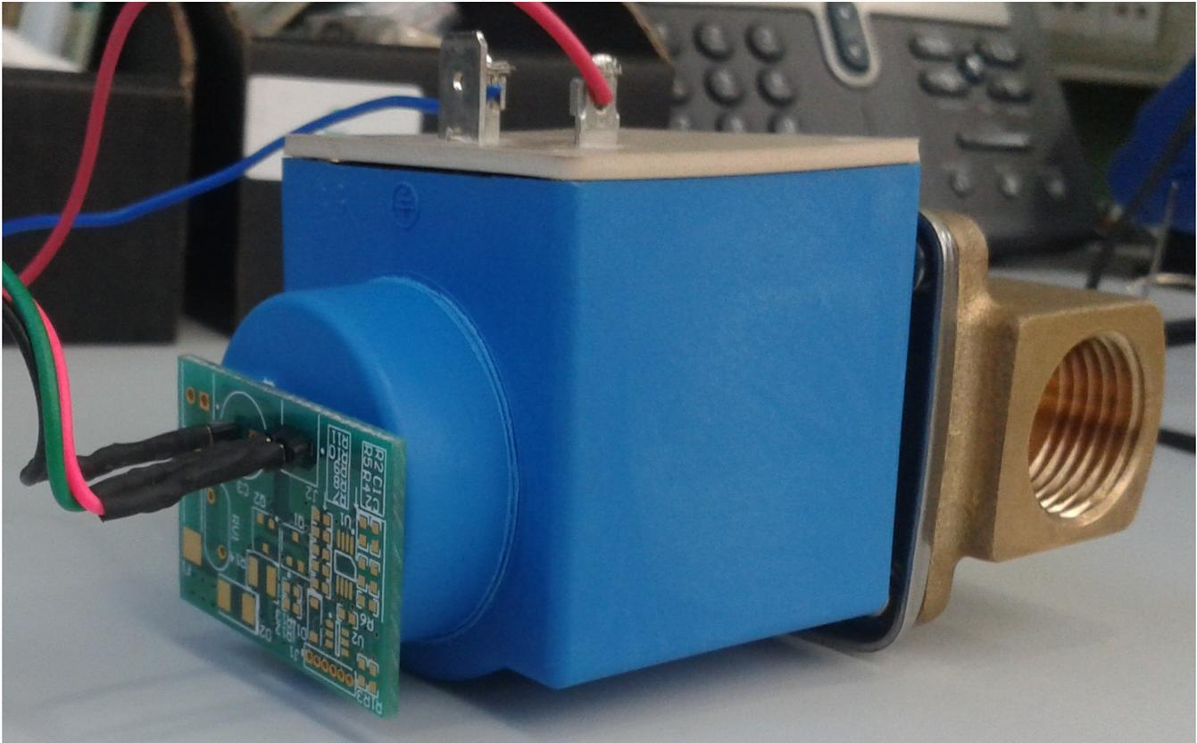
**Figure 15. Mounting of the Hall Sensor on the Solenoid Coil for Testing Purposes**
