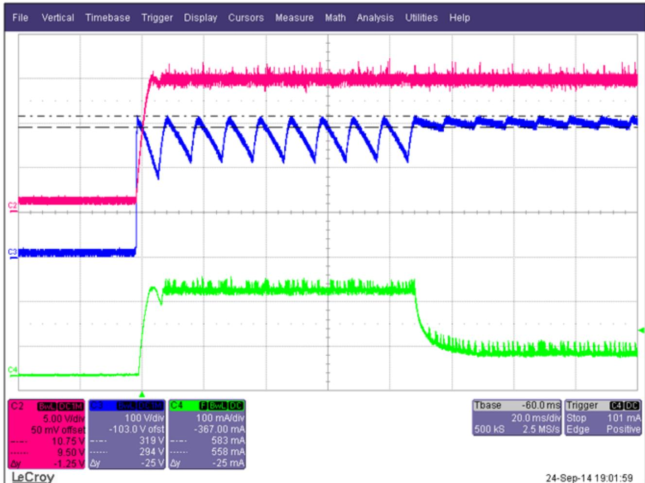
Ch2 - Regulated supply voltage of DRV110 ( $V_{IN}$ ) Ch3 – Rectified voltage Ch4 – Solenoid current
