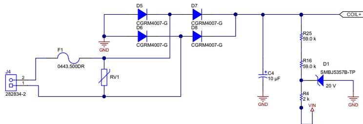
Figure 7. Input Supply and Voltage Regulation Circuit for DRV110
