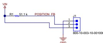
**Figure 16. Hall Sensor Connector Circuit**
