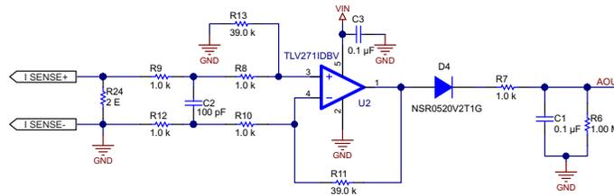
**Figure 14. Solenoid Current Amplification Stage**
