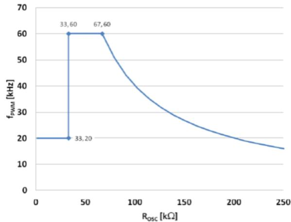
Figure 13. PWM Clock Frequency Setting for DRV110
