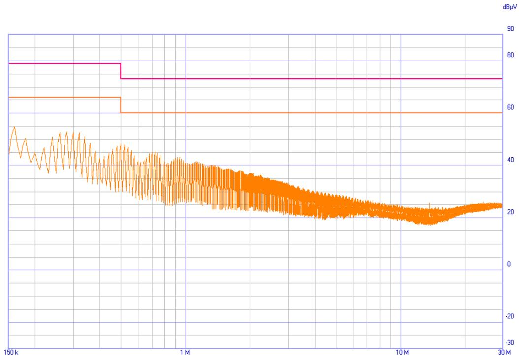
**Figure 31. EMC Test Results — Average Detector Output**
