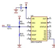
Figure 10. EN Signal Control Circuit
