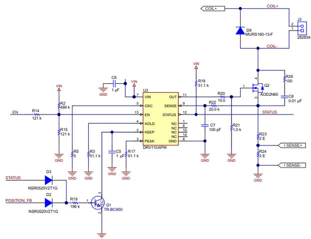
Figure 8. DRV110 Circuit and Solenoid Current Control Circuit
