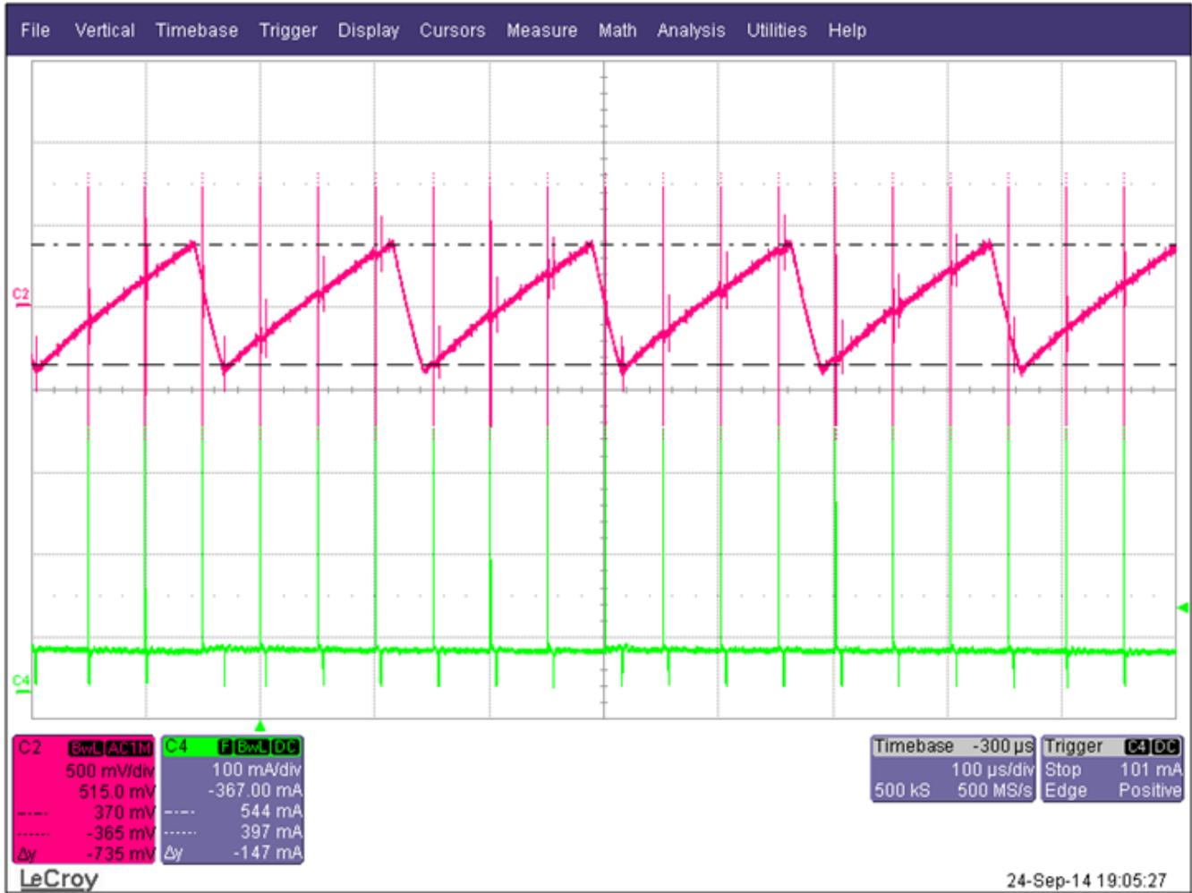
Ch2 – Ripple in regulated supply voltage of DRV110 ( $V_{IN}$ )
