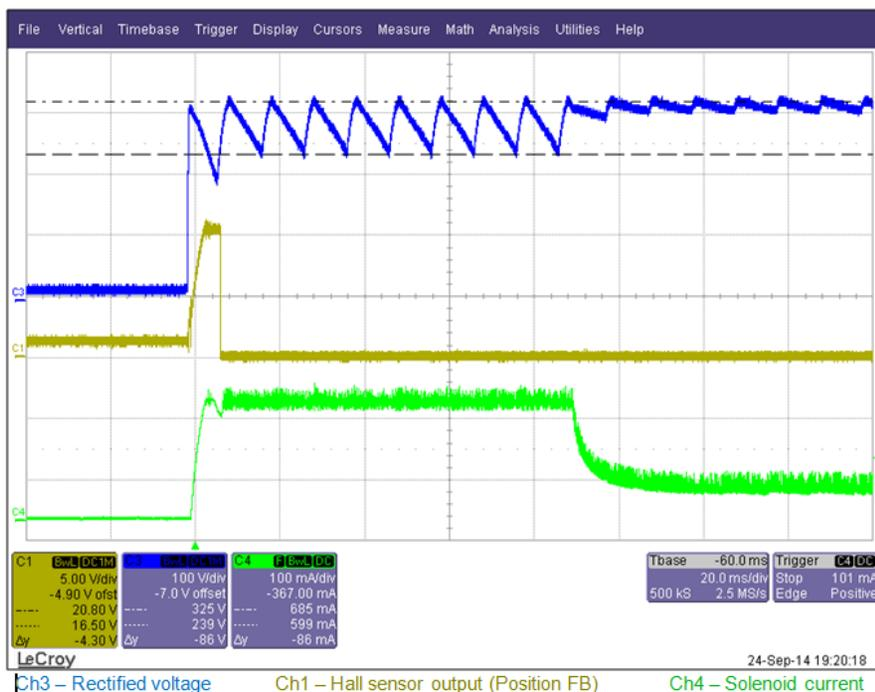
Figure 27. Test Results at the 230-V AC Input
