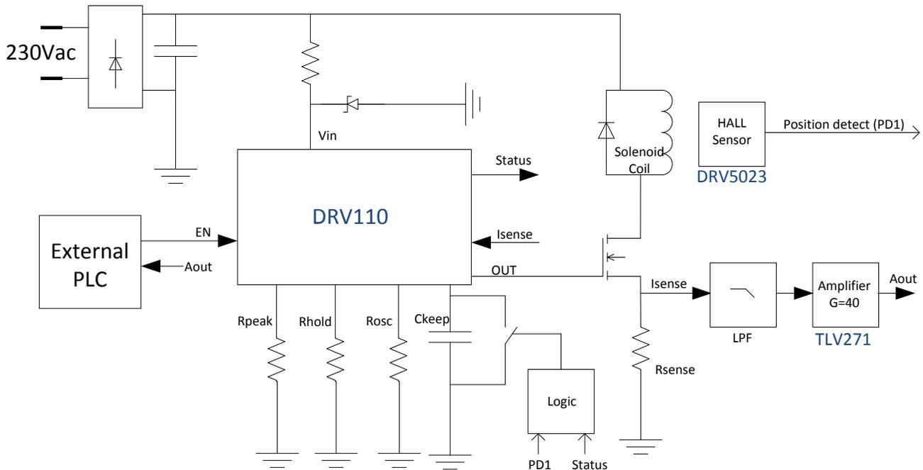
**Figure 6. Block Diagram of the Solenoid Driver Using DRV110**
