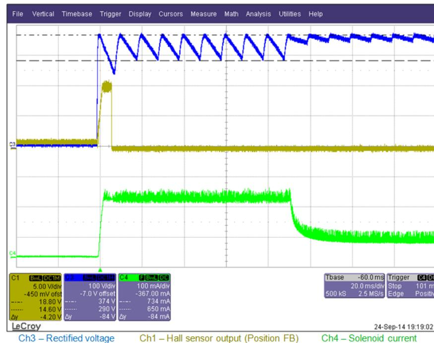
Figure 28. Test Results at the 265-V AC Input
