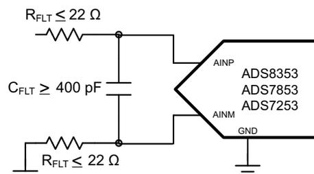
Figure 7. Anti-Aliasing Filter for ADS7x53
