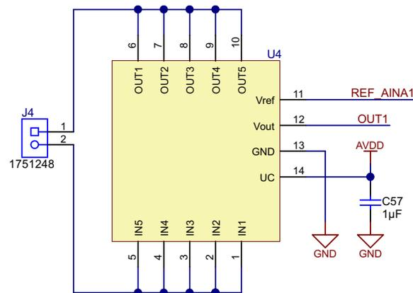
Figure 6. CKSR 6-NP with Capacitor Decoupling on Supply Pin
