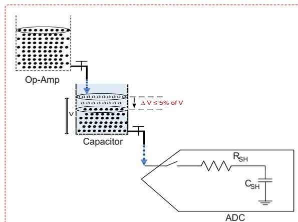
Figure 9. Filter Capacitor Delivering Charges to  $C_{SH}$
