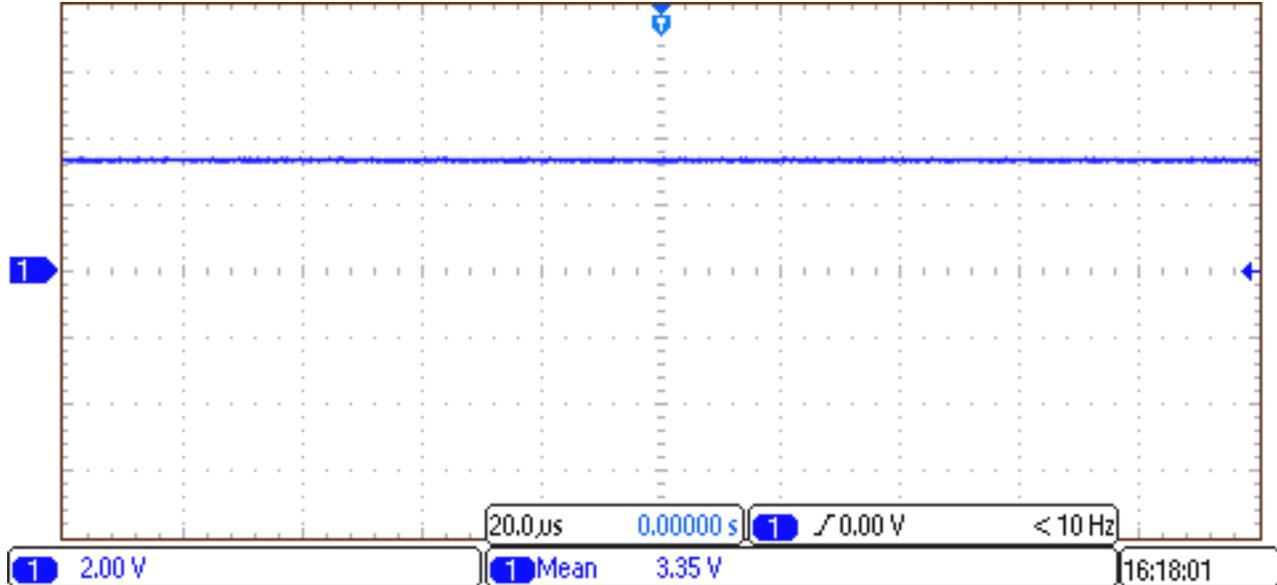
Figure 41. 3.3-V Reference Signal Generated by TLV70033
