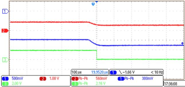
**Figure 51. Earth Fault Detection at VTH (neg)**
