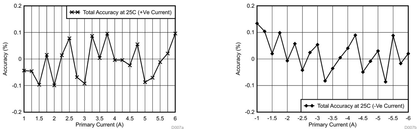
Figure 38. Total Accuracy While Using Internal ADC of Piccolo 28027 Controller (Left) for Positive Current (Right) for Negative Current
