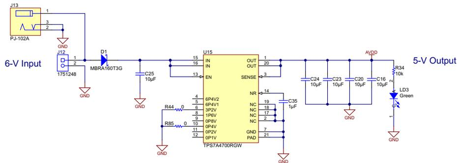
Figure 16. 6- to 5-V Conversion Using TPS7A4700
