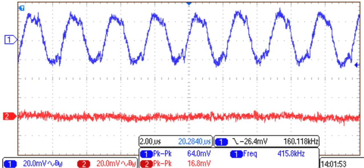
Figure 24. Noise Signal Before and After the Low-Pass Filter
