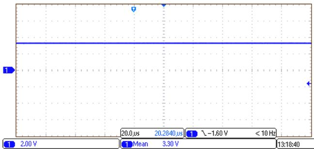
Figure 43. 3.3-V Reference Signal Generated by REF2033
