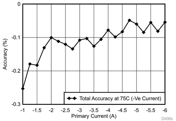
**Figure 36. Total Accuracy at 75°C (Left) for Positive Current (Right) for Negative Current**
