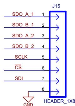
Figure 21. SPI Signals of External ADCs Taken Out on a Connector
