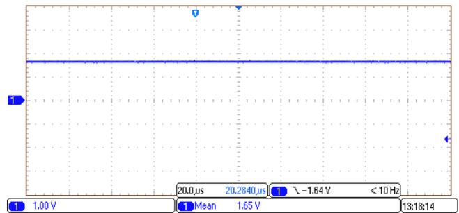
Figure 44. 1.65-V Reference Signal Generated by REF2033
