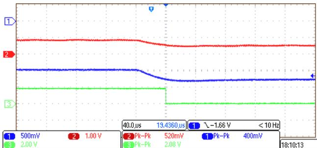
Figure 47. Overcurrent Detection at VTH (neg)
