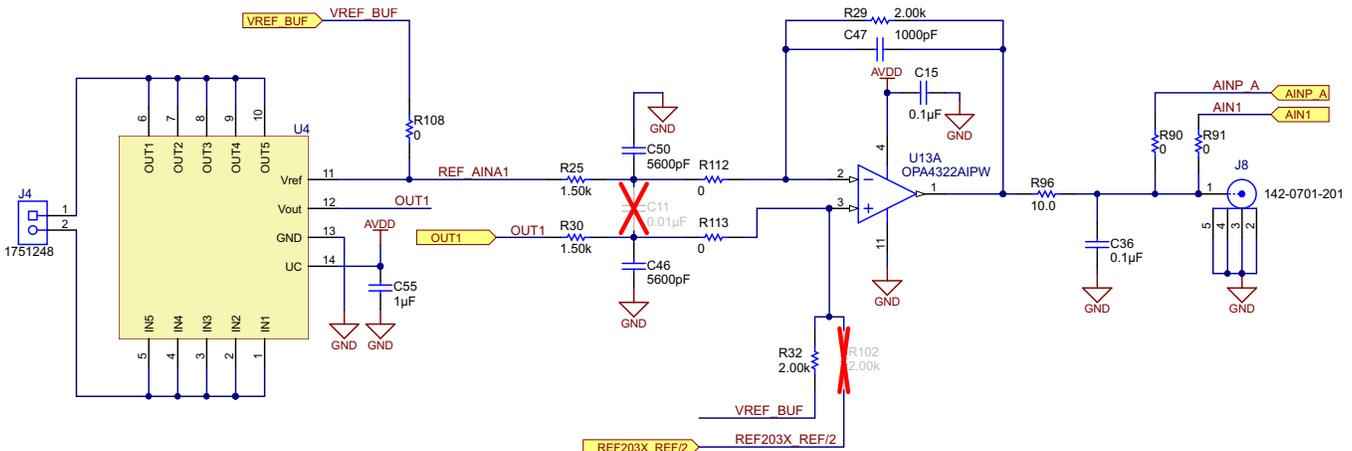
Figure 10. OPA4322 Interface Between Sensor and ADC
