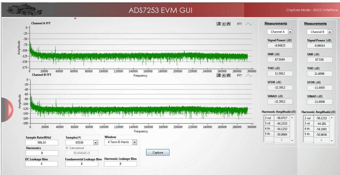
Figure 29. FFT and SNR Shown for Two Channels Using ADS7253 EVM GUI
