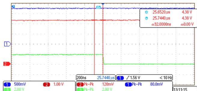
Figure 50. Earth Fault Detection at VTH (pos) — Zoomed
