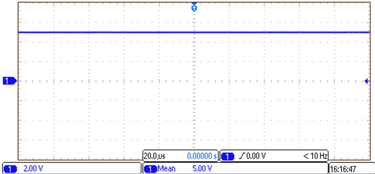
Figure 40. 5-V Signal From TPS7A4700
