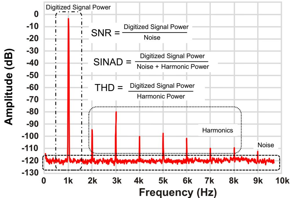
Figure 27. Typical FFT Plot Showing Different Dynamic Parameters
