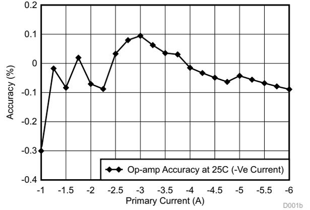
Figure 31. Op-Amp Accuracy at 25°C (Left) for Positive Current (Right) for Negative Current
