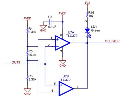
Figure 18. Overcurrent Protection Using TLC372
