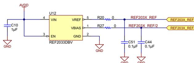
Figure 15. REF2033 Circuit to Provide 1.65 V and 3.3 V as Reference
