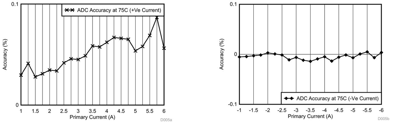
**Figure 34. ADC Accuracy at 75°C (Left) for Positive Current (Right) for Negative Current**
