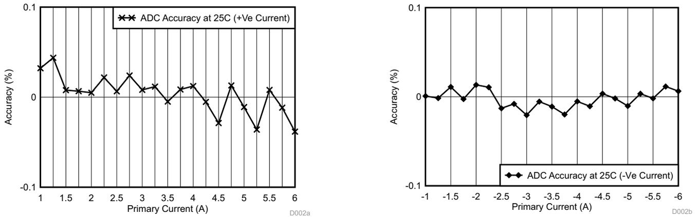
**Figure 33. ADC Accuracy at 25°C (Left) for Positive Current (Right) for Negative Current**
