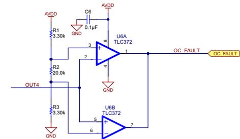
CH4 OVERCURRENT FAULT DETECTION
