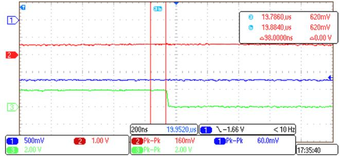
**Figure 52. Earth Fault Detection at VTH (neg) — Zoomed**
