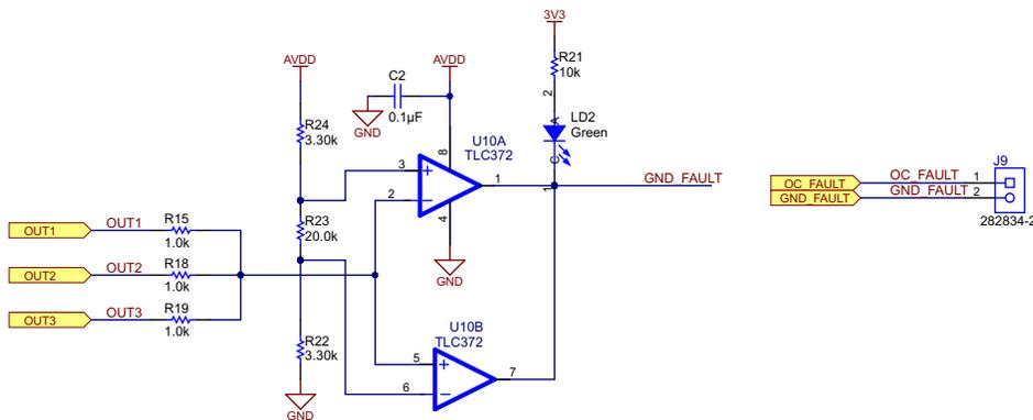
Figure 19. Earth Fault Protection Using TLC372
