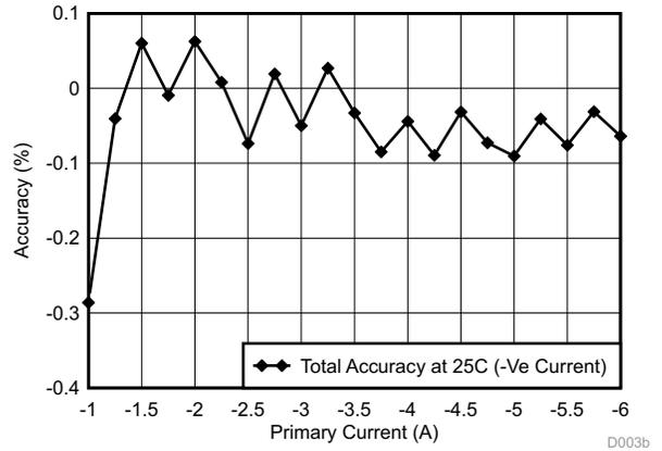
**Figure 35. Total Accuracy at 25°C (Left) for Positive Current (Right) for Negative Current**
