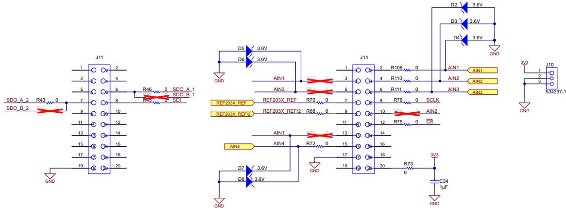
Figure 23. Schematic Capture for J11 and J14 (To Be Connected to 40-Pin Connector on LaunchPad)
