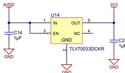
Figure 17. 5- to 3.3-V Conversion Using TLV70033
