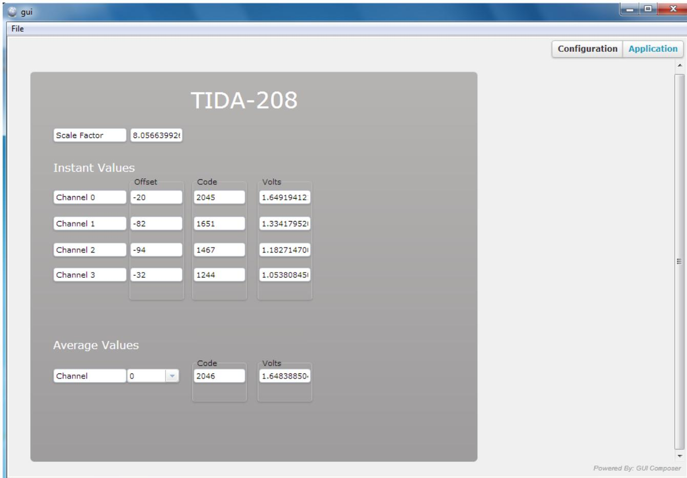
Figure 37. Screenshot of Internal ADC GUI for Piccolo Controller
