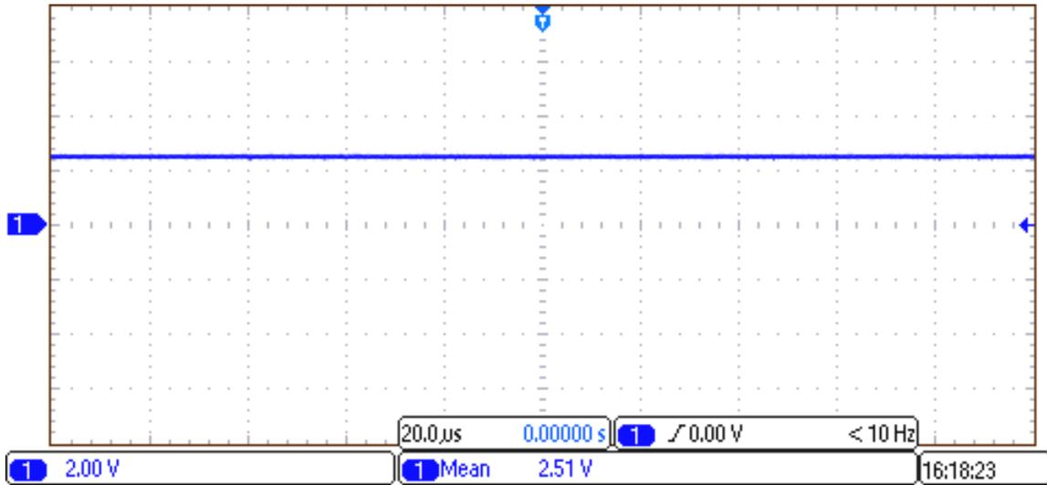
Figure 42. 2.5-V Reference Signal Generated by REF5025
