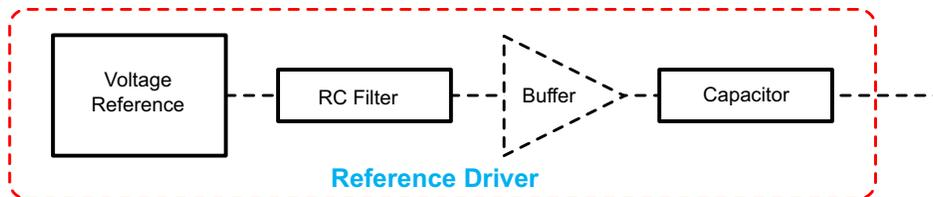
**Figure 12. Reference Driver Circuit**
