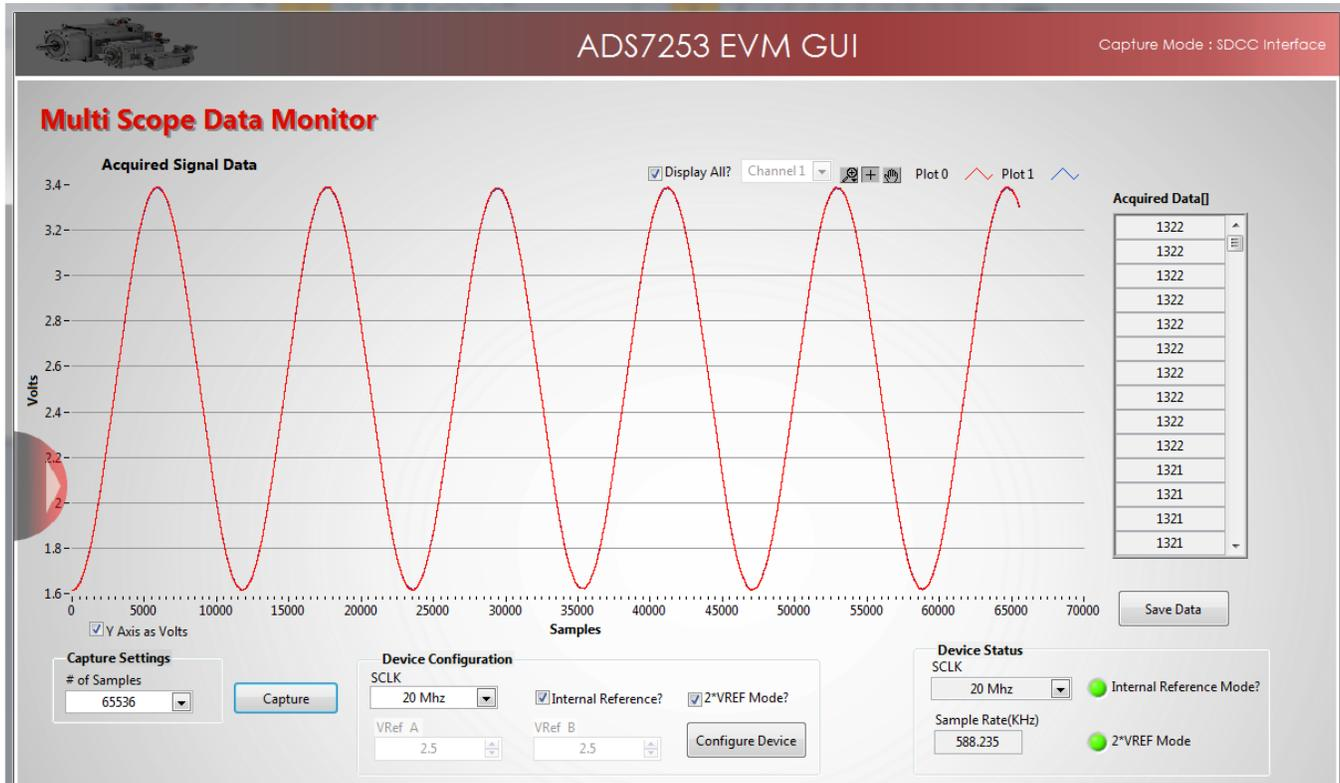
Figure 28. AC Signal Capture for Two Channels Using ADS7253 EVM GUI
