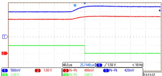
Figure 49. Earth Fault Detection at VTH (pos)
