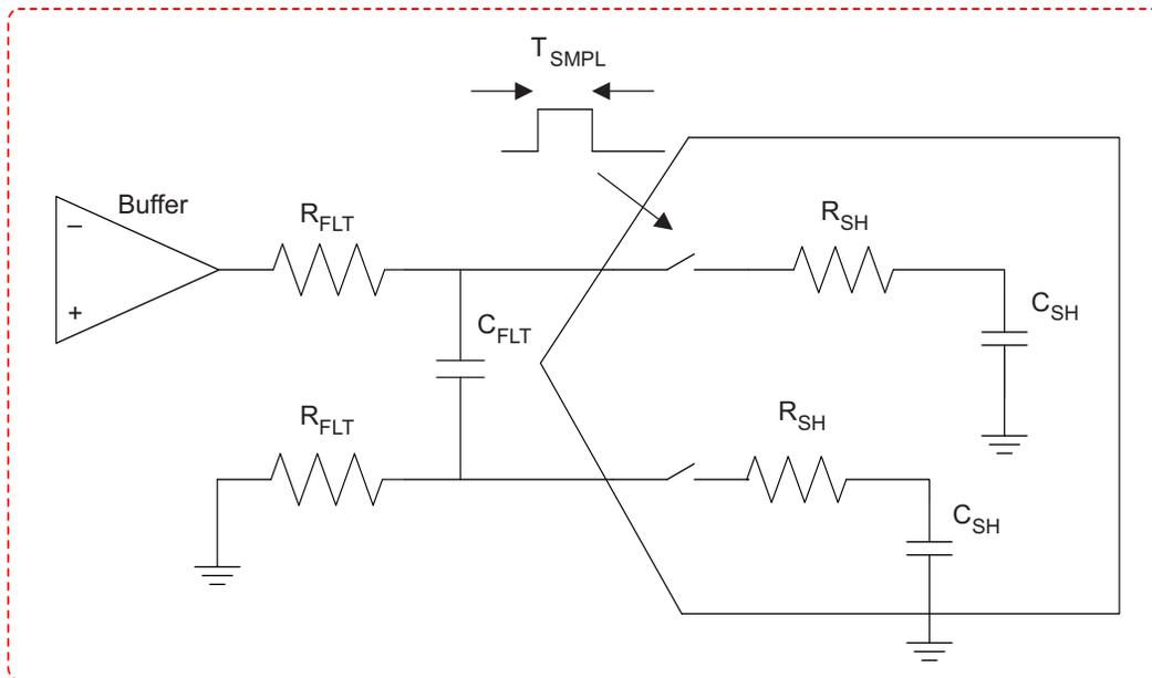
Figure 8. Input Capacitor  $C_{FLT}$  for Attenuating Noise
