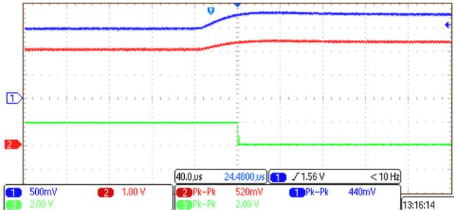
Figure 45. Overcurrent Detection at VTH (pos)
