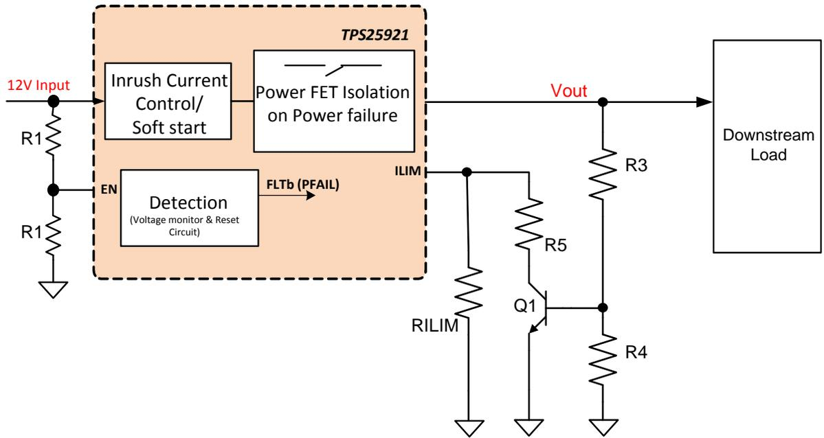
Figure 1: Block Diagram Precision Power Limiting Solution
