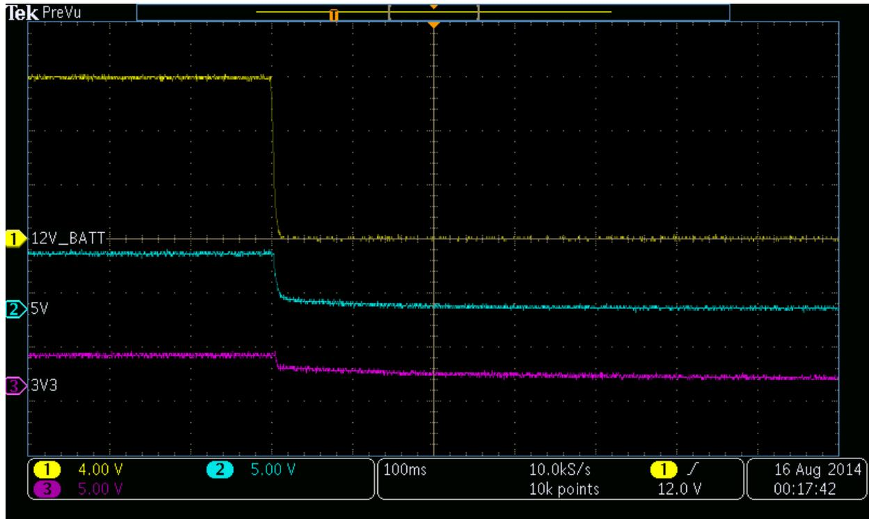
Figure 2 – Shut-down sequence
