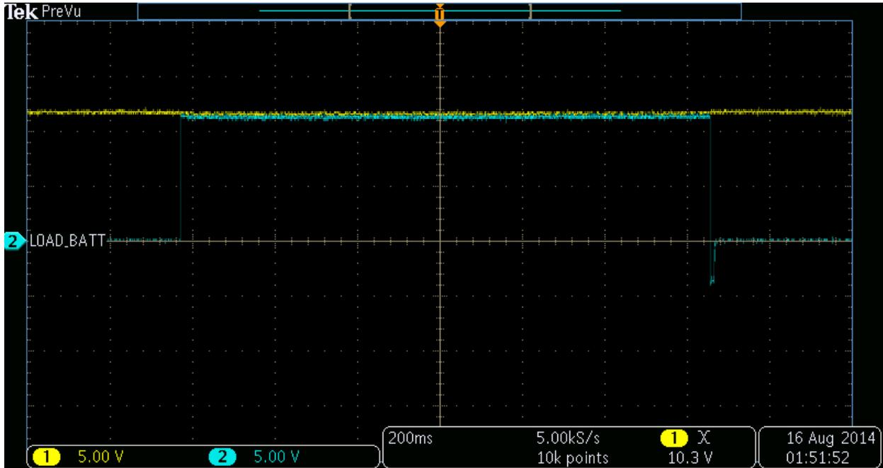
Figure 5 – LMD18400 drive test
