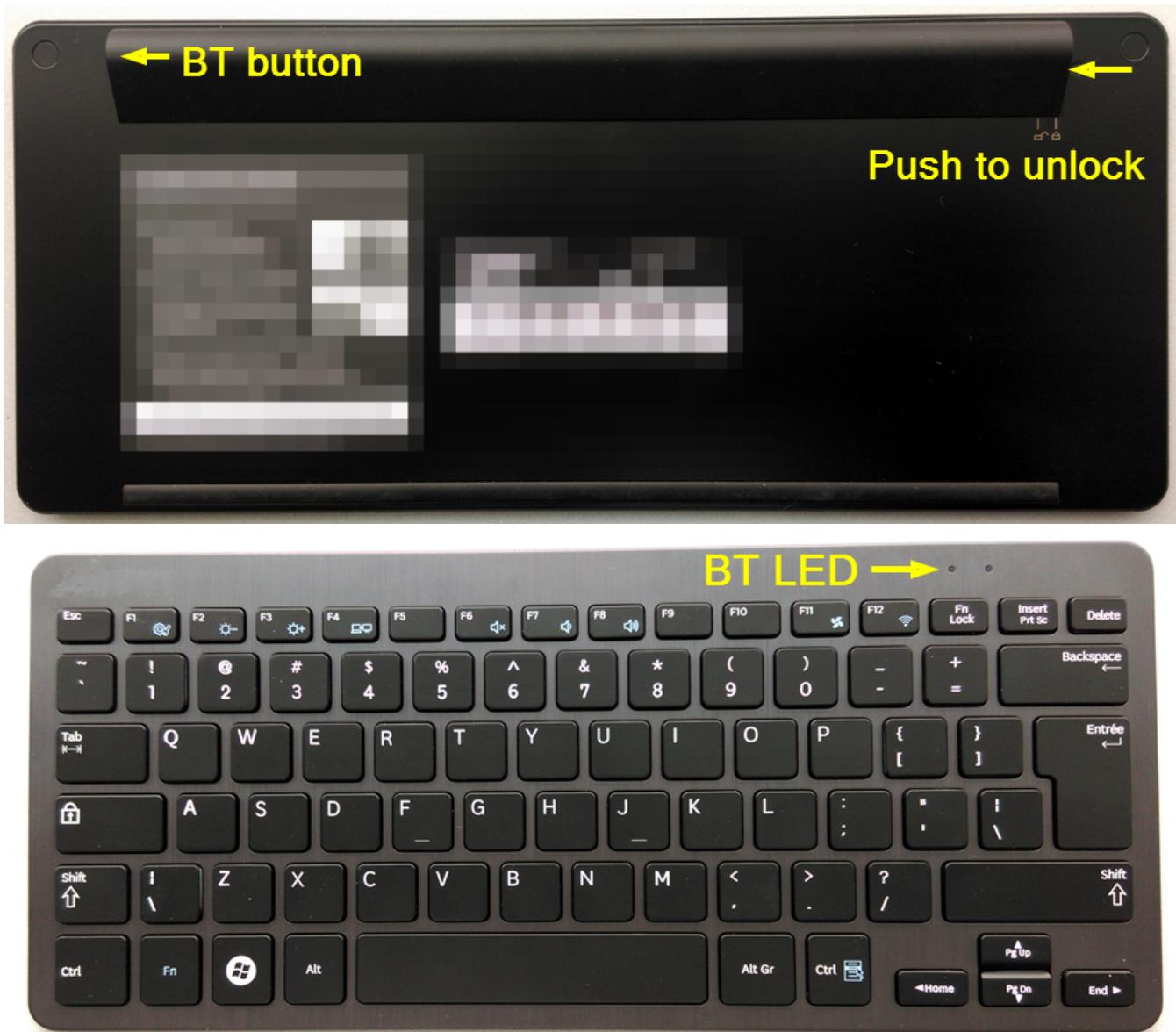
Figure 7. BT Button and LED
