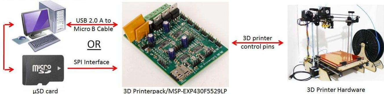
**Figure 1. 3D Printer System Diagram**
