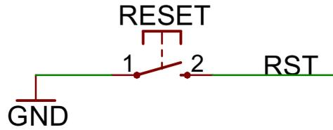
Figure 22. Reset Schematic
