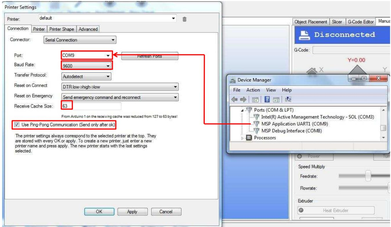
Figure 10. Printer Settings in Repetier
