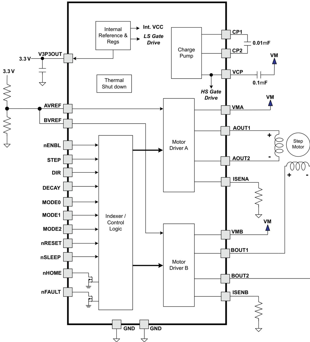
Figure 3. DRV8825 Functional Diagram
