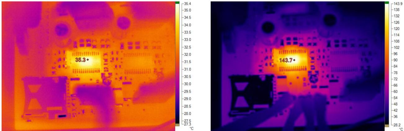
**Figure 14. DRV8825 Temperatures, Printer Operation on the Left and Maximum Operation on the Right**
