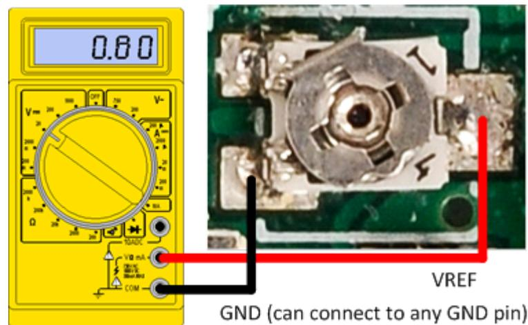
Figure 7. Tuning the VREF Potentiometers
