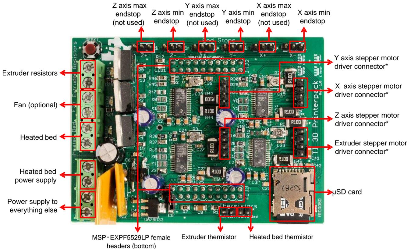
\*Stepper motor connectors can be flipped if motion on 3D printer is opposite of that expected
