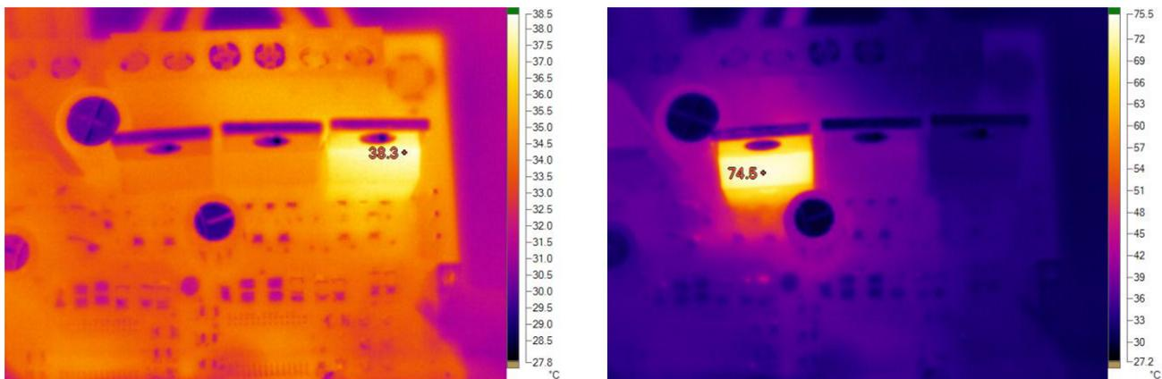
**Figure 15. CSD18534KCS Temperatures, Extruder Resistors on the Left and Heated Bed on the Right**
