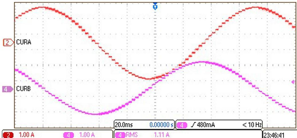
Figure 13. Output Current vs. Step Input for Maximum Driver Operation
