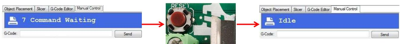
Figure 11. Printerpack Reset to Enable UART Communication
