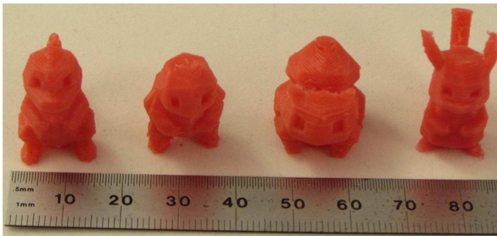
**Figure 17. Small Figurines Printed to Demonstrate Small Feature Sizes**
