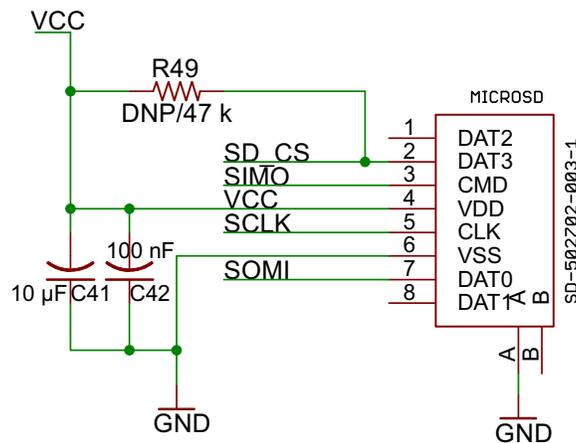
Figure 25. microSD Memory Card Schematic
