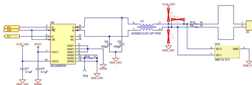
Figure 12. Isolated Transceiver
