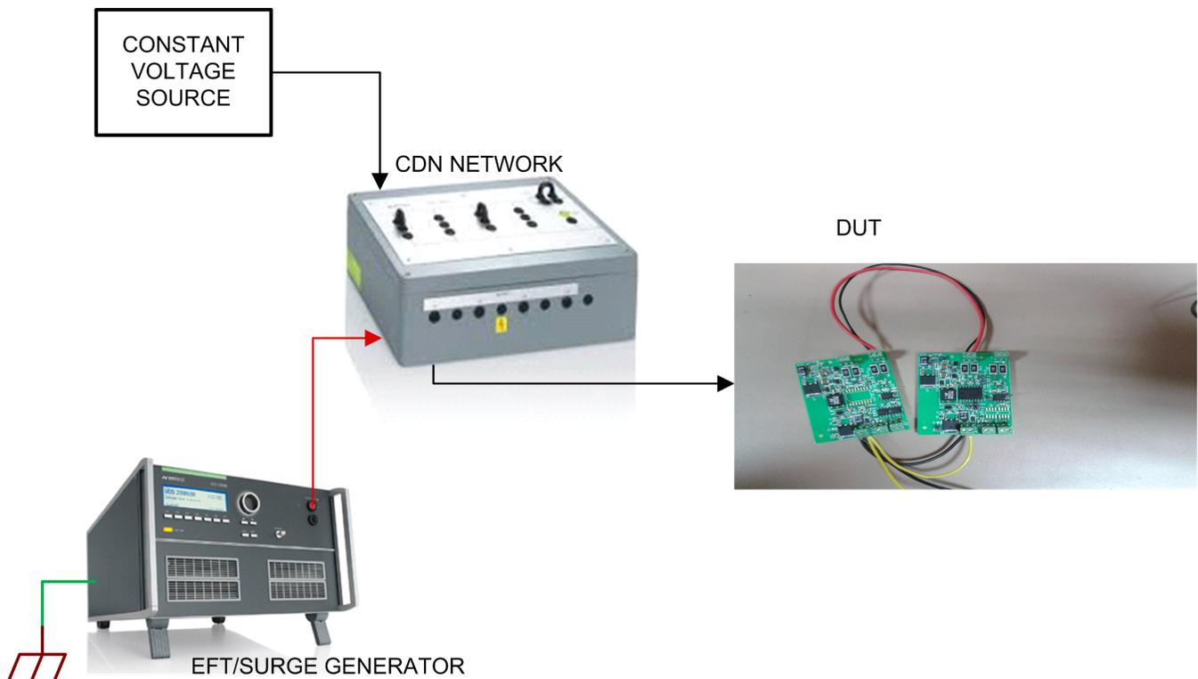
**Figure 23. Surge Setup for RS-485 Communication Board**
