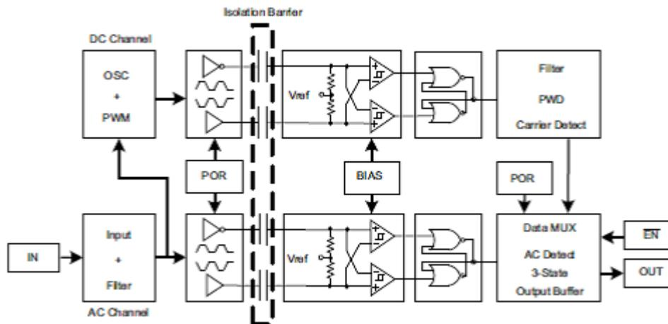
Figure 8. : ISO72x Isolator Internal Diagram
