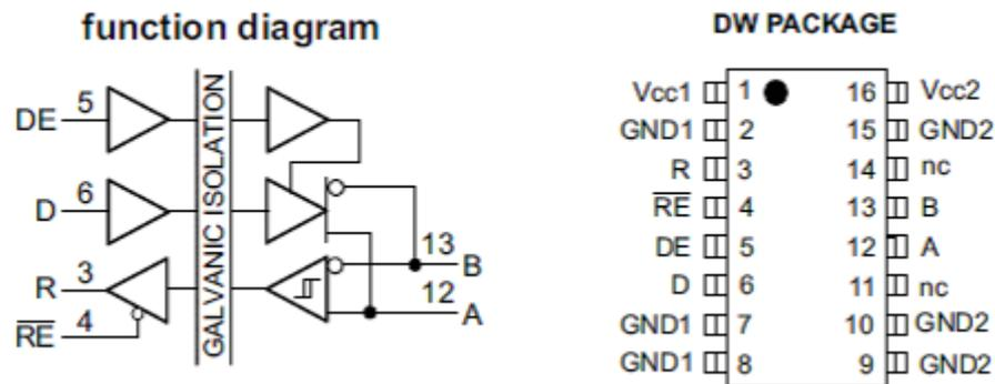
**Figure 7. The ISO15, ISO3082, and ISO3088 Half-Duplex Function Diagram and Pinout**
