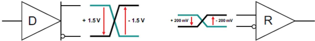
**Figure 1. RS-485 Specified Minimum Bus Signal Levels**
