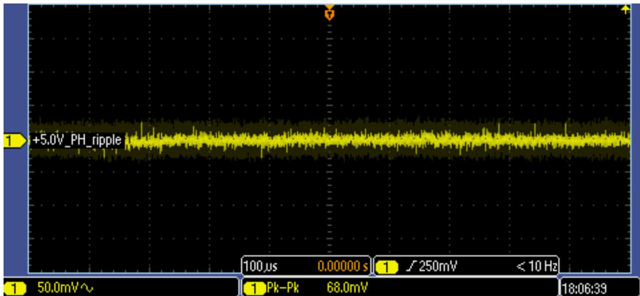
**Figure 19. Ripple on +5.0V\_VDC**
