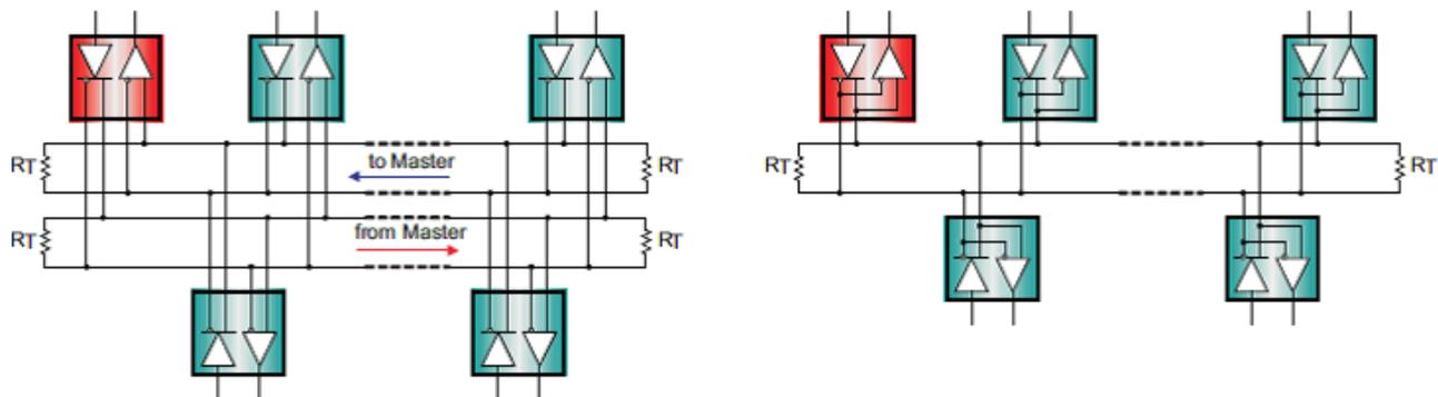
**Figure 3. Full-duplex and Half-Duplex Bus Structures in RS-485**
