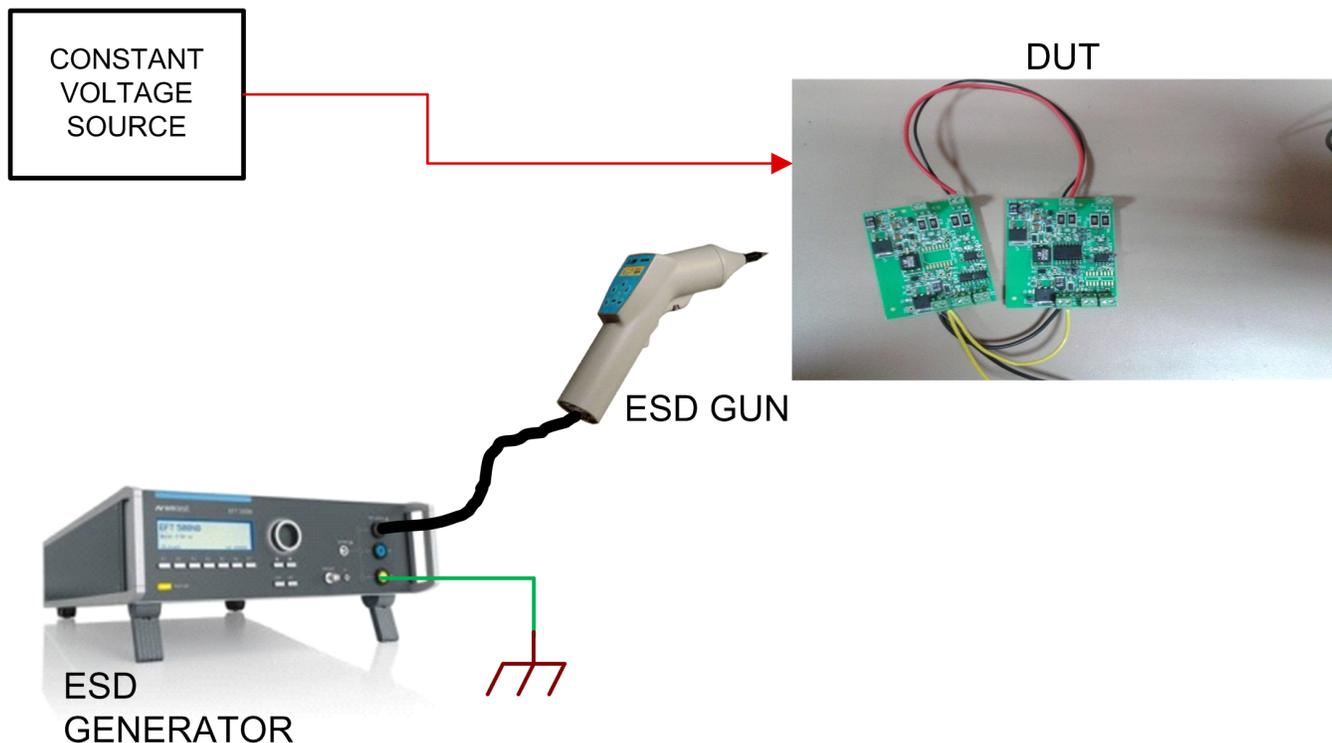
**Figure 22. ESD Setup for RS-485 Communication Board**
