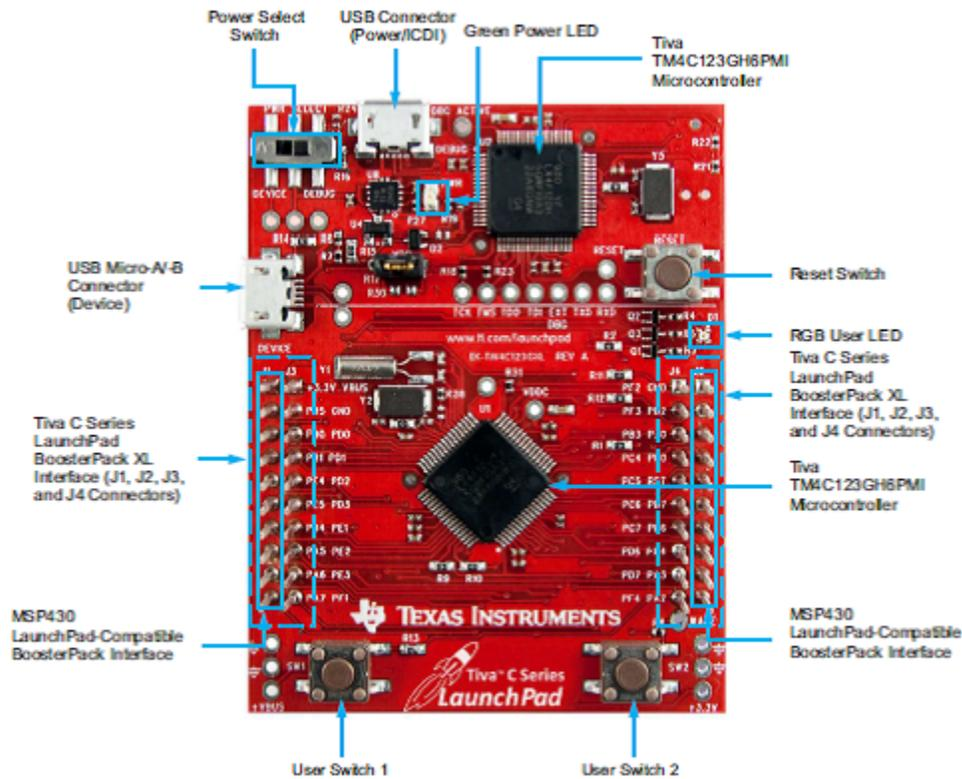
**Figure 18. Tiva C Series TM4C123G LaunchPad Evaluation Board**
