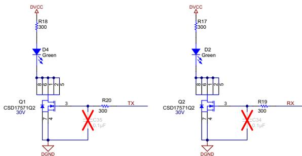
Figure 17. Communication Indication LEDs
