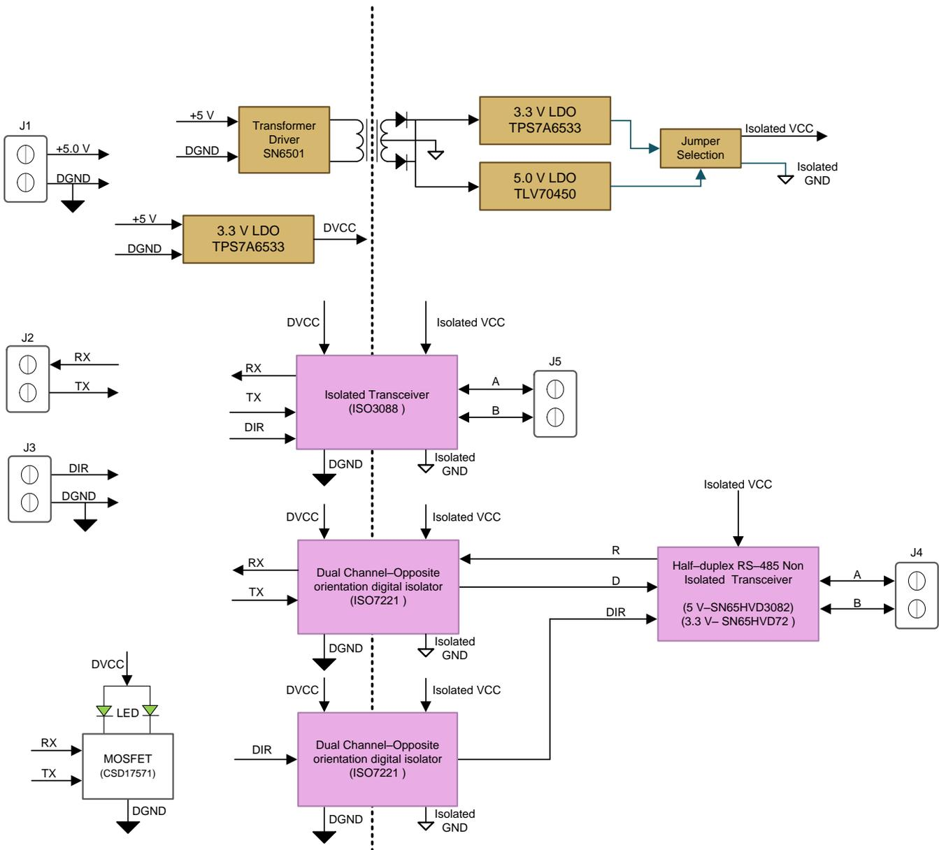
Figure 11. RS-485 Interface Module Block Diagram
