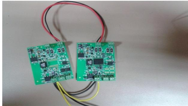
**Figure 21. Two RS-485 Boards Daisy-Chained**
