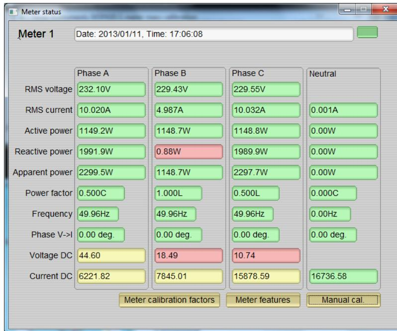
Figure 32. Metrology GUI Showing Metrology Parameter Values
