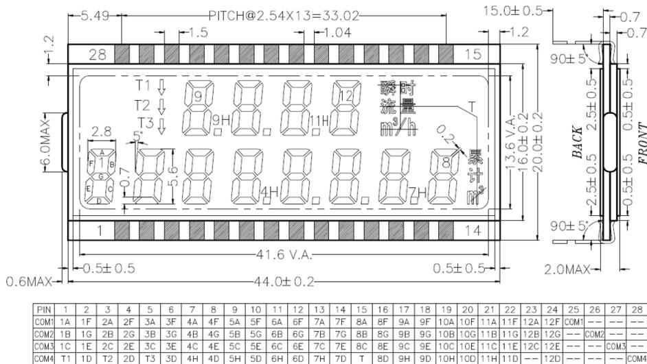
Figure 12. LCD Specification
