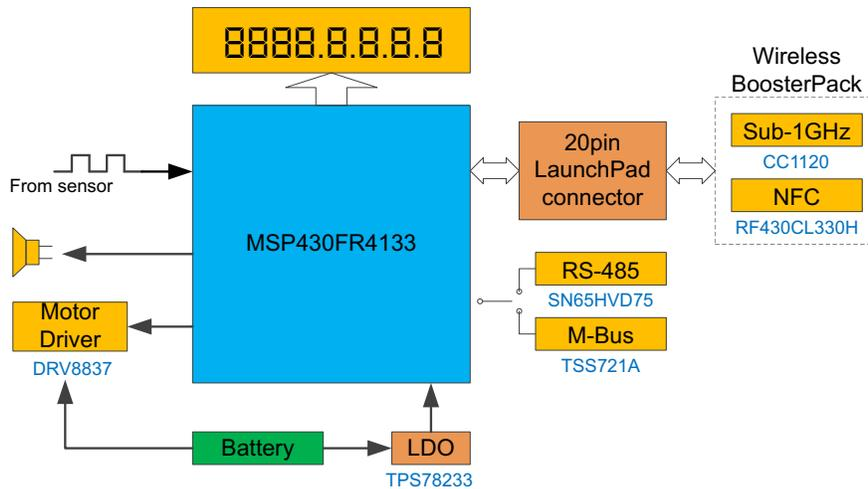
Figure 7. Block Diagram
