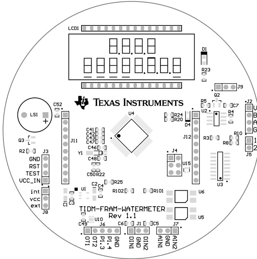
Figure 33. Top Assembly Drawing
