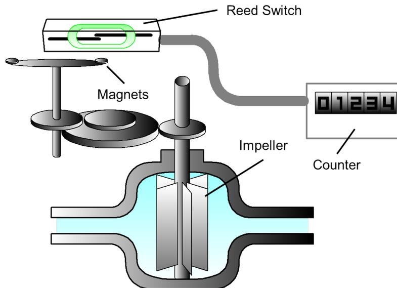
**Figure 4. Electromagnetic Pulse Measure Principle**
