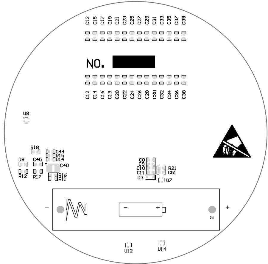
Figure 34. Bottom Assembly Drawing
