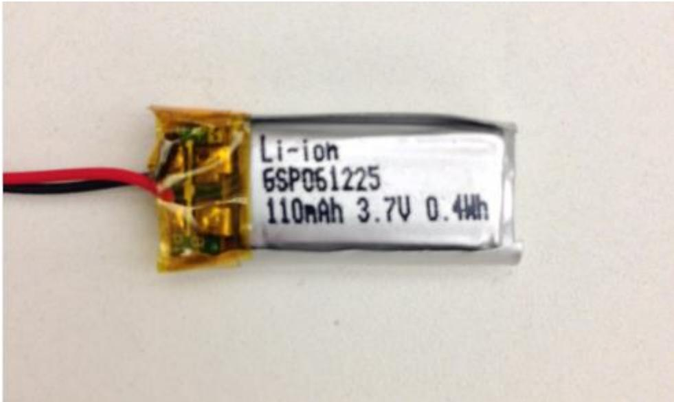
**Figure 5. 110 mAh Li-Ion Battery Pack**
