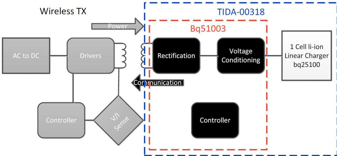
Figure 4. Block Diagram
