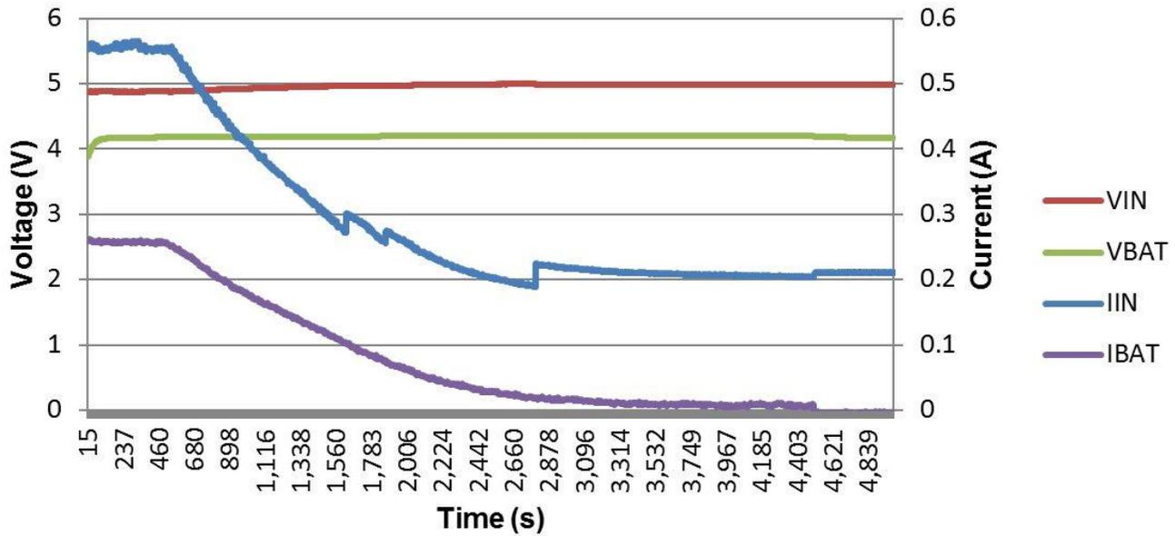
Figure 7. 4.2 V 250 mA Charge Cycle with 10 mA Charge Termination
