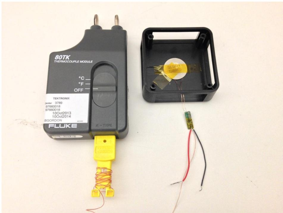
**Figure 6. FLUKE 80TK Thermal Couple**
