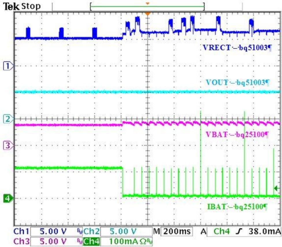
**Figure12. IBAT Load Transition from 100 mA to 0 mA**
