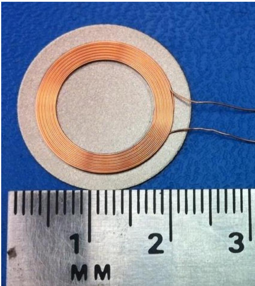
Figure 3. Receiver Coil
