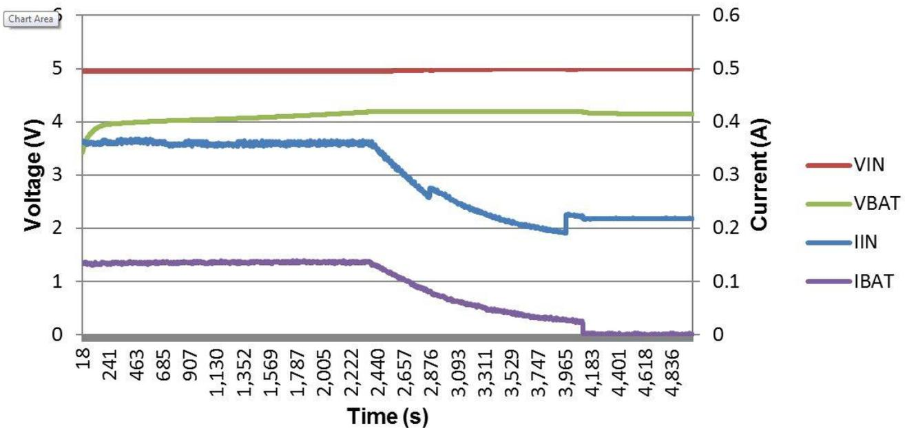
Figure 8. 4.2 V 135 mA Charge Cycle with 20 mA Charge Termination
