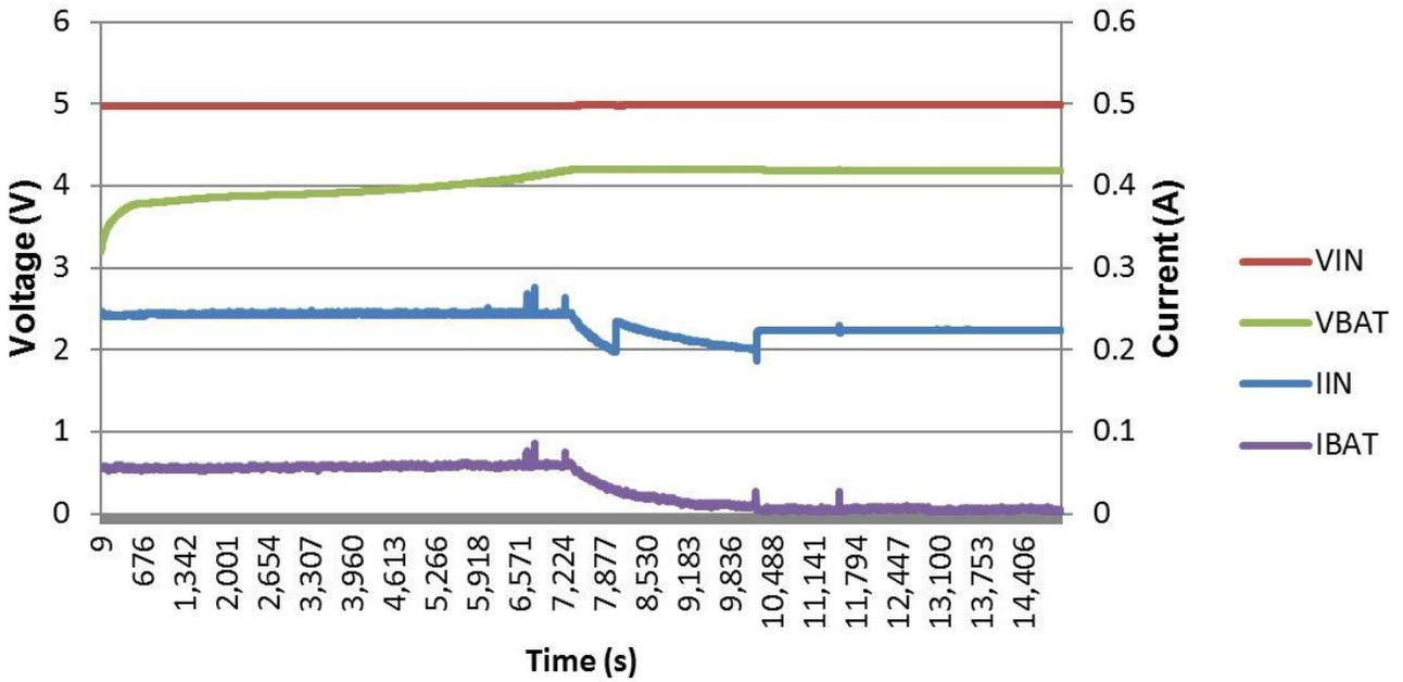
**Figure 9. 4.2 V 60 mA Charge Cycle with 1 mA Charge Termination**
