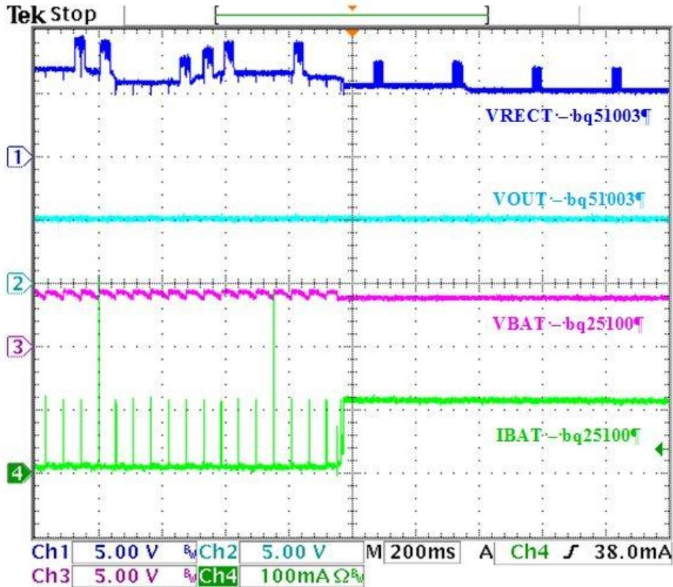
Figure 11. IBAT Load Transition from 0 mA to 100 mA
