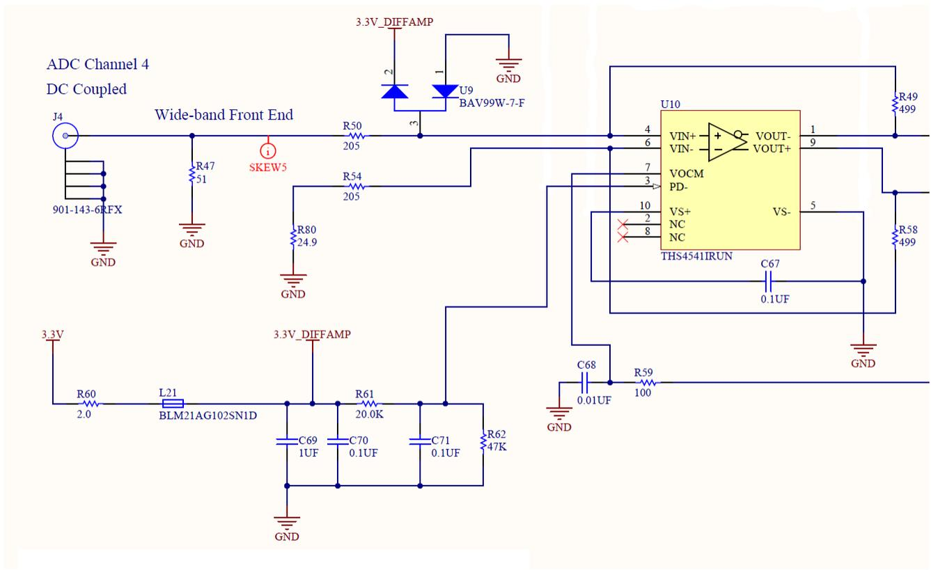
Figure 2. Amplifier Power Supply and Power Down option
