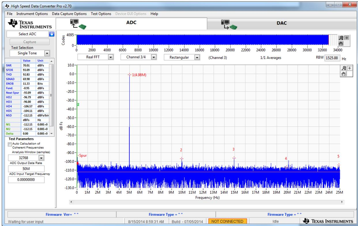
Figure 6. FFT performance of THS4541+ADC34J22 active interface
