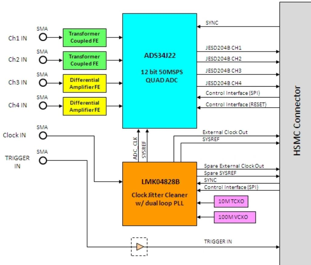
Figure 1. DEV-ADC34J22 block diagram.
