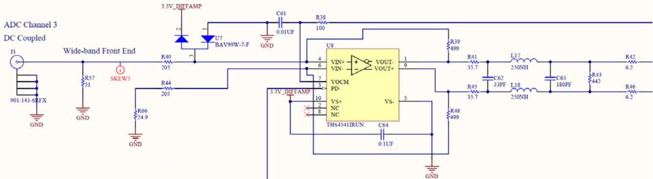
Figure 4. THS4541 circuit implementation with 20M Bessel LPF driving ADC34J22
