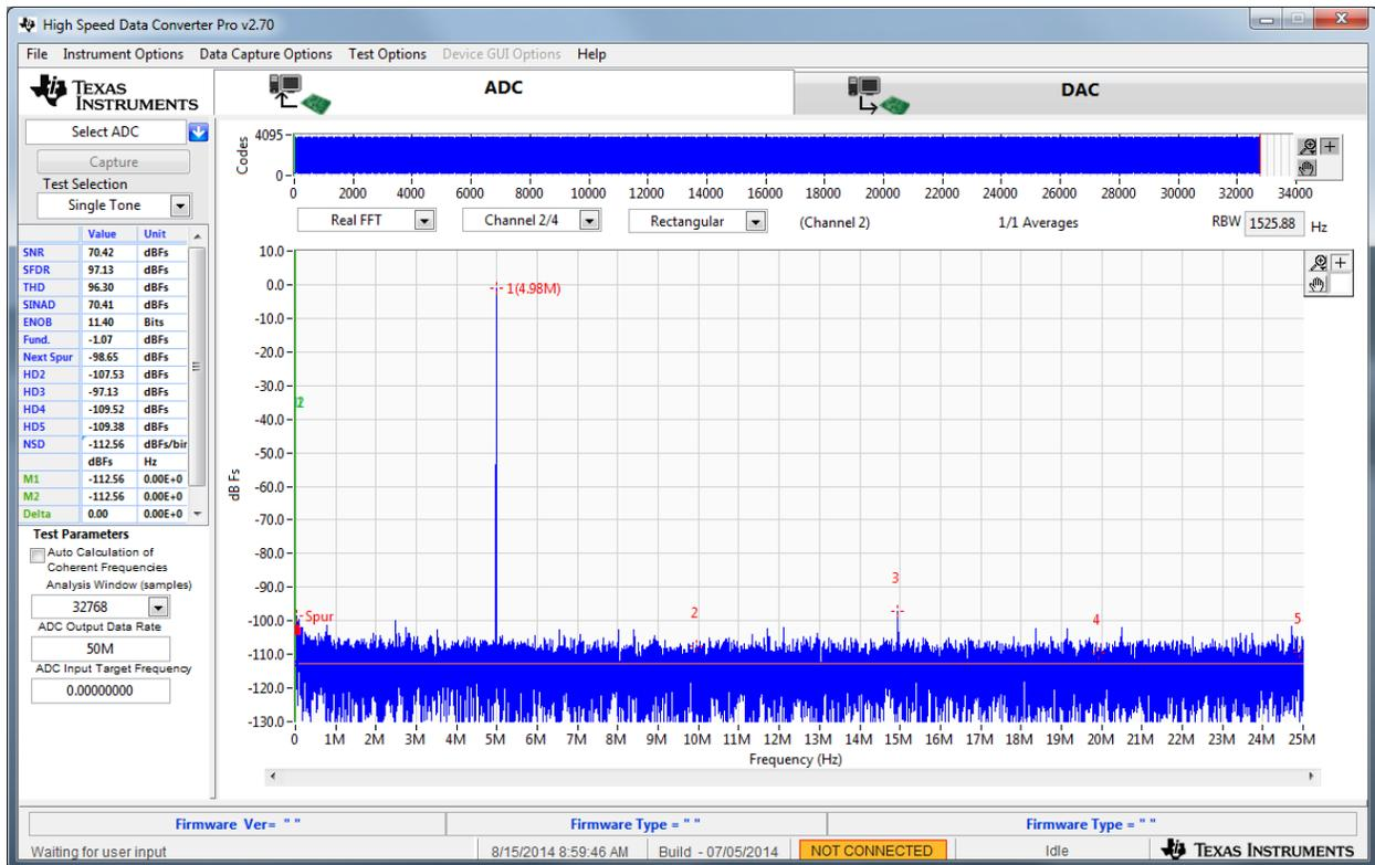
Figure 5. FFT performance of the ADC34J22 with transformer interface
