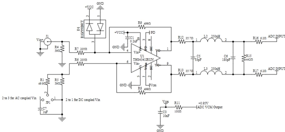
Figure 3. Example implementation of the THS4541 with 20MHz Low Pass interstage filter prior to ADC inputs.
