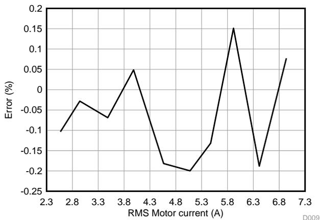
Figure 94. Motor Current versus Error, Tested with Motor Drive and Load Setup
