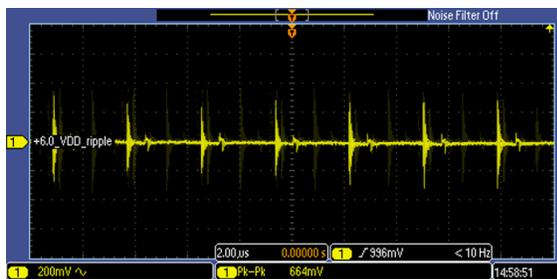
Figure 102. Ripple on 6.0\_VDD Power Rail, FMB Board
