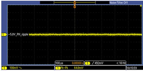
Figure 116. -5.0V\_PH Power Rail on DSM Board, Measured Across Capacitor C84, with Motor Turned On
