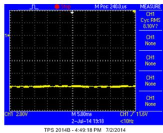
Figure 124. -6.0V\_USH Power Rail on DSM Board, Measured Across Capacitor C33, with Motor Turned On
