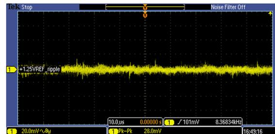
Figure 107. Ripple on 1.25-V Reference Voltage from REF3012, on FMB Board
