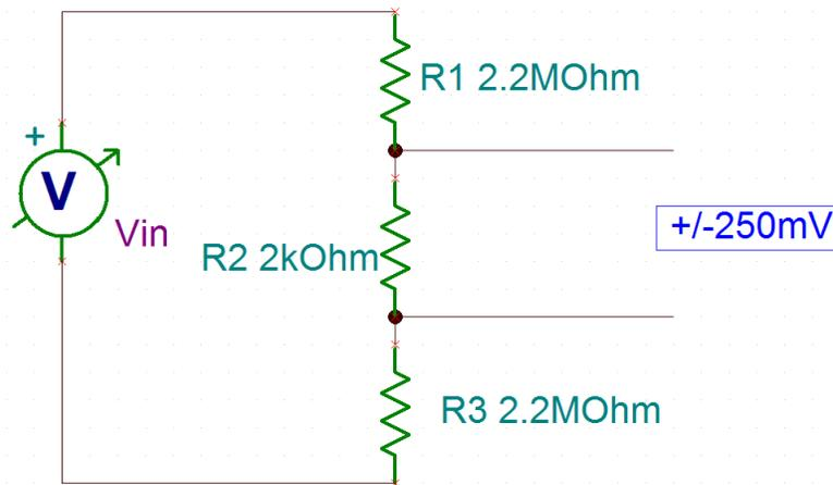
Figure 28. Phase-to-Phase Resistor Divider
