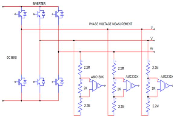
Figure 26. AMC1304 for Phase-to-Phase Voltage Measurement
