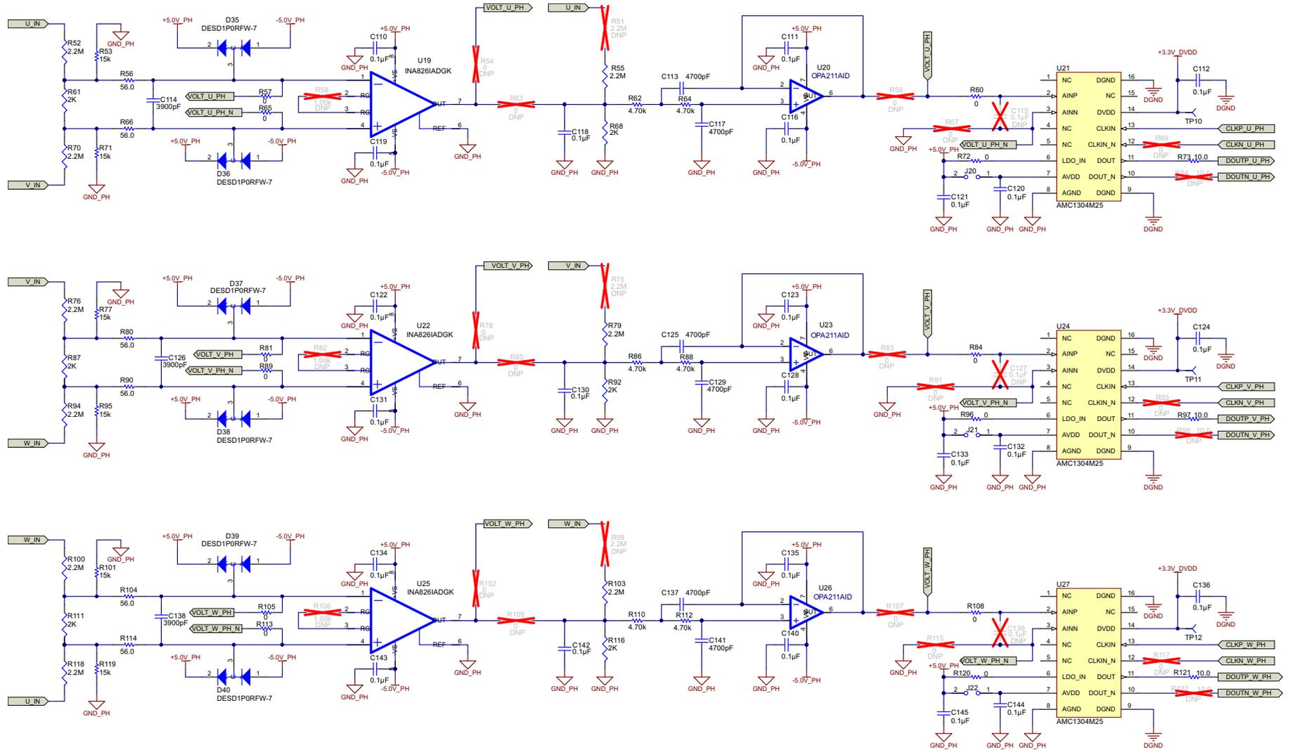
Figure 136. Voltage Conditioning Schematic
