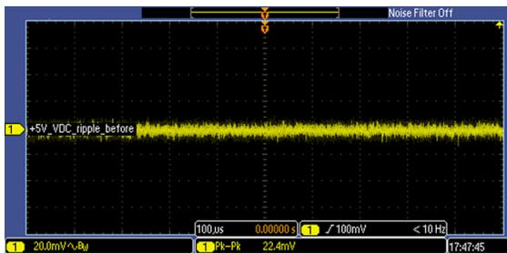
Figure 112. Ripple on 5.0V\_PH Power Rail on DSM Board, Measured Across Capacitor C96, with Motor Turned Off
