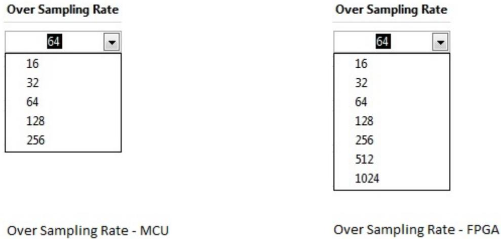
**Figure 68. Over Sampling Rate Selection**
