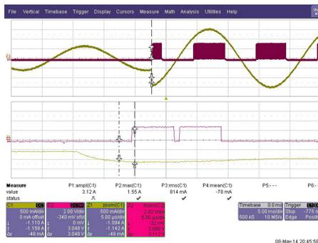
Figure 97. Short Circuit Current Waveform (Yellow) and Signal From MCU (Red) on GPIO1 Pin 10 on J2 Header on FMB Board
