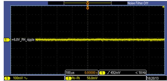
Figure 119. Ripple on 6V\_PH Power Rail on DSM Board, Measured Across Capacitor C107, with Motor Turned On
