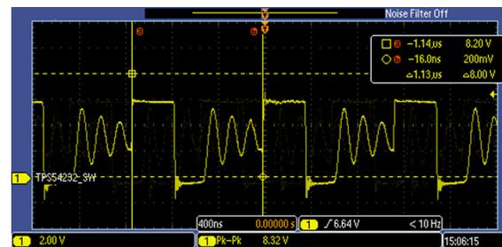
Figure 103. Switch Node Waveform for TPS54232, 6-V to 3.3-V DC-DC Converter, on FMB Board
