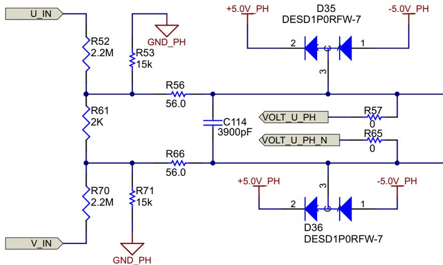
**Figure 29. Phase-to-Phase AC Voltage Direct Measurement**
