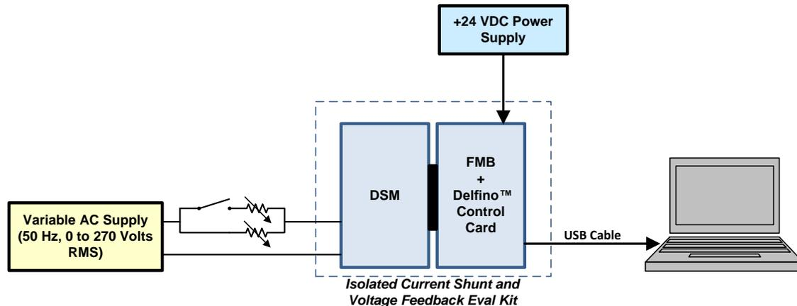
Figure 96. Test Setup for Short Circuit Testing
