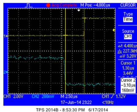
**Figure 98. Short Circuit Signal Applied to AMC1304 (Blue) and Signal From MCU (Yellow) on GPIO1 Pin 10 on J2 Header on FMB Board**
