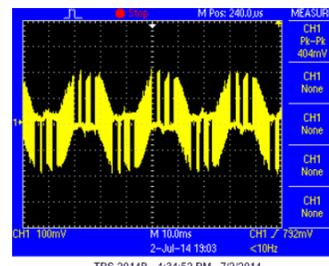
Figure 125. Ripple on -6.0V\_USH Power Rail on DSM Board, Measured Across Capacitor C33, with Motor Turned On
