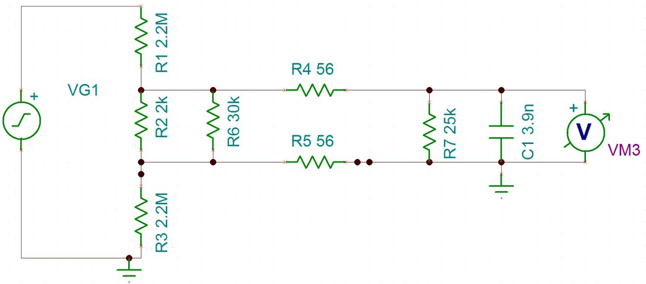
Figure 30. Direct Measurement Filter Simulation
