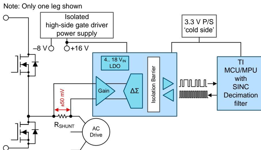
Figure 2. Delta-Sigma Modulator in Three-Phase Inverter
