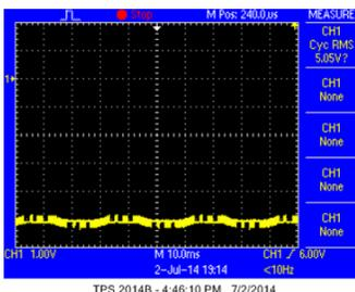
Figure 128. -5.0V\_USH Power Rail on DSM Board, Measured Across Capacitor C51, with Motor Turned On
