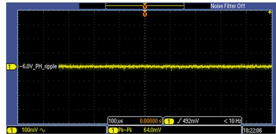
Figure 121. Ripple on -6V\_PH Power Rail on DSM Board, Measured Across Capacitor C83, with Motor Turned On
