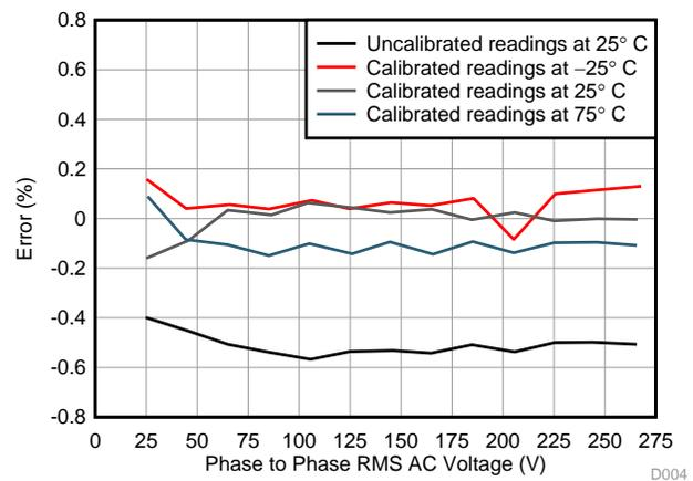
Figure 85. Phase-to-DC\_MINUS versus Error with Sallen Key
