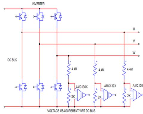
Figure 27. AMC1304 for Phase-to-DC\_MINUS Voltage Measurement
