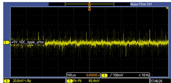
Figure 113. Ripple on 5.0V\_PH Power Rail on DSM Board, Measured Across Capacitor C96, with Motor Turned On
