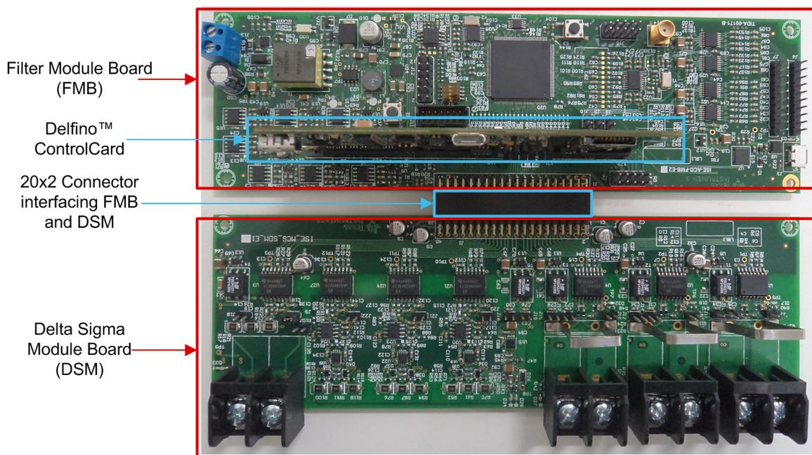
**Figure 14. Picture of Isolated Current and Voltage Measurement Kit**
