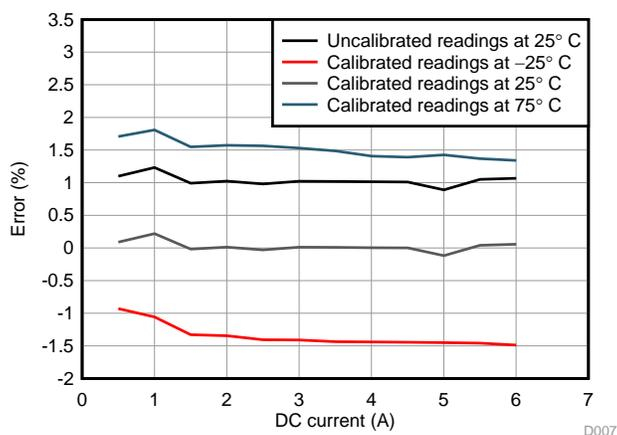
**Figure 90. DC Current versus Error**
