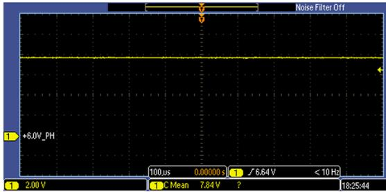
Figure 118. 6.0V\_PH Power Rail on DSM Board, Measured Across Capacitor C107, with Motor Turned On
