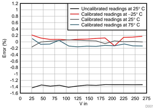
Figure 82. Phase-to-Phase Voltage versus Error
