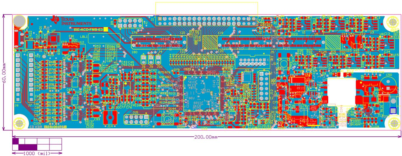
Figure 167. Multilayer Composite Print
