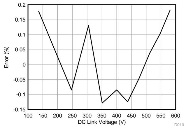
Figure 95. DC Link Voltage versus Error, Tested with Motor Drive and Load Setup
