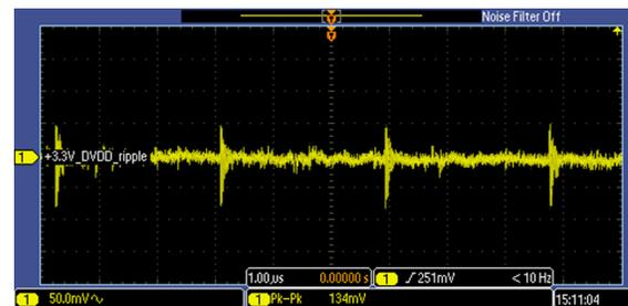
Figure 105. Ripple on 3.3V\_DVDD Power Rail, on FMB Board
