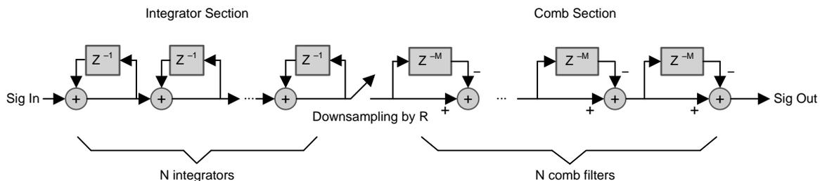
Figure 7. CIC Filter Structure
