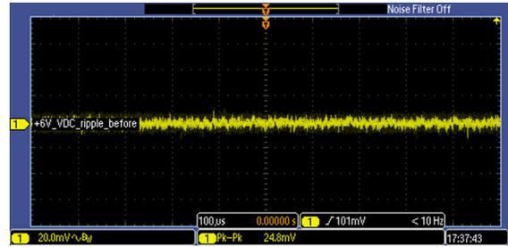
Figure 109. Ripple on 6.0V\_VDC Power Rail on DSM Board, Measured Across Capacitor C73, with Motor Turned Off
