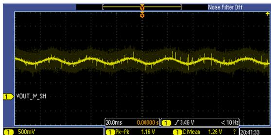
Figure 132. DAC Output, VOUT\_W\_SH, with Shunt Value of 5 mΩ
