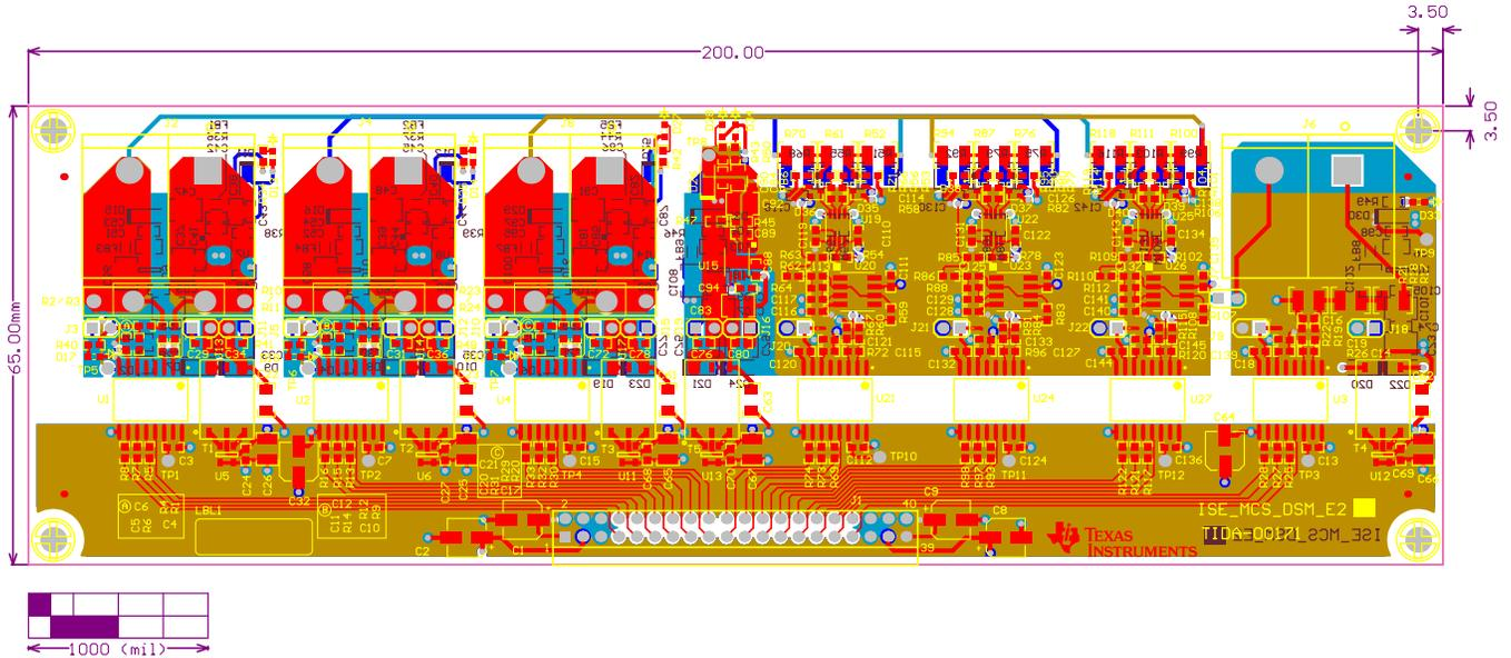
Figure 163. Multilayer Composite Print
