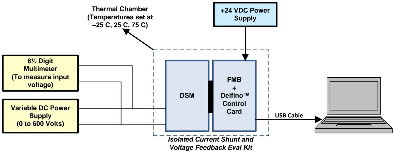
**Figure 86. Test Setup for DC Link Voltage Measurement Accuracy**
