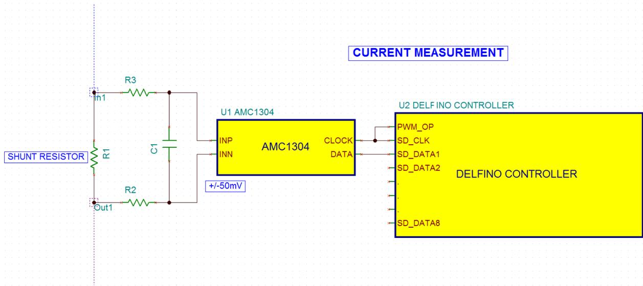
Figure 3. Current Measurement Using AMC130x and Delfino Controller
