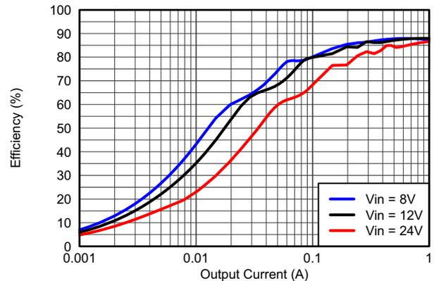
Figure 45. Light Load Efficiency
