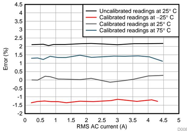
Figure 92. AC Current versus Error
