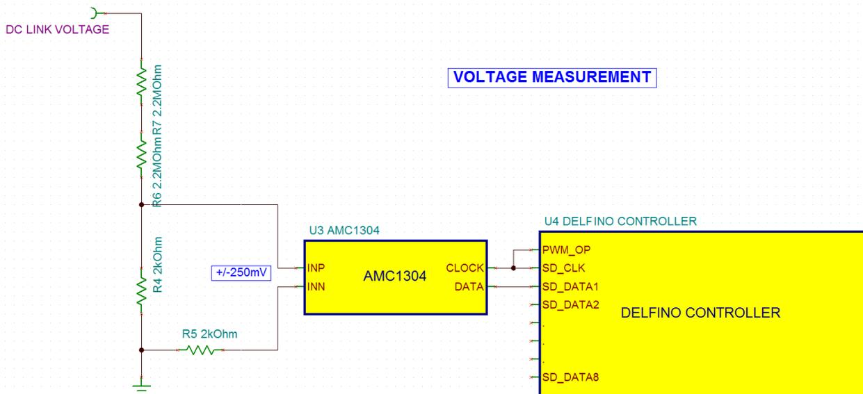
Figure 4. Voltage Measurement Using AMC130x and Delfino Controller
