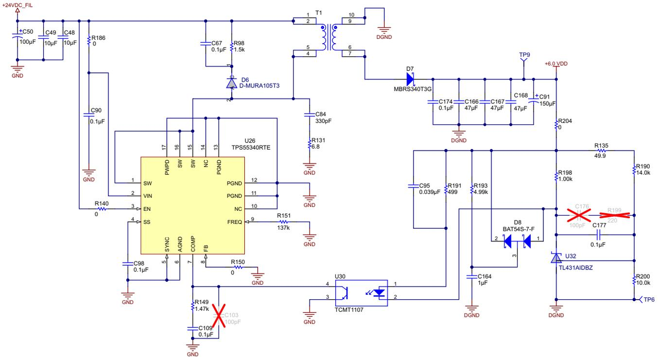
Figure 43. 24-V DC to 6-V DC Flyback Converter
