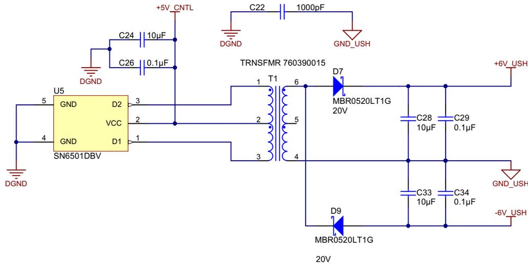
Figure 36. SN6501-Based Power Isolation
