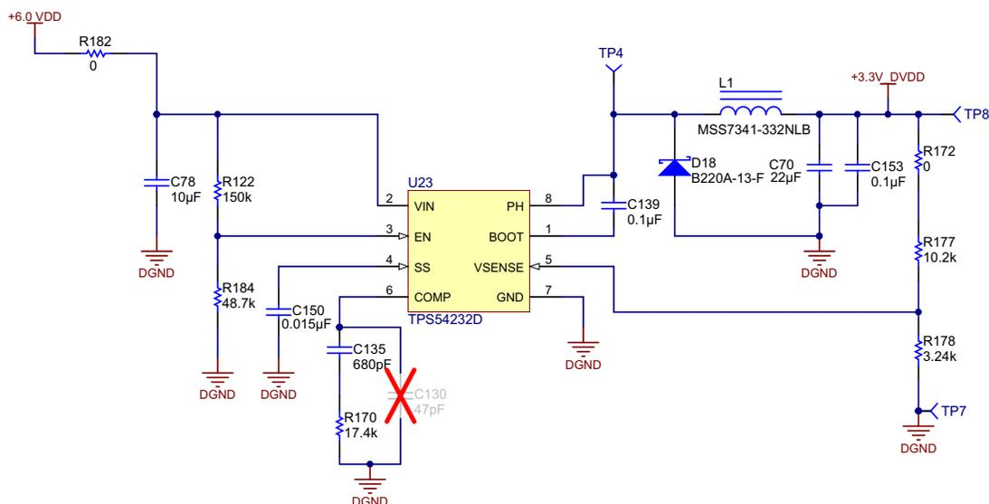
Figure 46. 6- to 3.3-V Step Down Converter
