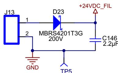
Figure 42. Input Polarity Protection
