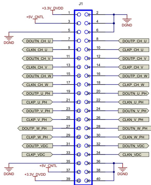
Figure 54. 2x20-Pin Connector to DSM Board
