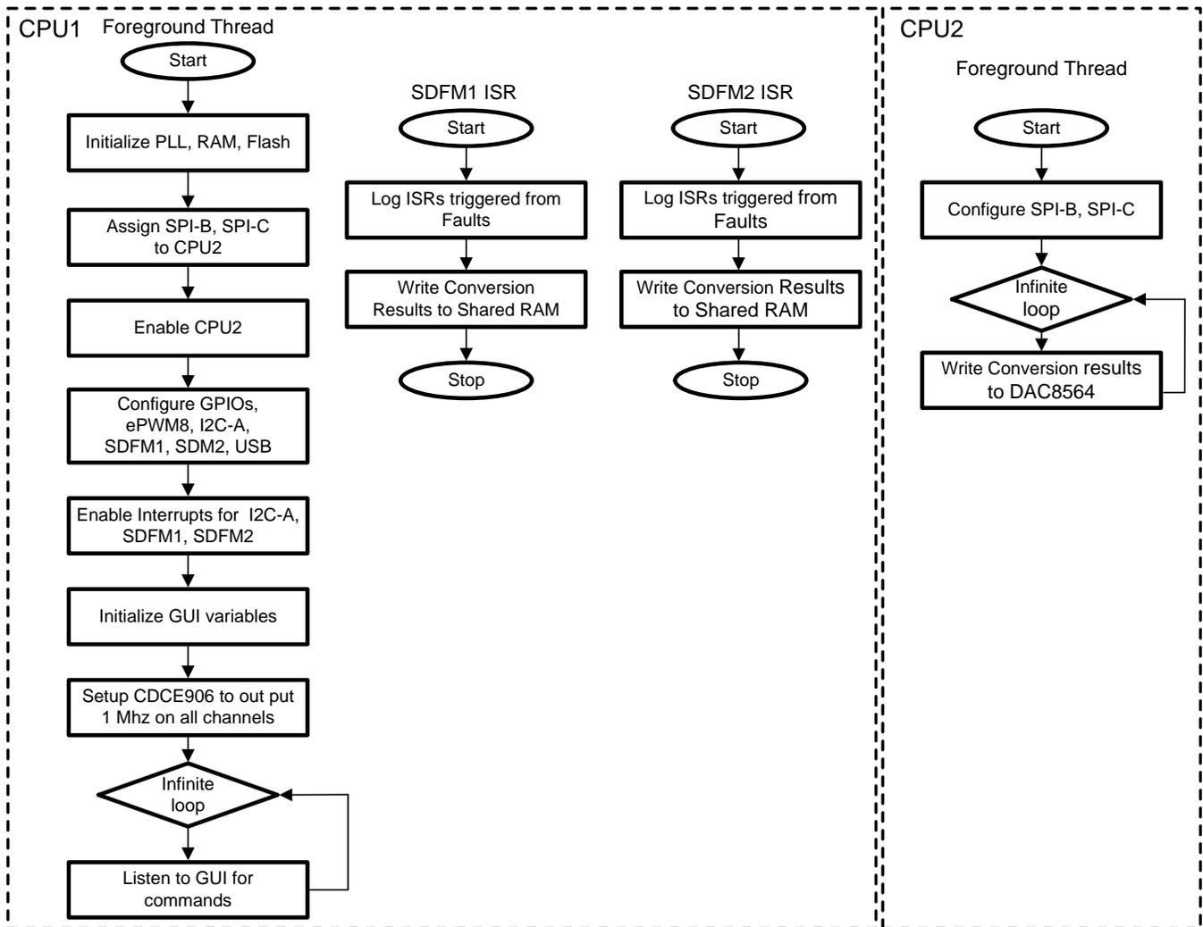
Figure 59. Firmware Flow Graph
