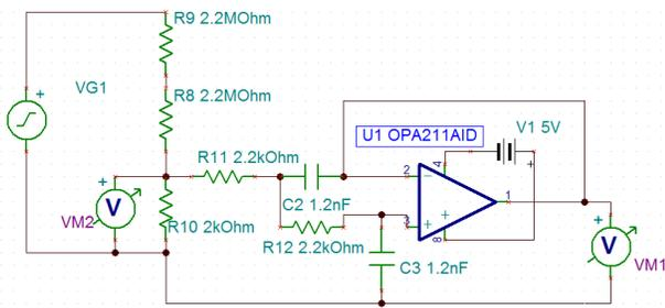
Figure 33. Phase-to-DC\_MINUS Sallen-Key Simulation
