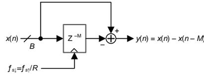
Figure 9. CIC Comb Filter Section
