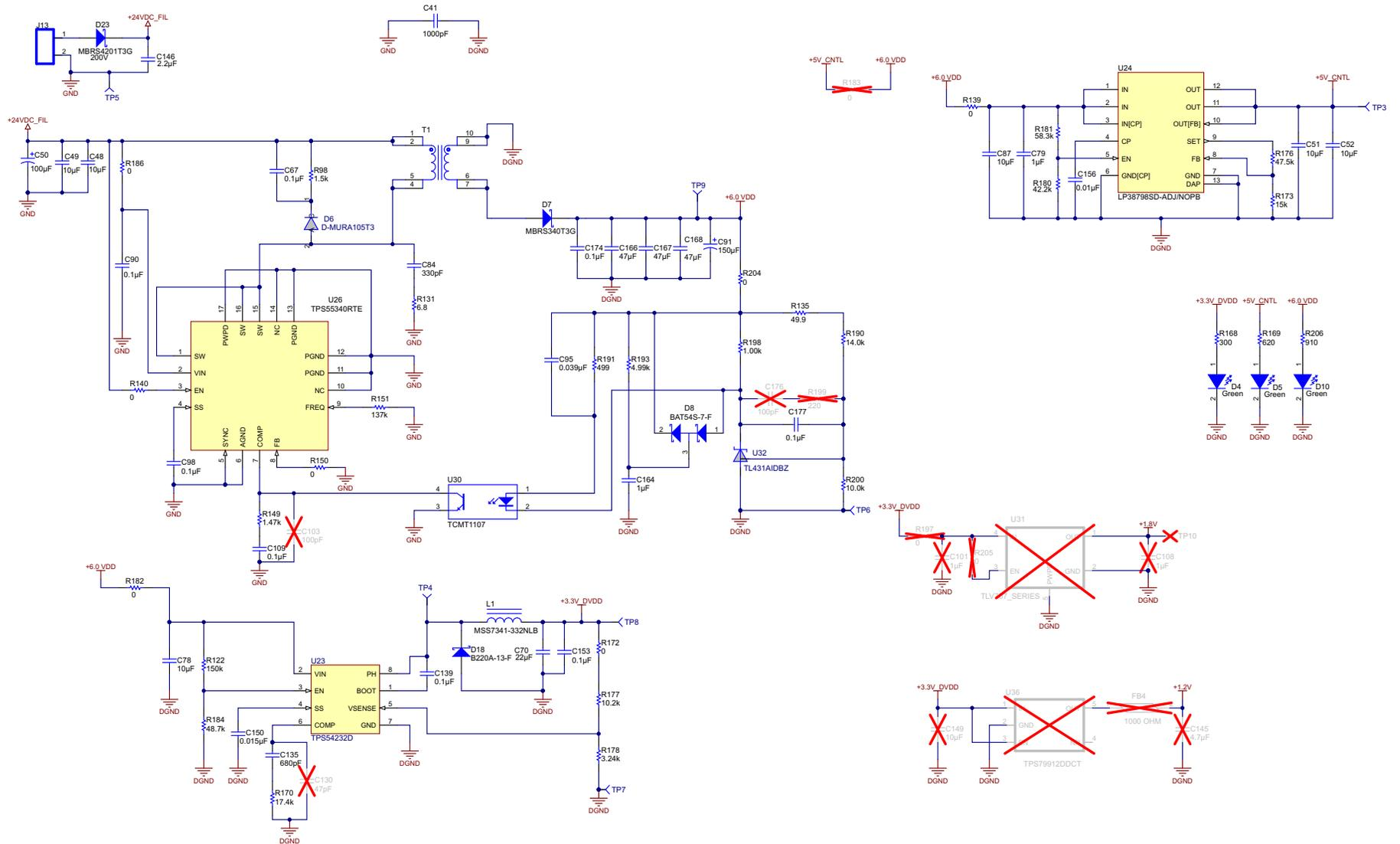
**Figure 139. Power Supply Schematic**
