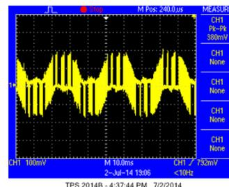
Figure 129. Ripple on -5.0V\_USH Power Rail on DSM Board, Measured Across Capacitor C51, with Motor Turned On
