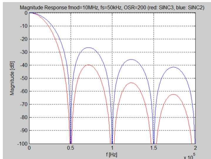
Figure 11. Magnitude versus Frequency Response of Sinc<sup>2</sup> Compared to Sinc<sup>3</sup> Filter
