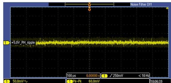
Figure 115. Ripple on 5.0V\_PH Power Rail on DSM Board, Measured Across Capacitor C103, with Motor Turned On
