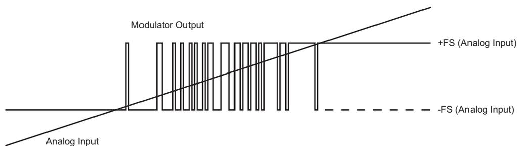
Figure 6. AMC130x Input Voltage versus Output
