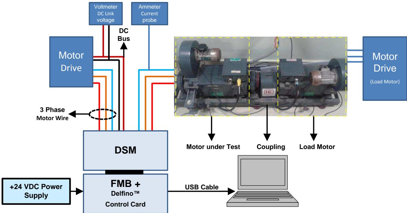
Figure 93. Test with Motor Drive and Load Setup
