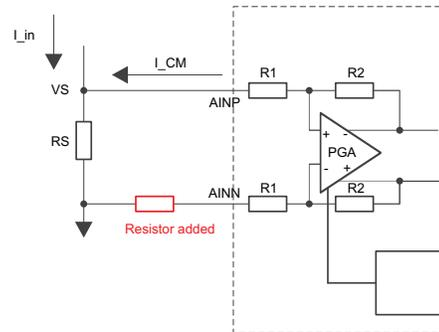
Figure 24. AMC1304 Input Offset Compensation Due to Bias Current
