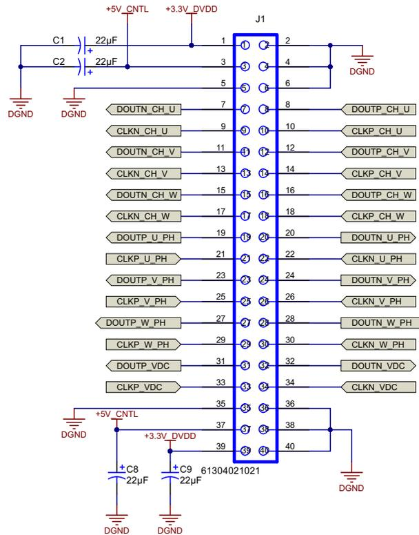
Figure 41. Board-to-Board Connector
