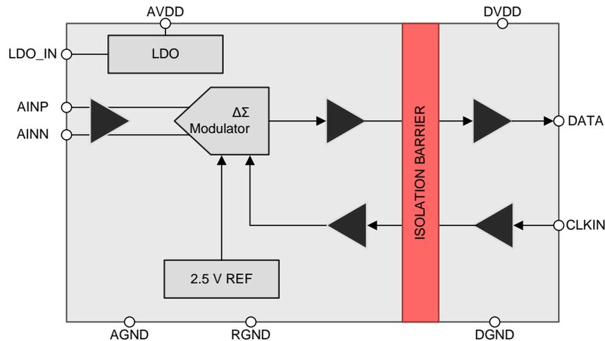
Figure 35. Block Diagram for AMC1304
