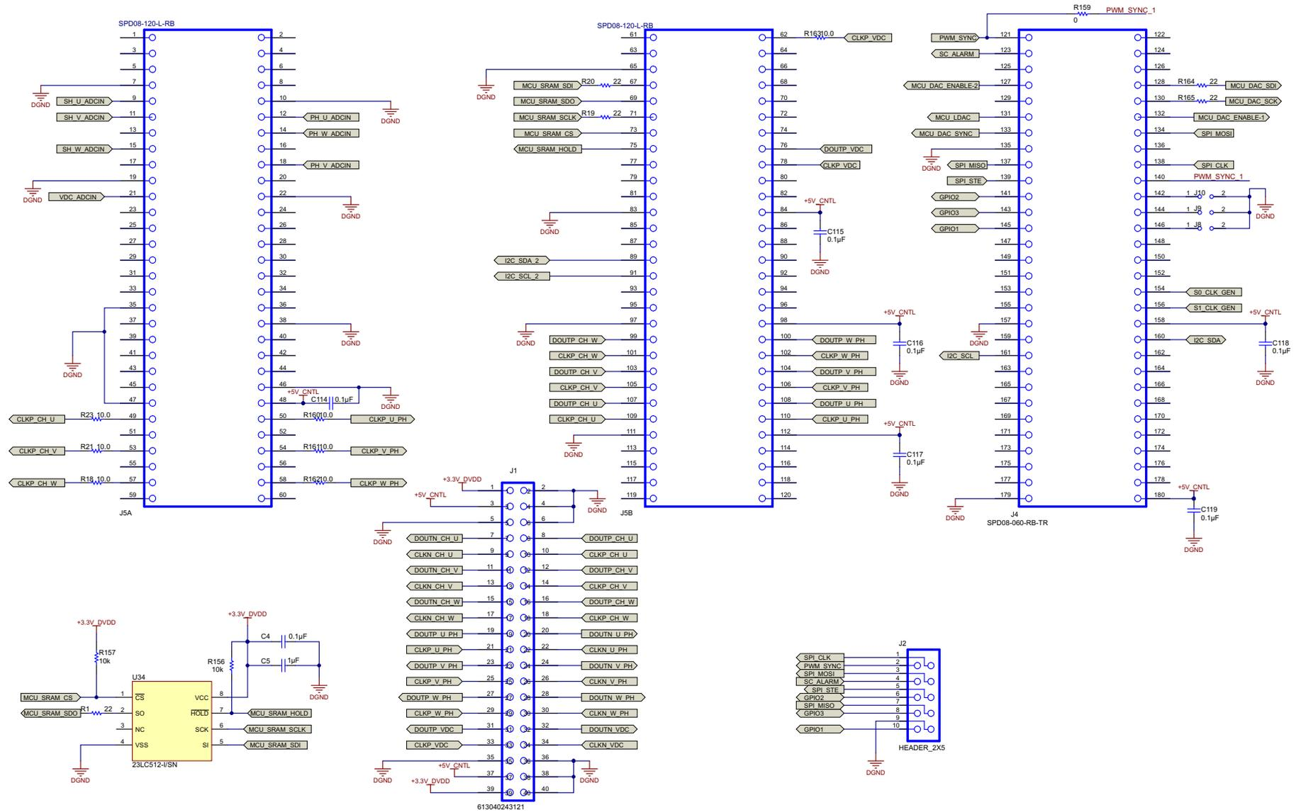
Figure 141. Control Card Connector
