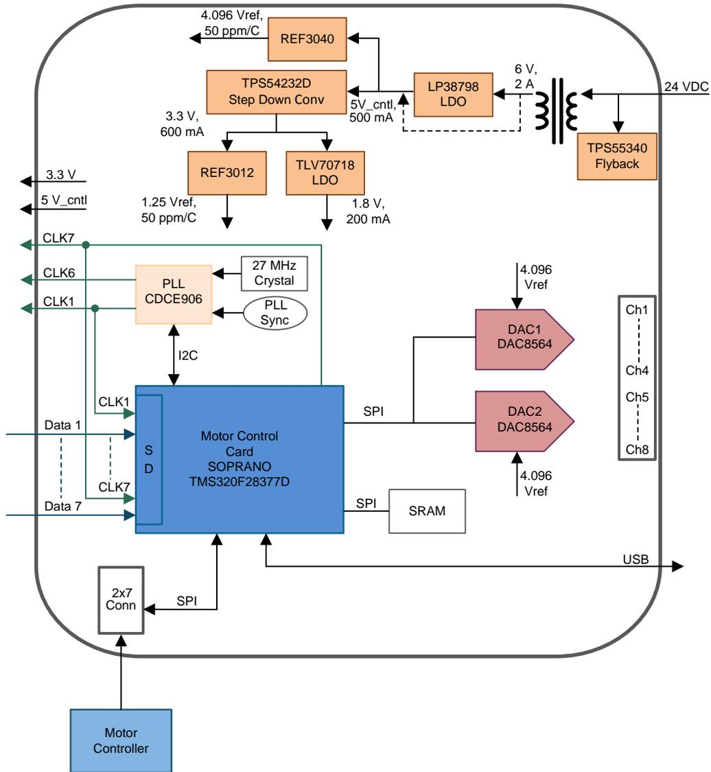
Figure 17. Block Diagram of FMB Subsystem
