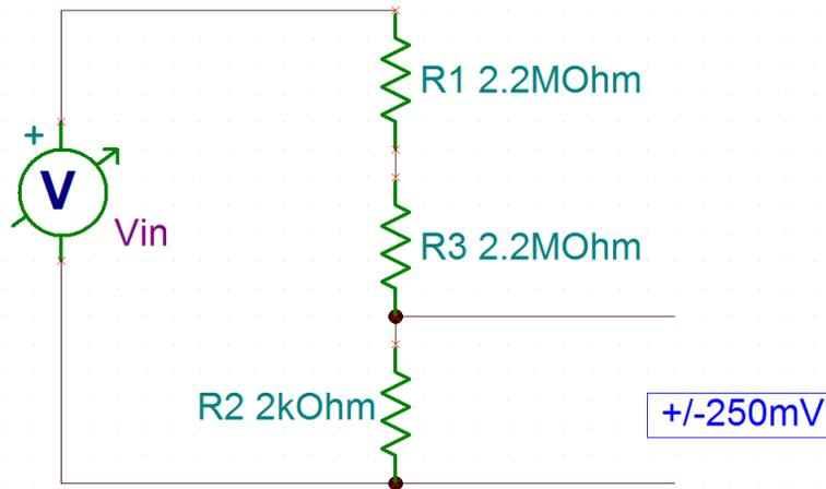
**Figure 32. Phase-to-DC\_MINUS Resistor Divider**
