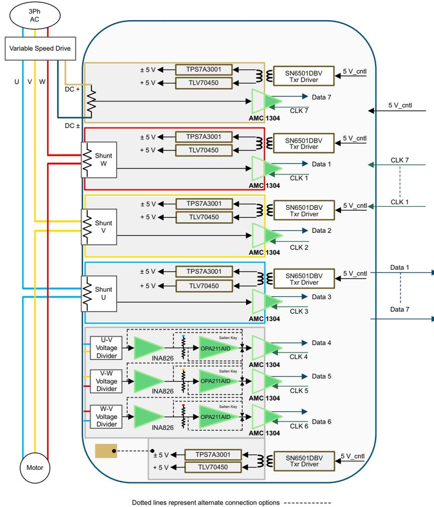
Figure 15. Block Diagram of DSM
