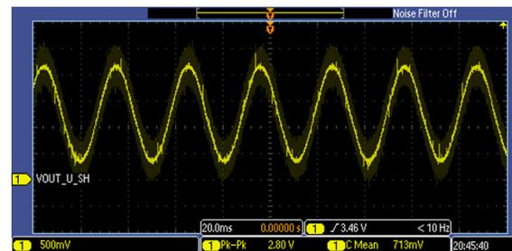
Figure 133. DAC Output, VOUT\_U\_SH, with Shunt Value of 50 mΩ
