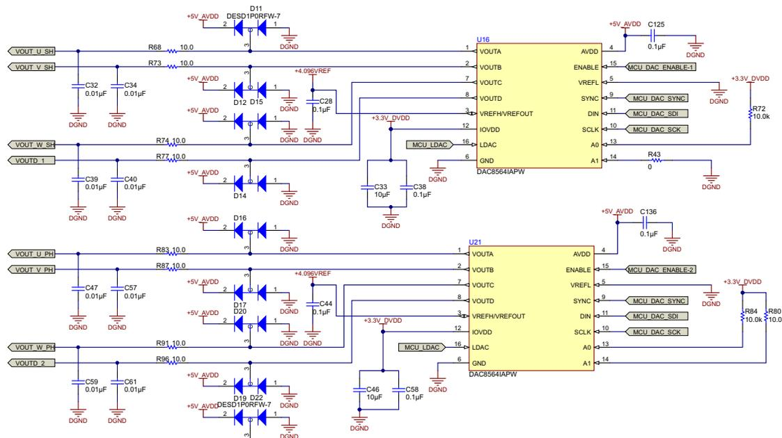
Figure 50. 16-Bit DAC Output
