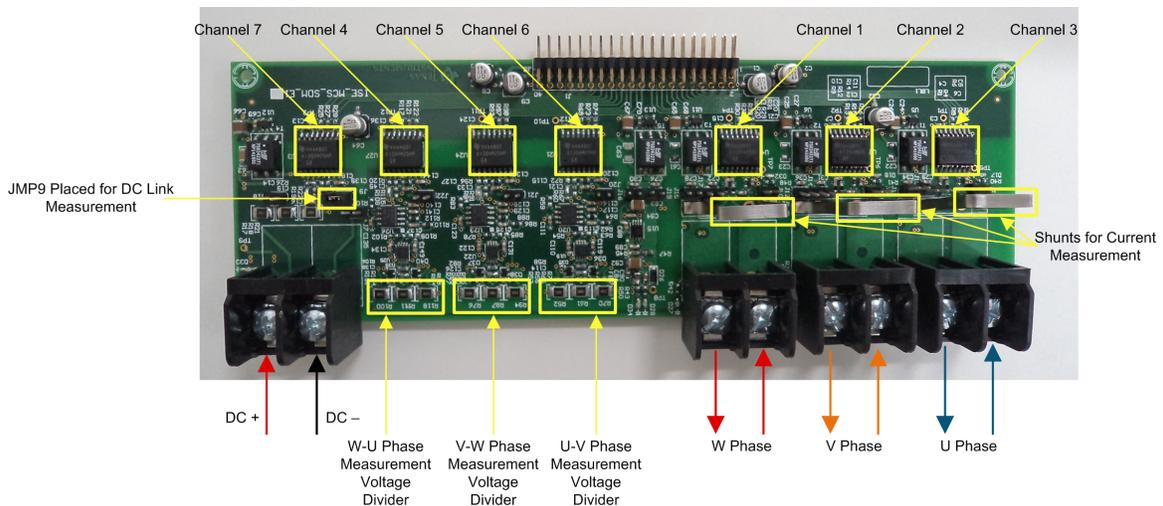
Figure 16. DSM Board
