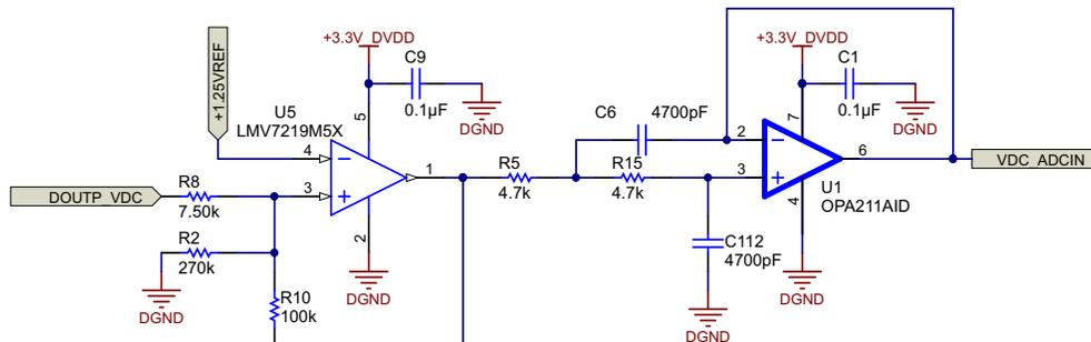
Figure 51. Amplifier and Sallen-Key Filter
