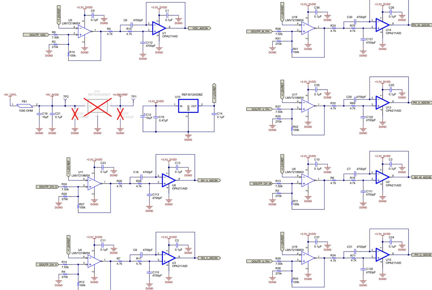
Figure 140. SDM OP Filtering Schematic
