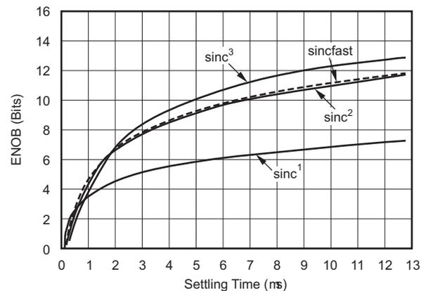
**Figure 13. Measured Effective Number of Bits versus Settling Time**
