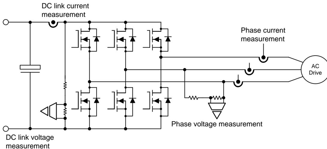
Figure 1. Current and Voltage Measurement in 3-Phase Inverters
