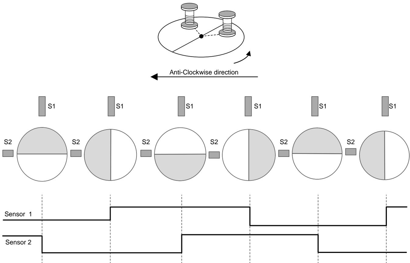
Figure 1. Logic Signal Compiled from LC Sensors
