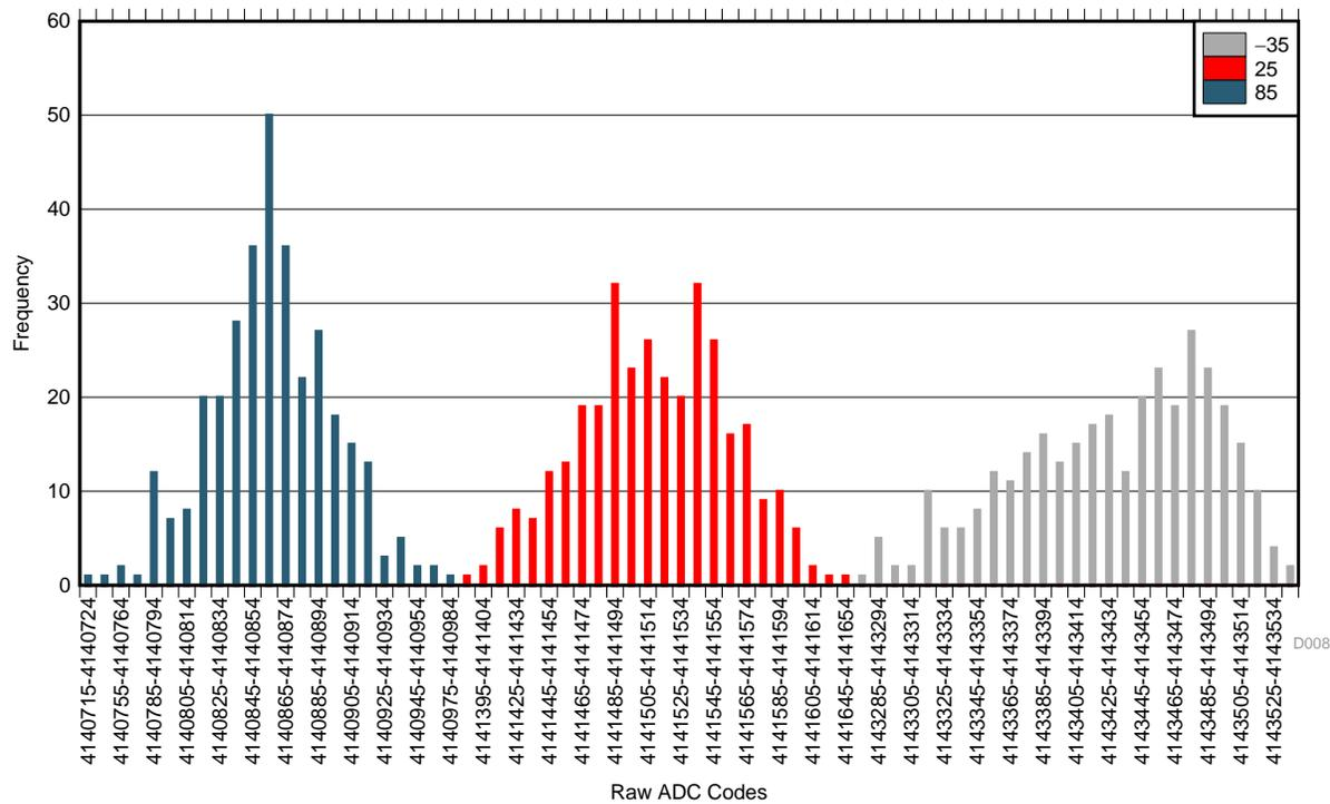
Figure 59. Noise Histogram of RTD Channel
