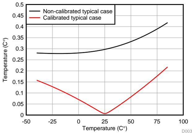
Figure 46. Typical Calibrated and Non-Calibrated Error of RTD
