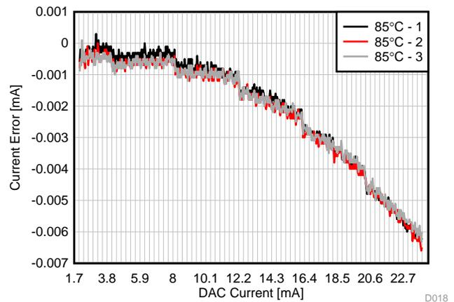
**Figure 69. Loop Current Error at 85°C (3 Sets of Measurements)**
