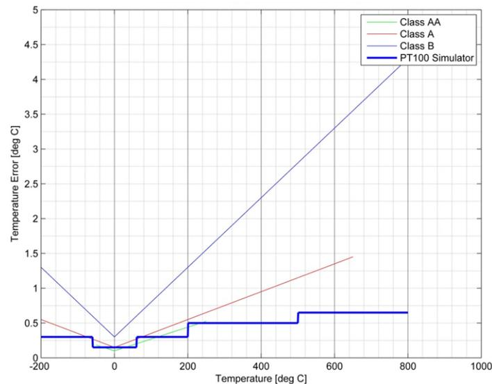
**Figure 58. Temperature Error vs Temperature of PT100 Sensors (Class AA, A, B) and PT100 Simulator**
