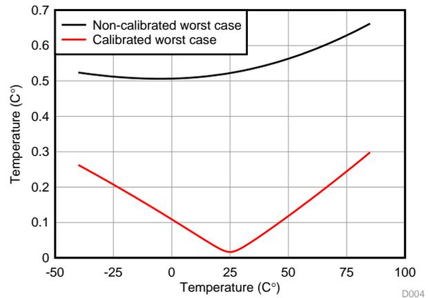
Figure 47. Worst Case Calibrated and Non-Calibrated Error
