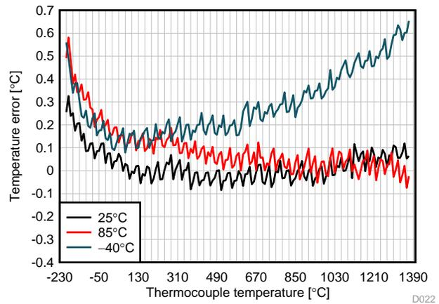
**Figure 73. System Temperature Error Over Ambient Temperature**
