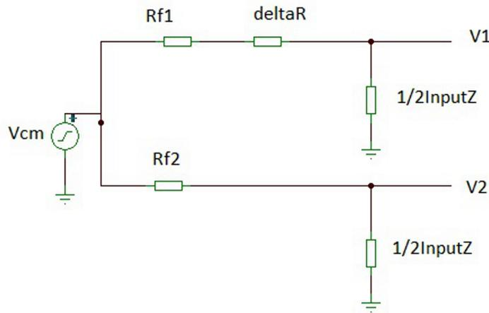
Figure 38. Simplified Circuit of  $R_{F1}$  Mismatched
