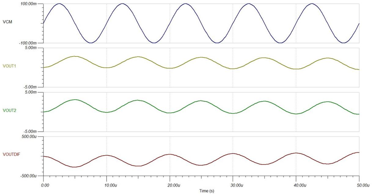
**Figure 30. Mismatched Common-Mode Capacitors**
