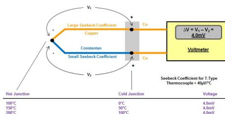
Figure 9. Simplified View of Cold Junction Compensation
