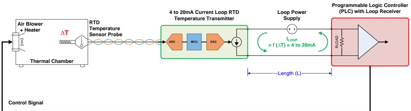
**Figure 18. Typical Block Diagram of a Current Loop System**
