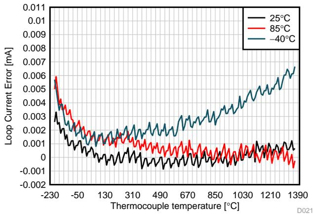
**Figure 72. System Loop Current Error Over Ambient Temperature**
