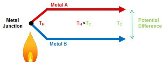
Figure 4. Thermocouple
