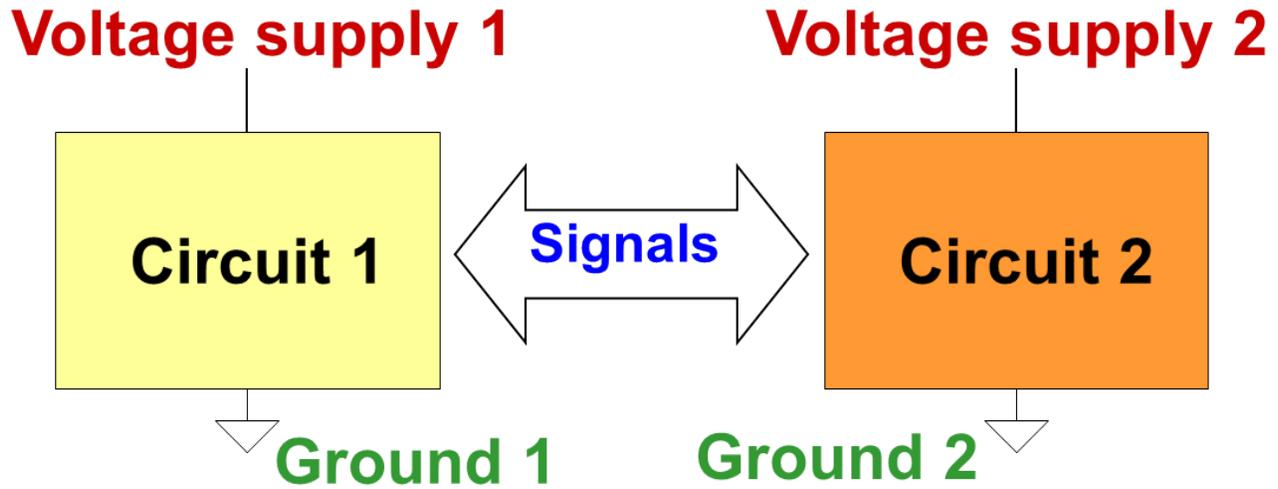
Figure 17. Definition of Galvanic Isolation
