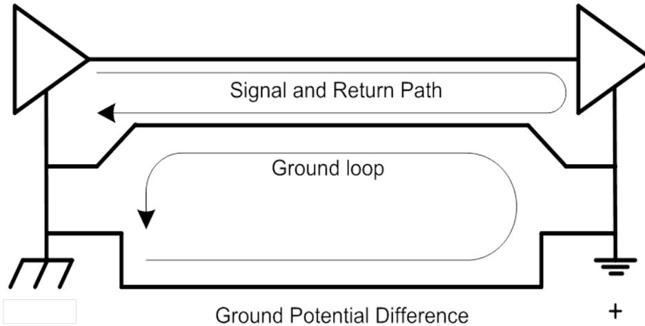
Figure 15. Ground Loops in Presence of Different Ground Potentials
