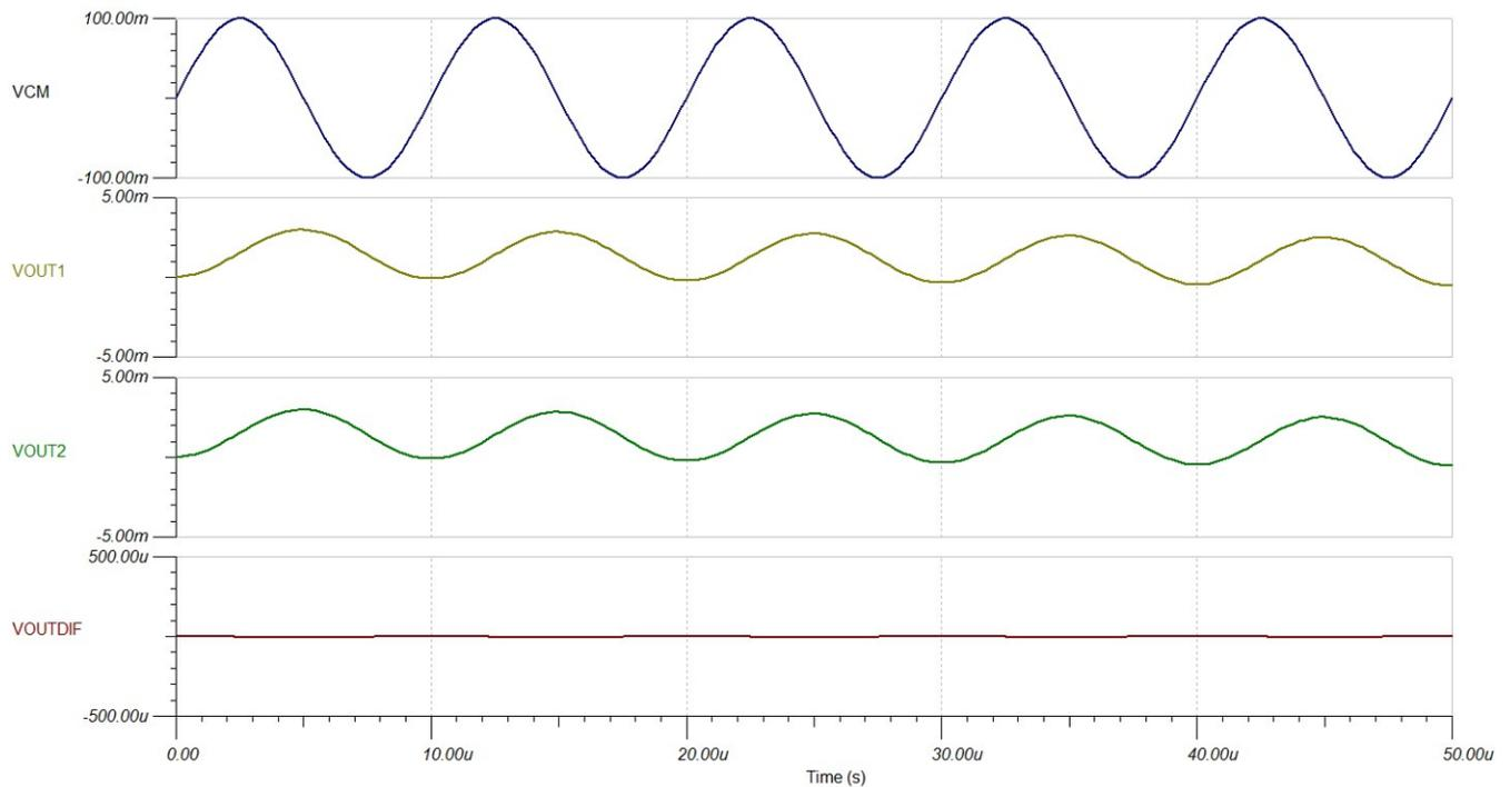
**Figure 32. Increase Differential Mode Filter Capacitor**
