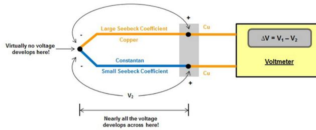
**Figure 5. Thermocouple and Developed Voltage**
