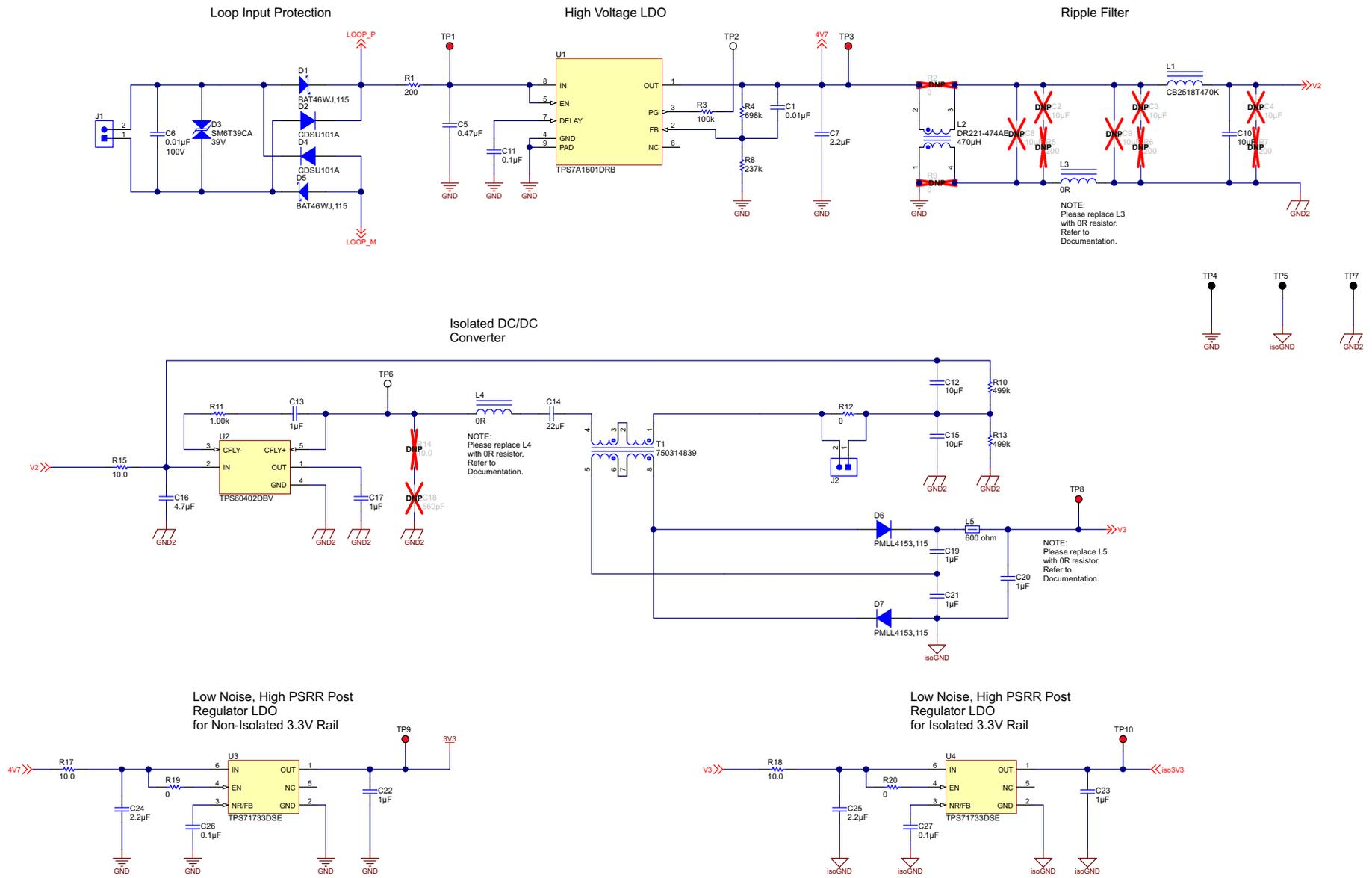
Figure 75. Schematic - Power Supply and Protection
