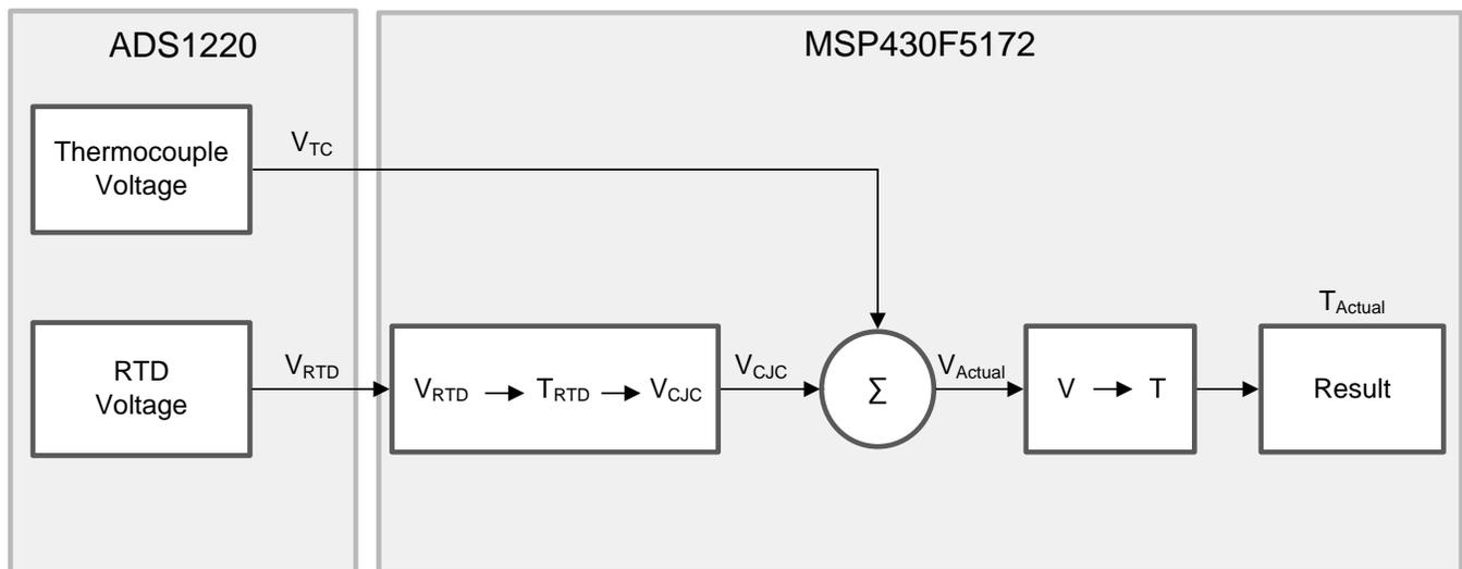
Figure 51. Software Flow Diagram for Thermocouple Linearization
