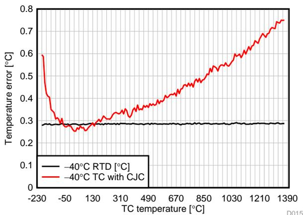
**Figure 66. Temperature Error with Cold Junction Compensation, Measured Cold Junction (Set to 0°C) at -40°C Ambient Temperature**
