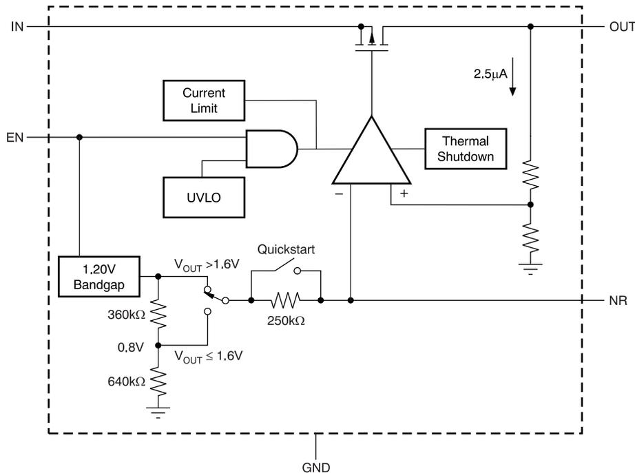
Figure 24. TPS71733 – Functional Block Diagram
