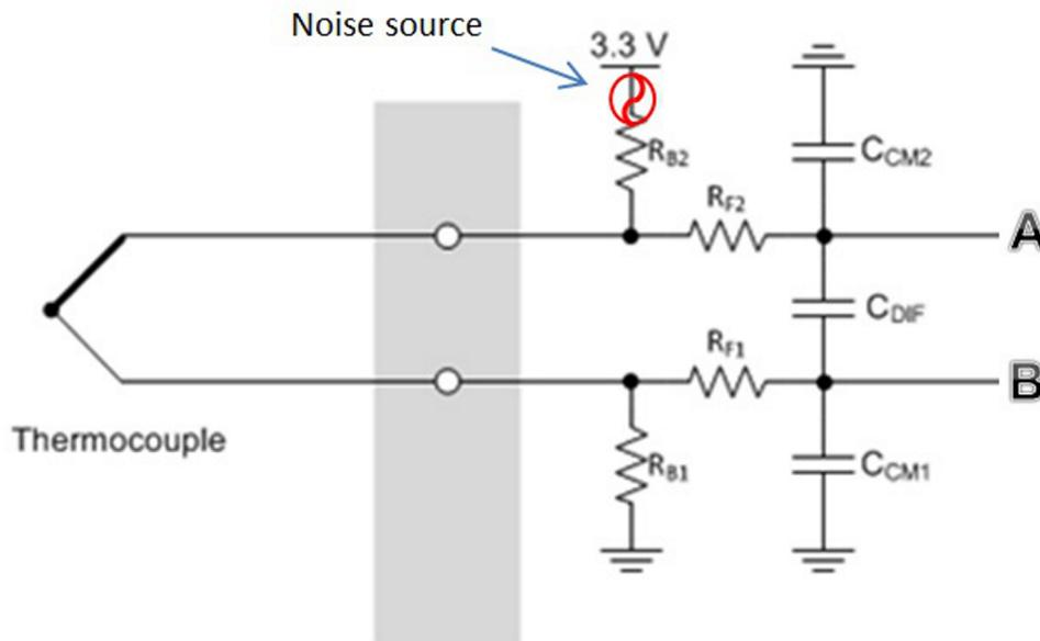
Figure 41. Biasing Resistors Noise Model
