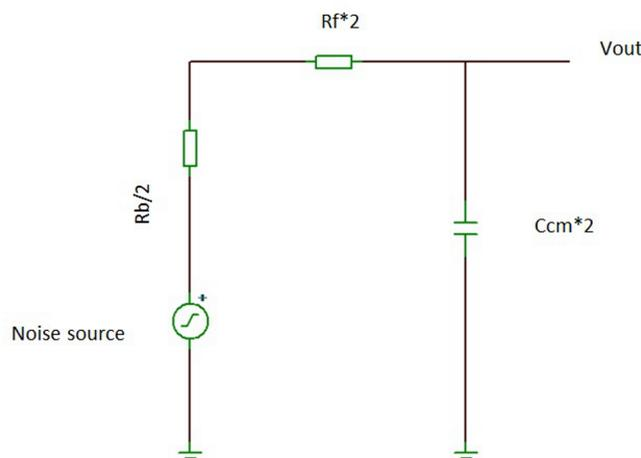
Figure 42. Simplified Circuit for  $R_{Bias}$  Noise
