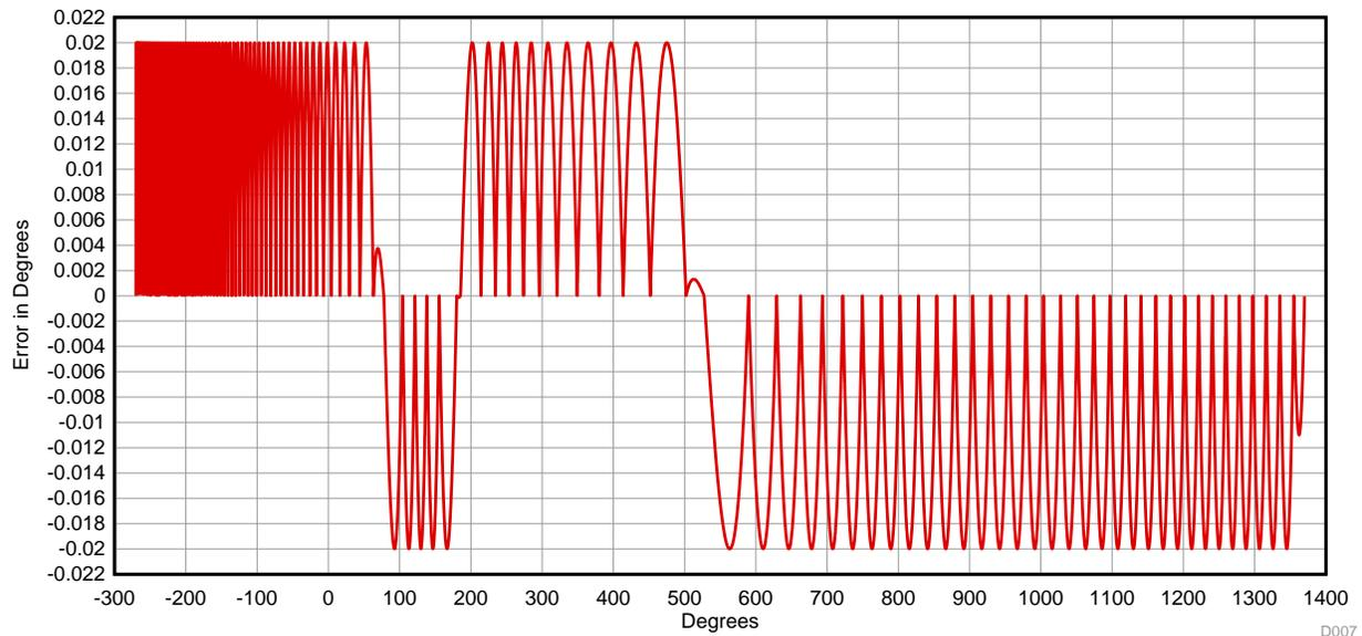
**Figure 50. Examples of the Error Intruded by the Software by Using Different Look Up Tables**
