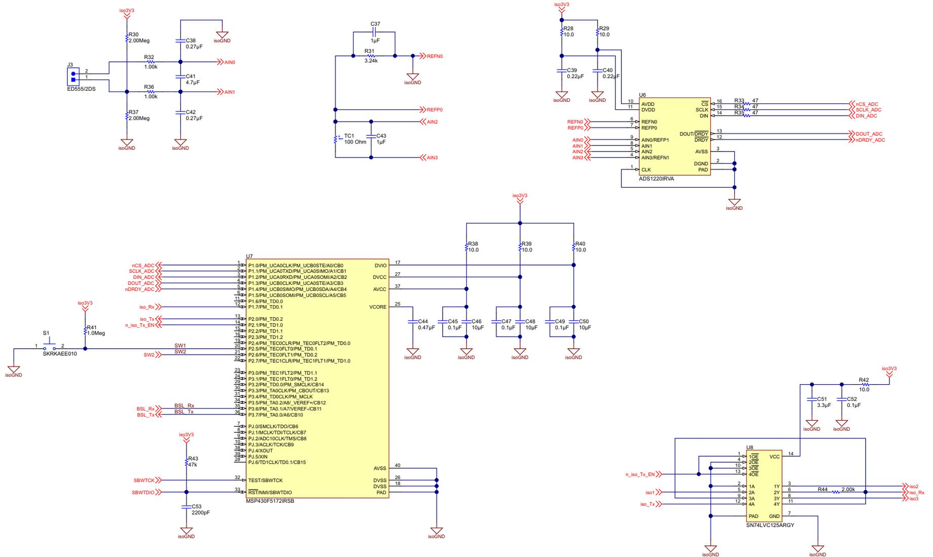
Figure 77. Schematic - Analog Front-End, MCU, and Isolated Data
