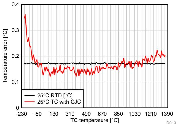
**Figure 64. Temperature Error with Cold Junction Compensation, Measured Cold Junction (Set to 0°C) at 25°C Ambient Temperature**
