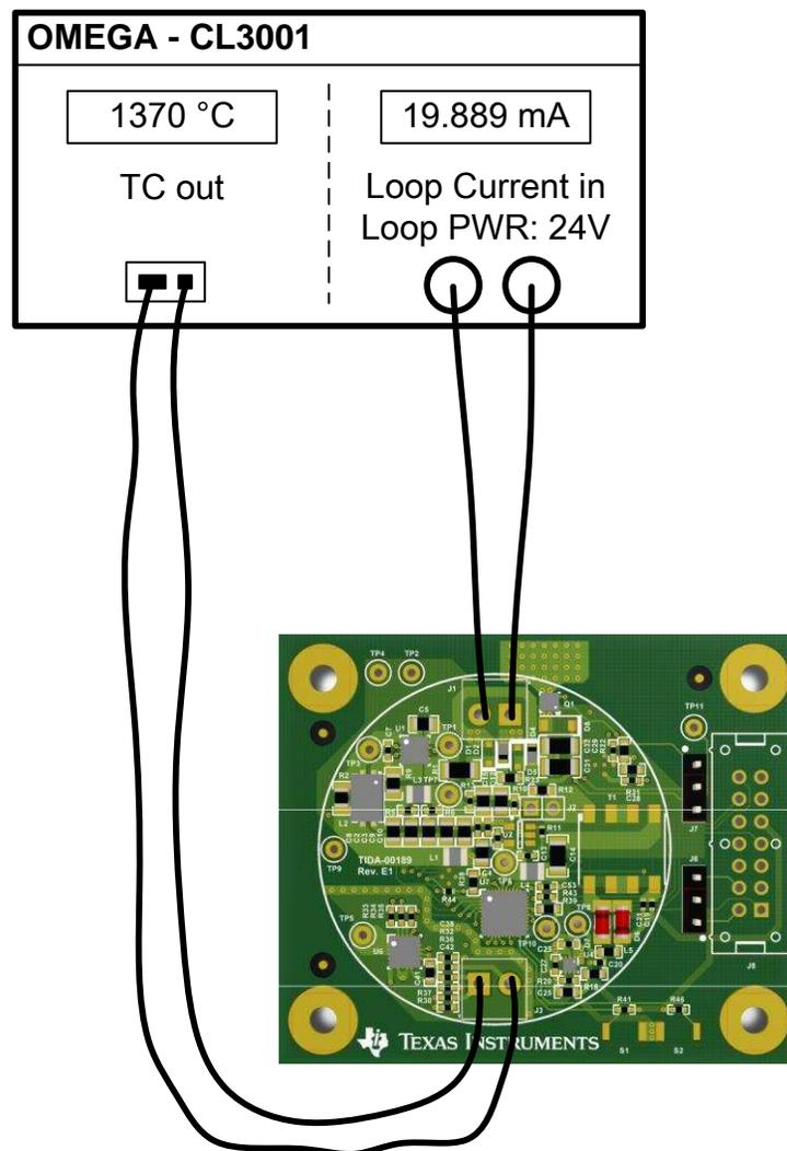
**Figure 56. Basic Test Setup**
