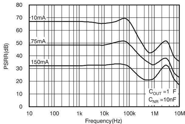
Figure 23. TPS71733 – PSRR vs. Frequency @ VIN – VOUT = 0.25V
