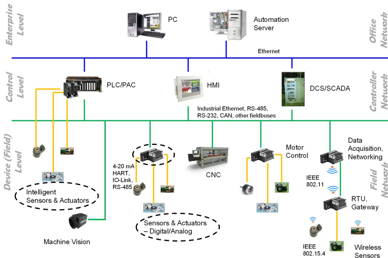
**Figure 1. Factory Automation and Process Control Ecosystem**
