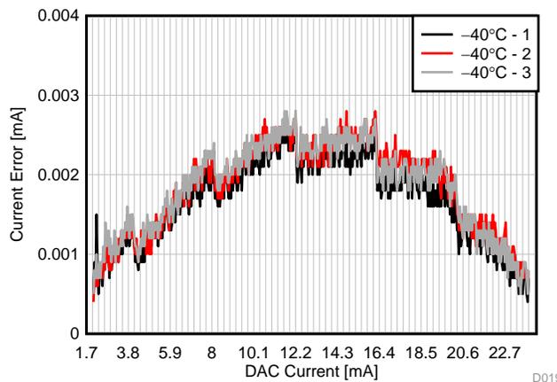
**Figure 70. Loop Current Error at -40°C (3 Sets of Measurements)**
