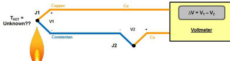
Figure 10. Unwanted Thermocouple Junction
