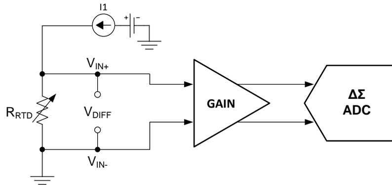
**Figure 12. Simplified RTD Application Circuit**
