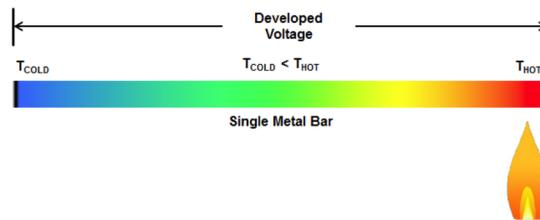
Figure 3. Voltage Developed Due to Temperature Gradient
