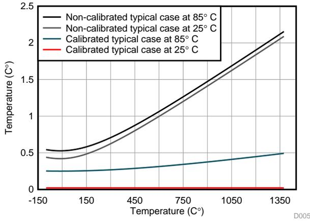
**Figure 48. Typical Calibrated and Non-Calibrated Total Front End Error (at 25°C and 85°C)**
