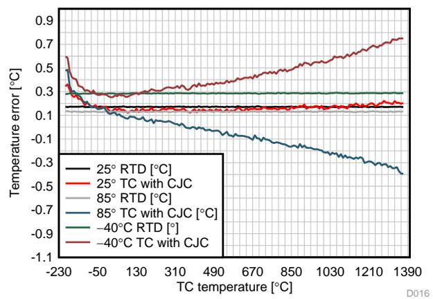
**Figure 67. Temperature Error with Cold Junction Compensation, Measured Cold Junction (Set to 0°C) Across Ambient Temperature**
