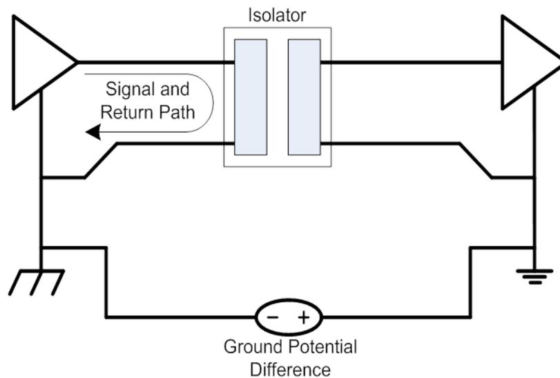
Figure 16. Galvanic Isolation Breaks Ground Loops
