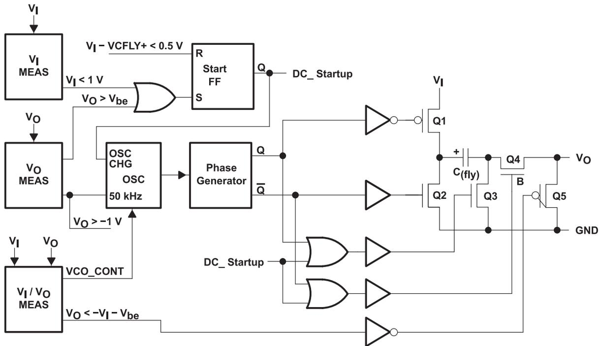
Figure 25. TPS60400 Family - Functional Block Diagram
