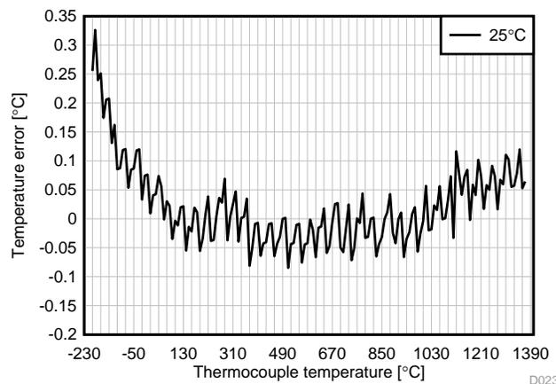
**Figure 74. System Temperature Error at 25°C**
