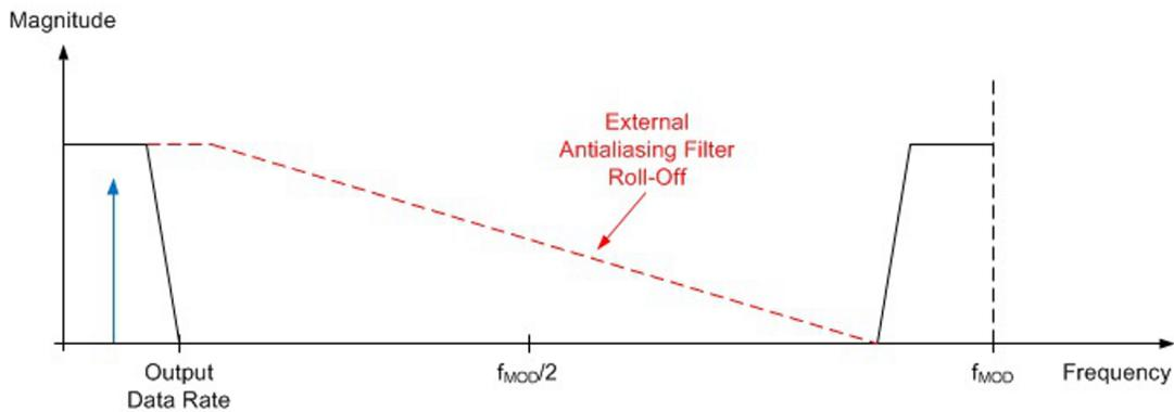
**Figure 35. Antialiasing Filter**
