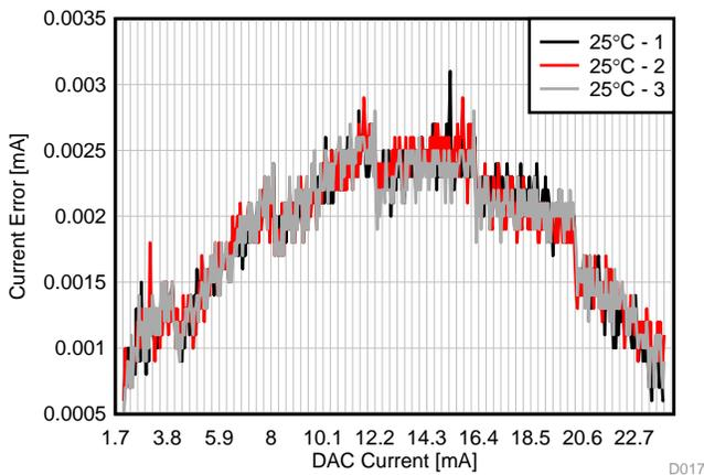
**Figure 68. Loop Current Error at 25°C (3 Sets of Measurements)**
