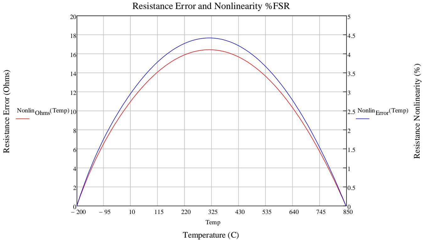
Figure 14. PT100 RTD Non-Linearity from -200°C to 850°C
