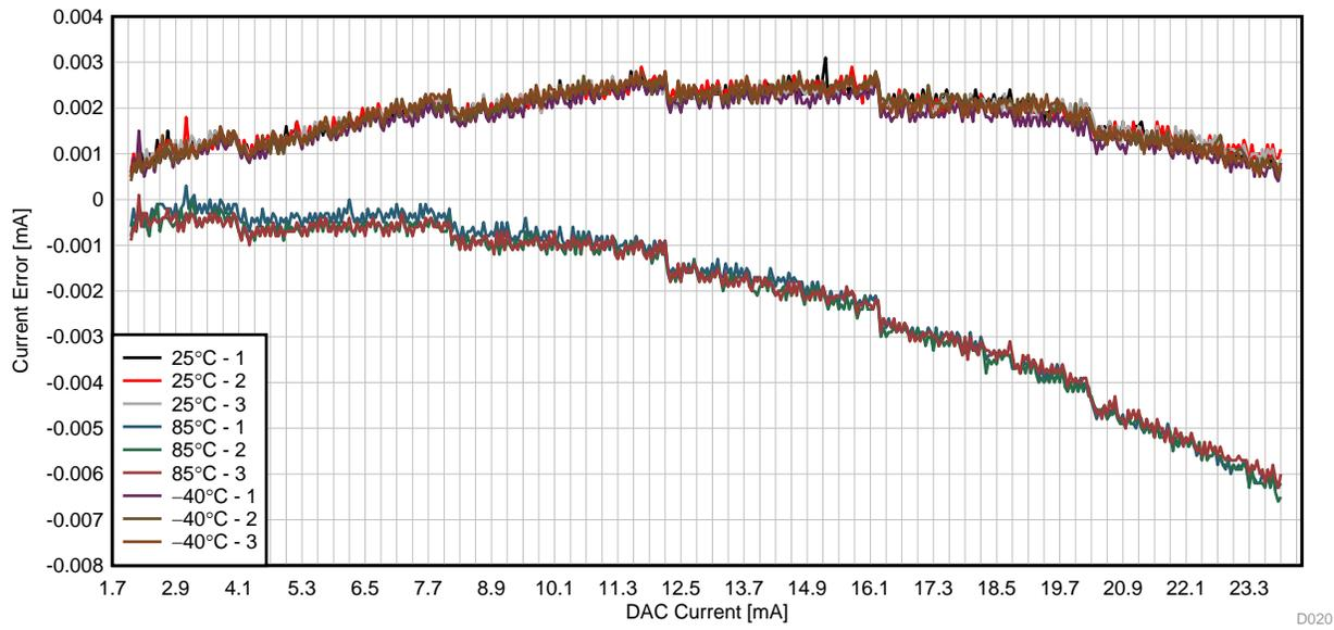
Figure 71. Loop Current Error Over Ambient Temperature
