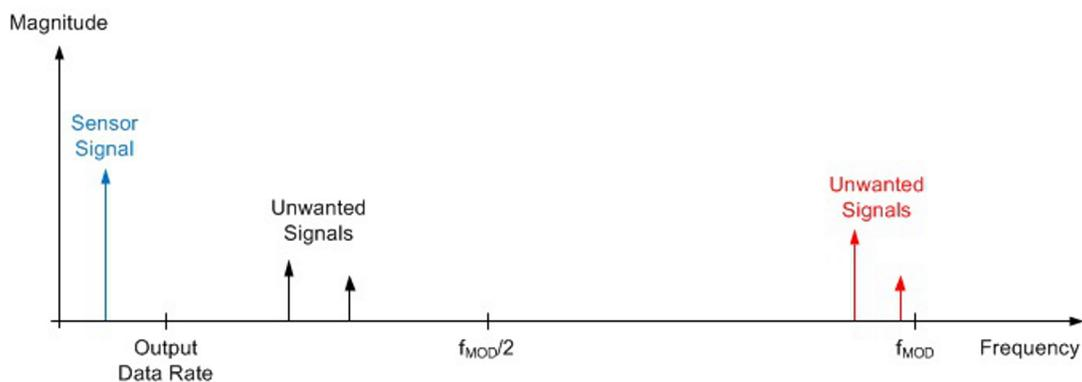
Figure 33. Unwanted Signal in the Frequency Domain
