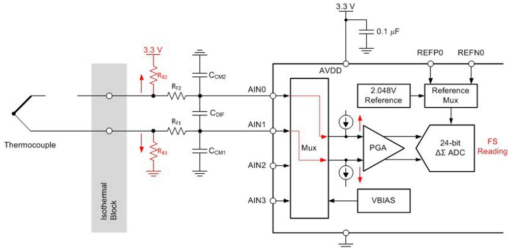
Figure 39. Biasing Resistors RB1 and RB2
