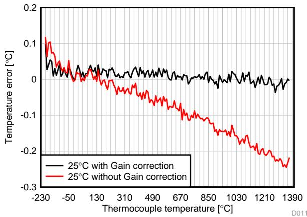
**Figure 62. Temperature Error With and Without Gain Correction at 25°C**
