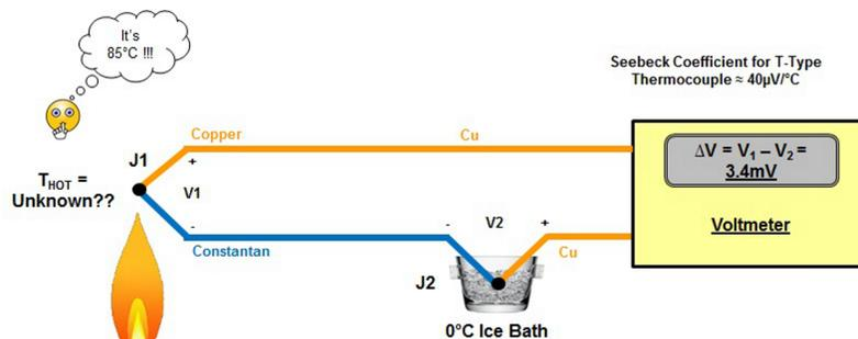
Figure 11. Measuring Absolute Temperature Using 0°C Ice Bath
