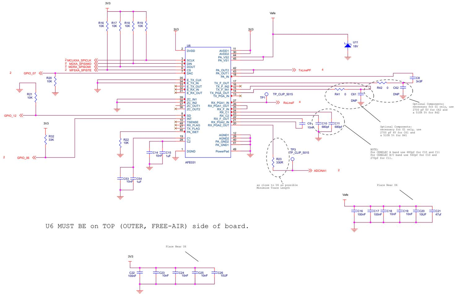
U6 MUST BE on TOP (OUTER, FREE-AIR) side of board.
