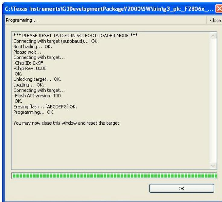
**Figure 7. Flashing G3-PLC Firmware (via SCI)**
