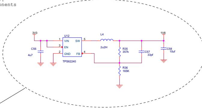
OPTIONAL: For reduced power consumption use a DC/DC converter instead of the On-Chip Linear Supply
