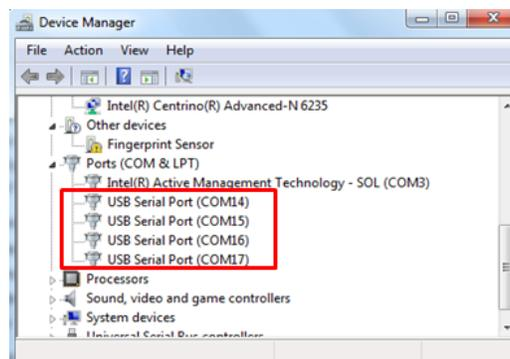
**Figure 12. Device Manager: Port Configuration**
