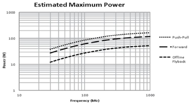
Figure 7. Power Level versus Operating Frequency for Selected Core
