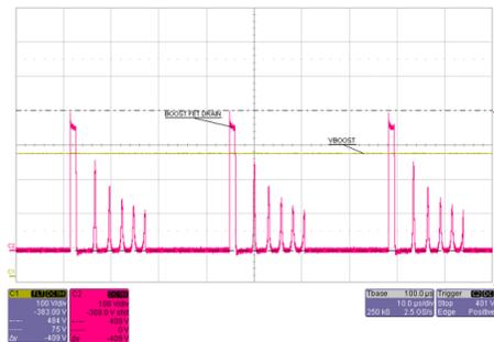
Figure 18. Booster Output  $V_{BOOST}$  and Booster FET Drain Voltage at 24-V DC Input
