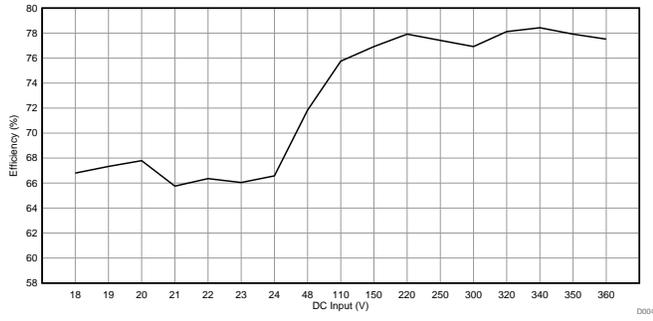
**Figure 13. Efficiency vs DC Input Voltage**
