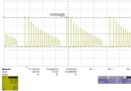
Figure 22. Booster Diode PIV at 88-V AC
