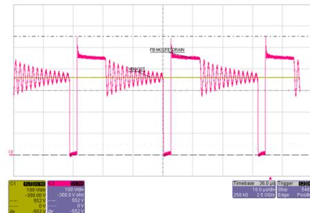
Figure 25. Booster Output  $V_{BOOST}$  and Flyback MOSFET Drain at 360-V DC
