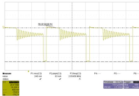
Figure 31. Flyback Secondary Diode PIV at 270-V AC
