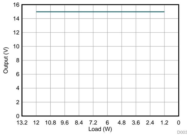
**Figure 15. Load Regulation — 24-V DC Input**
