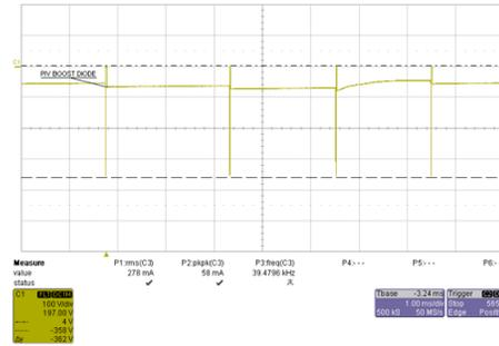
Figure 23. Booster Diode PIV at 220-V AC
