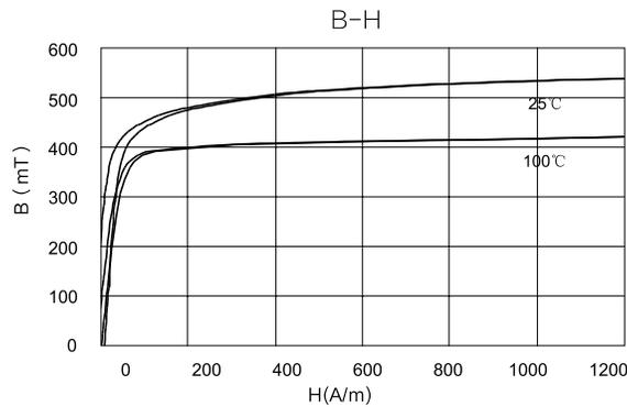
**Figure 8. B-H Curve for Selected Core**
