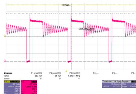
Figure 27. Booster Output  $V_{BOOST}$  and Flyback MOSFET Drain at 270-V AC
