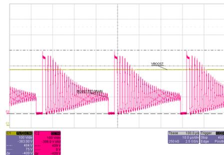
Figure 19. Booster Output  $V_{BOOST}$  and Booster FET Drain Voltage at 110-V DC Input
