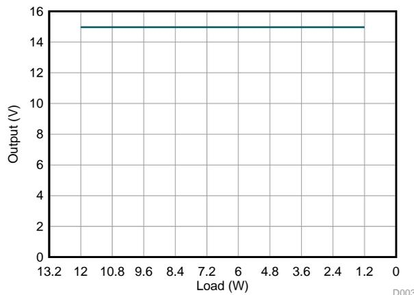
**Figure 12. Load Regulation — 230-V AC Input**
