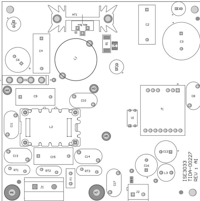
Figure 46. Top Assembly Drawing
