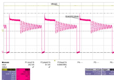
Figure 26. Booster Output  $V_{BOOST}$  and Flyback MOSFET Drain at 80-V AC
