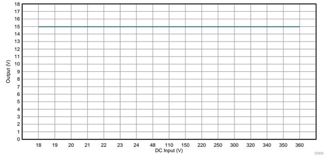
**Figure 14. Line Regulation at DC Input Voltage**
