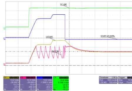
Figure 17. Start Up at 24-V DC, No Load
