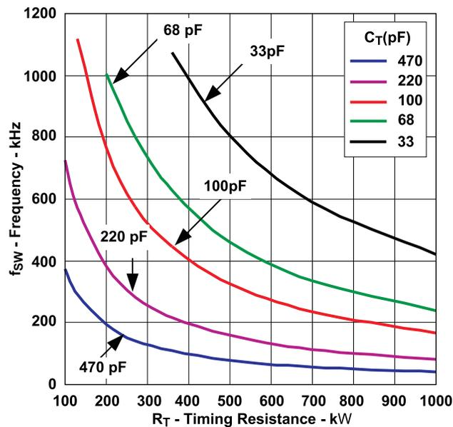
Figure 3. Frequency versus Timing Resistance for TPS40210
