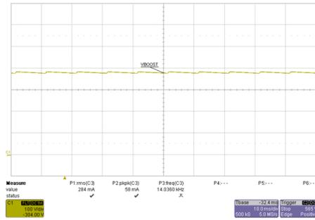
Figure 29. : Booster Output  $V_{BOOST}$  at 270-V AC
