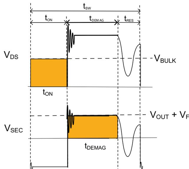
Figure 6. Volt Seconds During the On-Time Must Equal the Volt Seconds During the Demagnetizing Time for Energy Balance
