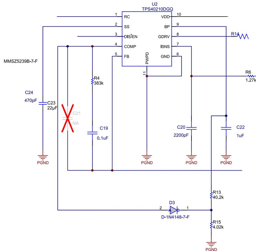
**Figure 4. Duty Cycle Limiting Circuit**
