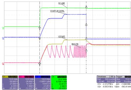
Figure 16. Start Up at 24-V DC, Full Load
