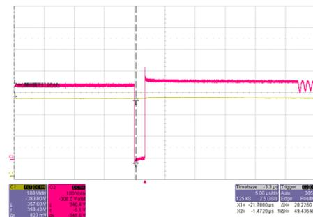
Figure 21. Booster Output  $V_{BOOST}$  and Booster FET Drain Voltage at 340-V DC Input
