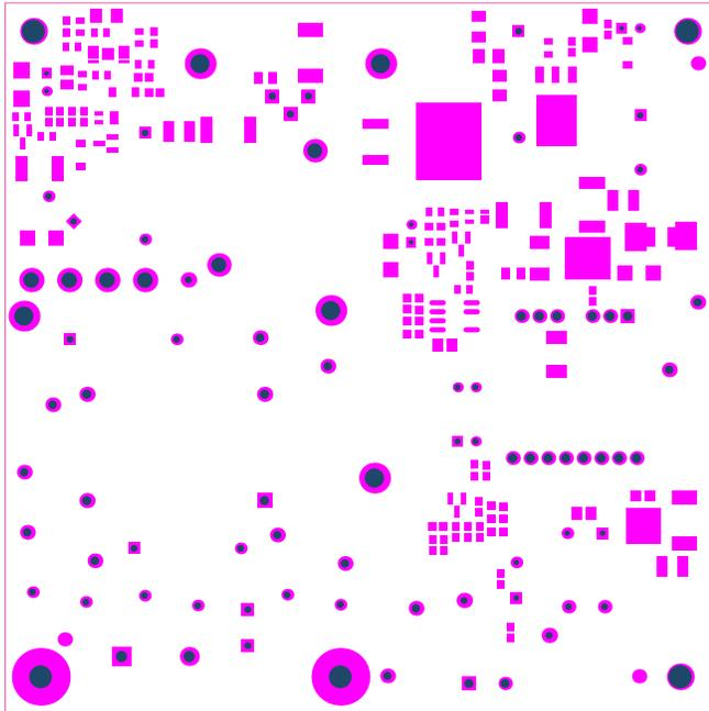
Figure 42. Bottom Solder Mask
