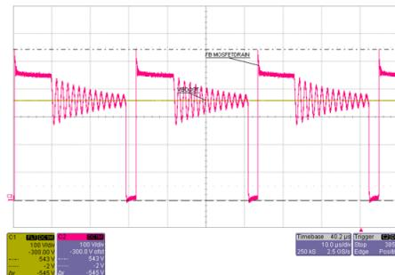
Figure 24. Booster Output  $V_{BOOST}$  and Flyback MOSFET Drain at 24-V DC
