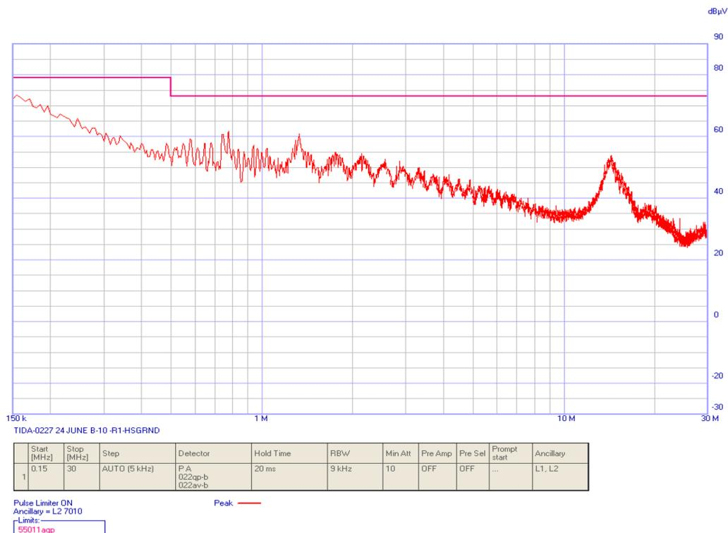
**Figure 35. Test Result with Peak-Mode Measurement — Tested at 230-V AC**
