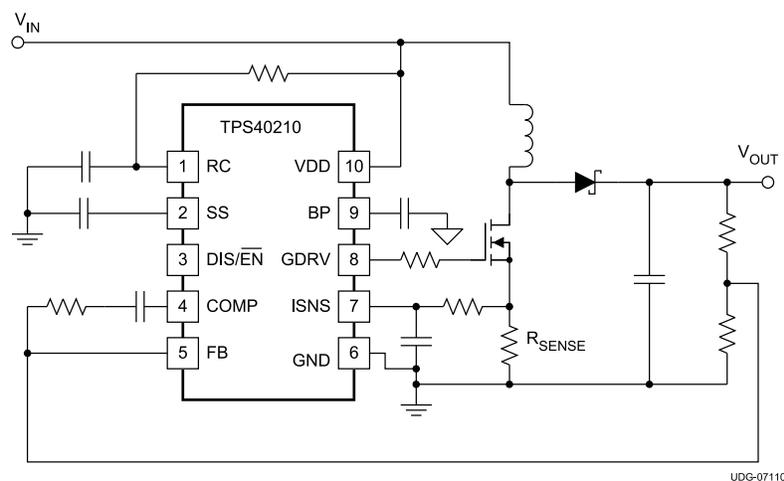
**Figure 2. DC-DC Booster Design Using the TPS40210DGQ**
