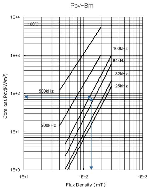
**Figure 9. 4 Core Loss vs Flux Density for Selected Core at Different Operating Frequency**
