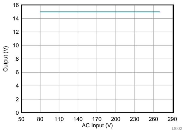
**Figure 10. Output Voltage vs AC Input Voltage**
