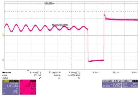
Figure 28. : Booster Output  $V_{BOOST}$  and Flyback MOSFET Drain at 270-V AC
