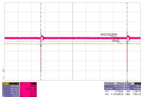
Figure 20. Booster Output  $V_{BOOST}$  and Booster FET Drain Voltage at 340-V DC Input
