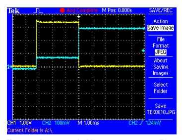
Figure 32. Response of GPIO-00 to Over-current Event
