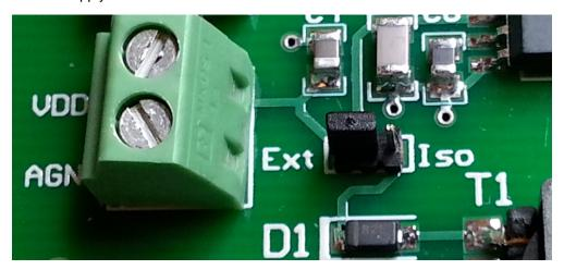
Figure 49. Jumper Setting for External Supply to AMC1304M25
