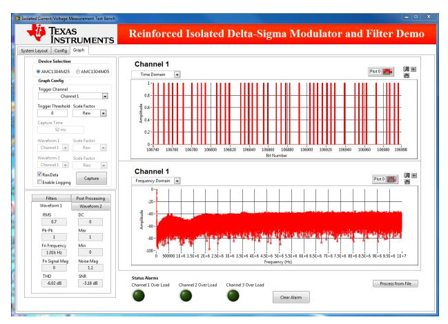
Figure 48. GUI - AMC1304M25 Raw Bit-stream Display
