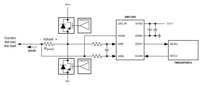
Figure 3. Typical Shunt Location
