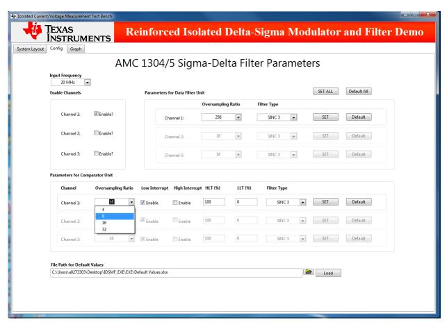
Figure 39. GUI - OSR Selection for Comparator Unit - Config Tab
