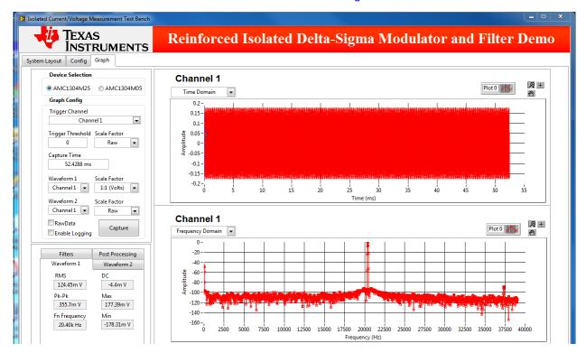
Figure 30. Measured Bandwidth
