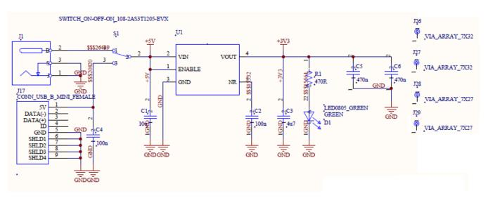
Figure 53. Schematic for Docking Station - Part 2
