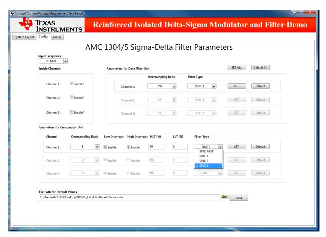
Figure 41. GUI - Comparator Unit Filter Selection - Config Tab
