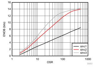
Figure 15. Measured Effective Number of Bits versus Oversampling Ratio
