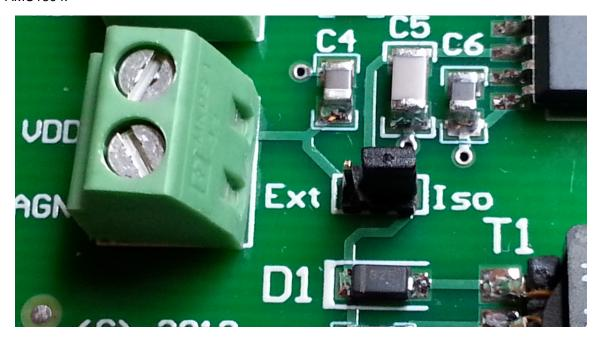
Figure 23. High Side of AMC1304 Supplied from T1
