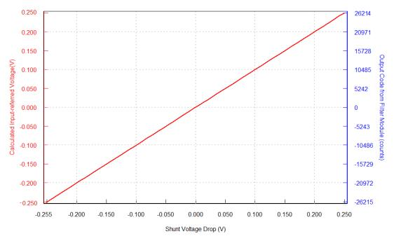
Figure 27. Transfer Function of the System
