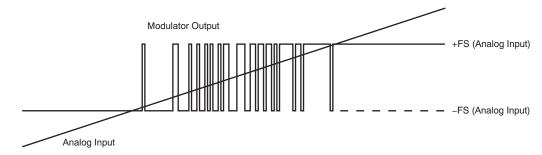
Figure 14. Analog Input versus AMC1304 Modulator Output
