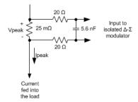
Figure 13. RC Passive Filter Selected
