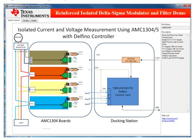
Figure 35. GUI - System Layout Tab
