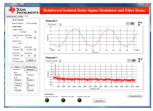
Figure 1. System Output for a Full Scale, 1kHz Input signal
