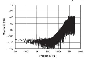
Figure 6. Quantization Noise Shaping
