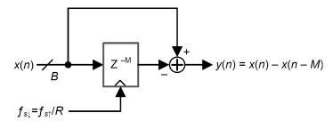
Figure 9. CIC Comb Filter Section
