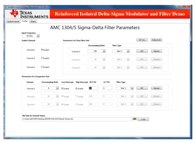
Figure 40. GUI - Comparator Unit - High Level Threshold Setting
