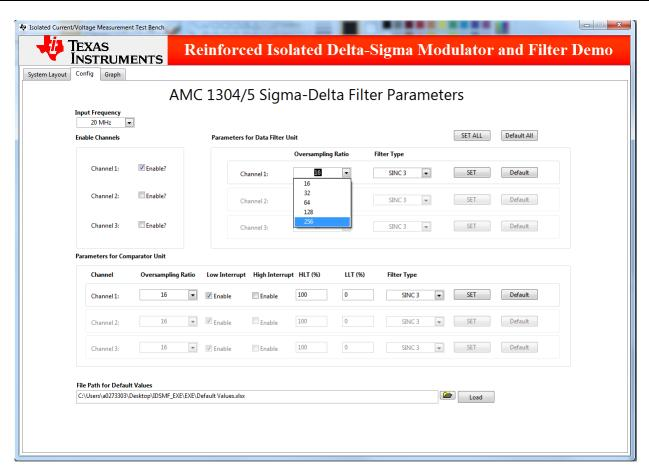
Figure 37. GUI - OSR Selection for Data Filter Unit - Config Tab
