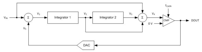
Figure 5. Block Diagram of a Second-Order ΔΣ Modulator
