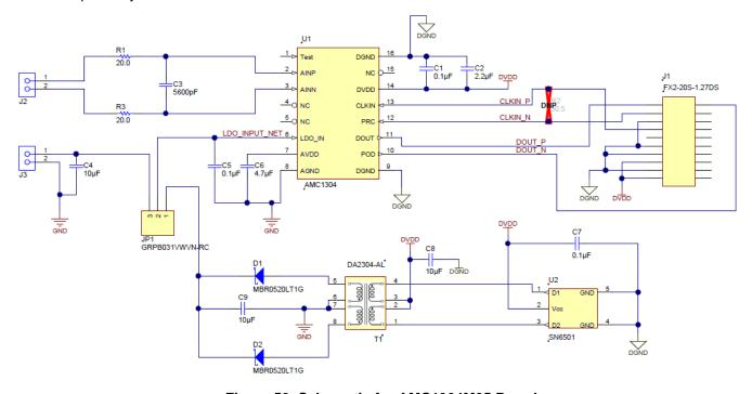
Figure 50. Schematic for AMC1304M25 Board
