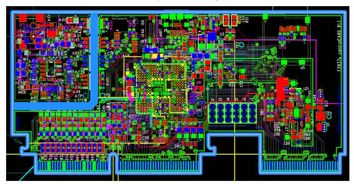
Figure 24. TMS320F28377D Control Card PCB Layout
