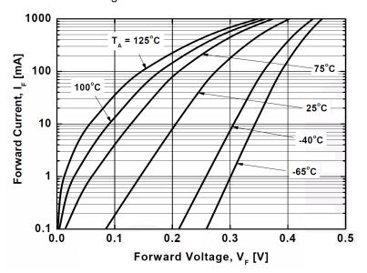
Figure 18. Forward Voltage of the Rectifier Diode
