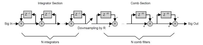
Figure 7. CIC Filter Structure
