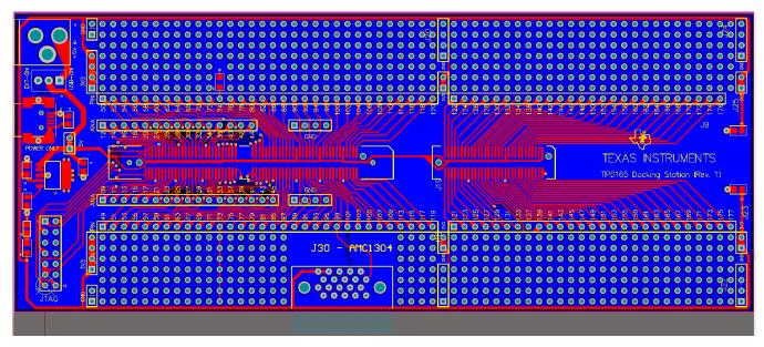
Figure 25. Docking Station PCB Layout
