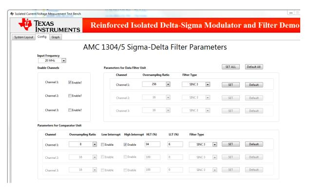
Figure 31. Threshold Settings for Over-current Detection
