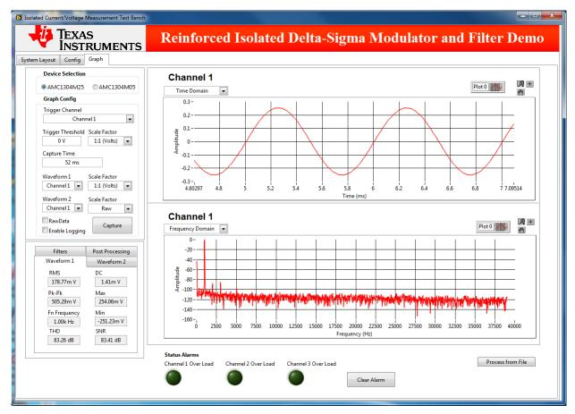
Figure 29. Measured AC Performance
