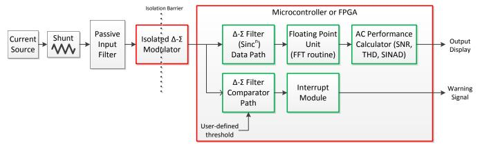
Figure 2. Data Acquisition System Using Isolated Delta-Sigma Modulator
