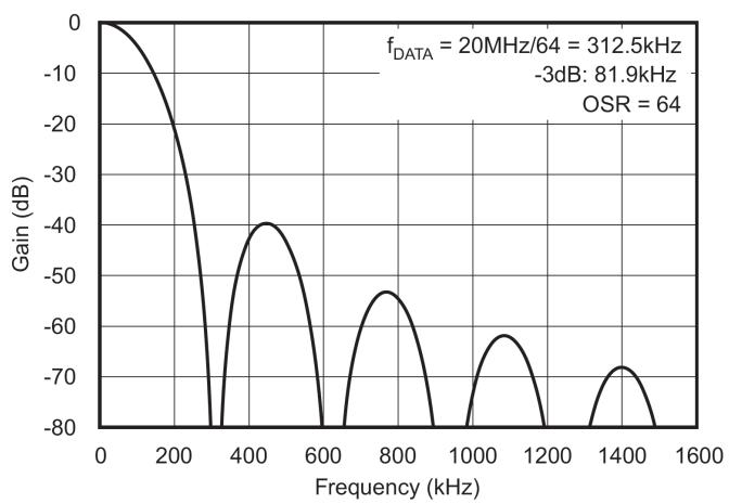
Figure 10. Frequency Response of Sinc3 Filter - Magnitude vs. Frequency
