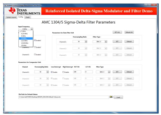
Figure 36. GUI - Frequency Selection - Config Tab
