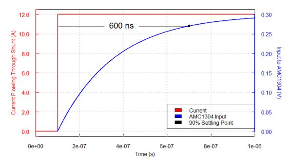
Figure 12. Typical Step Response of RC Passive Filter
