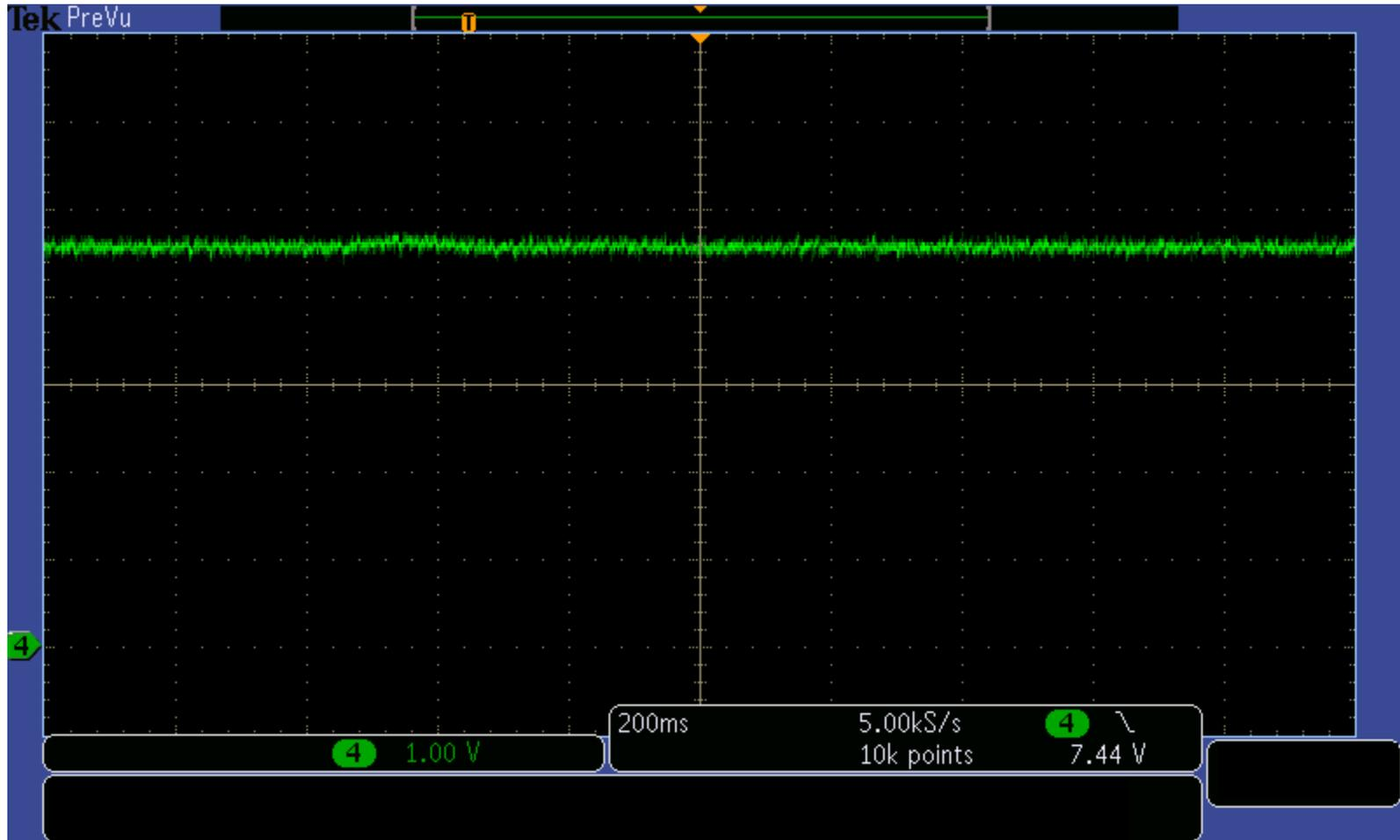
Again, the waveform amplitude represents 2054 RPM. During the first 500ms, a 90 mNm load was driven, and then there was a step-change in load to 22.8 mNm. The speed overshoot was about 1.5%.
