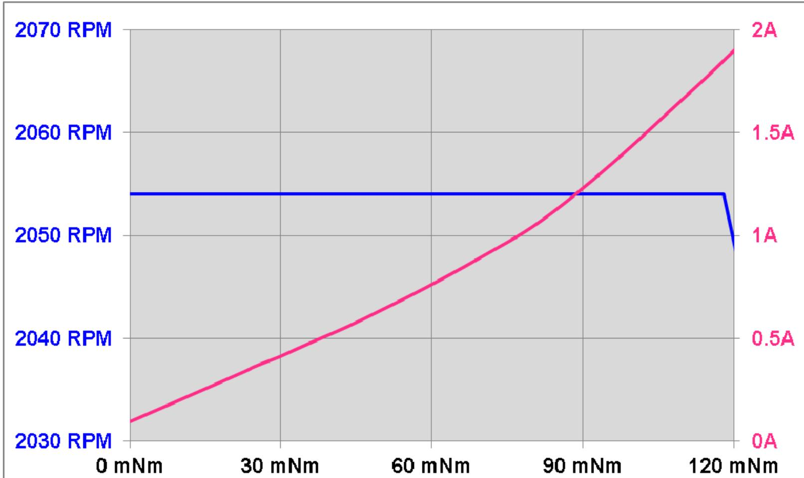
Most BLDC motors do not have closed-loop speed control, so RPM will decrease unpredictably as torque increases. But the DRV8308 maintains a precise RPM. The operating torque range of this design is 0 to 118 mNm (16.7 oz-in), and maximum motor power is 25W.
