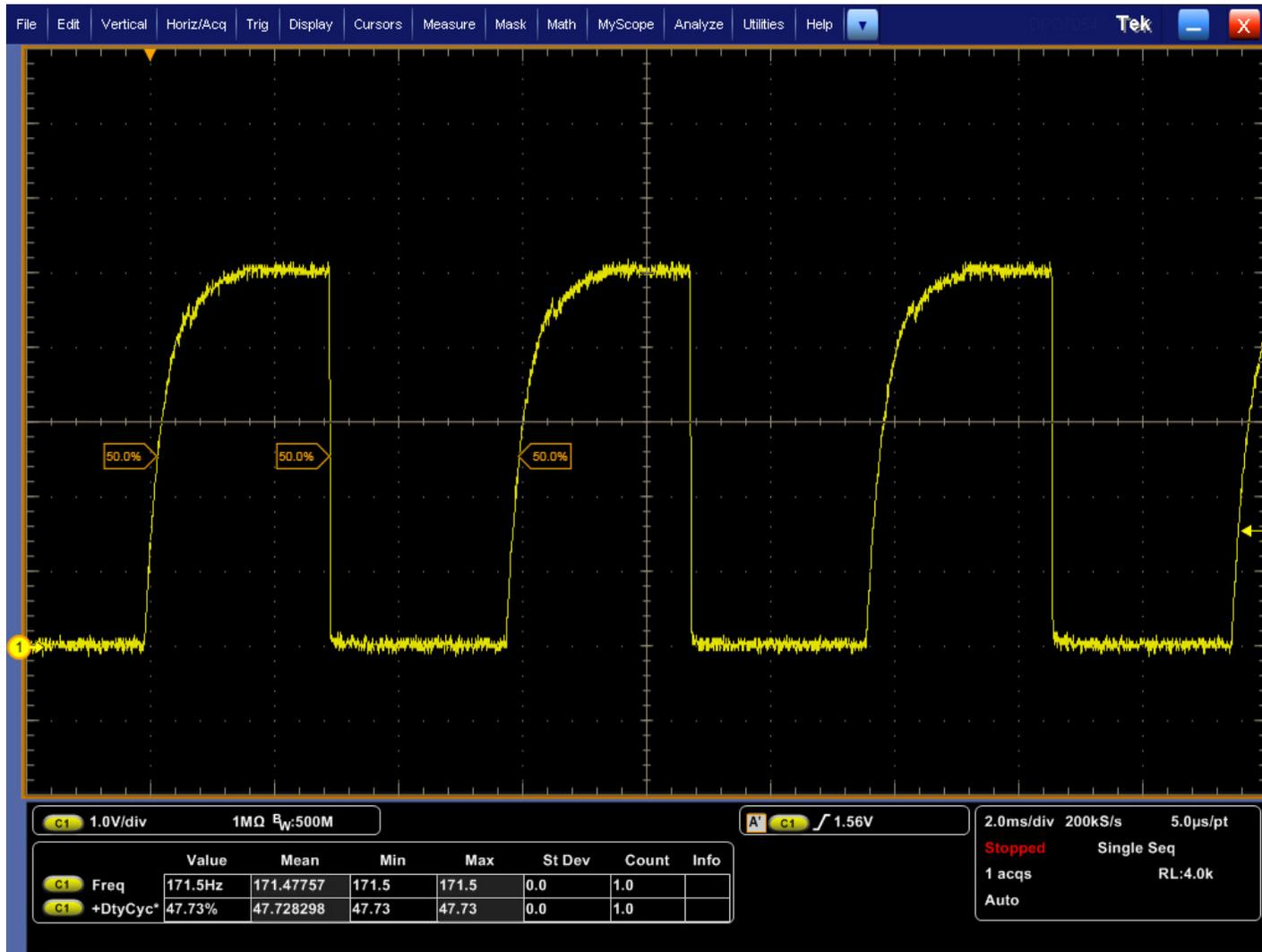
The motor has 10 permanent magnet poles, so there are 5 Hall cycles per revolution.  $171\text{Hz} / 5 * 60 = 2054\text{ RPM}$ .
