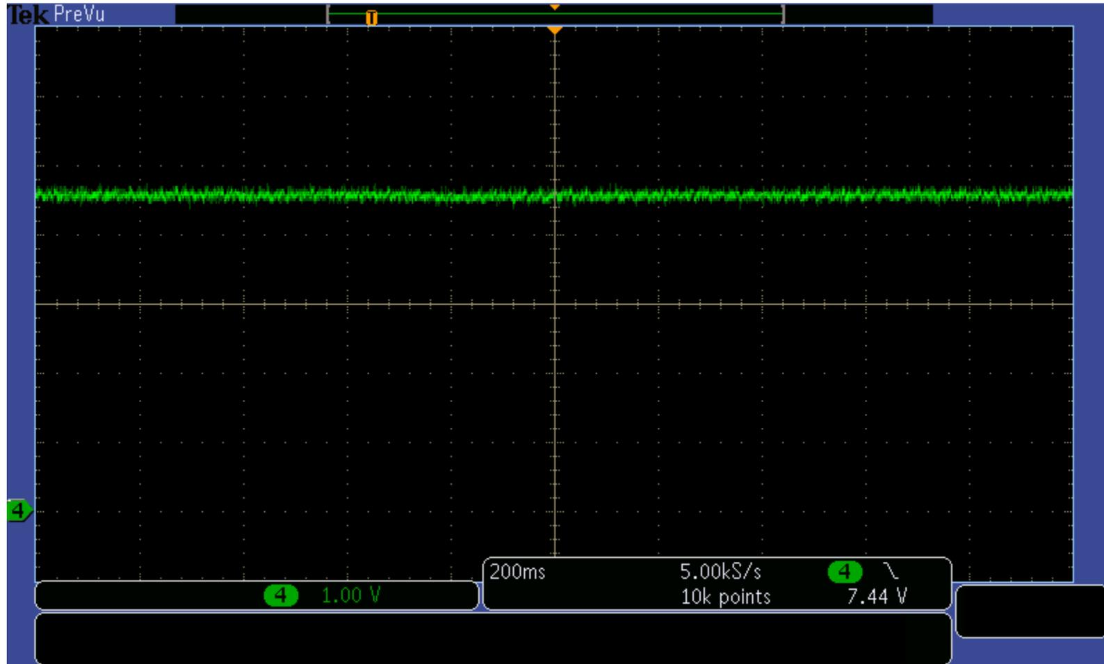
The waveform amplitude represents 2054 RPM. During the first 750ms, a 22.8 mNm load was driven, and then there was a step-change in load to 90 mNm. The DRV8308 closed-loop control compensated very effectively.
