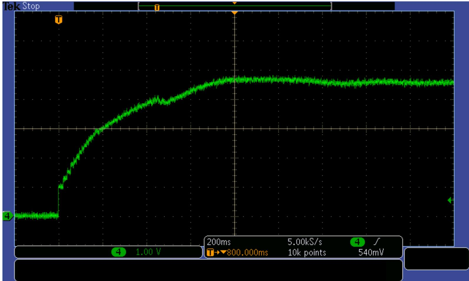
Again, motor speed was measured from the frequency of one Hall signal, and converted to this an analog waveform. Spin-up time was 680ms. The steady-state value represents 2054 RPM.
