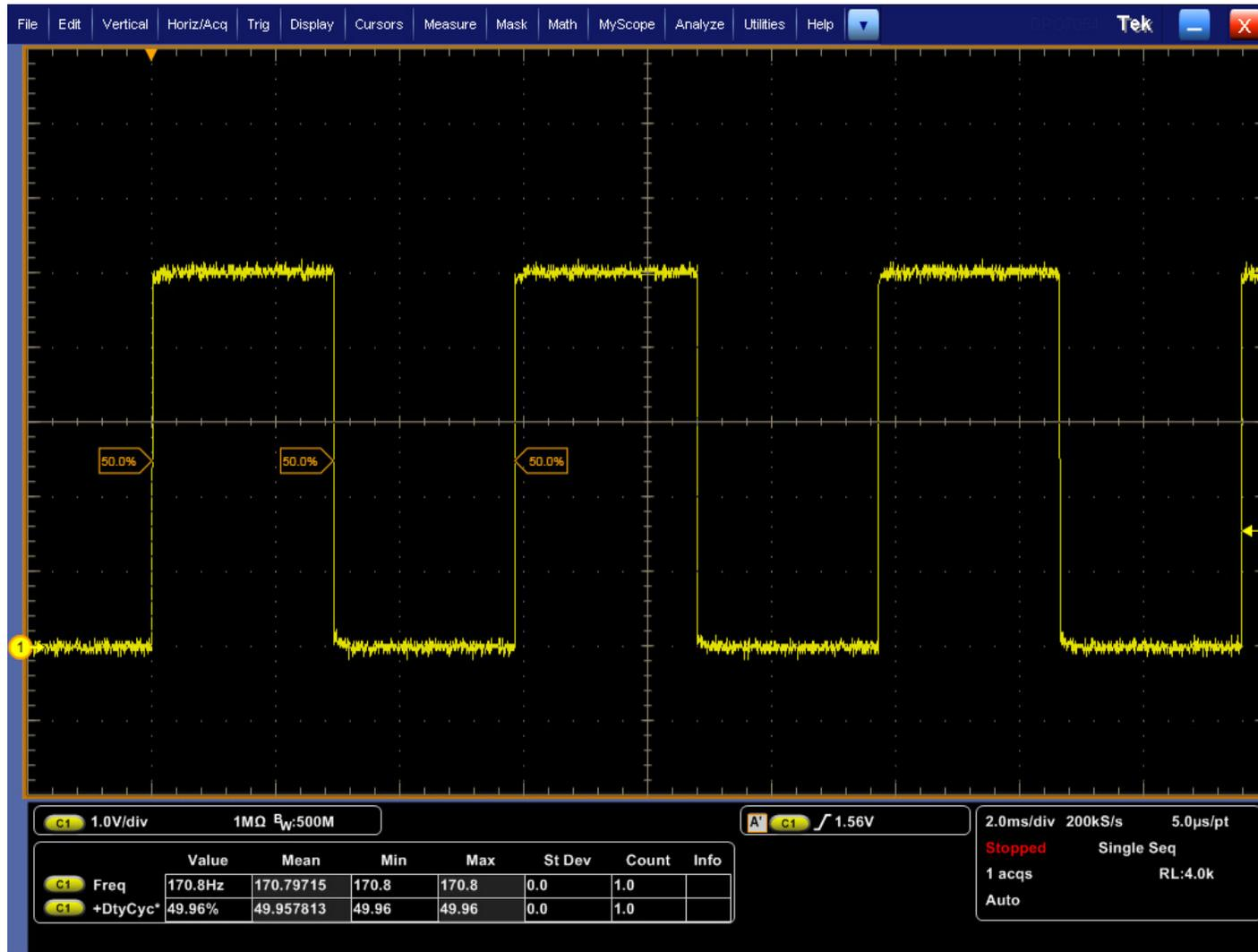
This clock is applied to DRV8308 pin “CLKIN”. The device matches the frequency of Hall U with the frequency of this reference clock.
