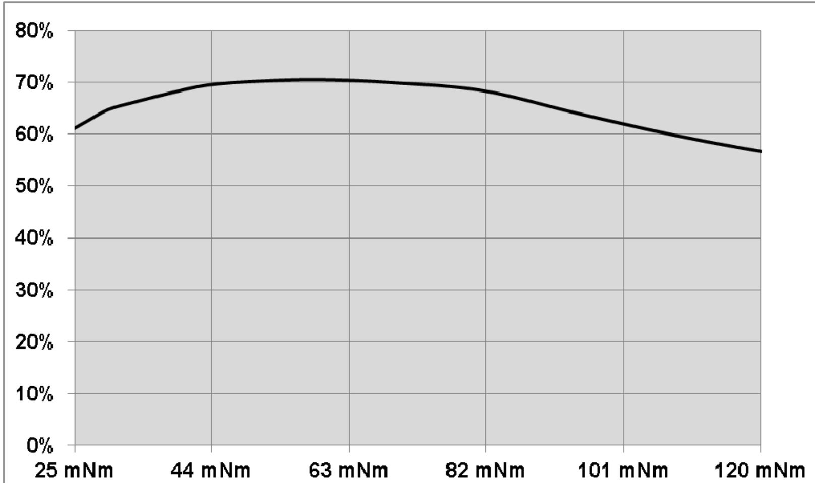
Power Efficiency = Motor Power / Supply Power = (Torque \* Speed) / (Voltage \* Current).
