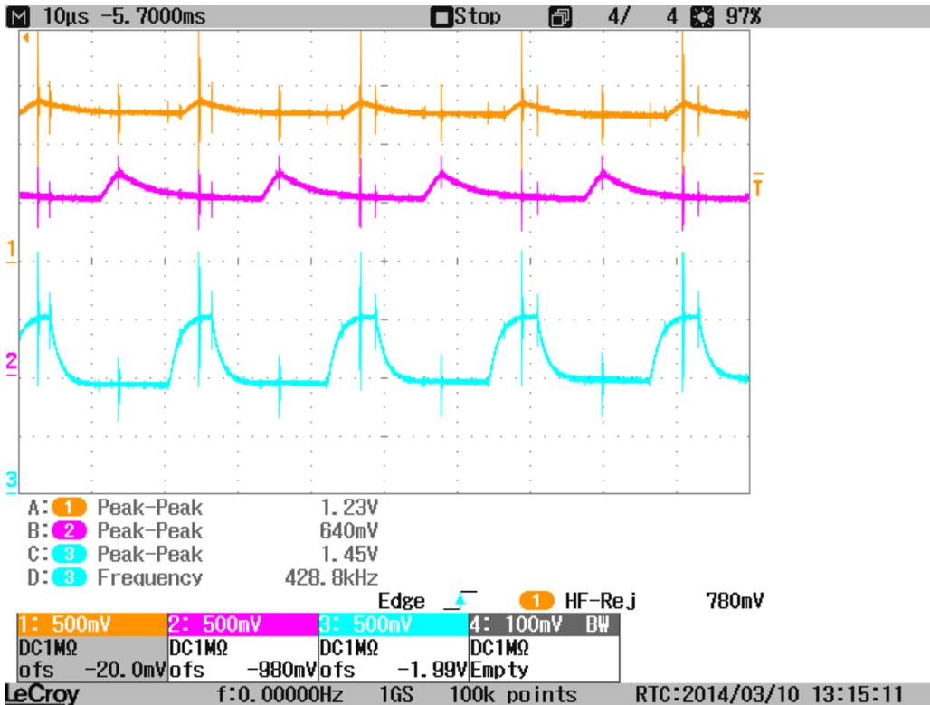
Figure 20 Detail of motor current sense signals
