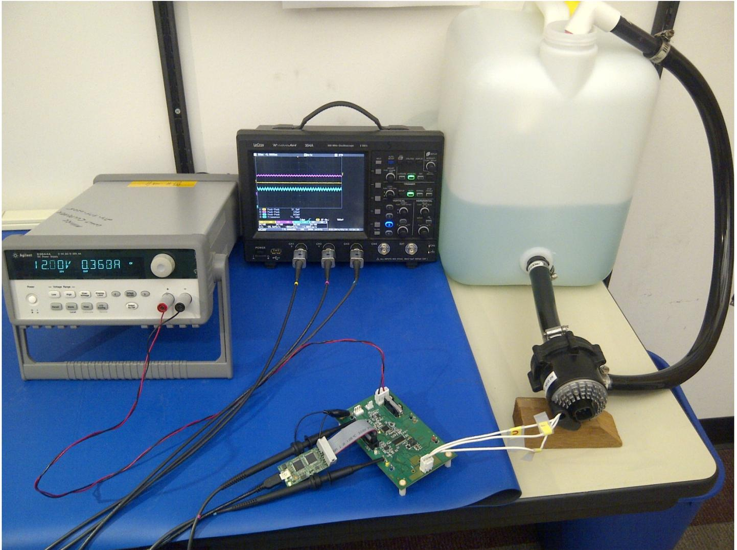
Figure 13 Test set-up with Cooper Standard 50W water pump
