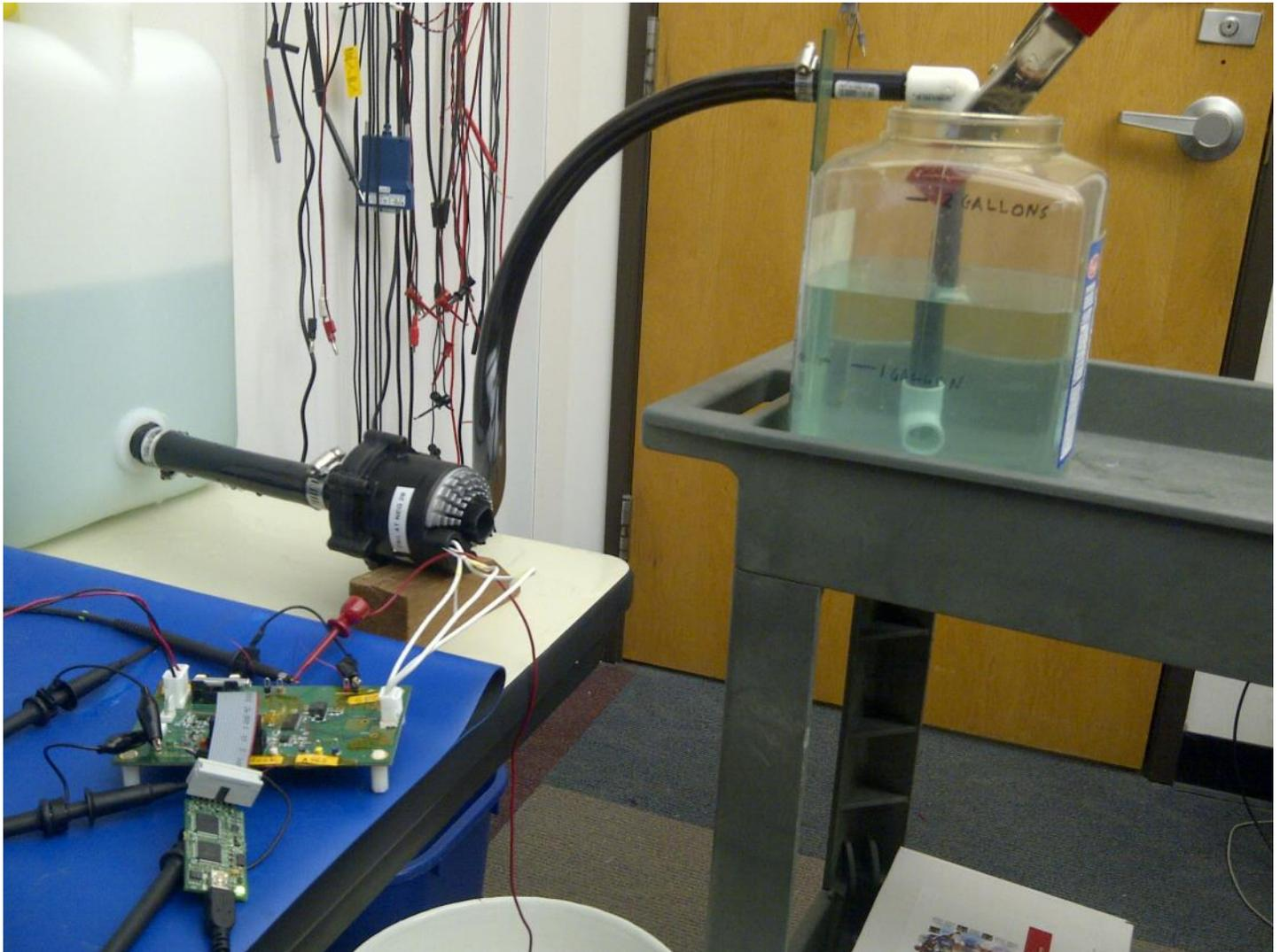
Figure 16 Flow rate measurement set-up
