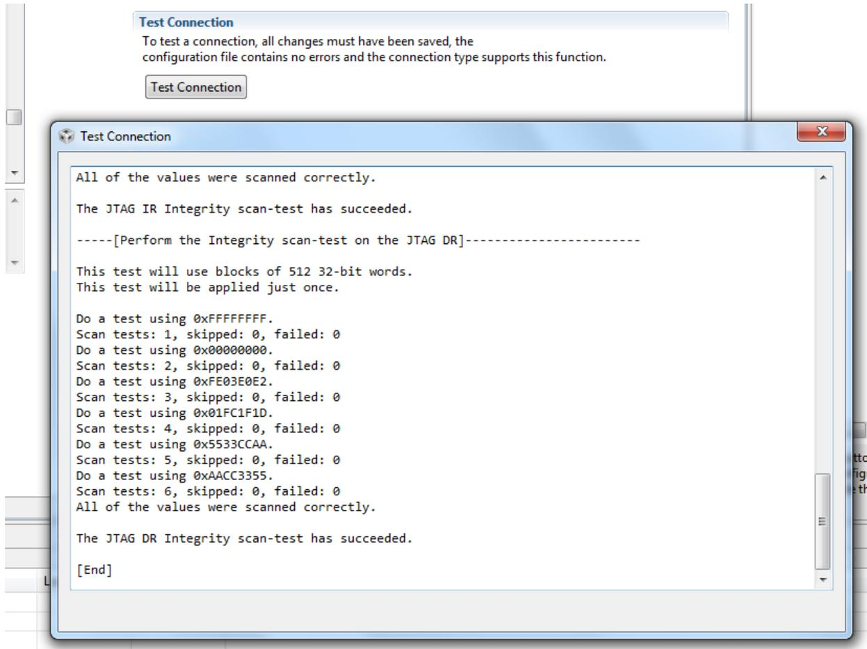
Figure 8 Test connection window after completion of connection test
