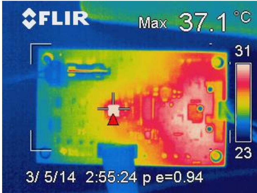
Figure 23 Infrared photo of SAT0042 E4 board in operation (top side)
