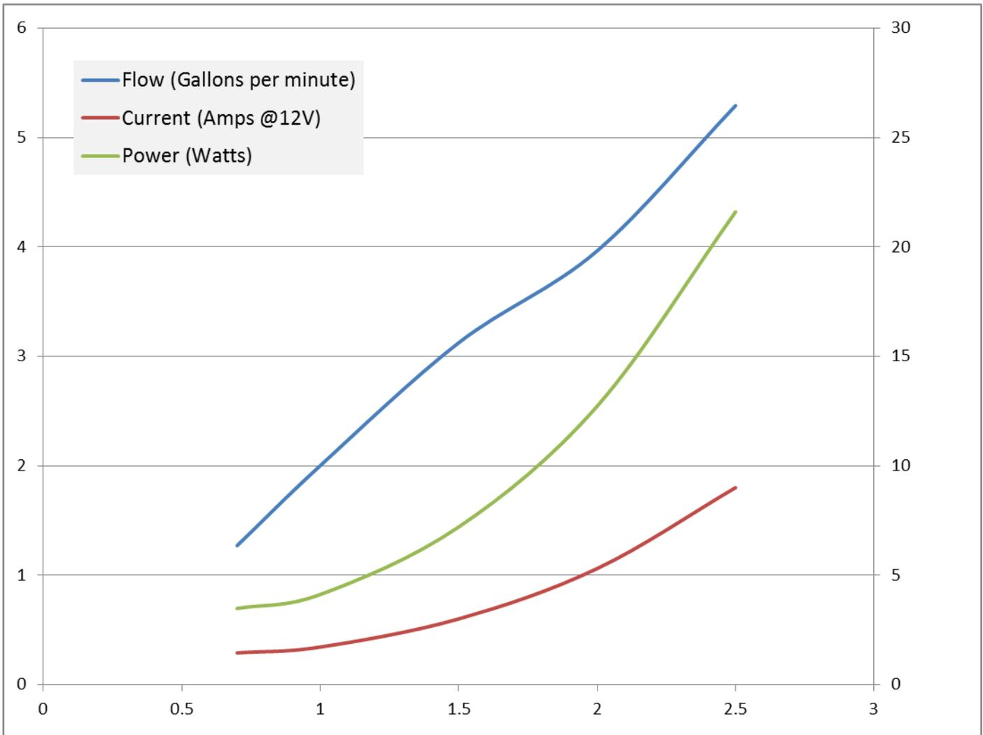
Figure 17 Flow rate measurements with Cooper Standard 50W water pump
