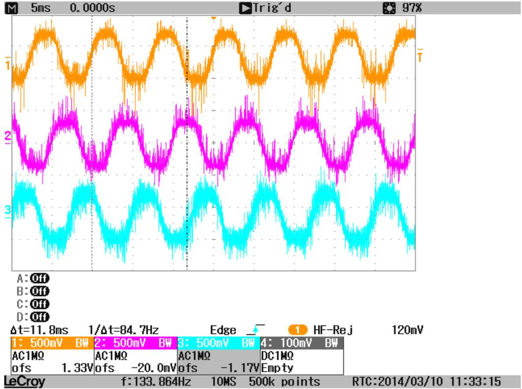
Figure 21 Three-phase motor voltages after filtering and scaling
