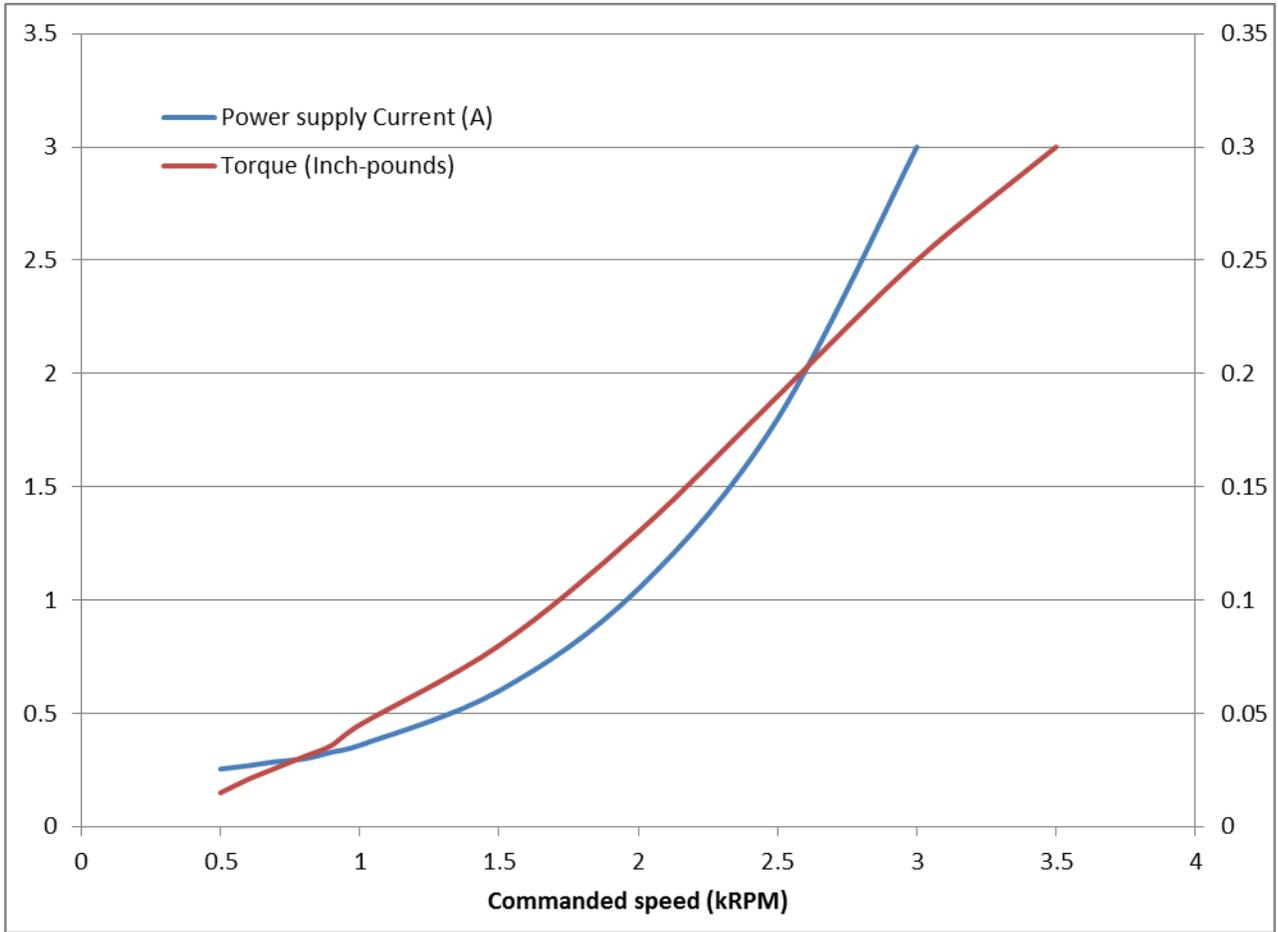
Figure 14 Power and torque as a function of motor speed
