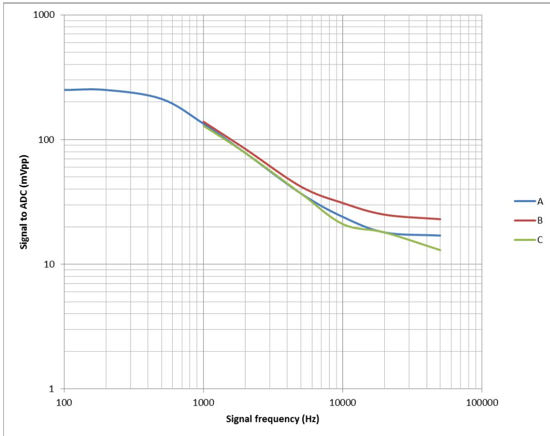
Figure 4 Frequency response of motor phase voltage filters
