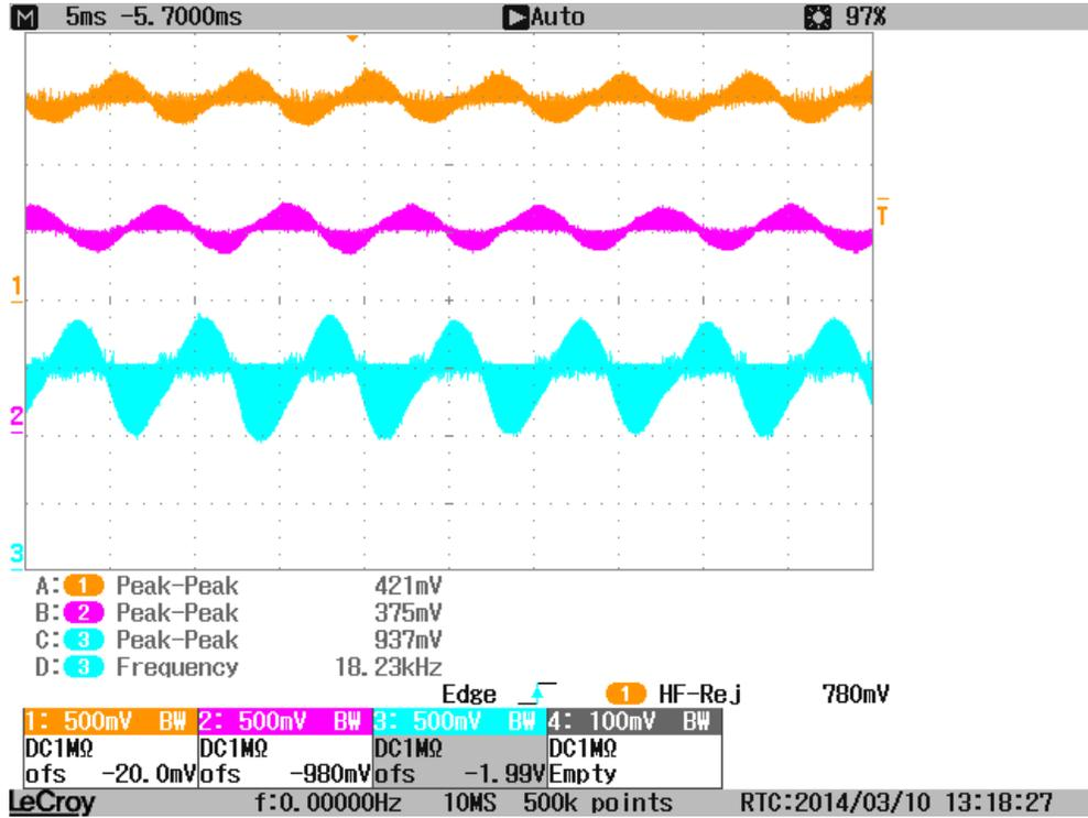
Figure 19 Motor current sense signals showing sinusoidal envelope
