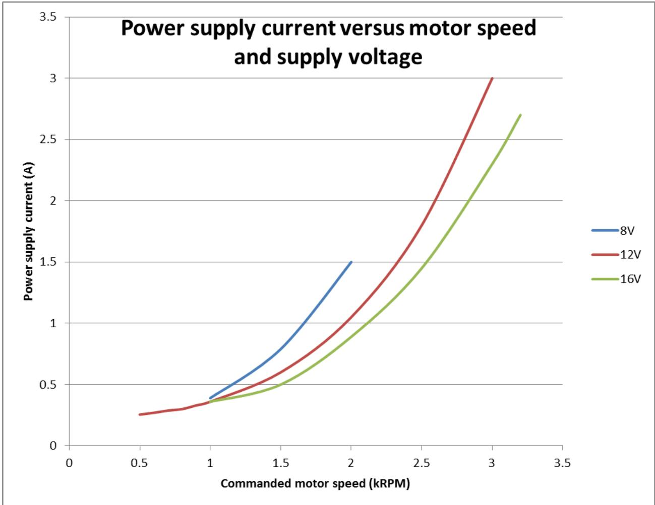
Figure 15 Power supply current versus supply voltage and motor speed
