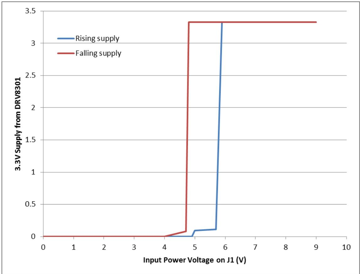
Figure 18 Operational range is indicated by 3.3V power supply versus input supply
