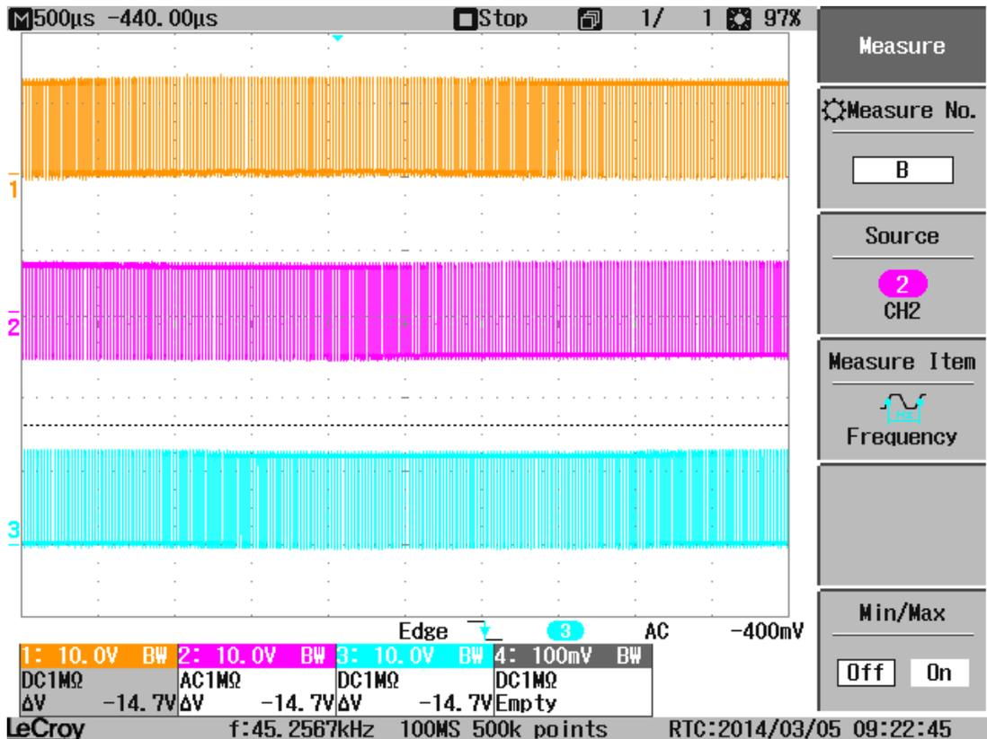
Figure 22 Three motor phase voltage signals - direct to motor windings
