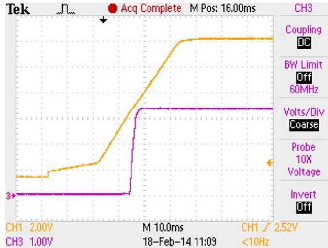
Figure 2 Top (orange) trace is 12V from bench supply, bottom (pink) trace is 3.3V on board
