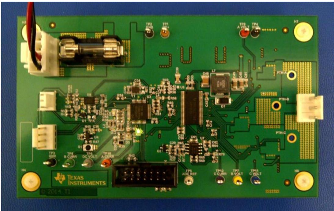
Figure 1 SAT0042 E4 board with 12V power applied and LED D6 illuminated (center)
