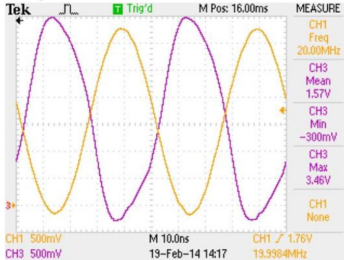
Figure 3 Scope traces of 20 MHz clock signal
