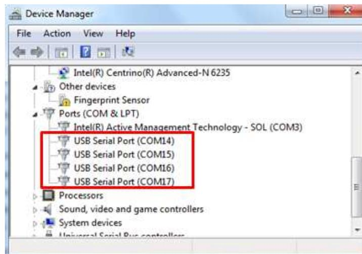
Figure 14. Device Manager Shows Four Ports
