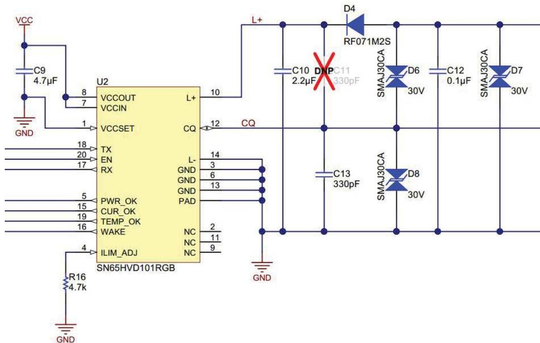
**Figure 18. Power and Data Interface with Protection Circuitry**
