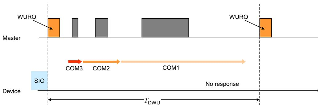
Figure 10. Example of Failed Transmission Rate Negotiation
