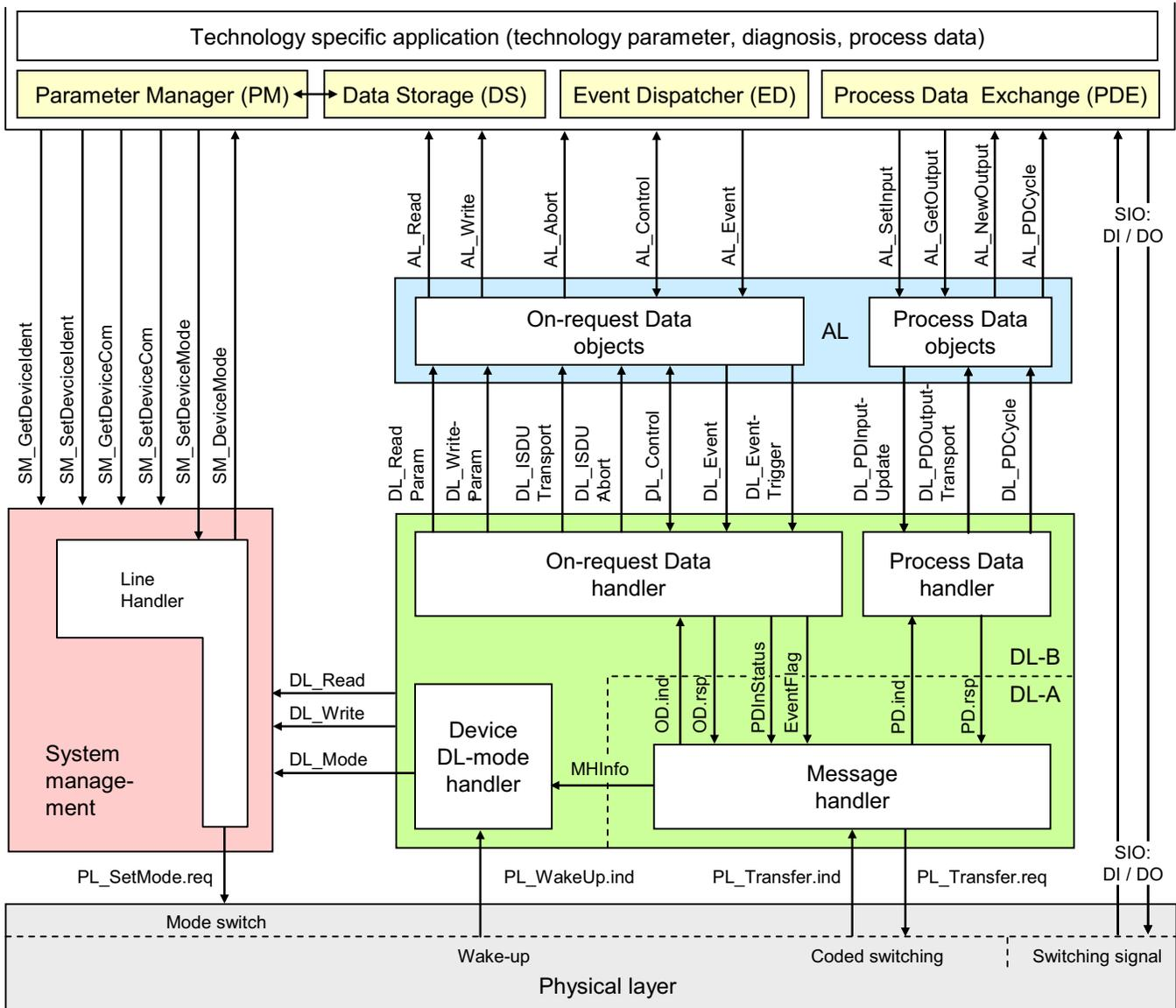
Figure 11. Structure and Services of the Device Application Layer
