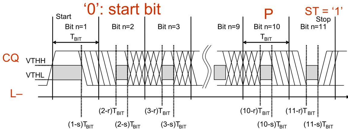
Figure 7. Eye Diagram for the Correct Detection of a UART Frame
