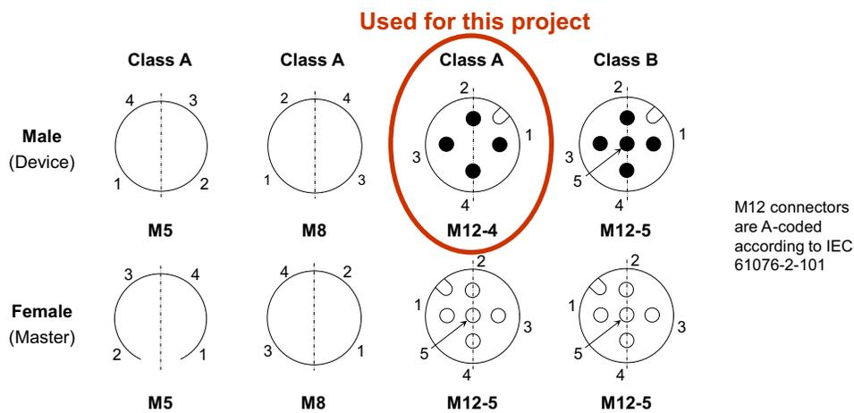
**Figure 3. M12-4 Pin Layout and Assignments**
