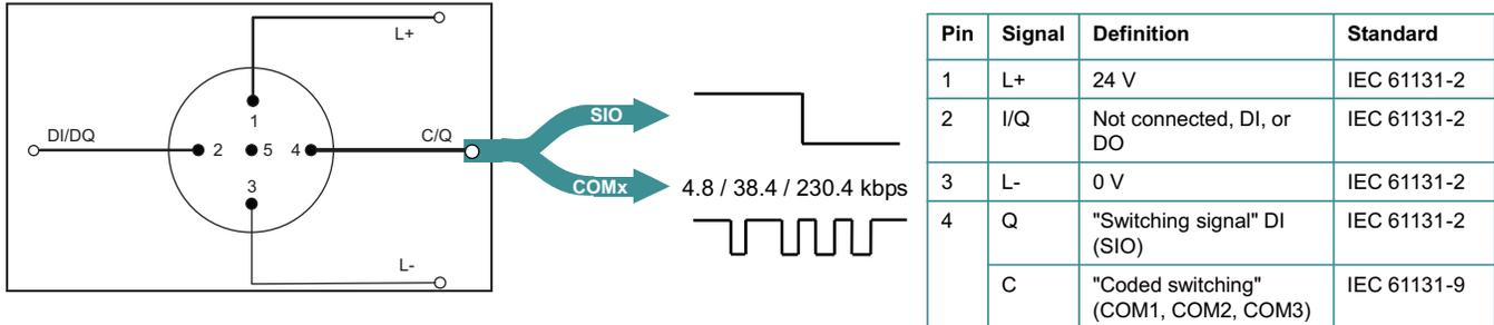
Figure 4. SIO versus SDCI (or IEC61131-9 versus IEC61131-2)
