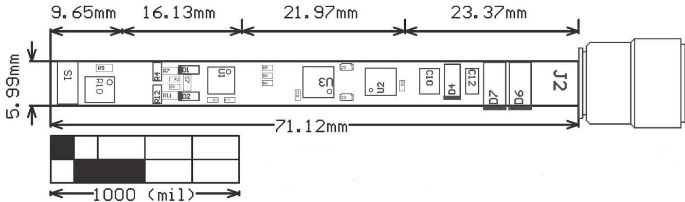
Figure 16. Full System PCB Dimensions
