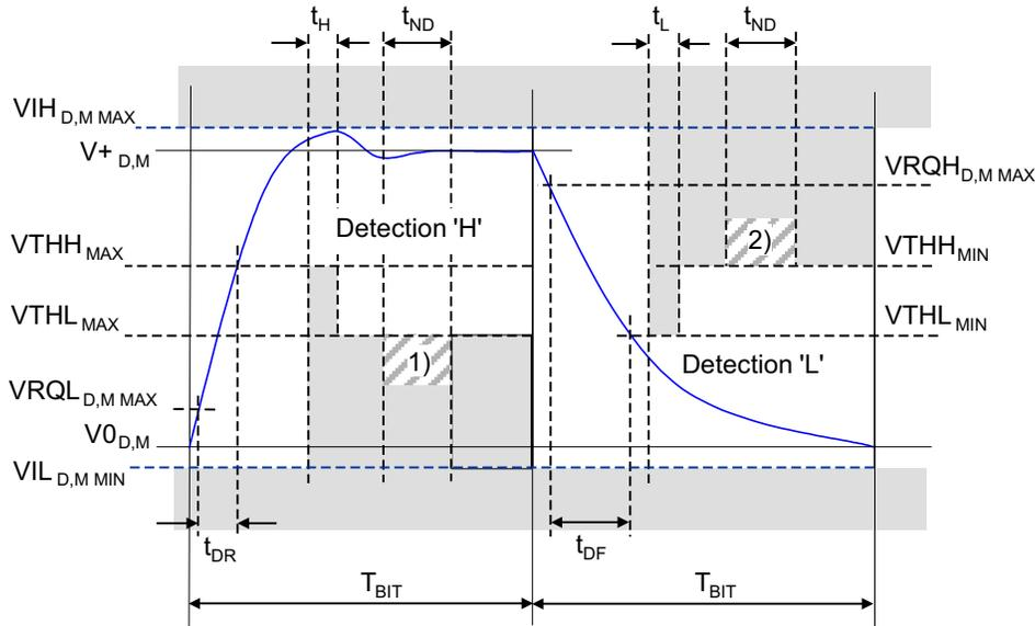
In the figure, 1) = no detection 'L'; and 2) = no detection 'H'
