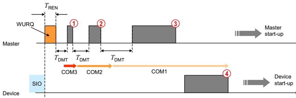
Figure 9. Example of Successful Transmission Rate Negotiation
