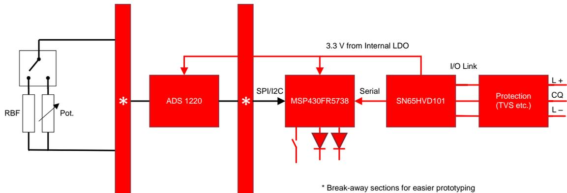
**Figure 1. IO-Link Transmitter Overview (System Block Diagram)**
