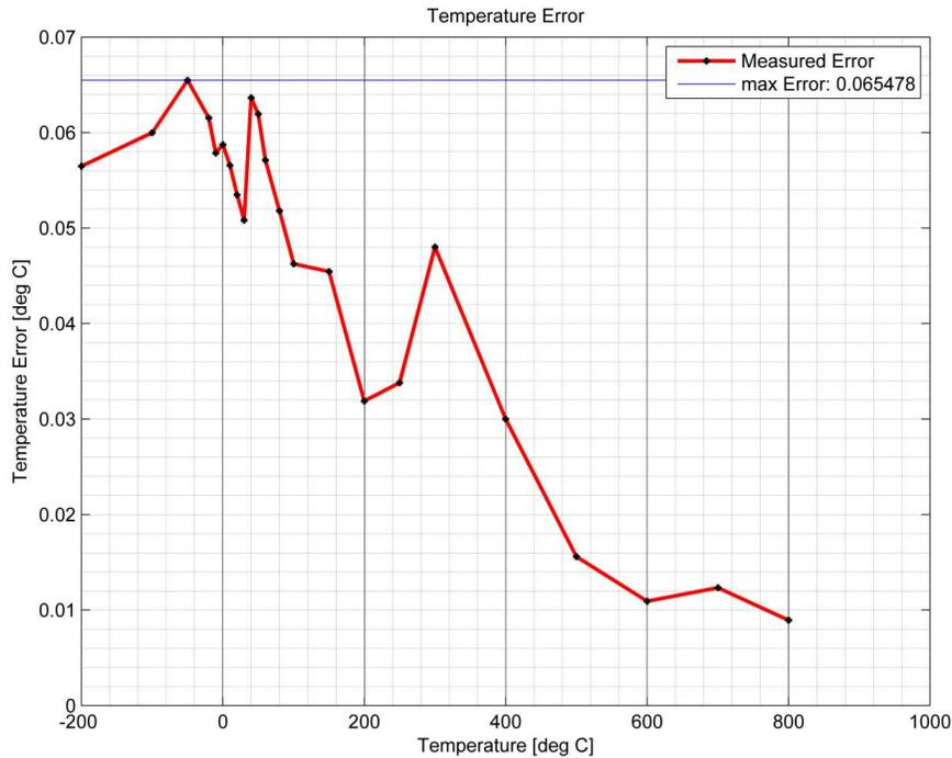
**Figure 25. Temperature Error Between the Mean of 1024 Measured Data Points and the PT100-Simulator's Provided Temperatures**
