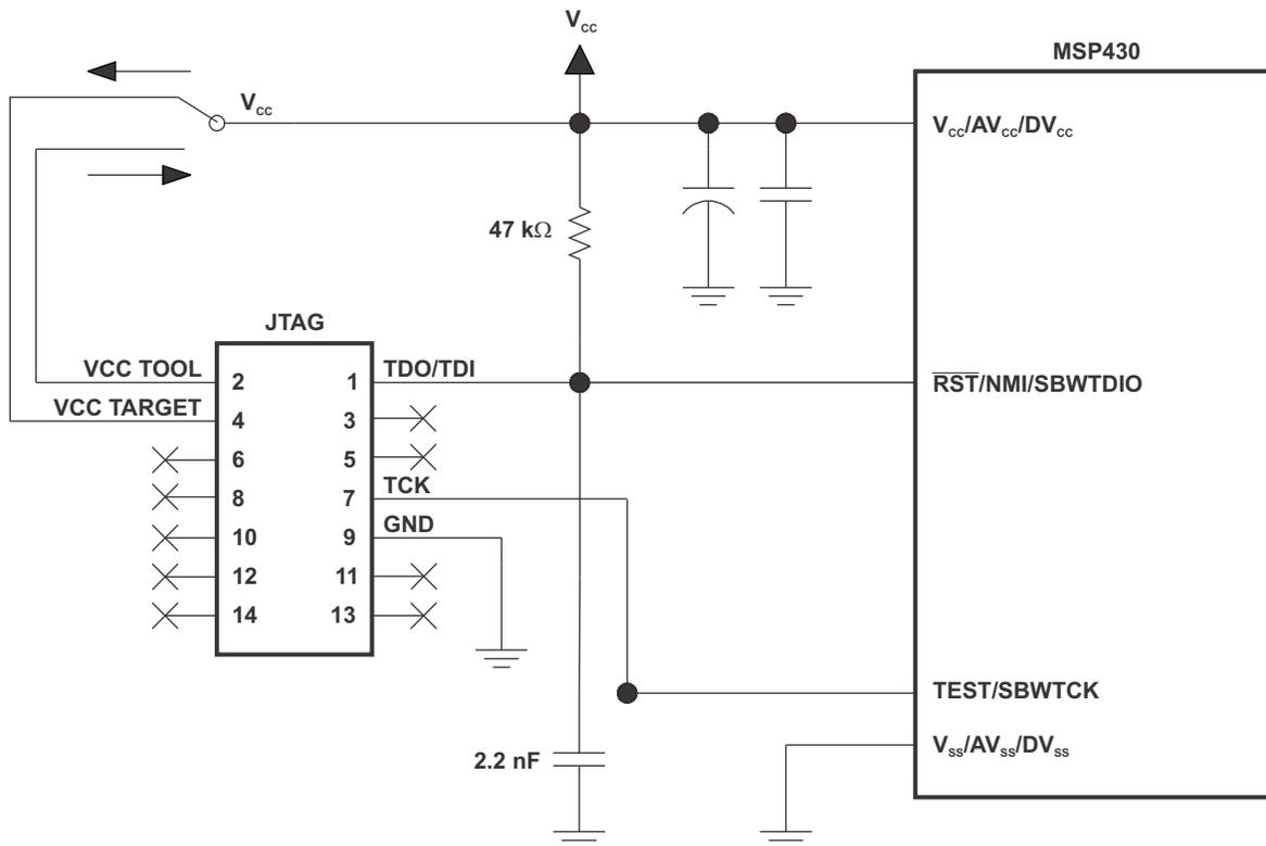
**Figure 22. Signal Connections for 2-Wire JTAG Communication (Spy-Bi-Wire)
