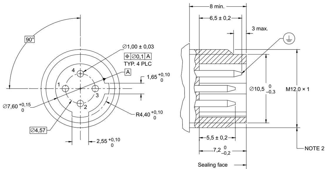
NOTE 1 Pin identification numbering is not necessary.
