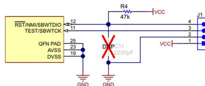
**Figure 21. JTAG Connection (Pin 1 is Marked on PCB)**
