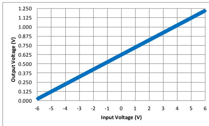
**Figure 1: Measured Transfer Function Over the Full  $\pm 6$  V Input Range**
