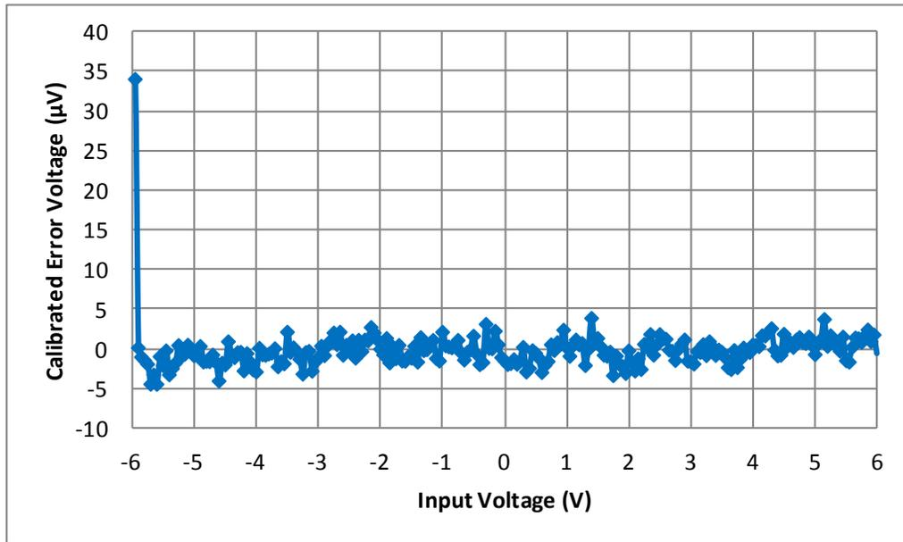
Figure 15. Calibrated Output Error with ±6V Input
