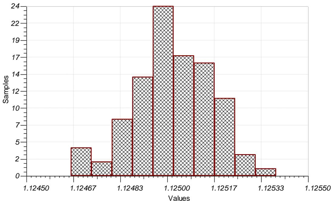
**Figure 10: Circuit Output Variation with a Full-Scale +5 V dc Input**
