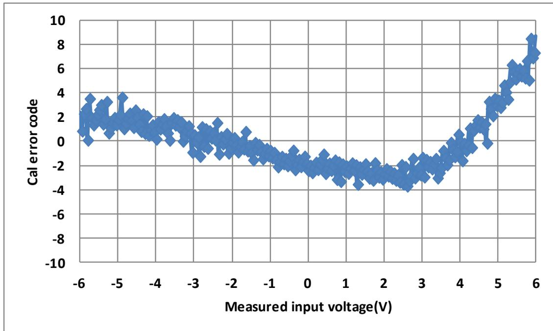
Figure 24: Calibrated Error Codes vs. Input Voltage
