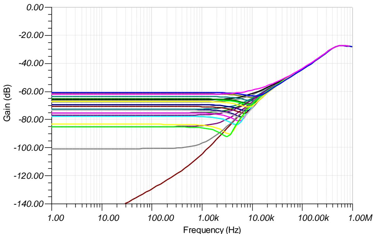
**Figure 11: Circuit CMRR Variation over Frequency from Resistor Tolerance**
