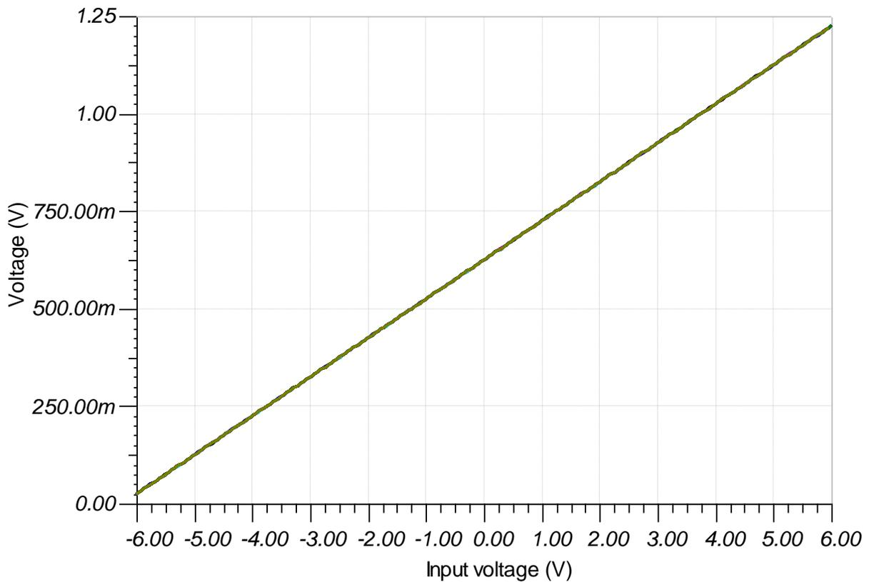
**Figure 18: Histogram Transfer Function Results**
