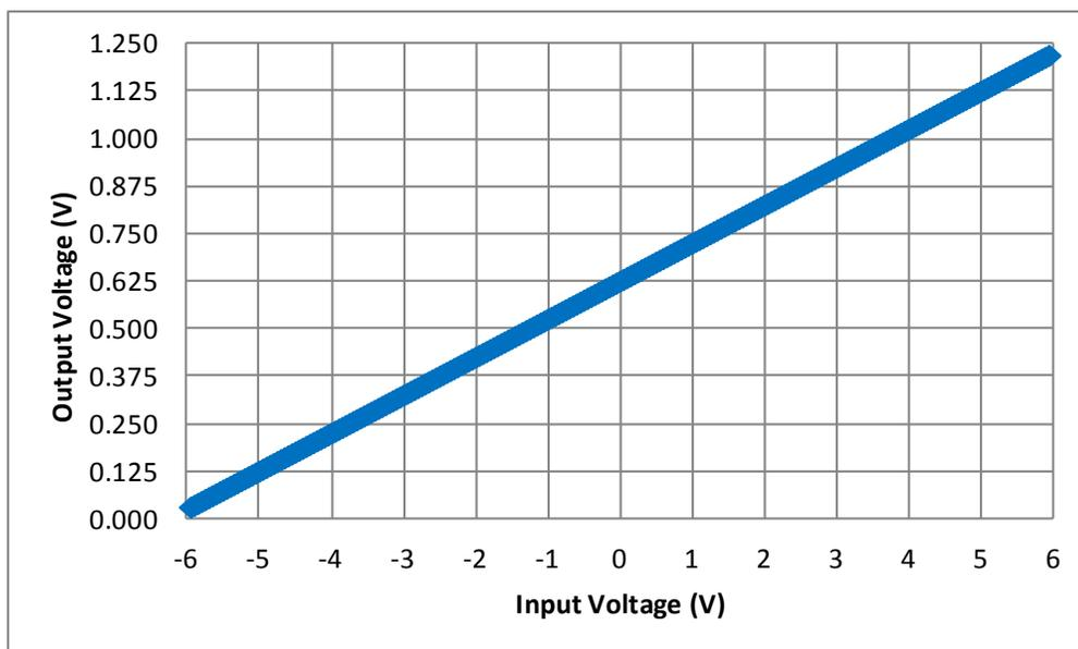
Figure 13. Measured DC Transfer Function with  $\pm 6\text{V}$  Input
