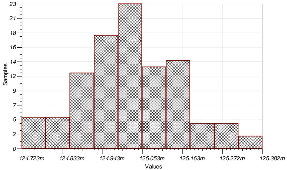
**Figure 19: Circuit Output Variation with a Negative Full-Scale +5 V dc Input**
