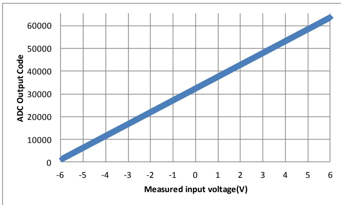
Figure 22: MSP430F2013 Output Code vs. Input Voltage
