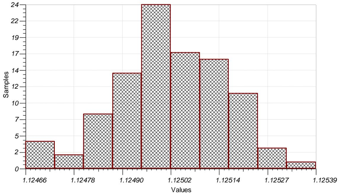
Figure 21: Circuit Output Variation with a Positive Full-Scale +5 V dc Input
