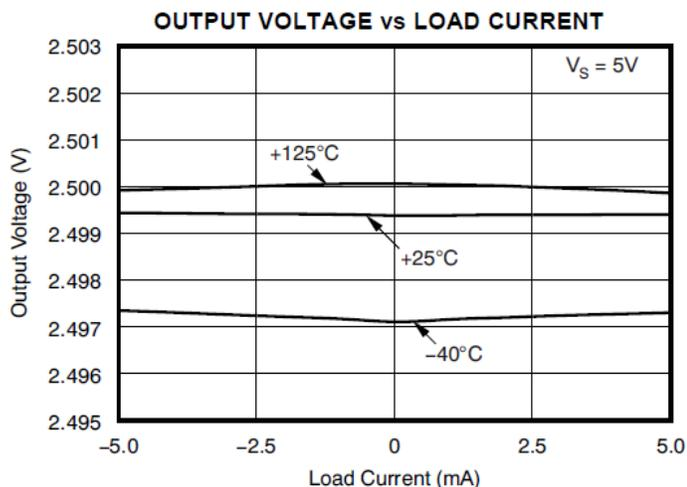
Figure 6: REF33xx Output Voltage vs. Load Current
