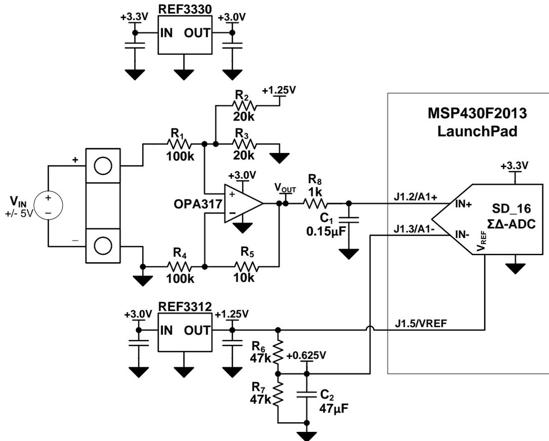
Figure 3: Simplified Circuit schematic
