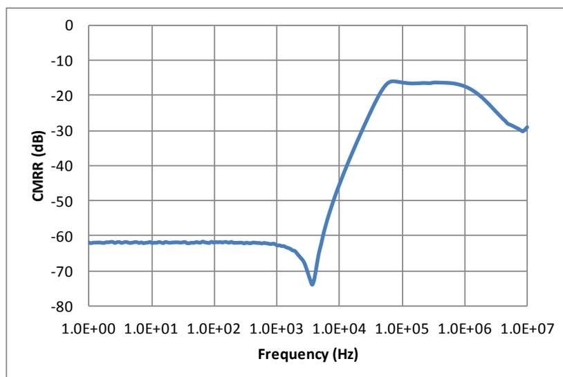
Figure 17. Measured ac CMRR Results
