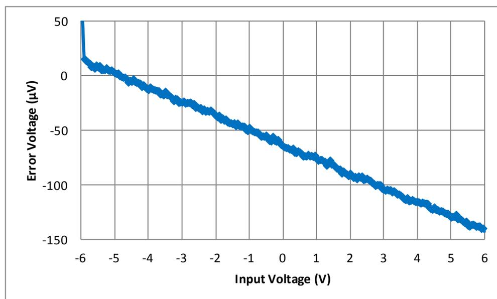
Figure 14. Measured Output Error with  $\pm 6\text{V}$  Input
