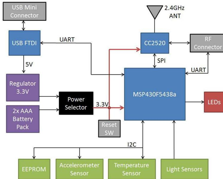
Figure 1. RF Sensor Node System Block Diagram
