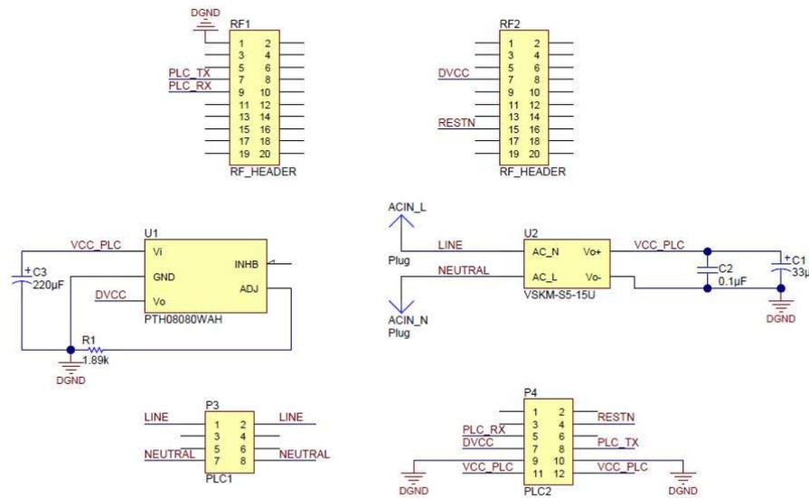
Figure 21. Interface Card Schematic
