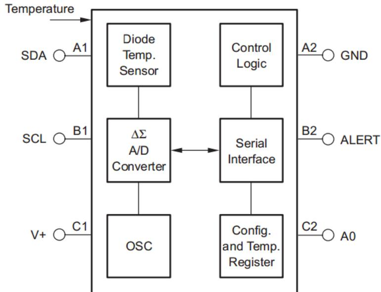
Figure 5. TMP106 Functional Diagram
