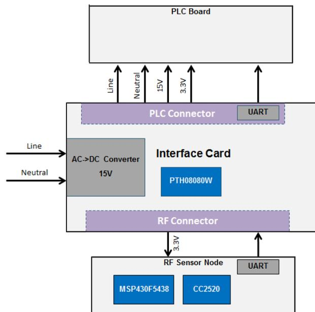
Figure 2. PLC Board, RF Sensor Node, and Interface Board Functional Block Diagram
