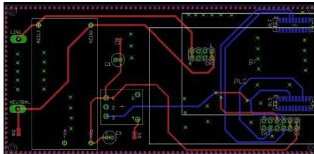
Figure 24. RF Sensor Node Layout
