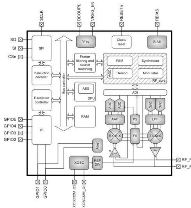
Figure 3. CC2520 Functional Diagram
