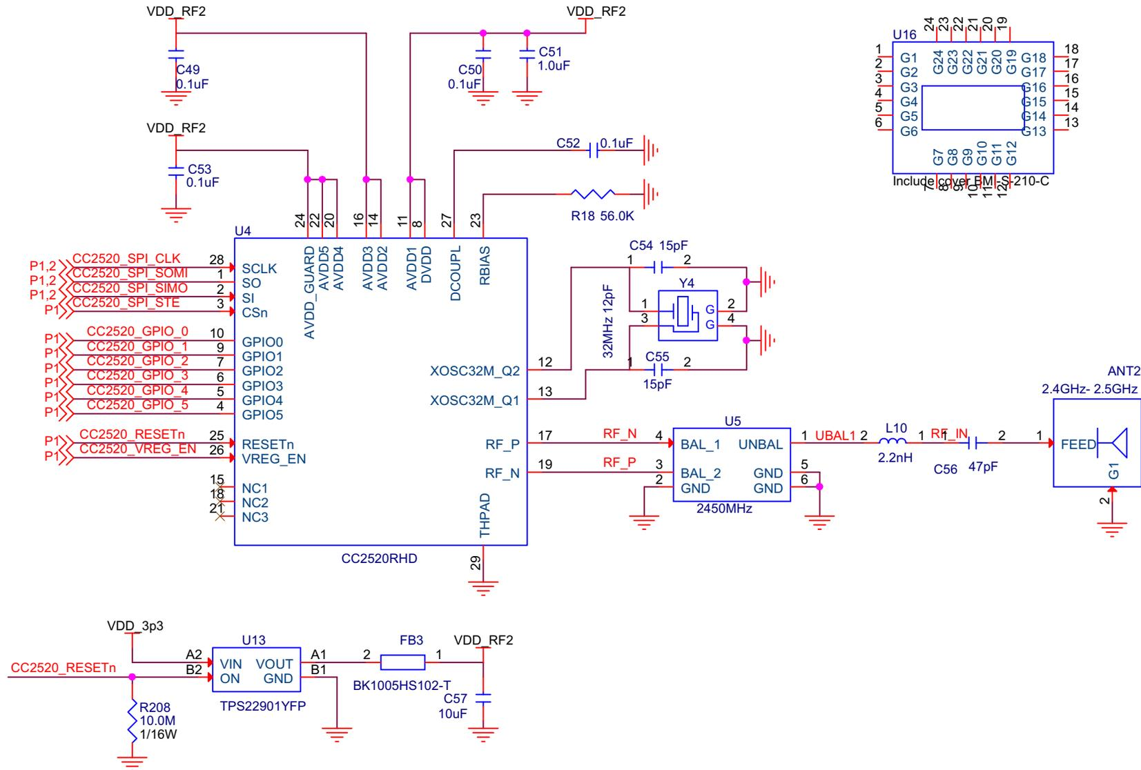
Figure 15. CC2520 Radio Schematic
