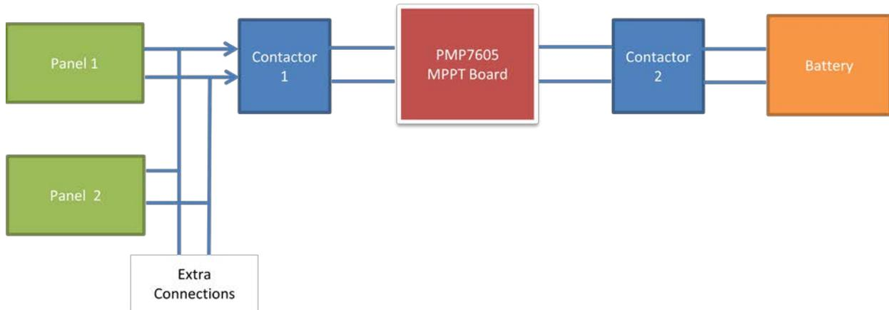
This test was done with an earlier similar design PMP7605. Setup Explains the Power flow from Panel to Battery during MPPT Operation. To connect Panel directly to battery, both contactors were opened and Extra connections were connected directly onto the battery.
