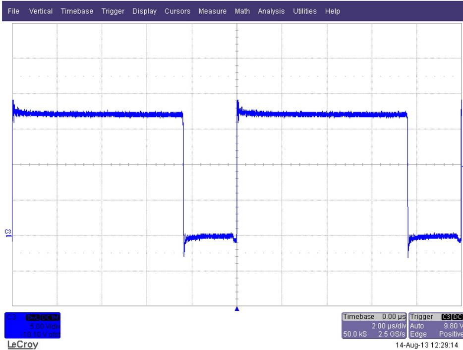
Boost converter switch node at 12LED, 700mA load
