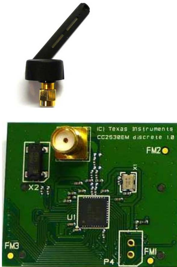
Figure 13. ZigBee Radio
