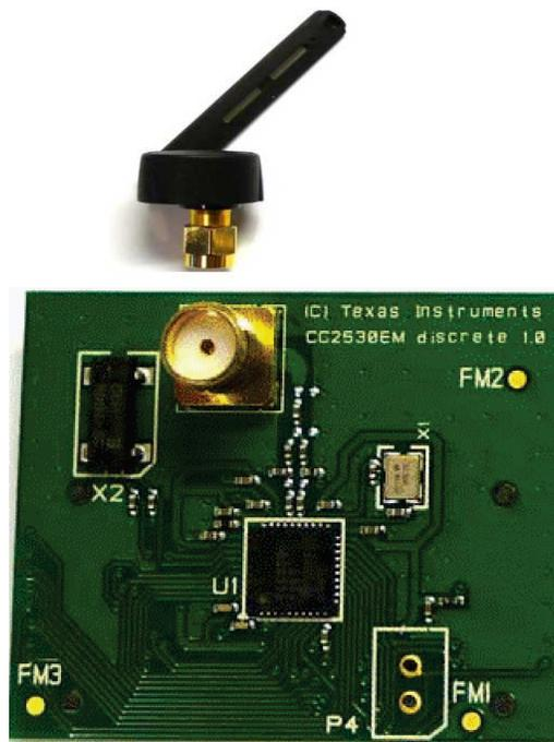
Figure 6. ZigBee Radio
