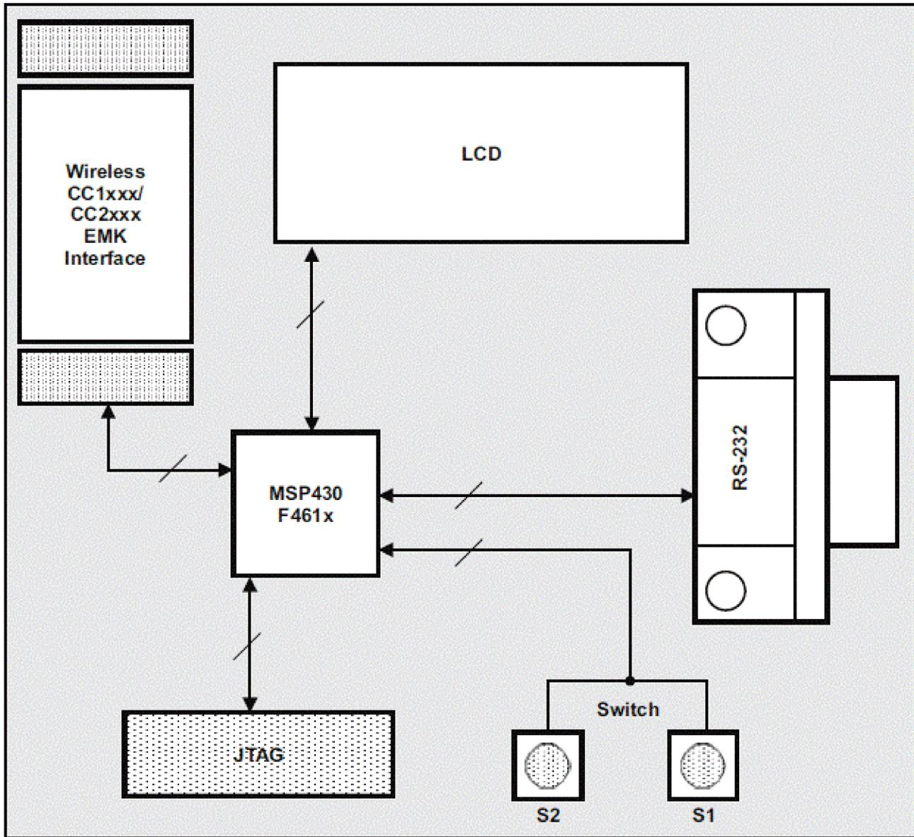
Figure 3. IHD430 Board Block Diagram
