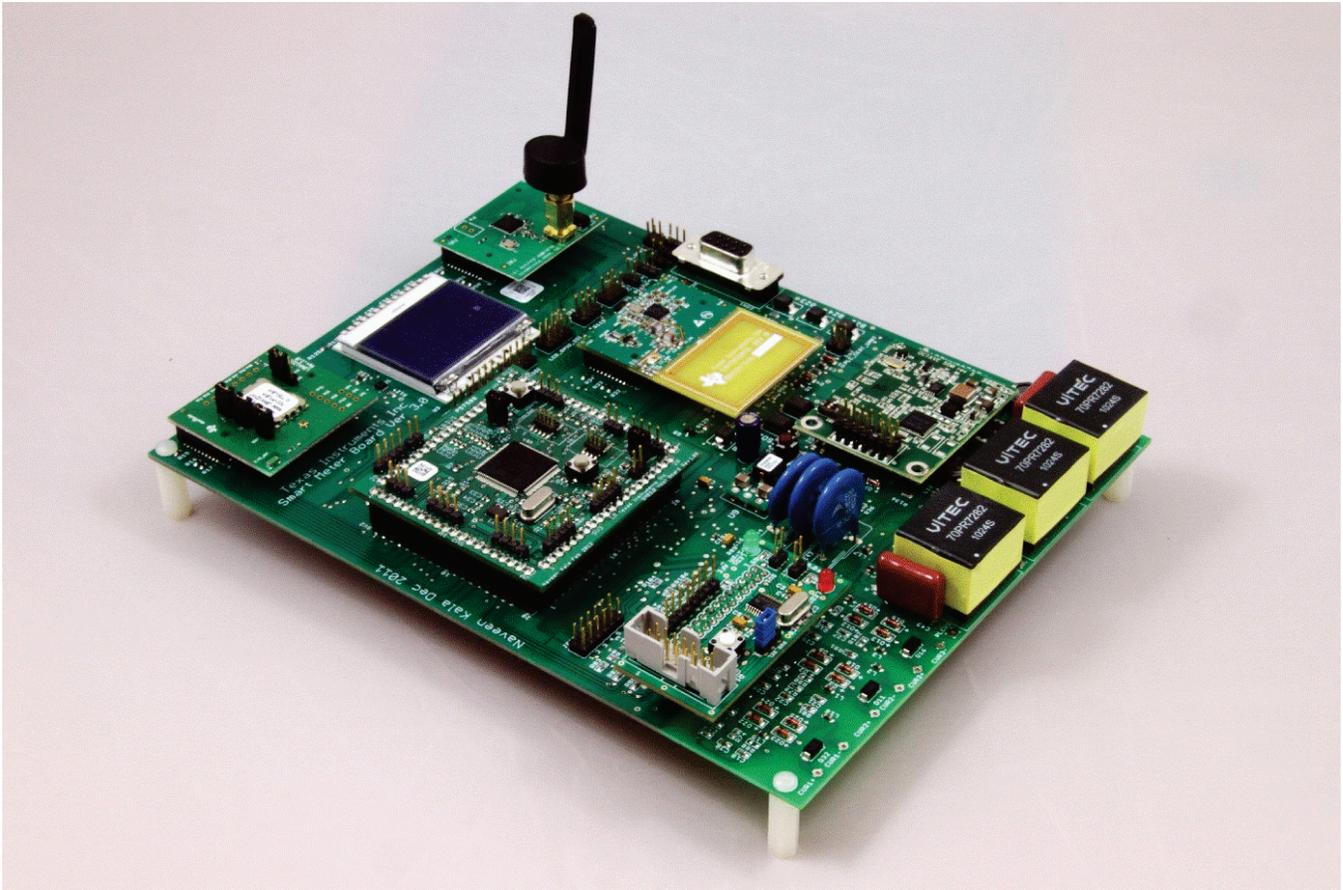
**Figure 1. Smart Meter Board (SMB)**
